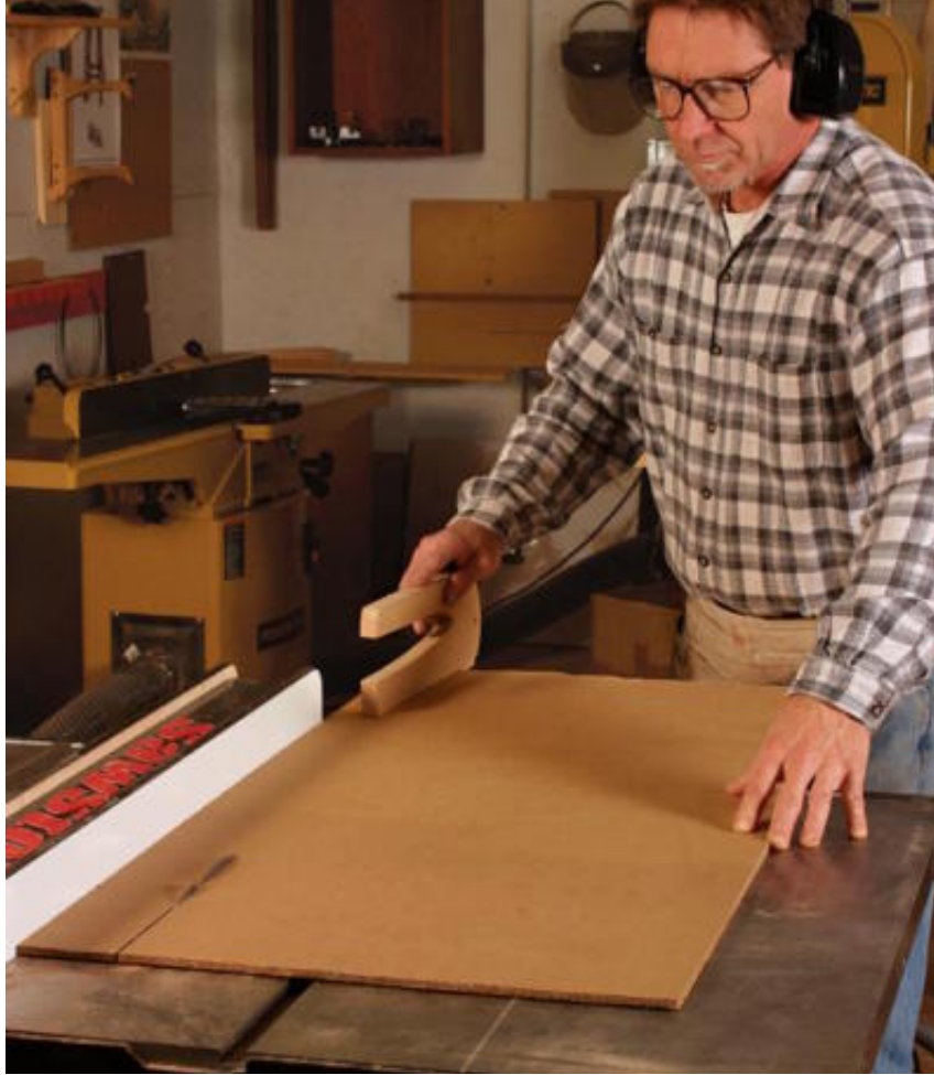
The material cuts easily. Components for a full-scale table model can be made in minutes. Just slice up cardboard parts on the table saw and glue them together.
