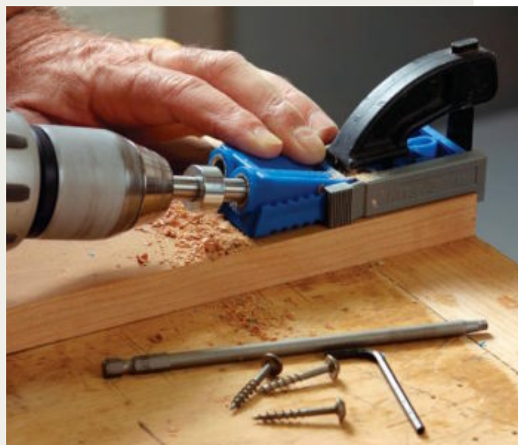
Pocket holes in a jiffy. The R3 jig attaches easily to the workpiece with almost any bar or C-clamp. The lip on the end references the edge of the workpiece.
