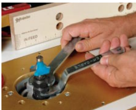
Easiest bit-changing. The Triton (above) has a well-designed spindle lock, and it lifts the collet above the table so you need only one wrench for bit changes. The Porter-Cable (left) is one of several routers that need two wrenches for bit changes; but at least you can do it from above the table.
