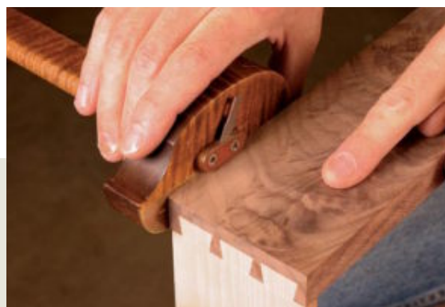
A marking gauge that cuts. This shopmade gauge works like a regular marking gauge, except that it uses the tip of a craft-knife blade as a cutter, allowing it to scribe a deep, clean line.
