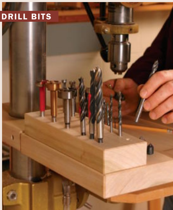
Bit rack clamps directly to drill press. This two-tiered rack easily holds most commonly used bits.
