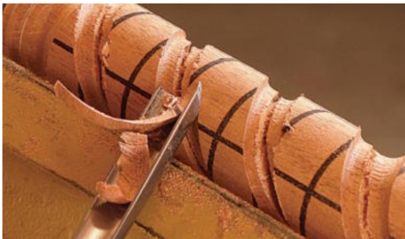
Widen the channel. Come back with a wider gouge to enlarge the channel. Again, always cut on the right side of the kerf. When complete, saw down another \frac{1}{4} in. and repeat the carving with the narrow and wide gouges.
