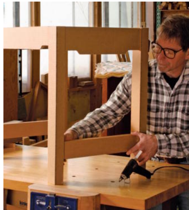
Hot-melt glue works great on cardboard. With the base constructed, it's easy to experiment with a variety of tabletop sizes and designs.
