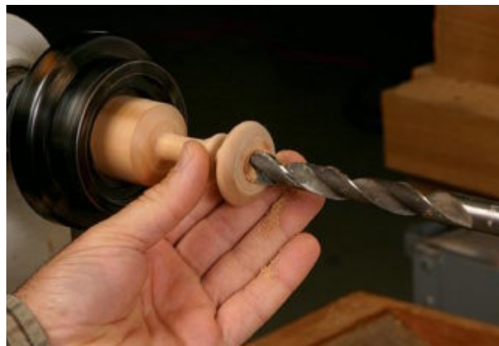
Dead center. Mount a drill bit in the tailstock of a lathe to center a recess for a decorative insert in a turned knob.
