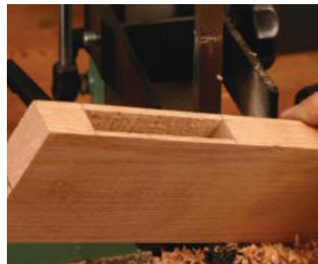
Clean cuts. A hollow-chisel mortiser is designed to make sharp, smooth cuts that need little, if any, handwork.
