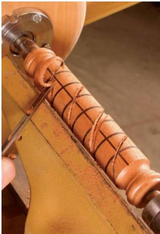
Carve the channel. Use a narrow gouge to carve a channel along each spiral. Stay to the right of the sawkerf so that you are cutting downhill and not against the grain. Flip the workpiece to carve the second half.
