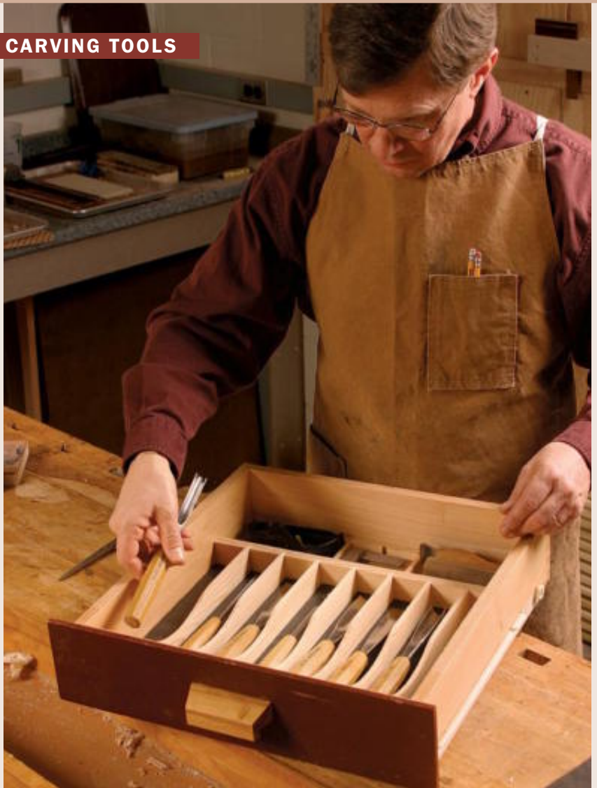
Lesser-used tools can be stored in drawers. Custom-made drawer dividers will help keep carving tools sharp.
