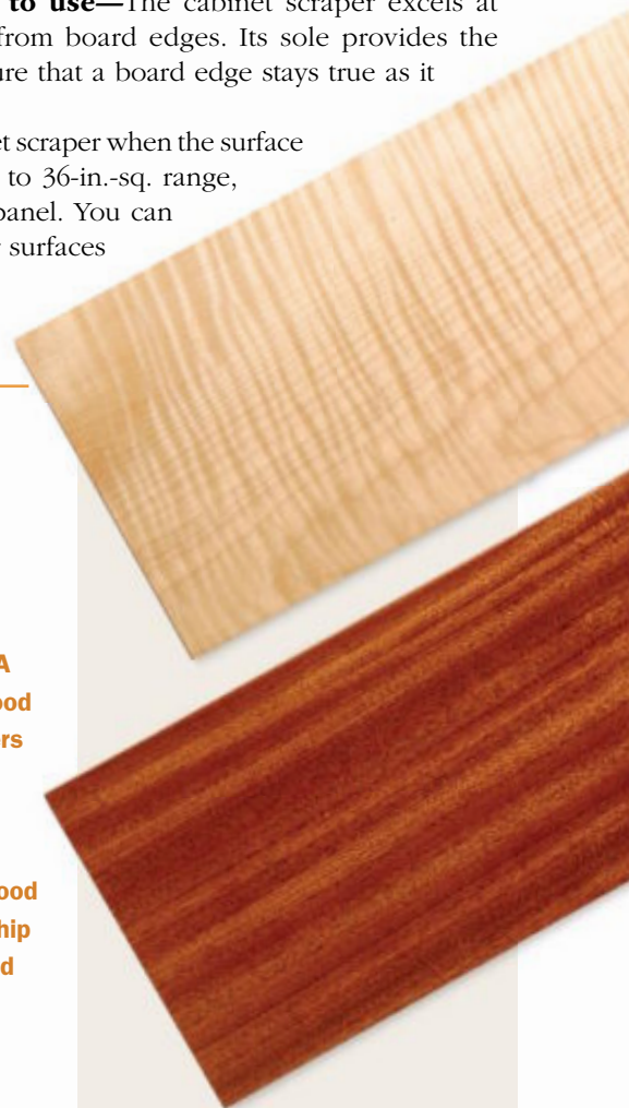
Figured grain begs a scraper. When smoothing wood with irregular grain, as in curly maple (top) and sapele (bottom), a scraper is less likely to create tearout than even a finely tuned handplane.
