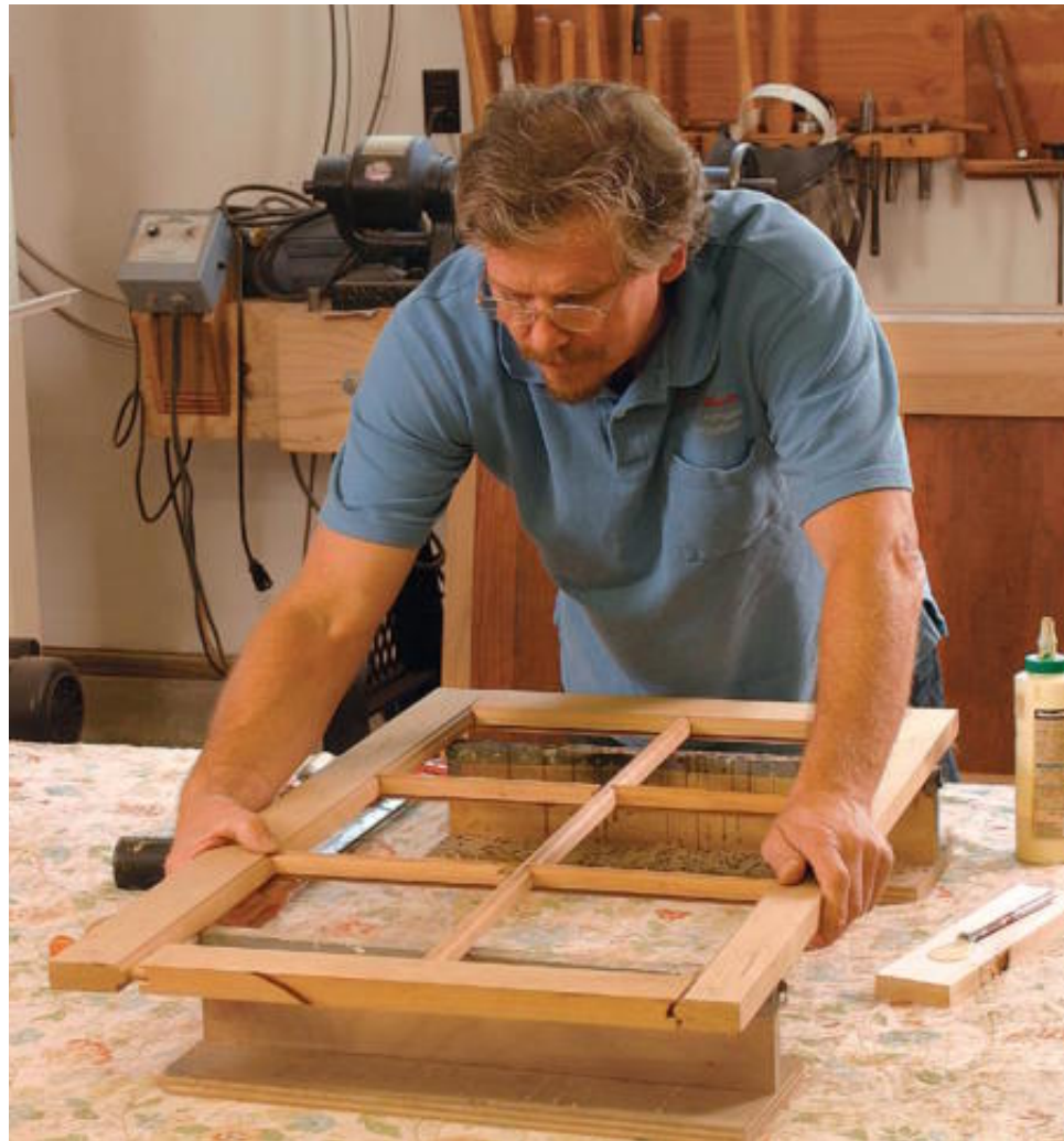
Assemble the door frame. Drive the horizontal muntins into the stile mortises, then install the vertical muntins in the rails (above). Elevate the frame so you can get clamps underneath, then bring all the parts together (right).
