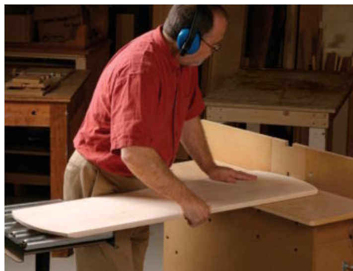
Support two ends. When you use a router table to profile the edge of a large workpiece, keep the opposite end supported.
