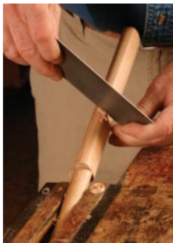
Finish shaping. Blend the contours and smooth the surface. Next, saw a kerf about 2 in. deep through the center of the tenon. The kerf should be parallel with the striking faces in the assembled mallet.
