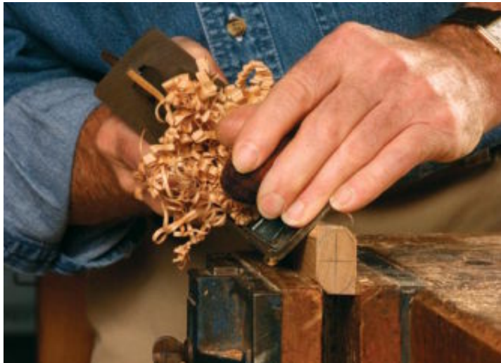
Chamfer the corners with a handplane. A simple ellipse layout is transferred to the handle's length with the same tangent method used for the tenon.
