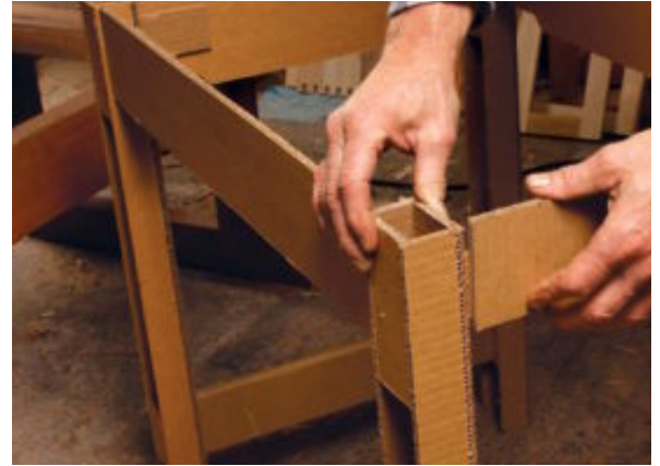
Cardboard is sturdy enough for mocked-up joinery. Rogowski glues a loose tenon to the inside of a rail and knives a mortise into a cardboard leg.
