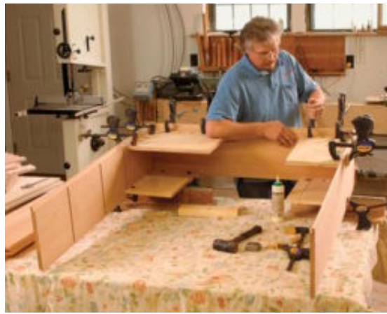
Connect the top to the sides. To ensure that the assembly remains square, the author clamps square sections of plywood into each corner.
