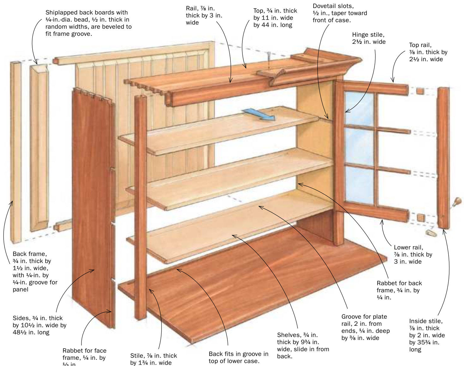
Add the front face frame. For a good fit, rip the rail and stiles so that they're a hair proud of the case, then plane the frame flush to the sides after the glue dries.
