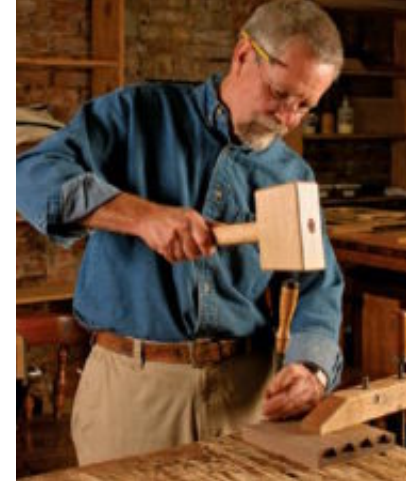
The driving force. A well-built mallet delivers a solid blow that powers chisels for chopping dovetails, mortises, and other joinery.
