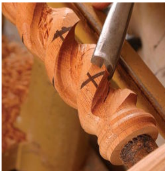
Widen the channel. Come back with a wider gouge to enlarge the channel. Again, always cut on the right side of the kerf. When complete, saw down another \frac{1}{4} in. and repeat the carving with the narrow and wide gouges.
