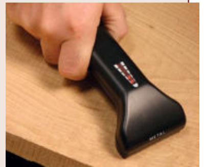
Recycled lumber may contain nails. Use a metal detector to find hidden fasteners that can ruin a cutter.
