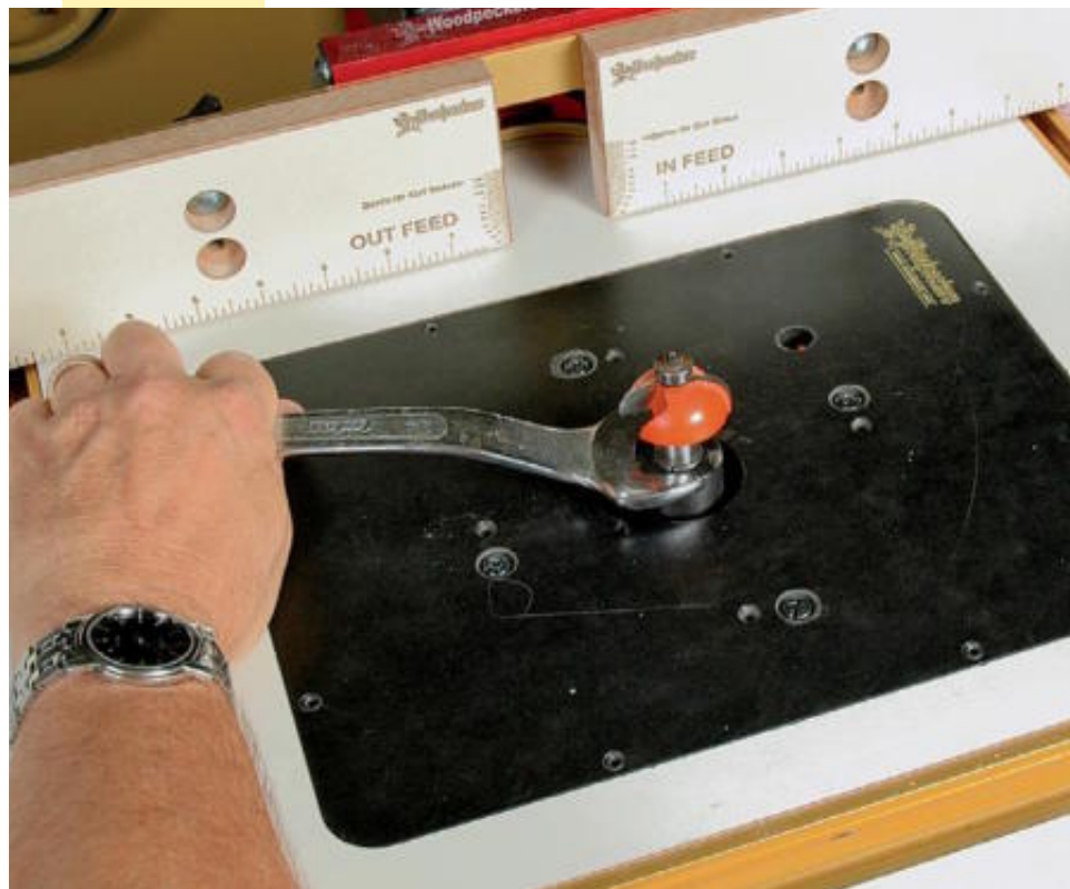
Easiest bit-changing. The Triton (above) has a well-designed spindle lock, and it lifts the collet above the table so you need only one wrench for bit changes. The Porter-Cable (left) is one of several routers that need two wrenches for bit changes; but at least you can do it from above the table.
