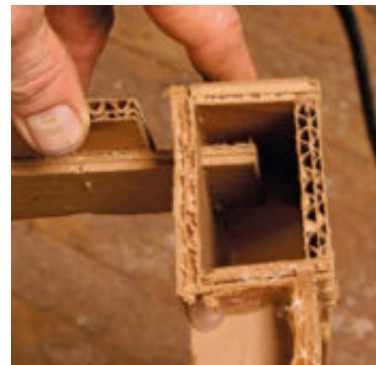
Cardboard is sturdy enough for mocked-up joinery. Rogowski glues a loose tenon to the inside of a rail and knives a mortise into a cardboard leg.
