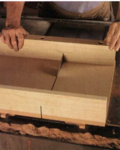
1 Make the kerf. Set the blade to its full height and cut through the sled.
