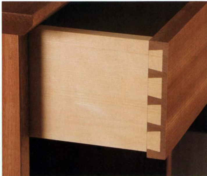
Making a mark. The line marking dovetail tails is often left to call attention to a traditional handcrafted joint, not one made by machine.
