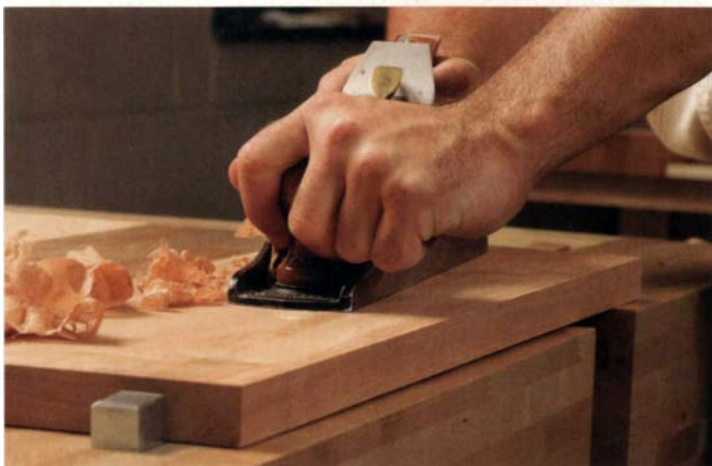
Unsteady workpieces. A combination of slop in the tail vise and dogs that angle backward under pressure causes the workpiece to rise off the bench when clamped.
