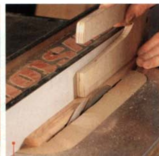
3 Trim to final width. Take light cuts and check the fit in the slot as you go. You also can use a planer or a handplane.
