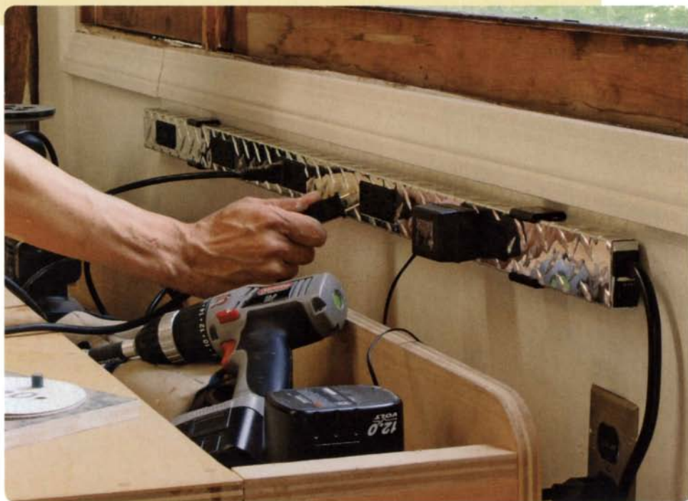
Workbench power. A Plugmold power strip gives you a convenient place to plug in power tools that are used often at your workbench.
