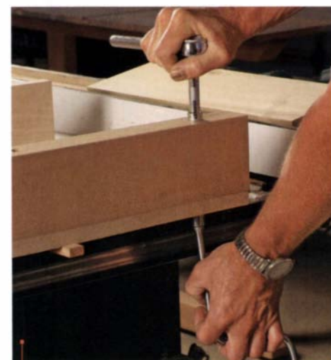
5 Tighten the fence. When you're done adjusting, crank the bolts home and you're ready to make crosscuts.
