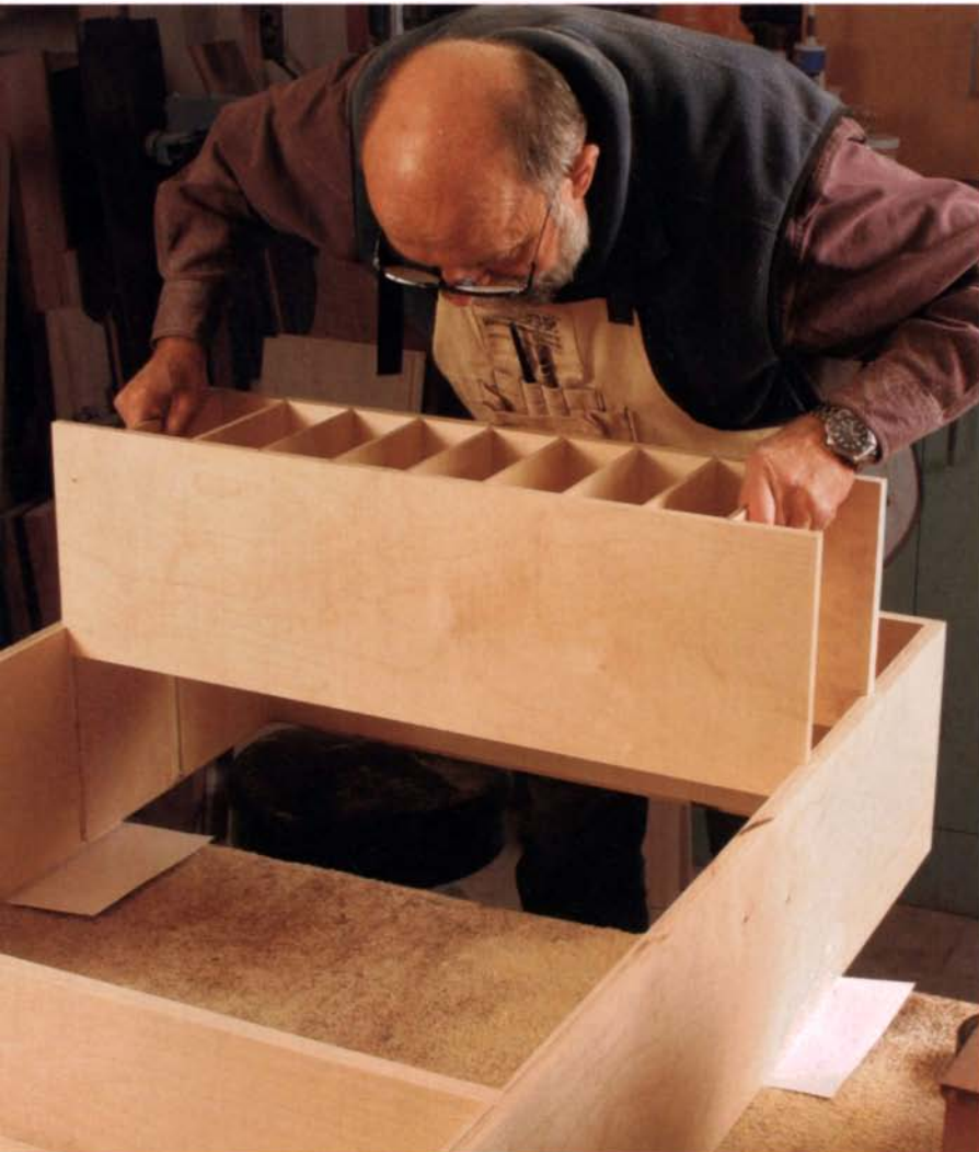
Install the upper shelf and gallery. Cut a dado on both sides of the cabinet and install the upper shelf. This gives the carcass extra rigidity. After routing the dados for the upper and lower shelves, test-fit the gallery and then glue it in.
