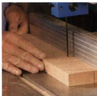
1 Bandsaw to rough dimensions. Set the fence using measurements taken from the tablesaw's miter-gauge slot.
