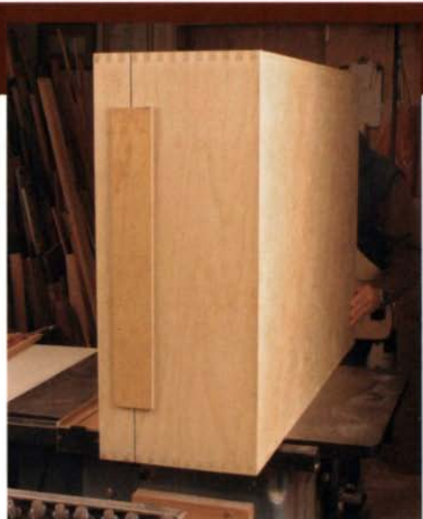
Cut away the door section. With the front and rear panels installed, cut away the front quarter of the box to form the main doors. Cut the short sides first, and then tack a batten across the cut to hold the section in place while cutting the long sides.
