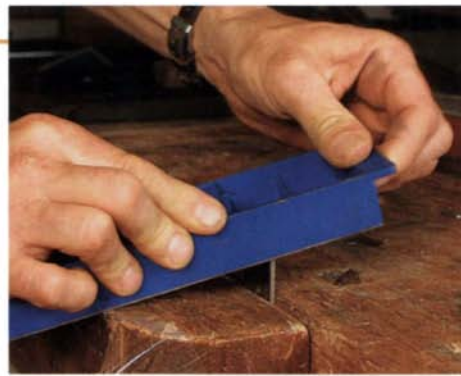
Grind the bevel. Guided by the edge of the bench, use a coarse diamond stone to establish the new bevel on the blade (above left). Clear tape protects the bench from wear. Polish the back of the blade with a fine diamond stone (below left). Finally, use a very fine stone such as a translucent Arkansas stone to polish both the bevel and the back of the blade.
