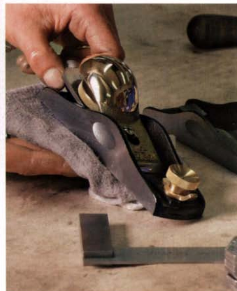
A plane is born. But before it's wrapped and boxed, every plane, handsaw, and chisel must pass a hands-on cutting test.
