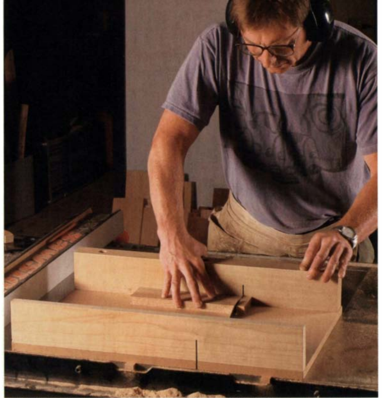
Every saw needs one. A shopmade sled makes it easier and safer to make accurate crosscuts on the tablesaw.
