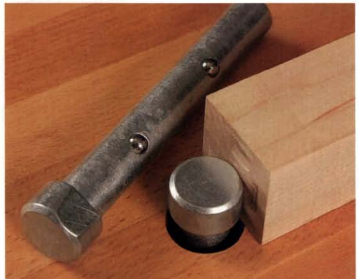
Good and bad dogs. The Laguna dogs slid in and out of the holes with the right amount of resistance, but editors disliked the small flat spot.
