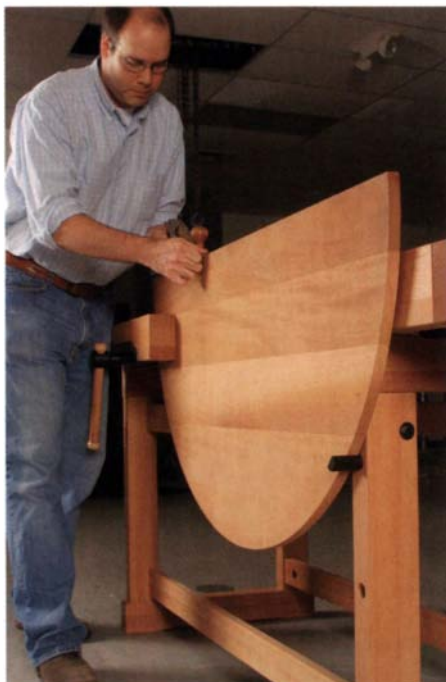
Edge-plane wide pieces. The legs are flush with the sides of the benchtop and contain dog holes so they can support long boards.
