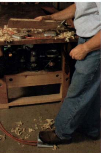
Clamping without clamps. The VacuClamp system holds a workpiece in place using vacuum pressure. To release the workpiece, simply press the foot switch.
