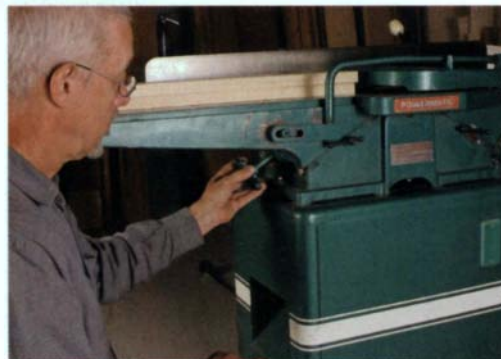
Outfeed adjustment. Many jointers have a handwheel for fine-tuning the height of the outfeed table. You'll need to do that after changing knives.
