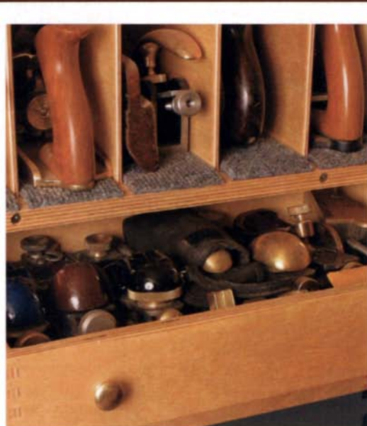
Drawers for small objects. The six drawers at the bottom of the cabinet hold small objects such as block planes.
