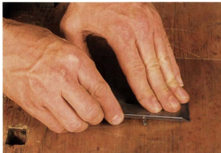
Roll a burr. Place a few drops of oil on a piece of float glass and roll the blade to and fro on a \frac{1}{8} -in. drill bit with the tip of the blade pressed firmly on the glass. After a few strokes, you should start to feel a burr.
