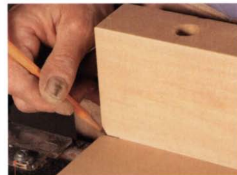
4 Mark your starting place. Before adjusting the fence, mark its original location as a reference point.
