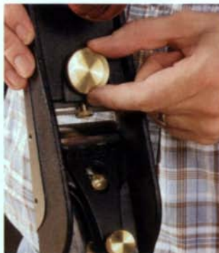
A big mouth. The adjustable sole plate on this Veritas plane makes it easy to adjust the blade for coarse or fine shavings.
