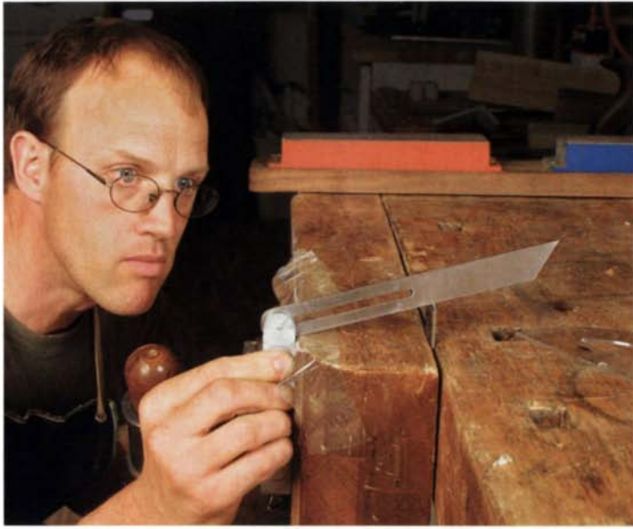
Establish the bevel angle. Use a sliding bevel to set the blade at the correct height in the vise for grinding a 75° bevel.
