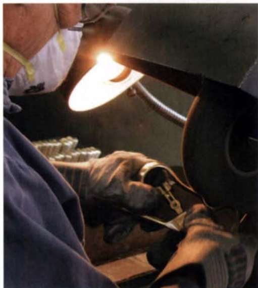
Bring out the shine. The operator of a polishing machine makes the body of a bronze edge-plane look like jewelry.
