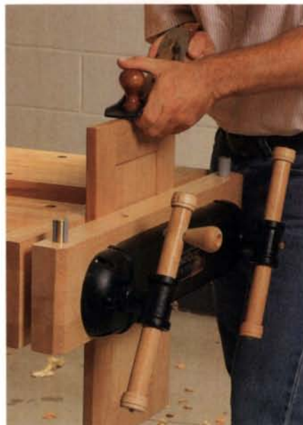
Wide clamping ability. The large distance between the guides in the tail vise allow wide boards to be clamped securely.
