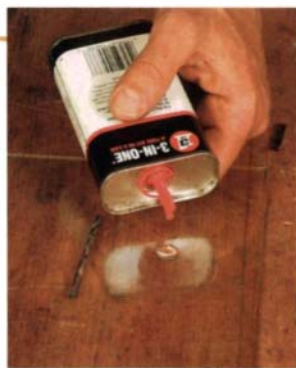
Roll a burr. Place a few drops of oil on a piece of float glass and roll the blade to and fro on a \frac{1}{8} -in. drill bit with the tip of the blade pressed firmly on the glass. After a few strokes, you should start to feel a burr.
