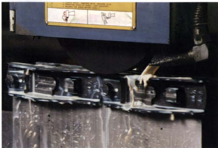
Side grinding. A pair of bench planes, clamped end to end, have their sides ground flat and square to the soles.
