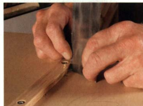
5 Trim the high spots. Push the completed sled back and forth in the slots a few times. Any places where the runners rub against the side of the slots will darken. Trim these areas with a scraper, then wax the runners and the bottom of the sled to reduce friction.
