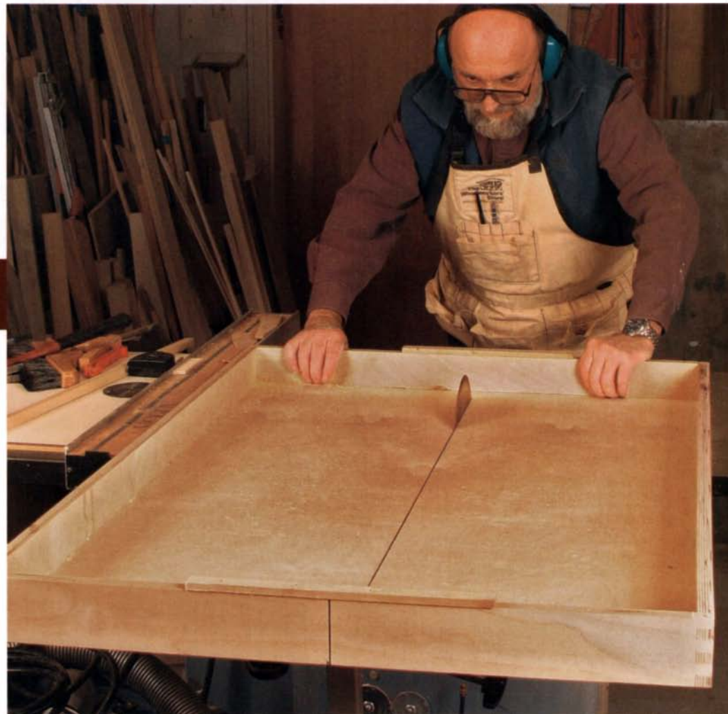
Next cut makes the two main doors. Tack two strips of wood across the cut line as shown. Then set the sawblade to just score the underside of the strips. In this way the panel is cut in half but won't bind on the sawblade.
