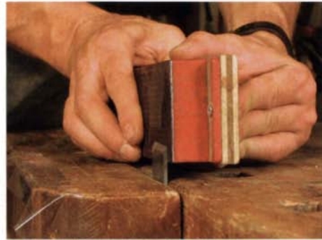
Establish the bevel angle. Use a sliding bevel to set the blade at the correct height in the vise for grinding a 75° bevel.
