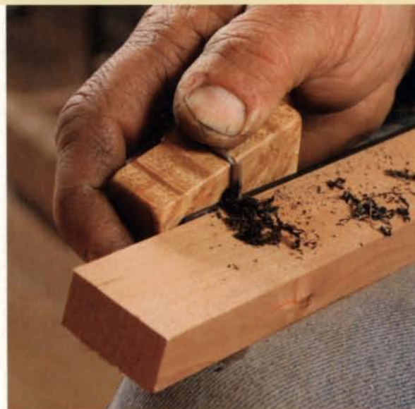
Simple jig for perfect miters. Clamp a 45° guide block to the frame members and chop the beading to length.
