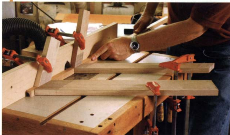
Top and side featherboards increase safety and accuracy when working with small, narrow stock. The setup ensures a straight, flat-bottomed dado on the table saw (right) and a cleanly cut molding or edge detail on the router table (below).
