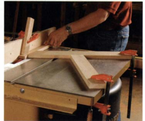
Top and side featherboards increase safety and accuracy when working with small, narrow stock. The setup ensures a straight, flat-bottomed dado on the table saw (right) and a cleanly cut molding or edge detail on the router table (below).
