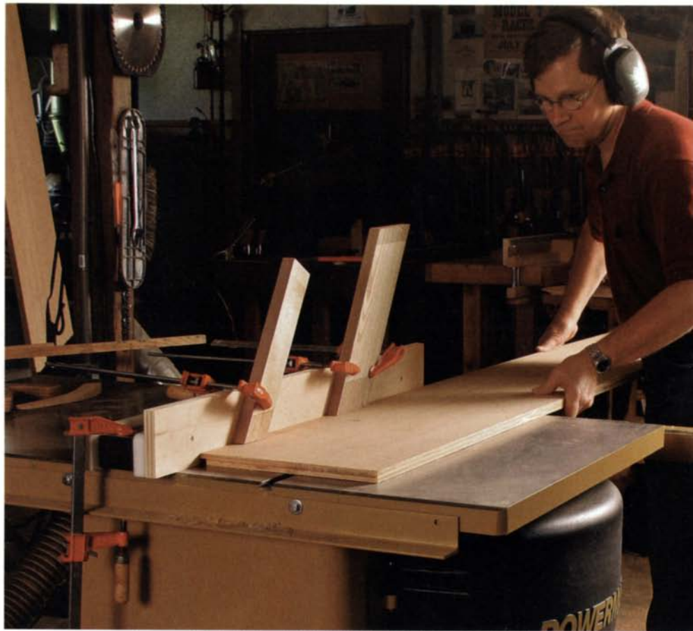
Fence-mounted featherboards apply pressure from the top down. This keeps stock firmly against the table for tasks like rabbeting an edge on the tablesaw (right) or cutting a molding profile or edge treatment on the router table (above).
