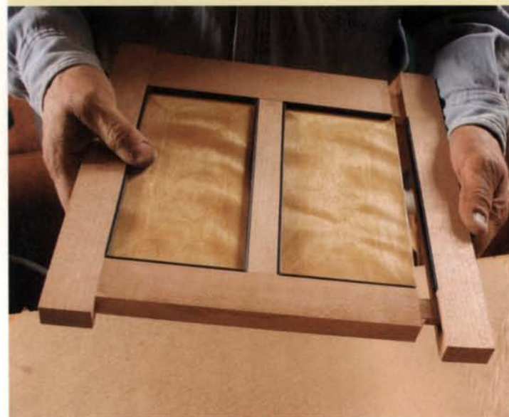
Scratch the bead. Run a simple scratch stock along the beading. You're done when the cutter just starts to bite into the frame.
