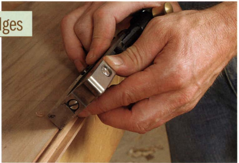
Go places other planes can't. The sharp edge adjacent to the beaded edge of the cabinet backboard is easy to soften with a shoulder plane.
