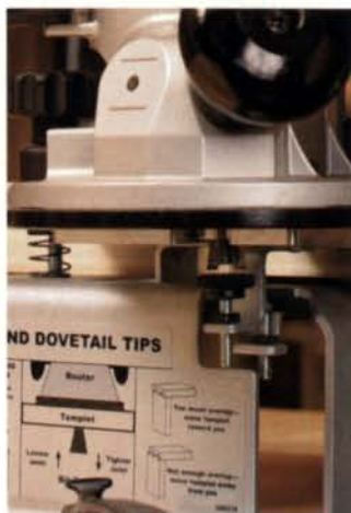
Another unique guide. The Porter-Cable is the only jig with built-in guides for setting bit depth. Instructions on the jig mean fewer trips to the manual.
