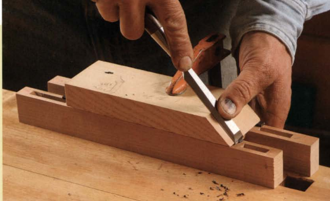
Simple jig for perfect miters. Clamp a 45° guide block to the frame members and chop the beading to length.
