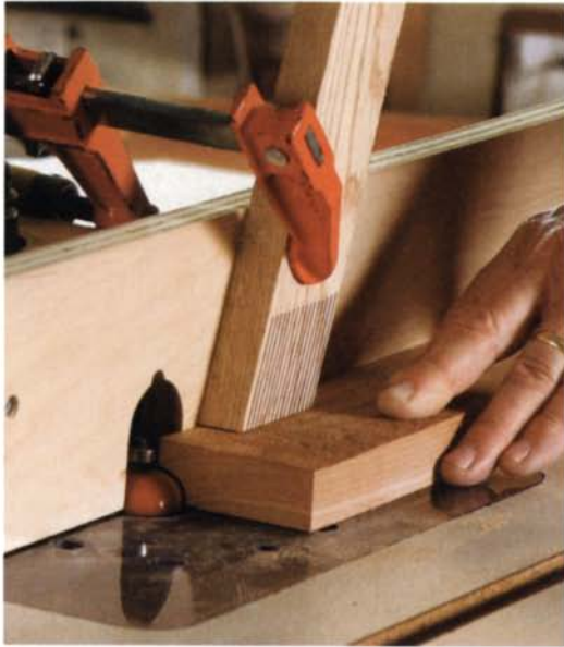
Fence-mounted featherboards apply pressure from the top down. This keeps stock firmly against the table for tasks like rabbeting an edge on the tablesaw (right) or cutting a molding profile or edge treatment on the router table (above).
