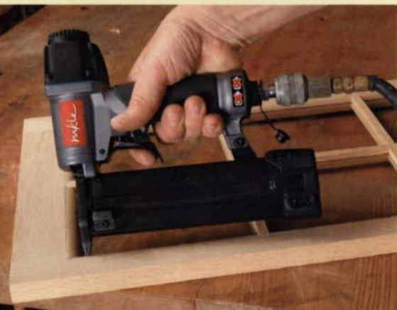
The Nikle holds 200 fasteners. And the carriage automatically adjusts to fit different lengths, from ½ in. to 1¼ in. long.
