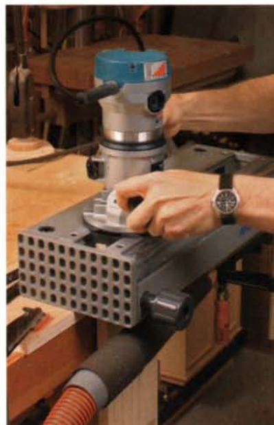
Good old pencil marks. After cutting the tails, you mark the jig at the center-line of each template finger and then align the pin fingers with those marks.
