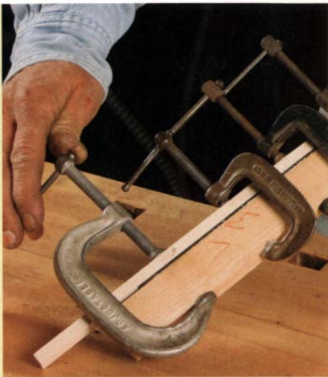
Glue the beading to the frame. The beading should be proud of the outside of the frame. Use plenty of clamps and a caul to ensure a good bond.
