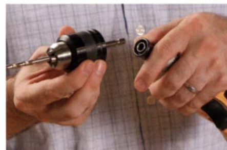
Now you can use round-shanked bits in your impact driver. DeWalt's keyless chuck adapter for impact drivers accepts round-shanked bits up to ⅜ in. dia.
