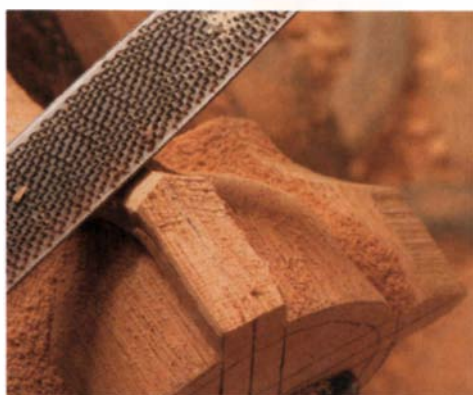
Rasp the talons. Use a patternmaker's rasp to flatten the triangular profile from the second knuckle to the base. Then create the concave profile between the second and third knuckles (above).
