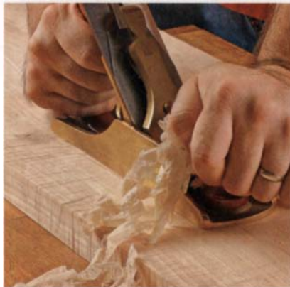
A different angle for different species. Easily worked boards of low-density hardwoods such as this piece of mahogany work best with the blade at a medium angle of around 45°.
