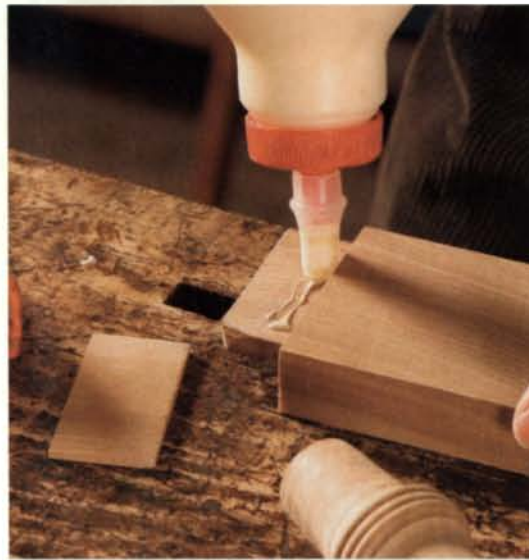
Add a shim. Make a shim from the material used for the workpiece and glue it to the tenon. Make sure that the grain runs in the same direction on both pieces.
