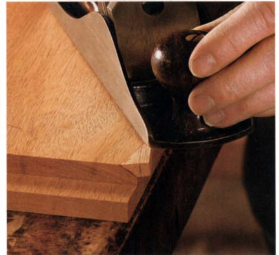
Custom-fit a repair piece. Mark out and saw the repair piece to fit the missing corner (left). Take care to ensure that the grain direction matches the workpiece as closely as possible. Glue the repair piece in place, leaving the outside surfaces proud of the workpiece. Once the glue has dried, carefully saw, pare, and plane it flush to the workpiece (above).
