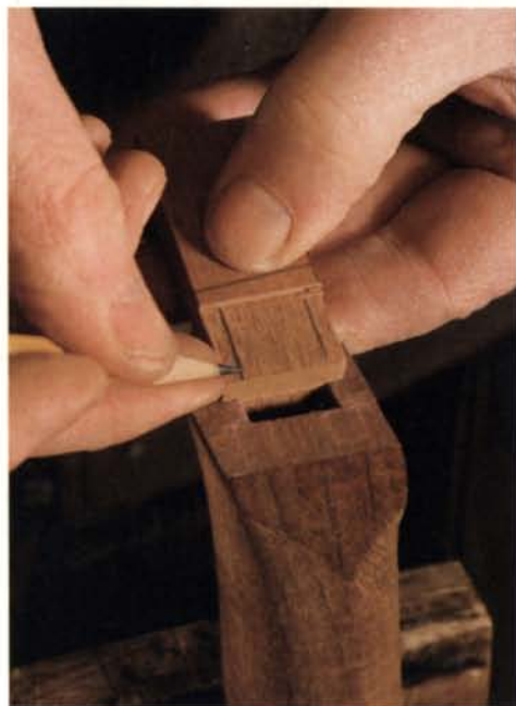
Fit the new tenon. Size and shape the repair piece to fit the newly created mortise. Then glue it in place.
