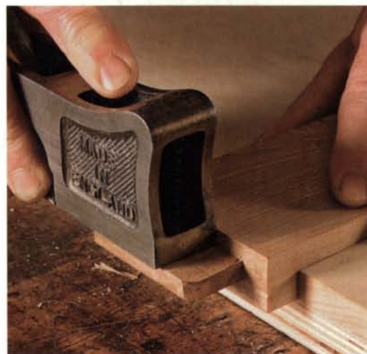
Trim the excess. After the glue has set, use a shoulder plane to pare the tenon to proper size. Check your progress frequently as you plane away the excess material. Stop when you have a snug push-fit.
