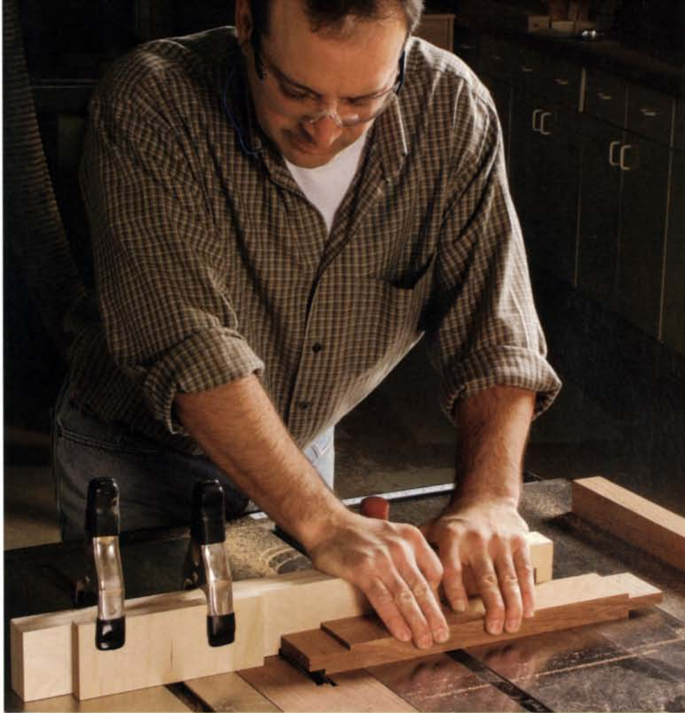
Tenons on the tablesaw. Use a dado set for quick tenons. For accuracy and clean cuts, outfit the miter gauge with an auxiliary fence and a stop block. Through-tenons must look good and fit right, so clean them up with a shoulder plane, a block plane, and/or a chisel.
