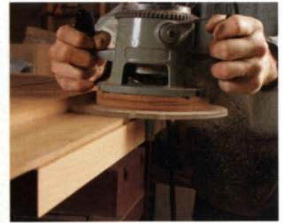
Router as jointer. With the help of a jig, you can clean up rough-sawn edges on large workpieces such as tabletops. Work from left to right.
