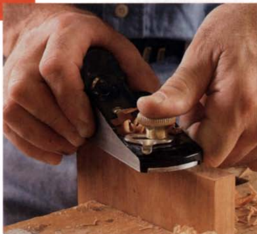
Block planes for small areas. A low-angle block plane is the best choice for planing small areas of end grain.
