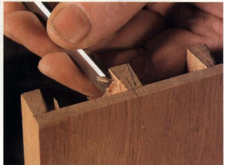
Use cutoff stock for the repair. Fit and glue in the rectangular repair piece (left). Trim the new piece flush with a saw and handplane. Use the tail board to mark out the sides of the new pin. Be more careful this time!
