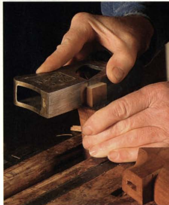
Trim the exposed end. After the glue sets, trim and pare the tenon cheeks to fit the mortise in the mating piece and get the parts to line up.
