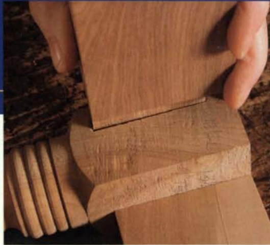
A too-slender tenon. A tenon that has been cut or trimmed too narrow creates a weak joint.
