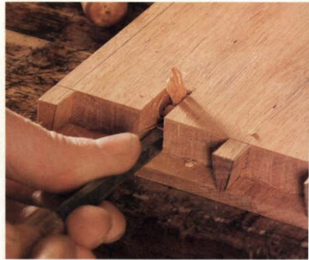
Mark out for pin removal. Scribe lines to create a rectangular mortise matching the maximum width of the pin (above). Remove material by making angled chisel cuts to create a ramp to the baseline at the front of the pin. Then pare from the front (right) until the bottom is square.
