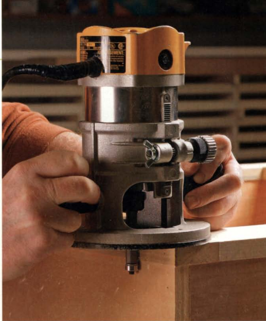
Trim face frames flush to case. The bearing on a flush-trimming bit is the same diameter as the cutter, allowing you to bring a frame flush to a carcass using a handheld router.
