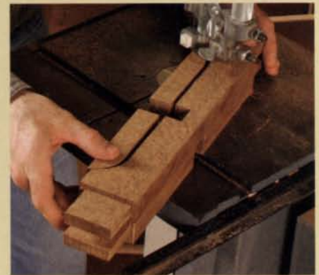
Profile the stretchers. Join the lower stretchers with double-sided tape and then bandsaw the profile.
