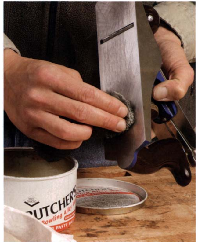
Corrosion prevention. A light coat of paste wax can help prevent tools from rusting. If you apply the wax with 0000 steel wool, you can remove light rust from the tool.
