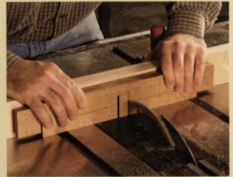
Cut the half laps. With the same miter gauge and auxiliary fence used to cut the tenons, cut the half-lap joint on each stretcher.
