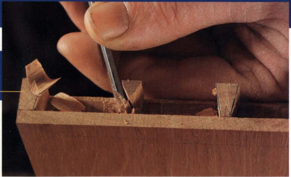
This can't be shimmed. A slip with the chisel left a broken pin.
