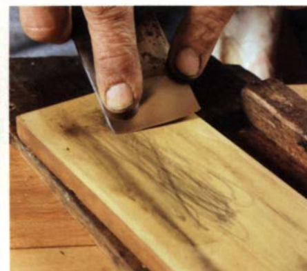
Rock and hone. To sharpen a scrub plane, begin with one edge against the stone (left), then rock it to the other side as you move it over the stone (right).
