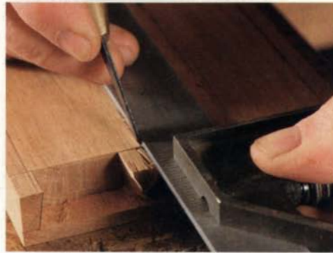
Mark out for pin removal. Scribe lines to create a rectangular mortise matching the maximum width of the pin (above). Remove material by making angled chisel cuts to create a ramp to the baseline at the front of the pin. Then pare from the front (right) until the bottom is square.
