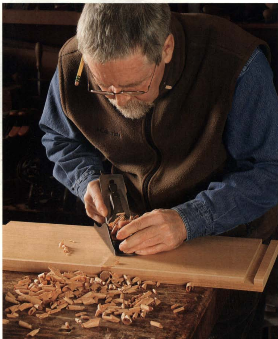
That sinking feeling. The wrong end of the workpiece was against the fence, so the center dado is in the wrong place.
