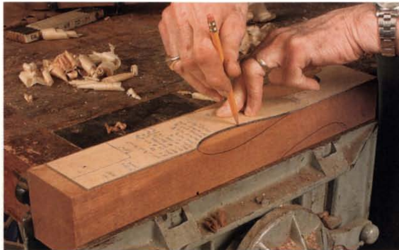
Lay out the leg. Use the template to lay out the cabriole leg on adjacent sides of the blank.
