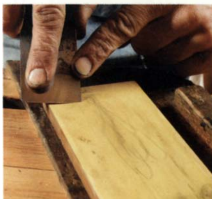
Rock and hone. To sharpen a scrub plane, begin with one edge against the stone (left), then rock it to the other side as you move it over the stone (right).
