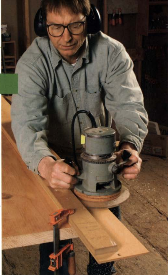
Router as jointer. With the help of a jig, you can clean up rough-sawn edges on large workpieces such as tabletops. Work from left to right.
