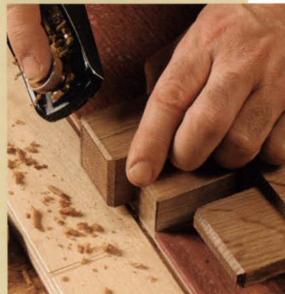
Chamfer the tenons and legs. A 1/8-in. bevel gives the exposed through-tenons and leg bottoms a softer look and creates interesting shadow lines.
