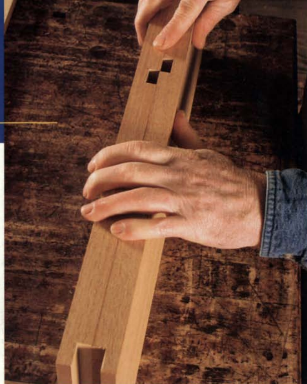
That sinking feeling. The wrong end of the workpiece was against the fence, so the center dado is in the wrong place.
