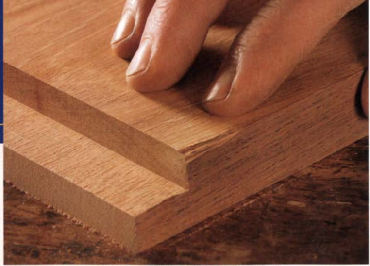
A chipped-out corner. An otherwise clean rabbet cut is marred by a triangular chip torn from the edge.
