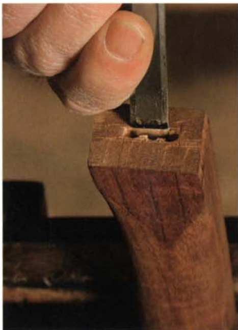
Create a mortise. Saw and chisel away the broken remnant of the tenon for a clean surface. Use dimensions from the mating piece to locate the new opening.
