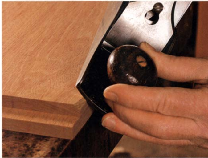
A chipped-out corner. An otherwise clean rabbet cut is marred by a triangular chip torn from the edge.
