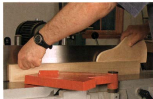
Use a pair of push blocks for face-jointing. It's best to have a nonskid block at the board's leading edge and a cleated block at the rear.
