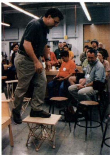
These aren’t Tinkertoys. This table of Siberian elm is supported by a lightweight structure of linked tetrahedrons.
