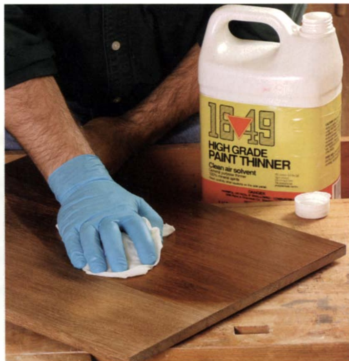
Remove surface oils. Use a cloth soaked in mineral spirits to wipe down the surfaces of a teak table before you apply a solvent-based brushing varnish.
