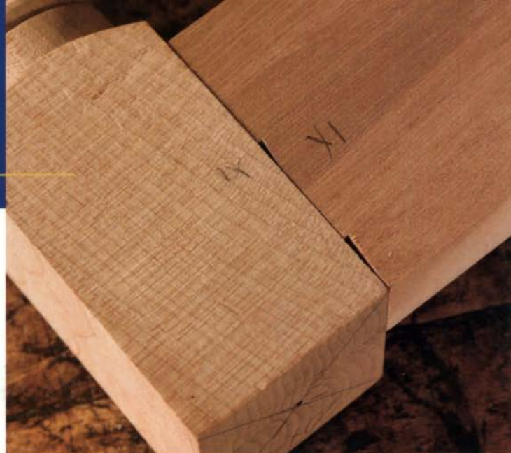
An ugly result. A slip with the shoulder plane can leave unattractive gaps.
