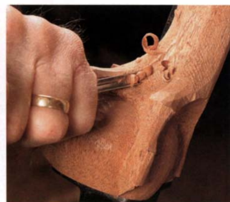
Carve the web. Use a #8-13 mm gouge to hollow out the areas between the center and side talons (left). Work upward from the ball until you feel the wood start to tear, and then make relief cuts downward. Use a #9-7 mm gouge to create the sharp transition from the web into the tendons (above).
