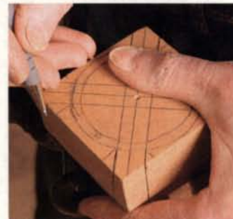
Define the talons. Use a fine-tooth saw to cut just outside the lines marking the width of the talons.
