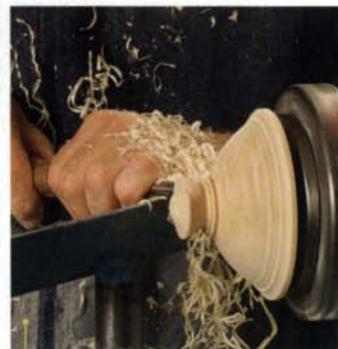
7 Complete the top. Trim the lid and finish off the knob. Then sand and finish.
