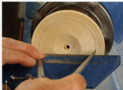
3 Use the dividers to scribe the diameter. Dig the left point of the dividers into the work as it is spinning, then see if the right point lines up with the scribed line.
