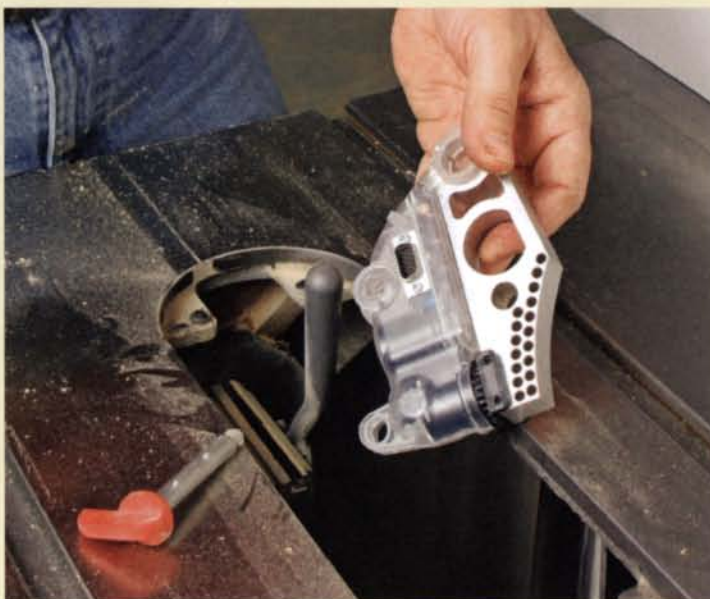
SawStop blade brake. This ingenious device on the SawStop stops a spinning sawblade the instant the blade is touched. Instead of a trip to the hospital, the user ends up with only a shallow cut.
