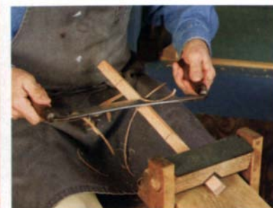
Shave the blanks. With the blank for a rung held in a shaving horse, a drawknife is used to turn it into a rough octagonal shape.
