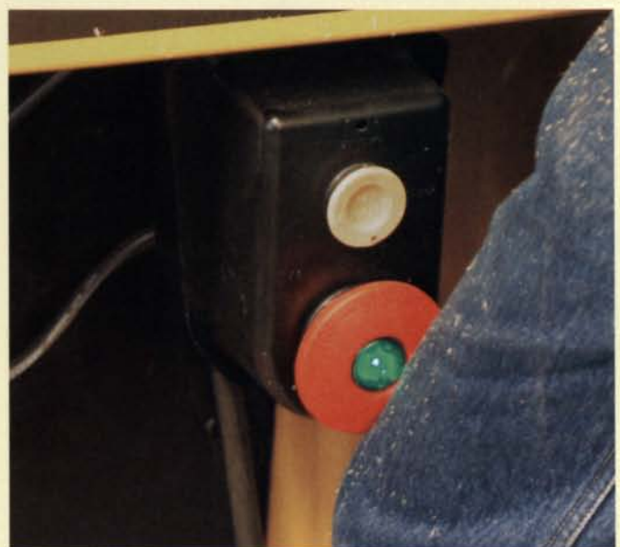
Kneable switch. In an emergency, the jumbo-size switch on the Powermatic PM2000 can be easily reached with a knee. The green-glowing center lets you know that the saw is powered up.
