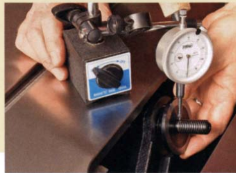
Arbor runout. An arbor that wobbles will cause vibration and rougher cuts, so Johnson looked under the hood to check each one.
