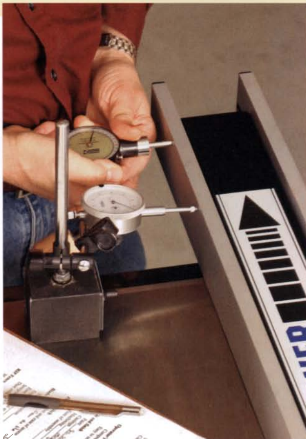
Fence deflection. With the rip fences locked, Johnson applied force to the end of the fences and measured deflection.
