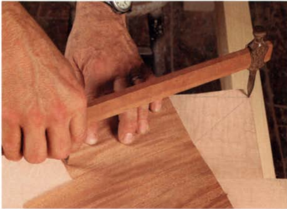
Fit the crossbanding. Use the compass, trammel points, and knife to mark and cut the crossbanding to fit the recess.
