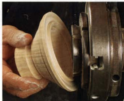
6 Cut a step for the chuck jaws. Similar to the base, cut an angled step on the inside of the lip for the expanding chuck jaws to grab before removing the lid and remounting it. Apply a finish to the inside surface.
