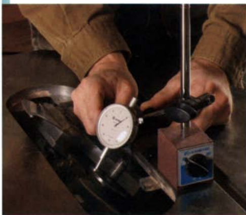
Check for runout. Use a dial indicator to check the tablesaw’s arbor flange. Any variations in the flatness of the piece can cause blade wobble, which leads to rougher cuts.
