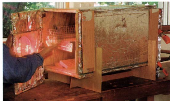
Dry the rungs. Because the rungs must be bone dry when inserted into the posts, a homemade kiln with heat lamps is used to dry them.
