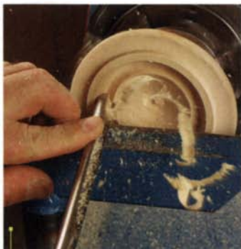
5 Hollow the top. With the lip sized, use a gouge to hollow out the inside of the lid.
