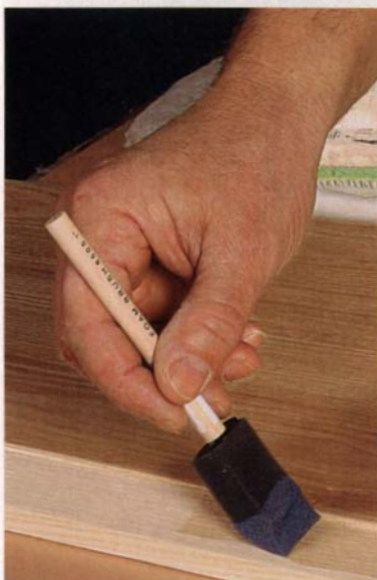
Padding wide areas. A paint pad works well when applying a water-based finish to a large area. Charge the pad on a plate containing the finish, and then remove the excess by touching it on another plate lined with paper towels.
