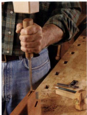
Chisels built for grunt work. The design of these tools is based on English mortising chisels of the mid-20th century. Thick, Sheffield (D2) steel with tangs buried into the tapered oval beech handles and a bolster fit flush to the handles make these mortise chisels virtually indestructible.
