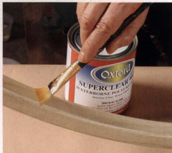
A choice of brushes. When applying a water-based finish to narrow surfaces, use either a foam brush or an artist's brush with man-made bristles.
