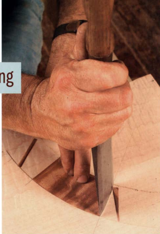
Cut the veneer to length. Use the lines on the workpiece that divide the arc into quarters as a guide for cutting each section of crossbanding to length.
