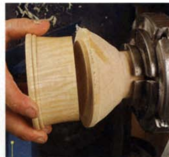
4 Turn the lip to the scribed line. Check the fit as you work. The lid should fit loosely because the wood will shrink and expand.
