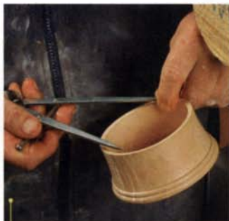
2 Measure the box opening with dividers. Transfer the inner diameter of the box to the lid, which is flipped and remounted.
