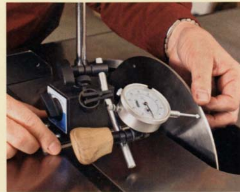
Blade/miter slot parallelism. A 10-in.-dia. flat plate and dial indicator were used to find out if the sawblade is parallel to the miter-gauge slot when the blade is at 90° (shown) and 45°. Misalignment can be corrected.
