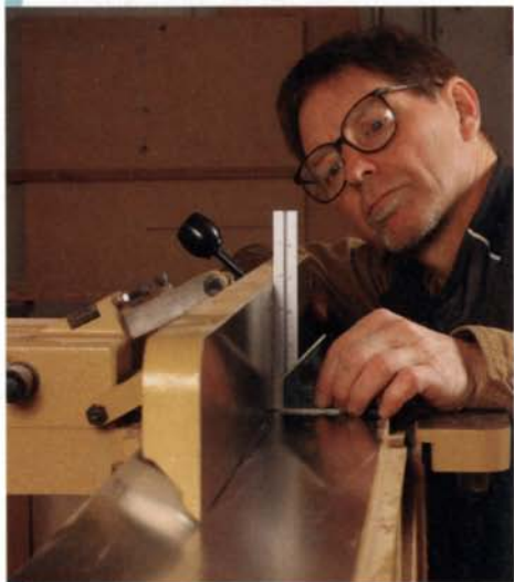
Check the fence. Use the combination square to ensure that a jointer's fence is set at 90° to the tables. Make similar checks on the tablesaw and bandsaw.
