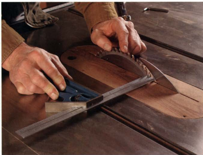
Adjust the miter slot. The combination square also can help check whether a table saw's miter slot is parallel to the blade. Mark a tooth at the front of the blade and measure the distance from the blade to the slot. Next, rotate the marked tooth to the back of the blade opening and measure again. If the readings are different, you need to adjust your saw's tabletop or trunnions to bring the slot parallel with the blade.
