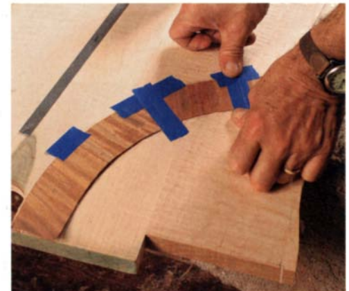
Glue the crossbanding. Because of its long open time, Headley uses white glue to secure the crossbanding. Tape across and in between the joints reduces the chances of the veneer slipping when clamps are applied.
