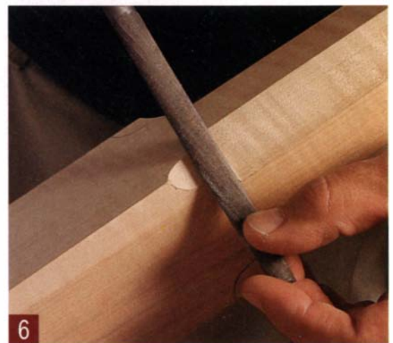
Define the base. Pound the tip of the 1-in. chisel into the base of the tongue to add definition to the detail (5). Clean up and smooth the surfaces with a 6-in. double-cut file (6).
