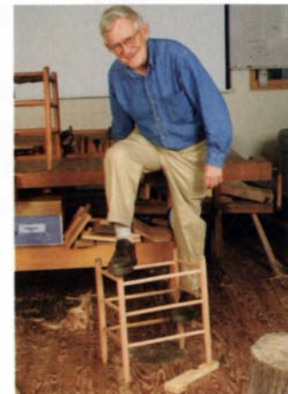
One strong frame. As soon as the frame has been assembled (left), check that all the legs touch the floor. If they don't, place a block under the longest leg and then stand on the frame to rack it straight (above).
