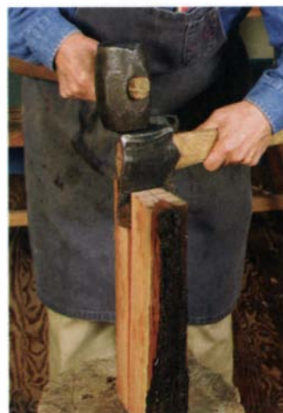
Rive green wood. Splitting or riving straight-grained green hardwood is necessary for this type of joint.
