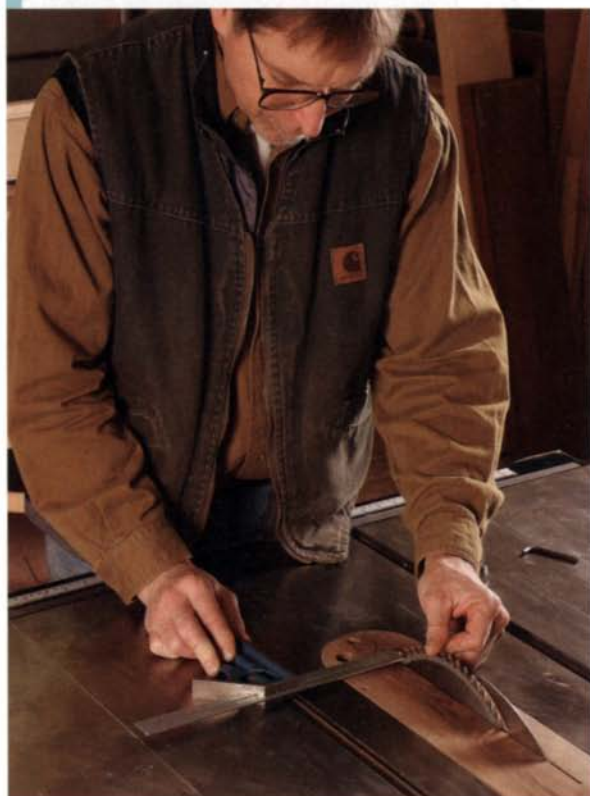
Check the fence. Use the combination square to ensure that a jointer's fence is set at 90° to the tables. Make similar checks on the tablesaw and bandsaw.
