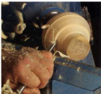
1 Mount the second blank on a center-screw chuck. Turn a round tenon on the end and rough-cut the exterior profile.
