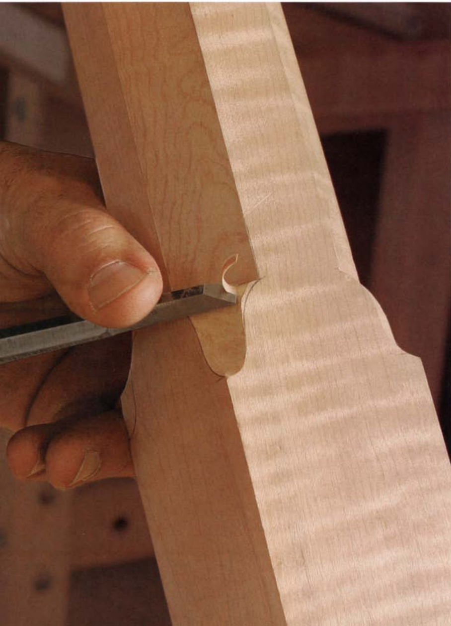
Define the base. Pound the tip of the 1-in. chisel into the base of the tongue to add definition to the detail (5). Clean up and smooth the surfaces with a 6-in. double-cut file (6).
