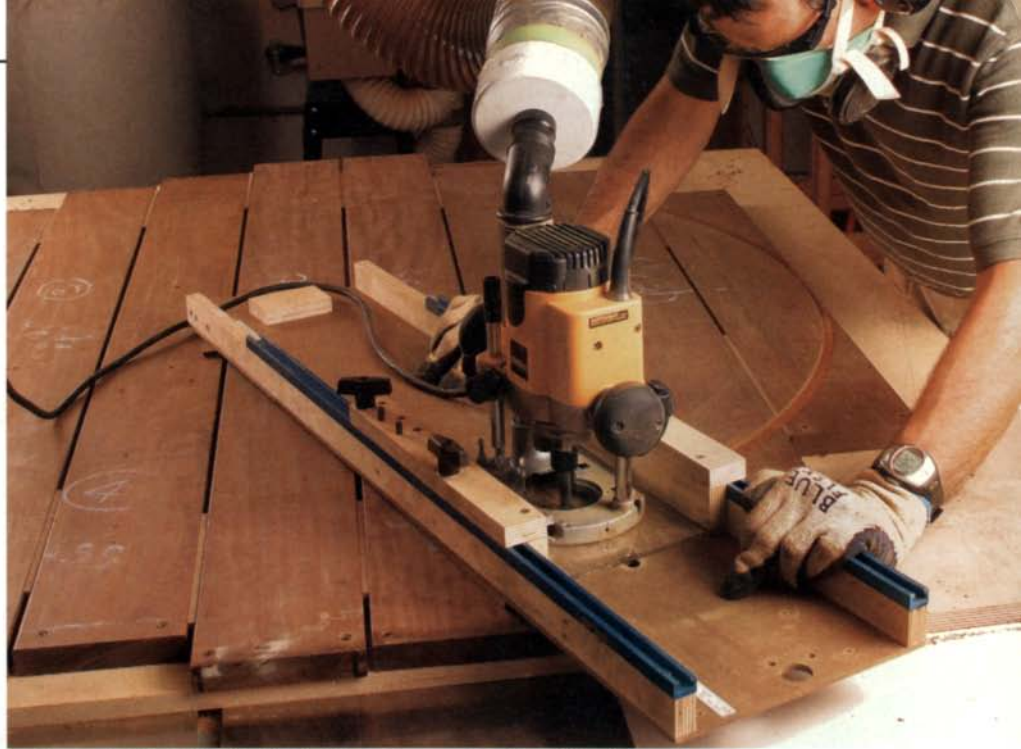
Route the tenons first. To minimize tearout, the author uses a ½-in. spiral up-cutting bit and ¼-in. MDF spacers between the boards where the router will pass. Take shallow passes until the tenon thickness matches the groove in the ring.
