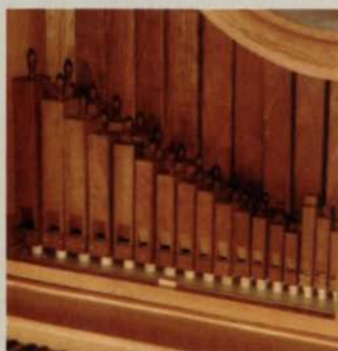
No ebony or ivory. The organ's 49 pipes are made of cherry. The case is quartersawn fir and the keys are bird's-eye maple and ipé.
