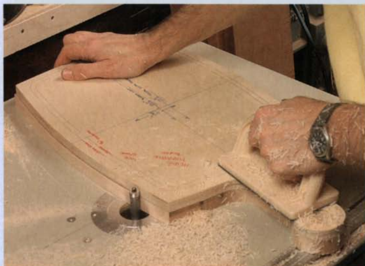
Saw and rout the perimeter. Saw close to the line before routing with a bearing-guided, flush-cutting bit.
