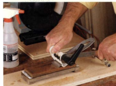
A jig for grinding and honing. The manufacturer designed this jig for grinding and honing flat plane blades and chisels. It slides side-to-side on a steel bar mounted in front of the grinder (top) and then slips off for honing on a benchtop stone (bottom).
