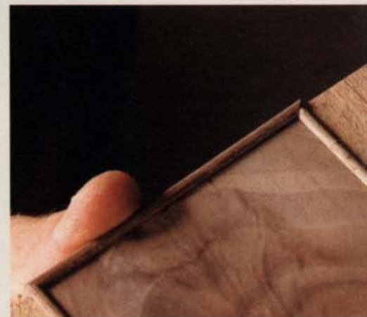
6 Fit the sides. With the top and bottom beads dry-fitted and clamped with cauls, fit the side beading.
