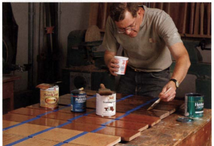
A variety of finishes. To see whether different clear finishes affected the final appearance, the author divided the oiled and non-oiled boards into four sections and finished them with shellac, water-based finish, lacquer, and varnish.
