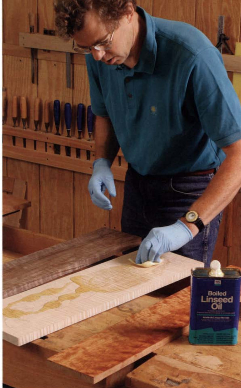
Applying the oil. Boards of curly cherry, tiger maple, and curly walnut were cut into three sections each. The first was wiped with boiled linseed oil, the second with tung oil, and the third left bare.
