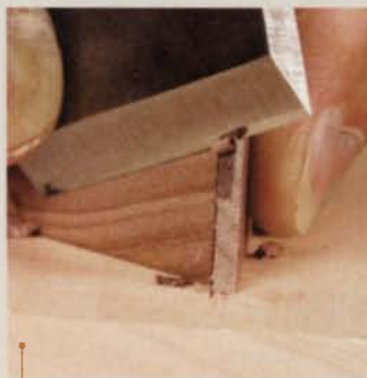
2 Slice the miters. Use an angled cutting block (see drawing, right) to guide the plane iron or chisel when cutting the stopped miters.
