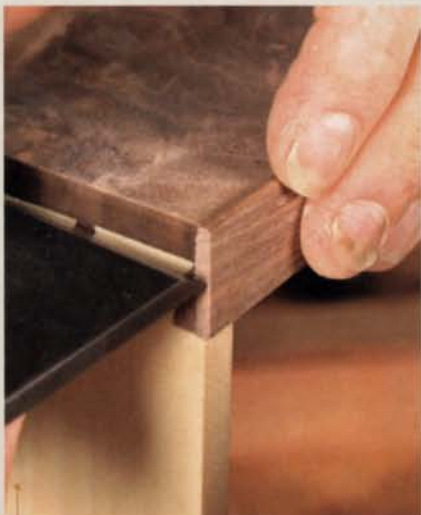
1 Mark the miters' depth. Use a plane iron resting on the bottom of the side rabbets to mark where the miters stop.
