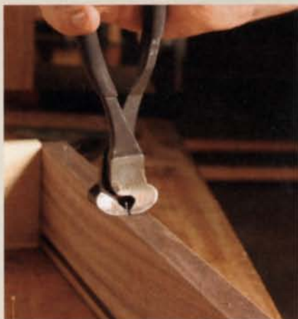
4 Clipped brads prevent sliding during fitting. Tap three brads into the top and bottom of the drawer front, and then remove the heads close to the surface.
