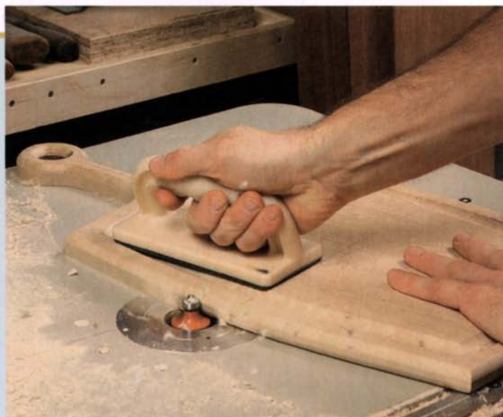
Shape the edges. A bearing-guided bit makes a partial roundover on this board. Flip the board to complete the profile.
