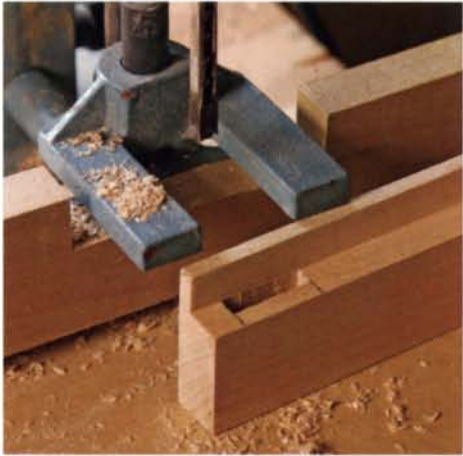
Cut mortises before tenons. The tenons then can be sized for a precise fit.
