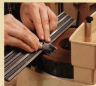
Not as good for everything else. Chisels and plane irons must be guided freehand on the tool rest.
