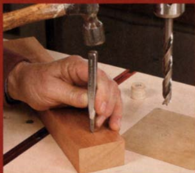
For greatest accuracy when using brad-point and twist bits, use a center punch before drilling.
