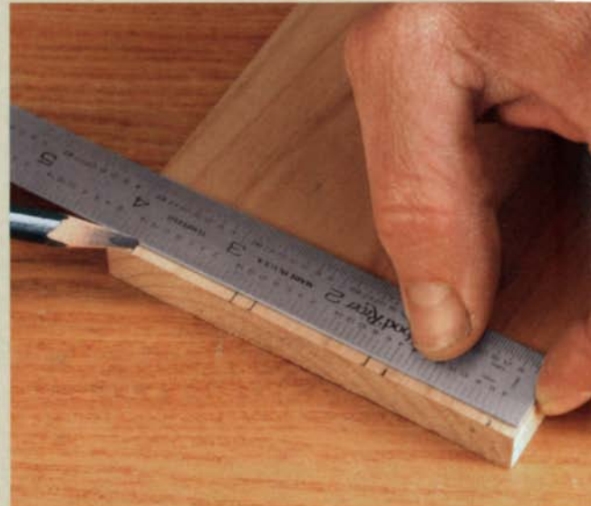
Easy to use. A short, easy-to-read, 6-in. steel rule is perfect for precise measuring and marking.
