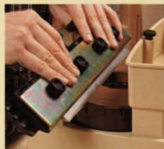
Great for planer knives. The tool rest and tool clamp are designed for sharpening planer and jointer knives and work well.
