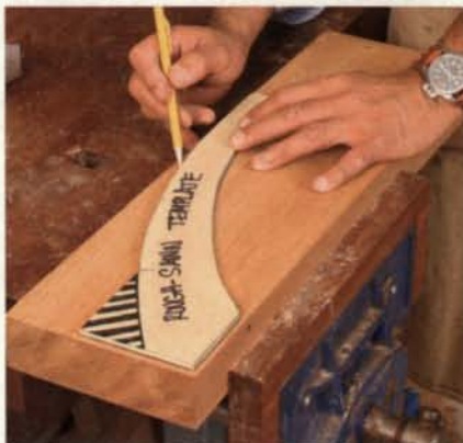
Use a template to trace the leg profile. Duplicating the legs is much more uniform with a template.
