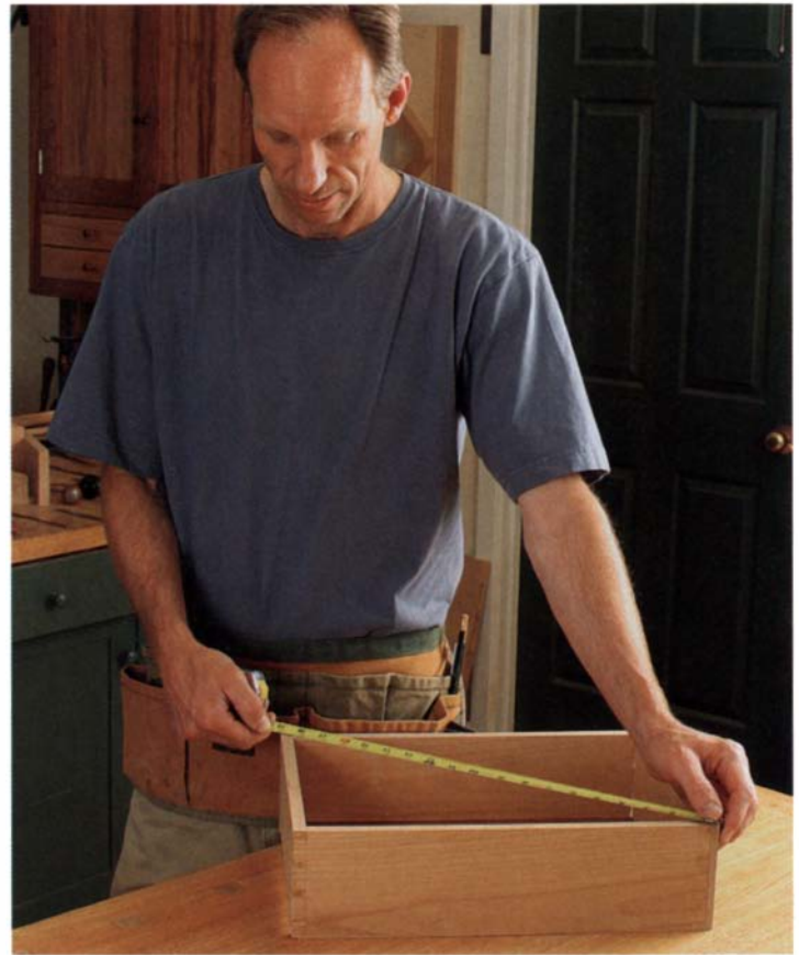
Tape measure gives all-around accuracy. As workpieces get bigger, a tape measure is the ticket to long measurements.
