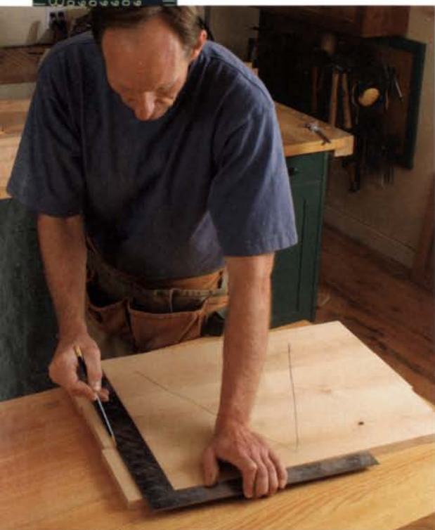
Framing square for bigger jobs. When scribing a line across a wide workpiece, like a panel, a framing square is Gochnour's tool of choice.
