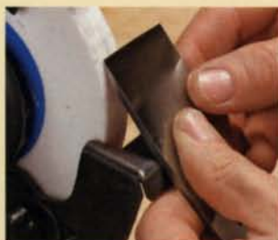
The dry wheel has a poor tool rest. It is rounded and too far from the wheel.
