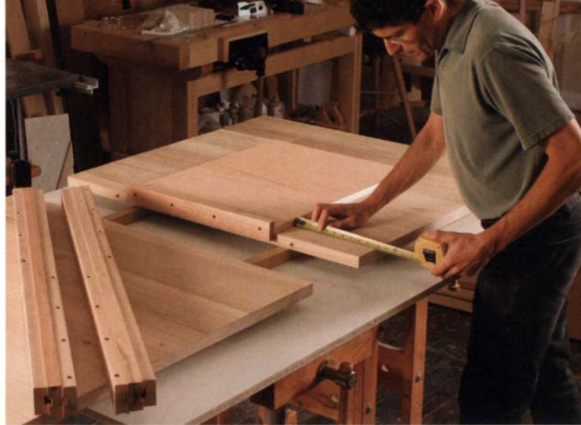
Center the jig. Miller uses a tape measure to help center the jig on one of the top halves.
