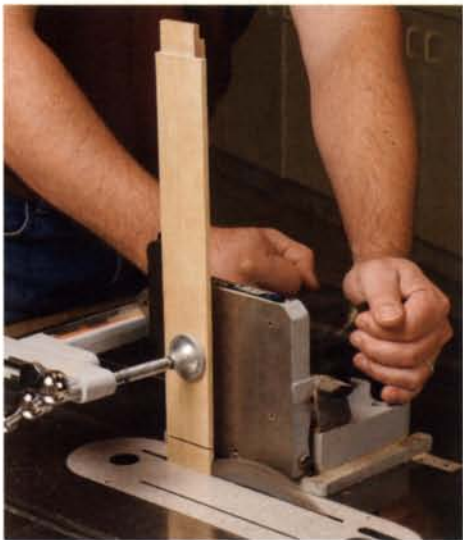
Rail tenons look lopsided. The joinery needs shoulders of different heights to seat properly in the rabbeted stiles.
