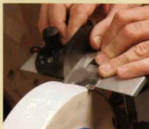
Wet wheels grind nicely but don't hone. On this machine, a small miter gauge keeps the tool square for an accurate grind.
