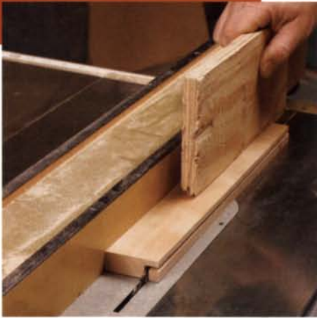
Rabbet all the rails and stiles at once. This means fewer setups on the tablesaw.
