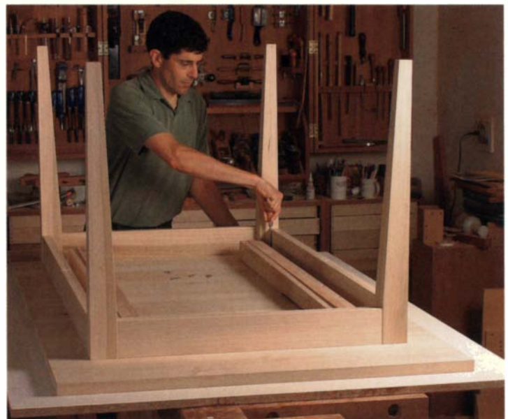
Attach the base to the top halves. With all the parts upside down, Miller mounts the table aprons to the underside of the top halves.
