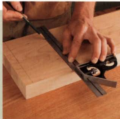
A square and more. Perfect for scribing a square line on boards up to a foot wide, this tool has several other features that come in handy.
