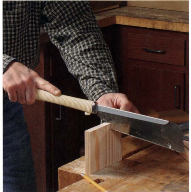
Hold the saw at the far end of the handle. Cut only on the pull stroke, and let the saw's weight do the work.
