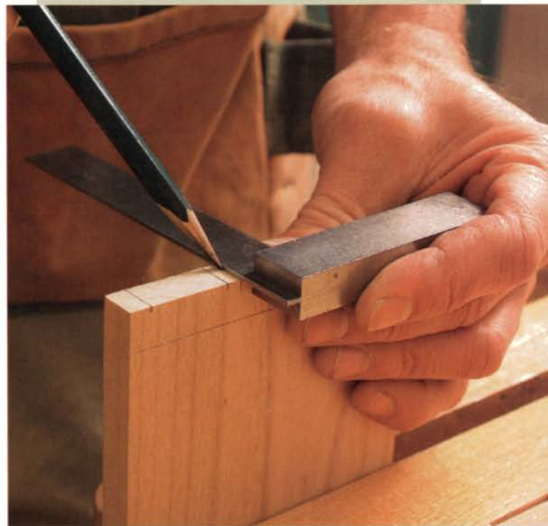
Compact and precise. Small enough to fit into the pocket of a shop apron, a 4-in. engineer's square has a lot of good uses in the shop, including, as shown, scribing the end lines on dovetail joints.
