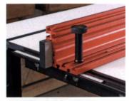
Scale helps with setups. Identical scales on both sides of the table are easy to read from above.
