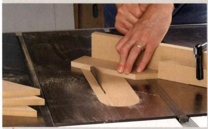
Make a series of cuts. Cut 45° miters at both ends of four pieces of stock, just as you would for a picture frame.
