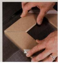
3 Look for the gap. If the final corner doesn't fit snugly, it means the miter gauge isn't set at precisely 45° to the blade.
