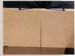
1 The moment of truth. Butt the two cut ends together. Any error will reveal itself as a tapered gap between the two ends.
