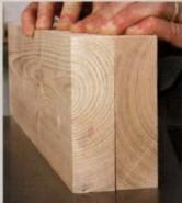
Prepare test pieces. Joint the face and edge of two pieces of stock, checking them on a flat surface. Place the jointed edges down and jointed faces together. A gap shows adjustment is needed.
