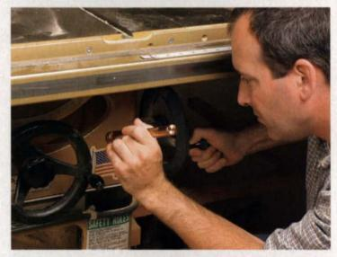
Use a flashlight to look at internal parts. Check the trunnions and trunnion supports, the arbor housing, and the motor mount for damage (top). Turn the wheels (above) and make sure all moving parts work smoothly. Look through the throat-plate opening (right) to examine the arbor and bearings.
