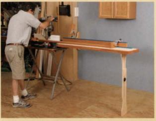
**Good cuts need good support.** A pair of extension wings with stop blocks support long pieces and make for accurate cuts.
