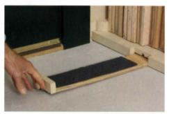
**Protective pad.** The outside bottom corner of sheet goods gets some protection from damage, thanks to a pull-out pad.
