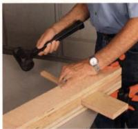
Clamping the leg. When the sections have been glued together. turn the assembly upward and apply the clamps. Waxed paper protects the work surface. When the glue has dried, knock out the taped spacer block with a mallet and a thin piece of wood to reveal the mortise.
