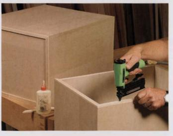
Apply thin banding cut to exact width, using your fingers to align it. Dry-fit each piece first to fit the mitered ends. A 23-ga. micro-pinner leaves almost invisible holes.
