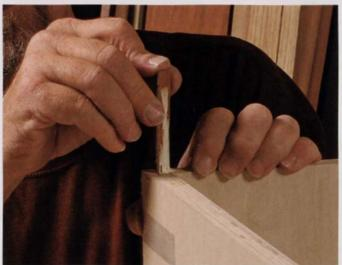
Two pairs of panels make a box. After spreading glue on the miters, stand up the panel assemblies and draw the last two joints together with more tape (above). Apply glue to the spline stock and insert pieces roughly halfway into the joint (left), working from both ends. Nail and glue the back panel into its rabbet, and trim the splines flush.
