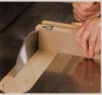
2 A test cut is more revealing. Use two pieces of lumber or medium-density fiberboard (MDF). Stand the pieces on edge and cut them in the same pass.
