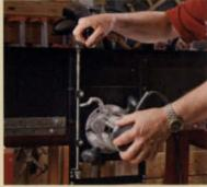
Tilting table adds options. This router table can become a slot mortiser, or standard bits can be used at various angles to produce unique moldings. A crank moves a carriage and the router up or down, and when the table is horizontal, front to back.
