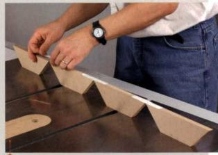
2 Tape the corners. This helps hold the pieces in place as you assemble the frame.
