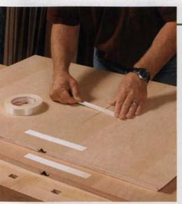
**Packing tape will be your clamps.** For these large boxes, it is easiest to tape up pairs of panels at a time. To close the joints, pull on the tape as you apply it.
