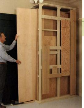
**Choose and use.** This vertical rack makes it easy to flip through the sheets and pull one out without damaging it.
