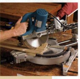
"On the flat." If your saw does not have the capacity to cut wide molding in position, you must lay the molding on the saw's table, and then make a compound-angle cut employing both the miter gauge and the less-accurate bevel gauge.
