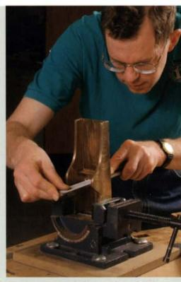
**Opening the mouth.** The mouth needs to be filed open very gradually until the blade just has clearance.
