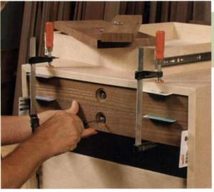
Fit and attach the drawer fronts. Drill a slightly oversize hole in the round mortise for a pan-head screw. Use credit cards to set the gaps, and use the screw to lock the drawer front in place. Then screw the front permanently from the inside, remove the temporary screw, and install the pull.
