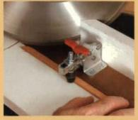
When cutting a short piece, don't try to hold it. Instead, clamp it to the auxiliary fence.
