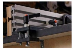
**T-tracks make for a versatile fence.** Commonly available T-track hardware can secure jigs to the Woodhaven fence in a number of spots.
