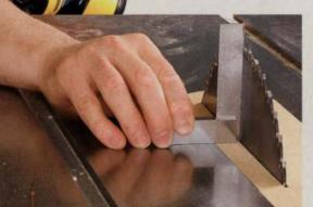
**Start with a square.** An accurate square can help set the sawblade at a 90° angle, but this is only the start of a precise setup. Very small errors can be hard to see with a square alone.
