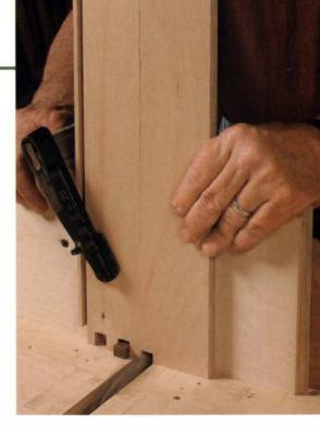
changes in humidity. First, cut the drawer fronts to length and width so that they all fit together into the opening, with no gaps. With all of them in place, mark a centerline for the finger pulls, remove the fronts, and mortise for the pulls. All of the mortising is done easily on the drill press, with just a bit of chisel work afterward.
