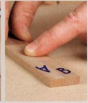
Mark the ends of the strip. This identifies the front and back of the final cut. Make corresponding marks on the MDF square for future reference. Snap the final strip in two, lay the pieces on their sides, and compare the thickness of the two ends. Any variation means the crosscut sled's fence needs adjustment.
