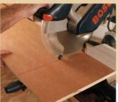
Complete the cut. After flipping the board and ensuring that it is against the stop block, score the uncut section of wood and then make a full-depth final cut.
