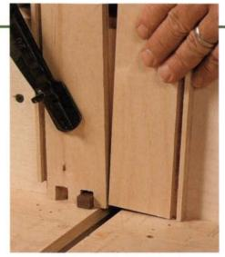
**Locating the mating side.** Flip the first side, put its first notch on the key, and clamp it. Butt the mating side against the first side (above). Cut the first notch on the mating side (right). The dado blade should just clear the first side.
