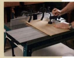
Sliding table carries the workpiece. Clamped by the miter gauge, this panel can be fed at an even rate for smoother cuts.
