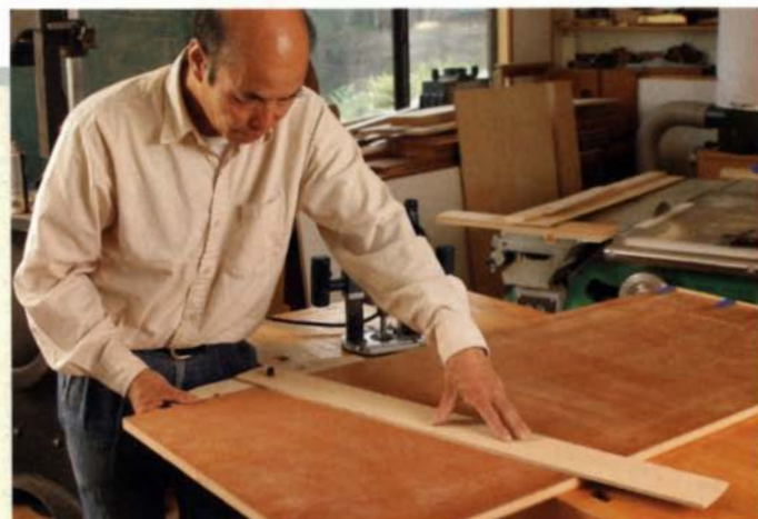
Variable-angle jig. Although dados usually are perpendicular to the long edges of a panel, this jig can make cuts at other angles.
