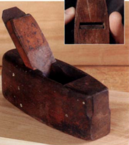
Worn wooden plane. An enlarged mouth will create coarse shavings and result in tearout. A narrower mouth will put pressure near the cutting action, minimizing tearout.
