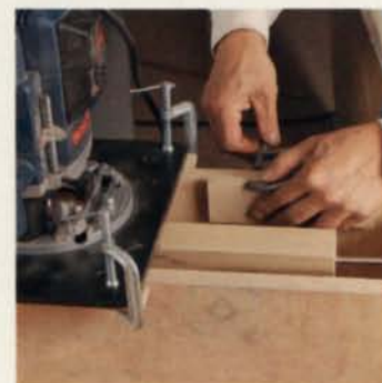
Stopped turnings. Clamp blocks to the side of the jig to leave a square section on the turning.
