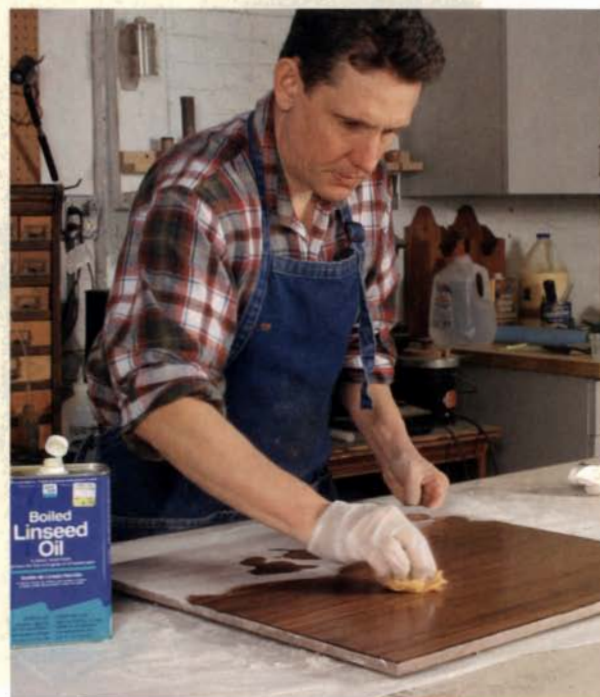
Work fast with this filler. Pack the pores quickly, working in one small section at a time (top). When the surface feels dry, remove the excess with a damp cloth (above).
