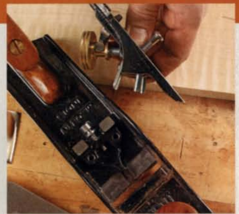
Classic Bailey-style design. The adjustable frog on the Anant plane allows for easy vertical and lateral adjustments.
