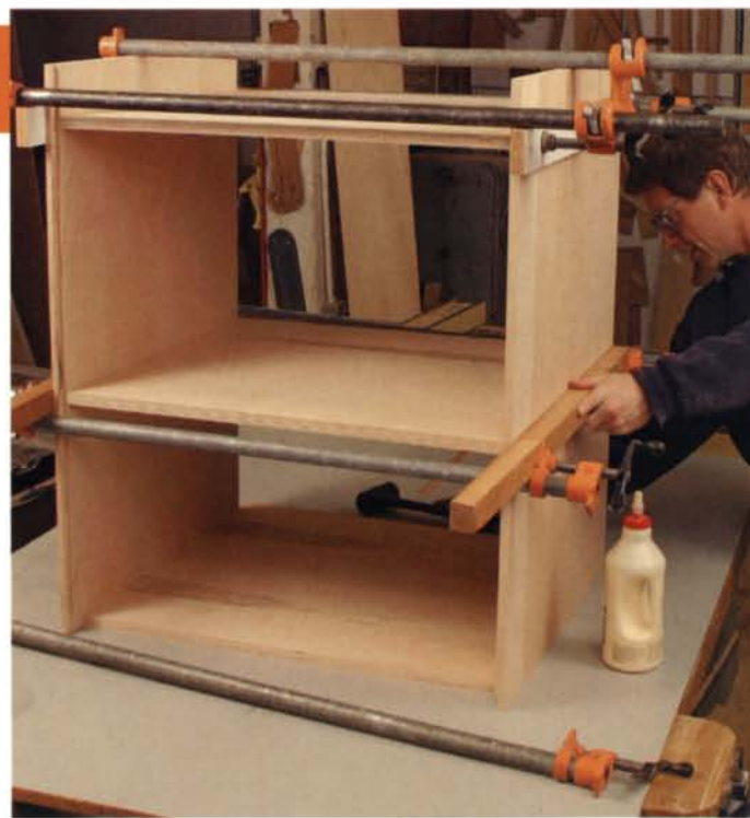
Glue large cases in stages. Here the case is upside down, and the top panel is only dry-fit in its rabbet, while the other panels are glued. To apply pressure along the entire edge of the middle shelf, Rogowski uses a convex caul.
