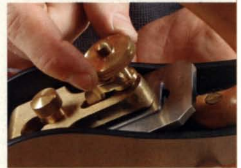
Simple to adjust. The knurled knob on the Lie-Nielsen No. 164 plane serves as the depth-of-cut adjuster.
