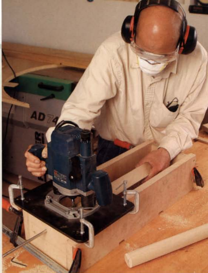
Router-cut turnings. By guiding the router back and forth while turning the workpiece, a square blank gradually becomes a cylinder.
