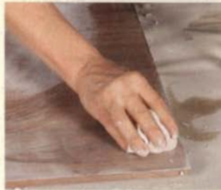
Work fast with this filler. Pack the pores quickly, working in one small section at a time (top). When the surface feels dry, remove the excess with a damp cloth (above).
