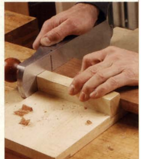
Well-designed for use with a shooting board. Dimples in the square body make the Veritas easy to hold while on its side.
