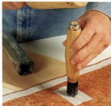
A cloud-shaped punch is best for burl. This type of punch is commercially available or can be made by hand from steel pipe.
