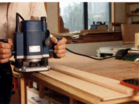
Straighten edges. Rough-cut the panel, then clean up the cut with this straight-edge jig.
