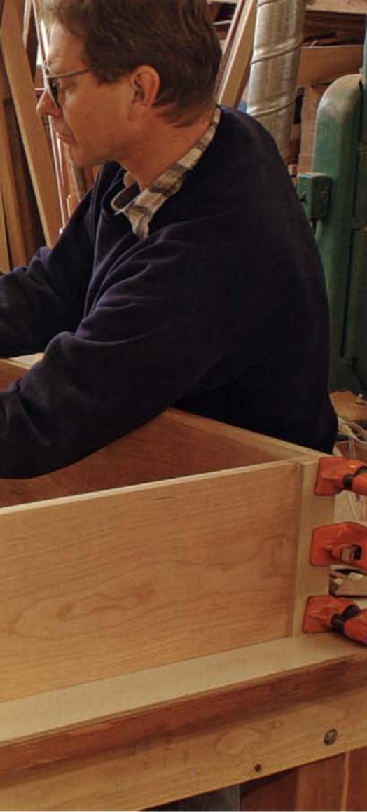
Use melamine cauls and check the diagonals. On dovetails, Rogowski keeps the long grain proud, which allows him to use flat cauls. Later, he planes the sides flush with the pins and tails. If the diagonals don't match, use a long clamp to draw the assembly square.
