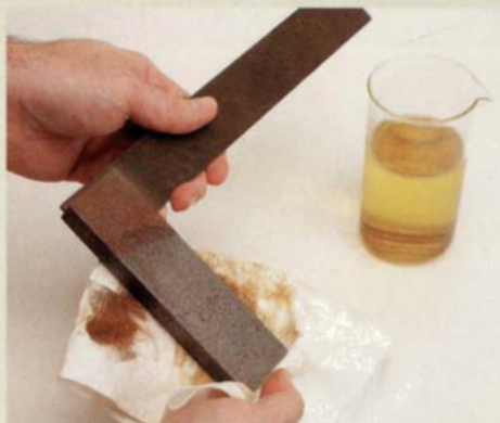
Let it soak. For Evapo-Rust to do its job, rusted metal must be immersed in the solution for 20 minutes or more.
