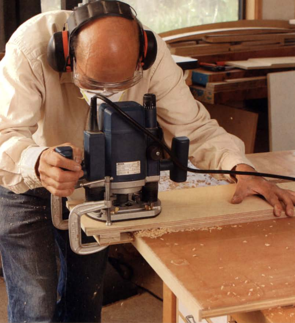
Flush-cut edge-banding. This jig allows you to cleanly cut solid-wood edge-banding flush with the plywood panel.
