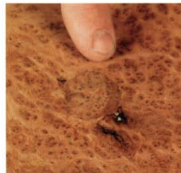
Flip over the leaf to inspect your work. A good patch will blend into the surrounding material.
