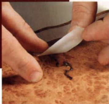
Tape over the void to prevent it from checking. Work the sheet with the face side up and never leave tape on the underside.
