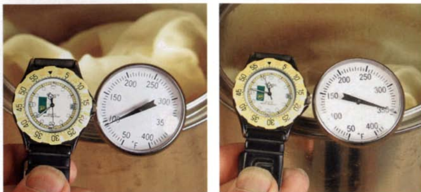
Heating up fast. In seven minutes, the internal temperature of this wadded-up cloth soaked in linseed oil rose from less than 100°F to 350°F and started to smoke (above). Less than five minutes later, the temperature rose from 350°F to almost 500°F, and the cloth caught fire (right).
