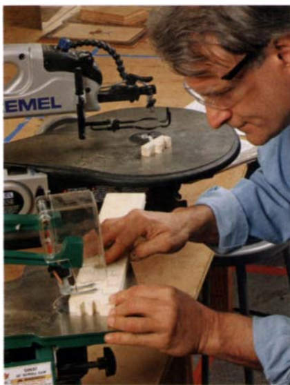
Schürch used each saw to make a variety of cuts in a variety of common materials. He graded the smoothness of cut by feel and by looking at the cuts under magnification.
