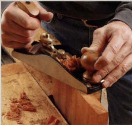
Low-angle planes excel at slicing end grain. Dampening the stock with paint thinner will help reduce tearout.
