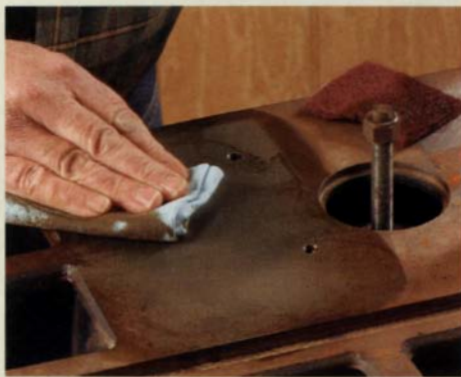
TopSaver requires some elbow grease. Spray the solution on the surface and scour it vigorously with synthetic steel wool. More than one application may be necessary.
