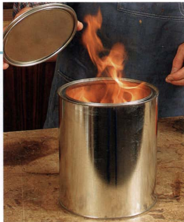
Heating up fast. In seven minutes, the internal temperature of this wadded-up cloth soaked in linseed oil rose from less than 100°F to 350°F and started to smoke (above). Less than five minutes later, the temperature rose from 350°F to almost 500°F, and the cloth caught fire (right).
