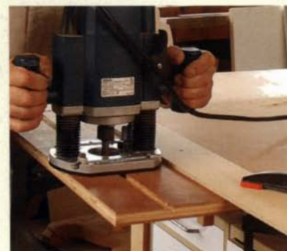
Cut clean and accurate dados. Clamp the dado jig at both ends and make the cut in two or three passes.
