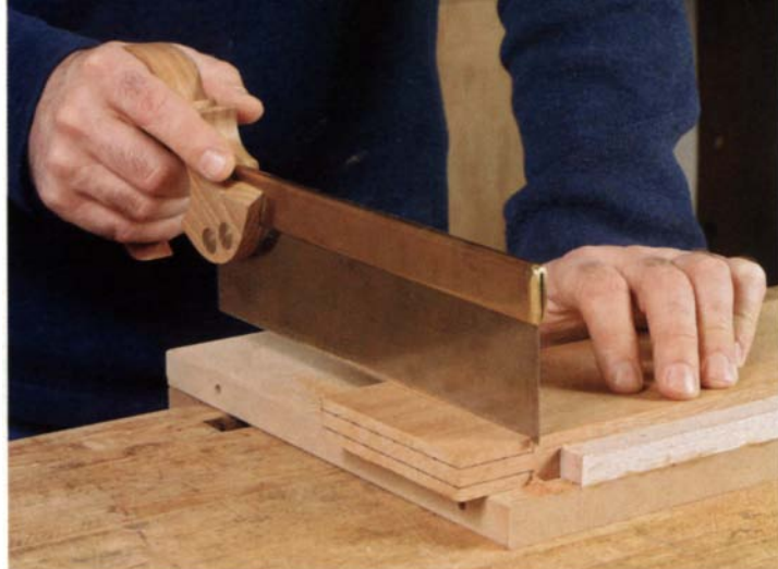
Made the old-fashioned way. The thin steel blade is made rigid by a folded brass back on these tenon saws, which also excel at dovetails.
