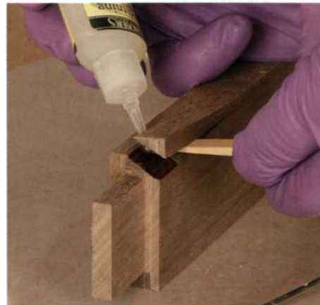
Cyanoacrylates need very little setting time. Within a minute of making a quick repair, you'll be able to go back to work.
