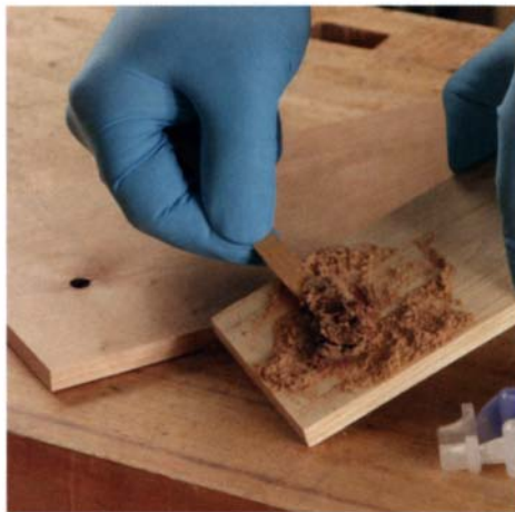
Filling knots with sawdust and five-minute epoxy. Not only does the glue secure the knot, but also it fills the gap and will accept tints and finishes.
