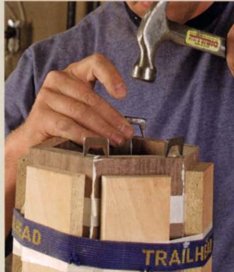
Roll up and clamp the column. Lay all of the staves with their outside faces up and tape them together. Then flip them over in concert and apply glue to the joining edges. Roll up the column (left) and apply pressure to the joints with strap clamps. Zeitoun also uses steel pinch dogs from Lee Valley to help draw together the pieces at the joints (above).
