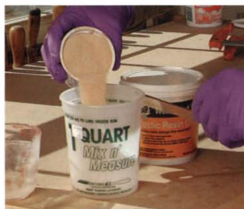
Prepare water and powder quantities separately. Add powder to a portion of the water, then add the remaining water.
