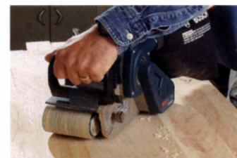
For coarse- to medium-grit paper, there is very little difference between the two grading systems.
