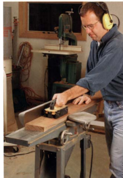
A good performer at a reasonable price. A 6-in. jointer can flatten and edge-joint most boards and costs considerably less than an 8-in. jointer.
