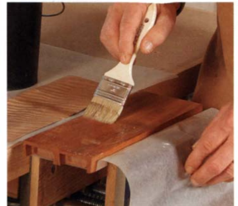
Hide glue starts to set as it cools. Apply glue on both bonding surfaces, the substrate (above) and the underside of the veneer.
