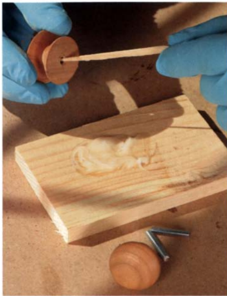
Metal meets wood. Epoxy forms a strong bond between dissimilar materials.
