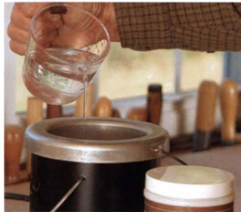
Dried hide glue needs water and heat. A dedicated glue pot will keep the glue at the optimum temperature of 140°F.
