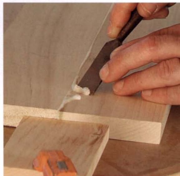
Wait six to eight hours before cleaning up squeeze-out. Once hardened, polyurethane foam is removed easily with a chisel.
