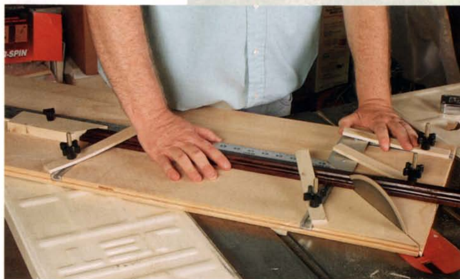
The second cut. Clamp the molding to the long fence and set the stop block at the correct distance from the blade (above). Then cut the left-hand miter (below).
