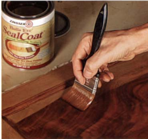
Seal the dye with shellac. After the dye has dried, brush on a thin coat of dewaxed shellac such as Zinnser's SealCoat.
