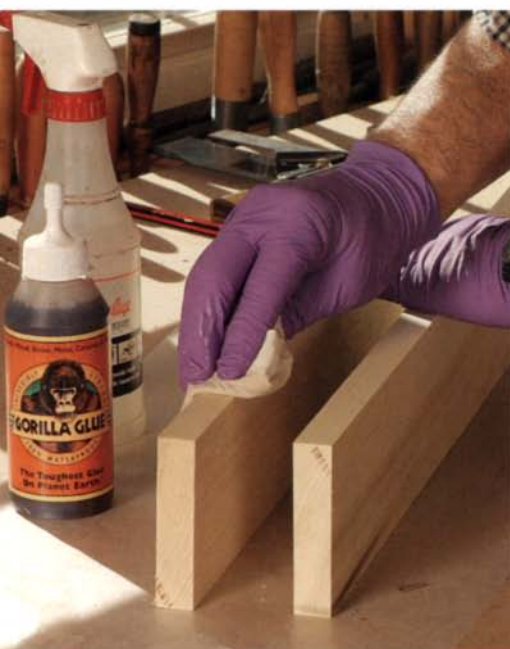
Moisten mating surfaces. Polyurethane glue needs moisture to cure, so use a damp cloth to wipe down both surfaces if using hardwood.
