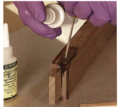
Accelerators speed up the already fast-bonding glue. No clamps are needed when using an accelerator.
