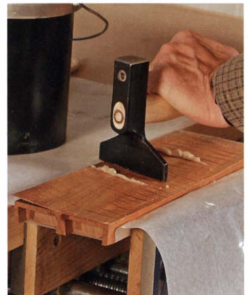
Rub the veneer with a veneer hammer. The glue on the veneer acts as a lubricator. Starting from the center outward, apply steady pressure with the edge of the hammer.
