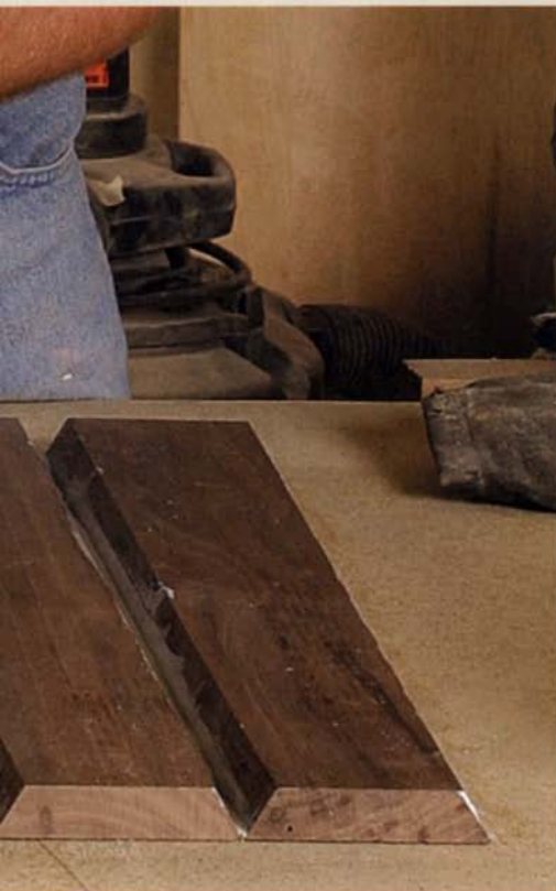
Roll up and clamp the column. Lay all of the staves with their outside faces up and tape them together. Then flip them over in concert and apply glue to the joining edges. Roll up the column (left) and apply pressure to the joints with strap clamps. Zeitoun also uses steel pinch dogs from Lee Valley to help draw together the pieces at the joints (above).
