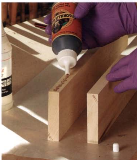
Apply glue sparingly. Polyurethane glue creates a very thin bond line, but squeeze-out will foam up when exposed to air.
