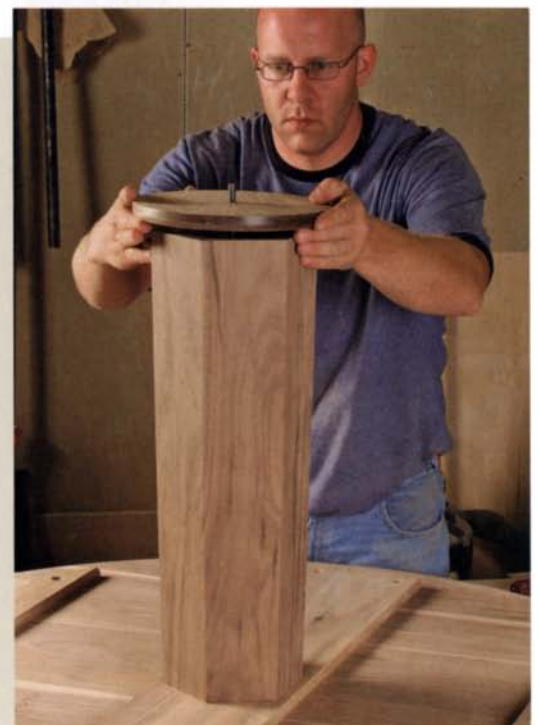
Assemble the table. A threaded steel rod feeds through each section of the table. Secure the nut at the top with Thread Lock, then tighten the nut at the bottom.
