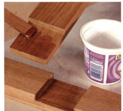
Ideal for oily woods. Epoxy will provide good bonding and plenty of strength for this lap joint made with teak stock.
