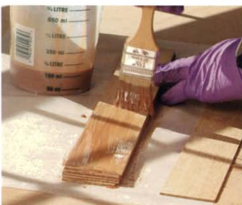
Apply a thin layer of glue. When gluing up laminations, apply glue to only one face of each piece.
