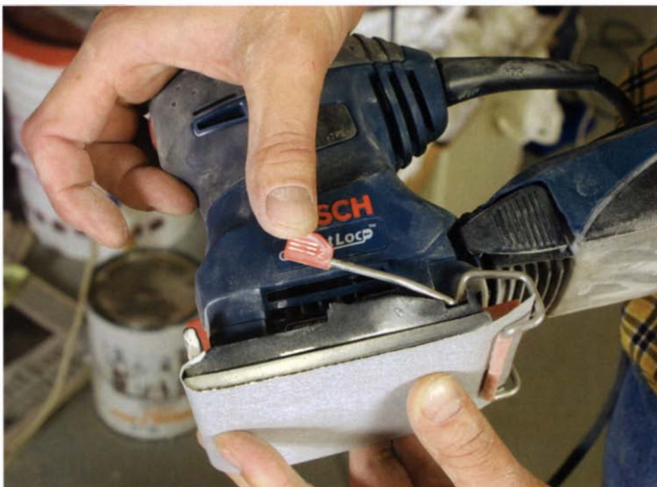
A locking lever. With the SheetLoc system, a spring-loaded device on the front of the tool holds one edge of the paper in place. Then a steel bar draws the paper tight and secures it to the sander.
