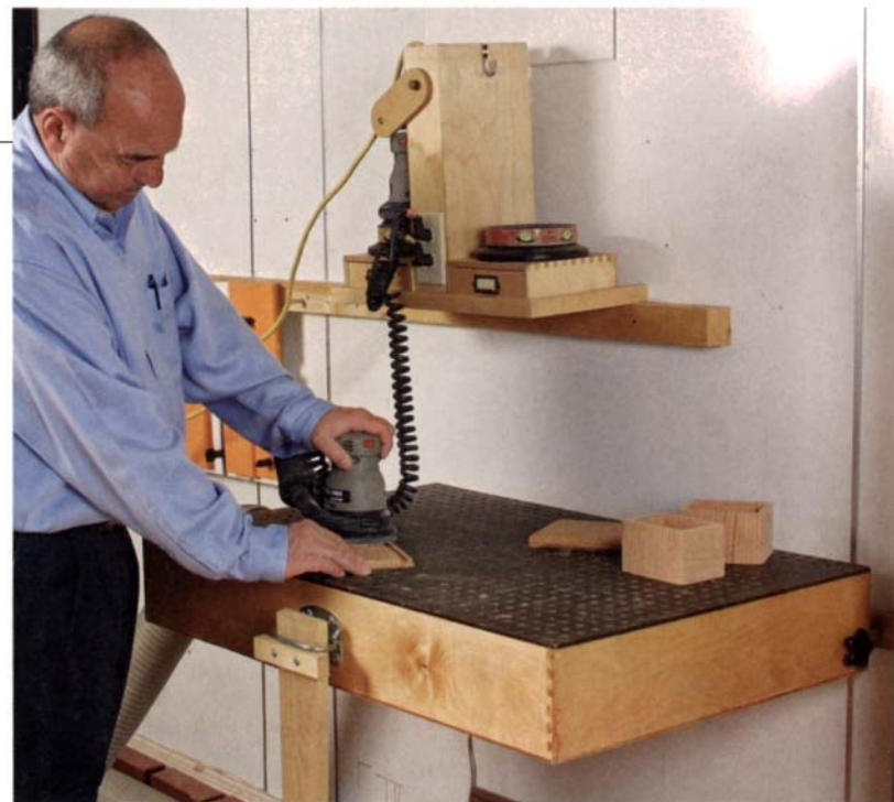
Handle doubles as leg connector. The handle not only is used to lift and lower the table, but it also connects the leg to the table.
