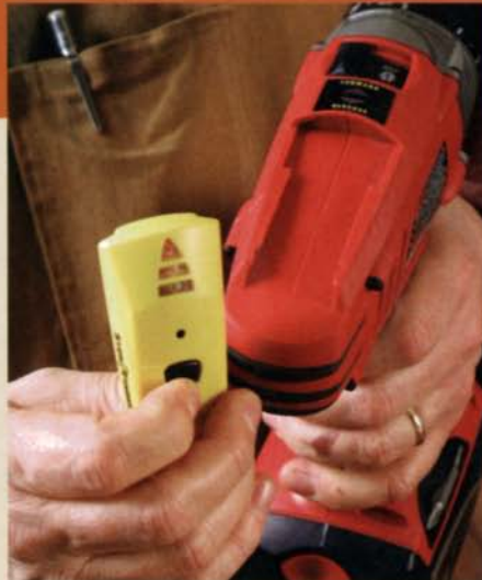
Bells and whistles. Skil wins the prize for the most doodads on its drill-driver, including a removable stud finder, which also lights up when the drill is in use.
