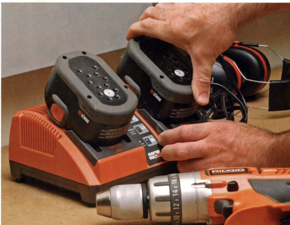
Charge it. Nearly all of the drill-drivers tested come with a single, one-hour battery charger. The Ridgid is an exception; it recharges two batteries at a time and takes only a half-hour for each.
