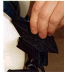
Gauge sets bevel angle. Setting the bevel angle on the Veritas is easy, thanks to a gauge (left) that comes with the tool rest.
