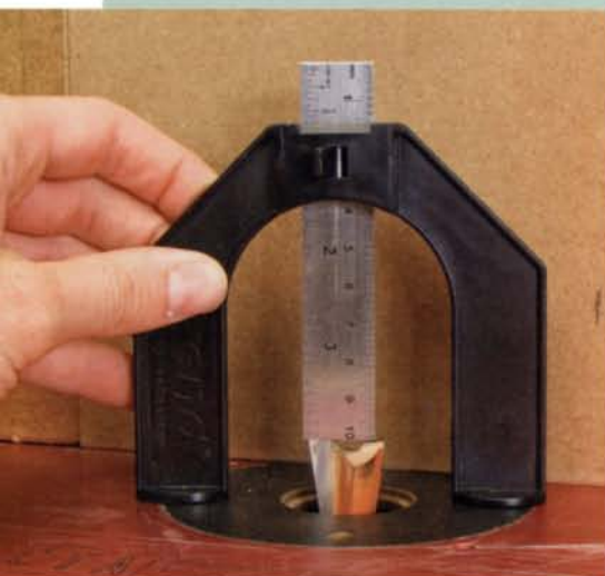
Simple but effective depth gauge. The cam lever at the top of the tool locks the stainless-steel rule in place.
