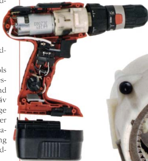
Black & Decker's transmission assembly is mostly plastic, but metal is used for select components.
