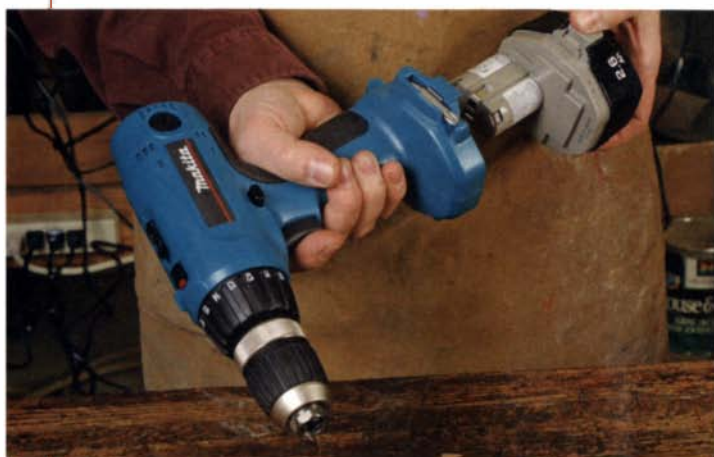
Drop-release batteries. About half of the drill-drivers tested have batteries that drop from the handle. This design can be cumbersome if the battery is large, as you have to stretch your hand around the battery to release it.
