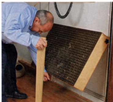
Down and out of the way. Simply removing the leg allows the table to fold flat against a wall.
