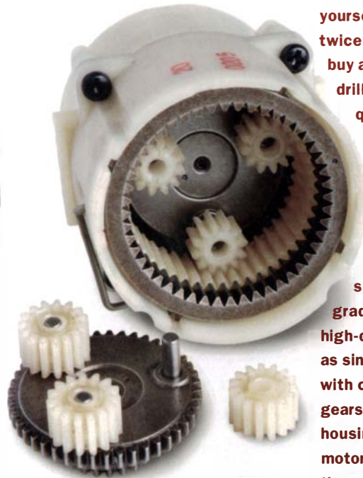
Black & Decker's transmission assembly is mostly plastic, but metal is used for select components.
