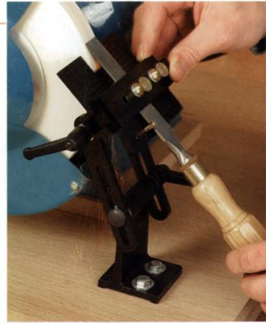
Gauge sets bevel angle. Setting the bevel angle on the Veritas is easy, thanks to a gauge (left) that comes with the tool rest.
