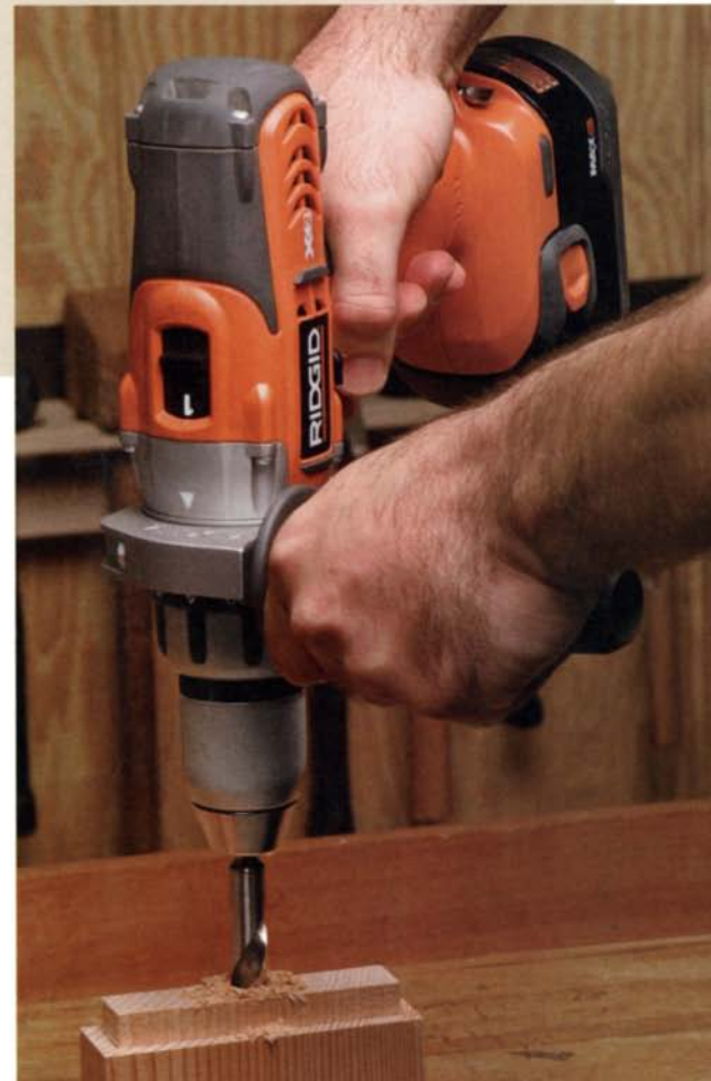
Get a handle on your drill. The Ridgid, as well as the Milwaukee and Bosch, comes with a removable auxiliary handle that provides extra leverage when boring large holes or driving large screws.
