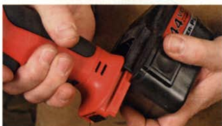
Better balance. The Milwaukee is one of several drill-drivers with a battery that slides on and off. The battery on the Milwaukee is unique in that it can be mounted in two directions (bottom) to change the center of balance for different operations.
