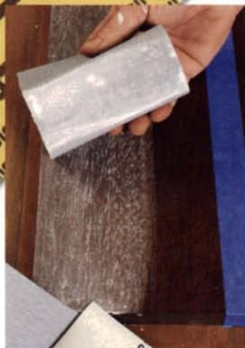
Generic sandpaper clogs fast. After just a few passes, this standard grade of 320-grit paper has already lost its cutting power, and finish has lumped on the paper.
