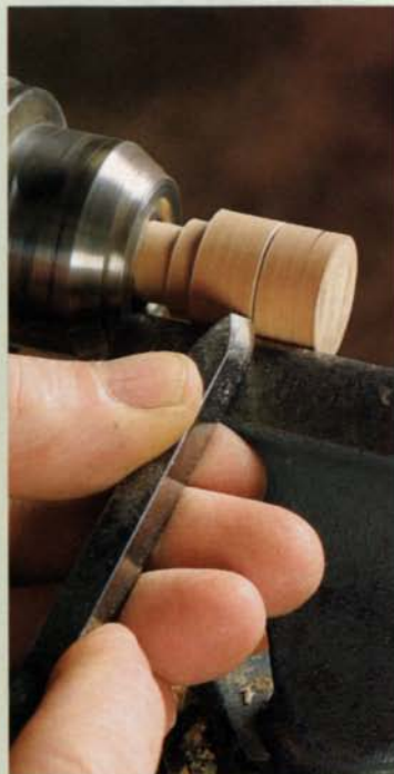
Mark for the cove and bead. Cut grooves at the pencil marks with a skew.
