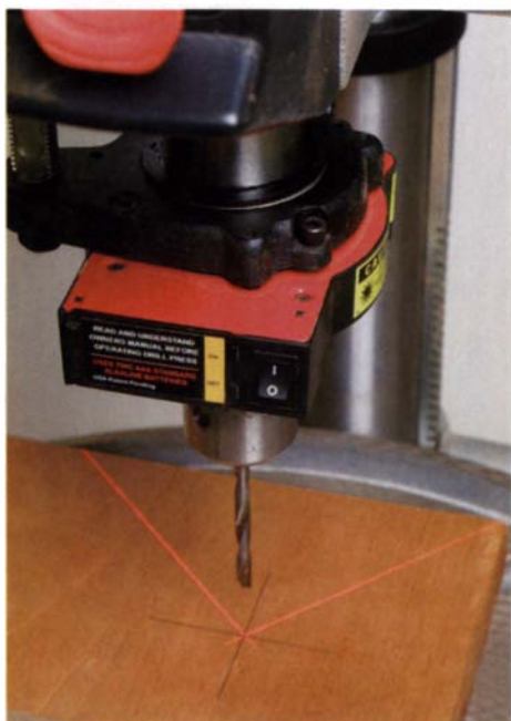
"X" marks the spot. Because the intersecting laser lines are directly in line with the centerpoint of the bit, it's an easy matter to align the bit with a hole to be drilled.
