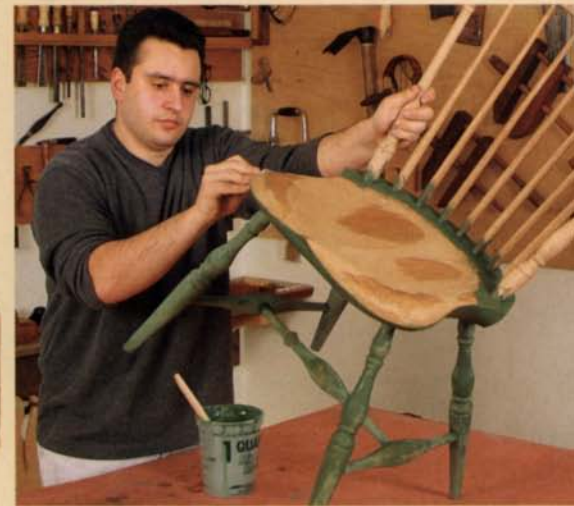
Wax the wear areas. Rub paste wax onto those areas of the chair that get rubbed the most during normal use.
