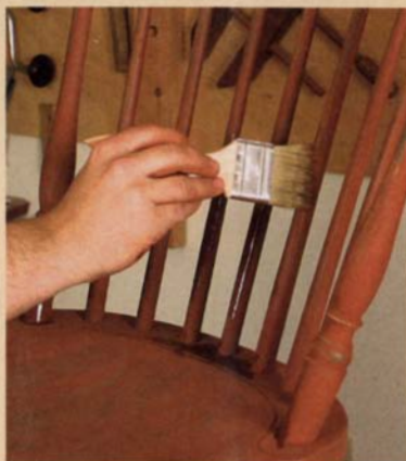
Secret to making an ancient-looking crackled finish. Apply hide glue or Antique Crackle to small areas only. Then apply wax and the last coat of paint.
