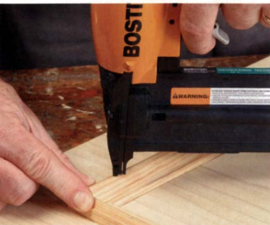
Smallish nose is a plus. A small nose on the Bostitch BT200K-2 allows the user to place nails more precisely.
