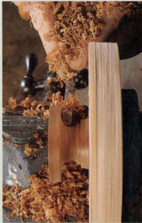
Turn the cove with a rounded scraper. The cove is asymmetrical and spans from the base diameter to the major diameter of the knob.
