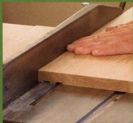
Cut grooves for the lower track. These shallow grooves can be cut directly into the cabinet bottom.
