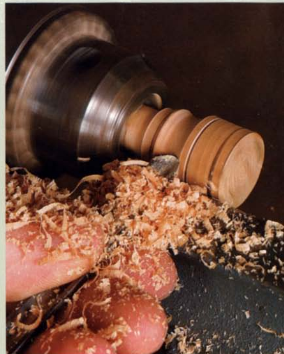
Turn the cove. Use a spindle gouge to turn the asymmetrical cove, also known as a scotia.
