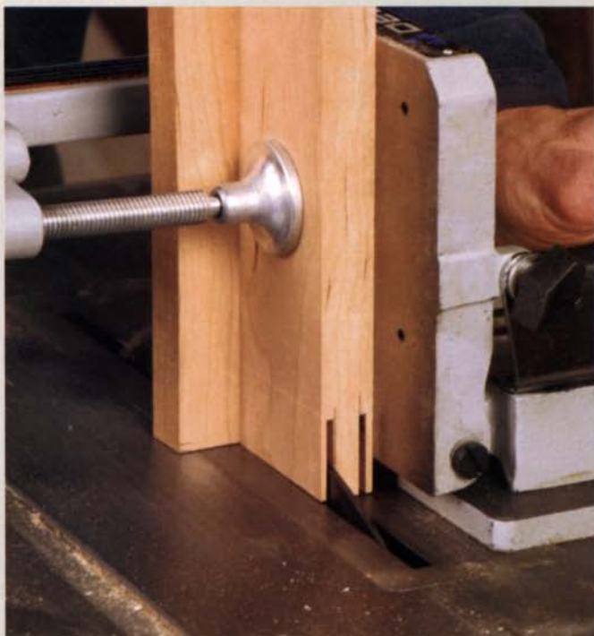
Spacer-free second cut. After making the first cheek cut, remove the spacer and slide over the workpiece to clamp it directly against the jig.
