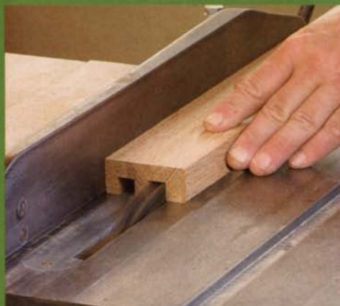
Cut grooves for the upper track. These are deeper than the lower ones and go in a separate piece so as not to weaken the cabinet top.
