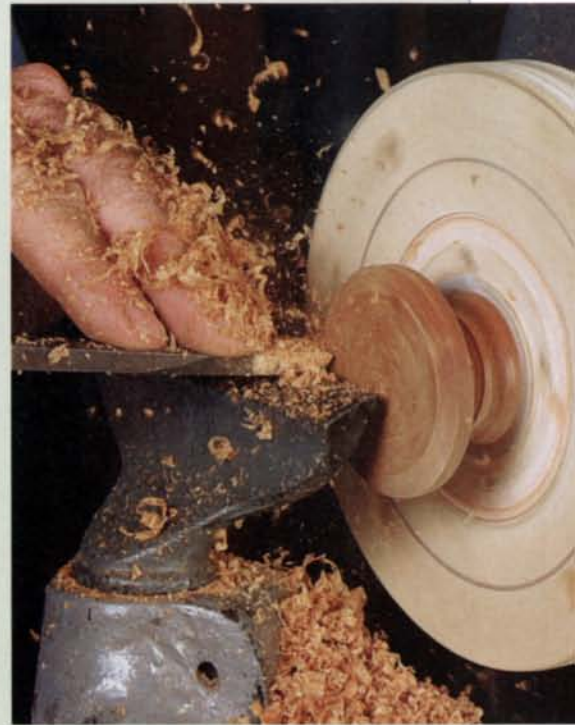
Round the face of the knob. Use a scraper to round over the face of the knob. Polish the shape before sanding to a finish.
