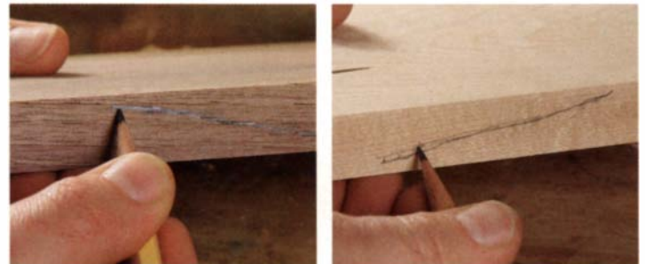
The direction of the vessels on this piece of walnut (left) indicates the direction of the grain and determines which way the adjacent surface should be worked. On a maple board (right), the figure points the way.
