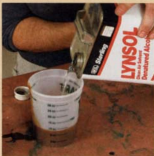
Set fire to your finish. Prepare a 1-lb. cut of shellac (above). Brush it on and have a friend immediately set it on fire (top right). The alcohol will burn off in a few seconds and leave the paint oxidized and aged-looking. Then rub a mixture of paste wax and roofing cement over the whole chair (bottom right) to complete the aging process.
