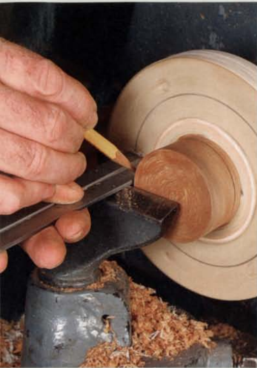
Lay out the elements of the knob. After turning the workpiece round, locate and mark with a pencil the beginning and end of the fillet, cove, and bead.
