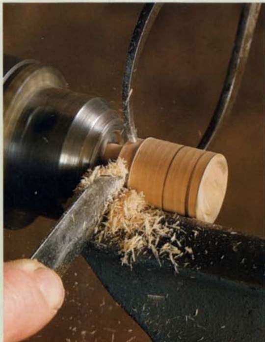
Remount a knob blank. Clamp the tenon end in a Jacobs chuck and turn the base of the knob to a diameter greater than that of the tenon.
