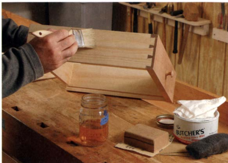
Use shellac on drawer parts. A light finish on the sides, back, and bottom seals the wood, and a light coat of wax ensures smooth operation.
