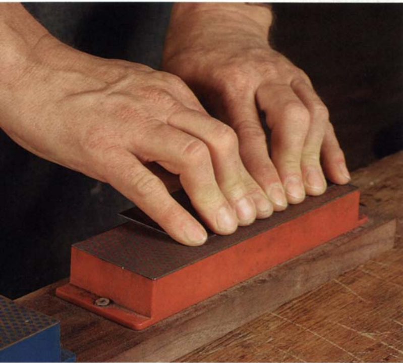
Hone the sides of the scraper. Polish the sides of the scraper on a fine diamond plate or sharpening stone.
