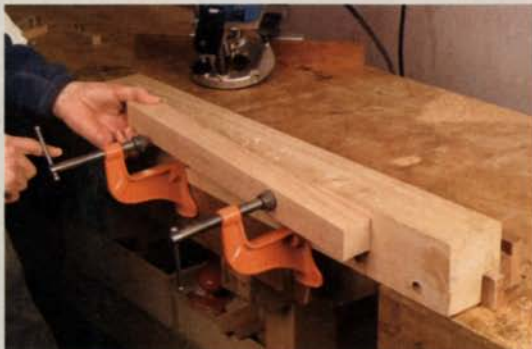
Clamp the workpiece to the mortising jig. A pair of sturdy hold-downs anchors the workpiece to the jig.
