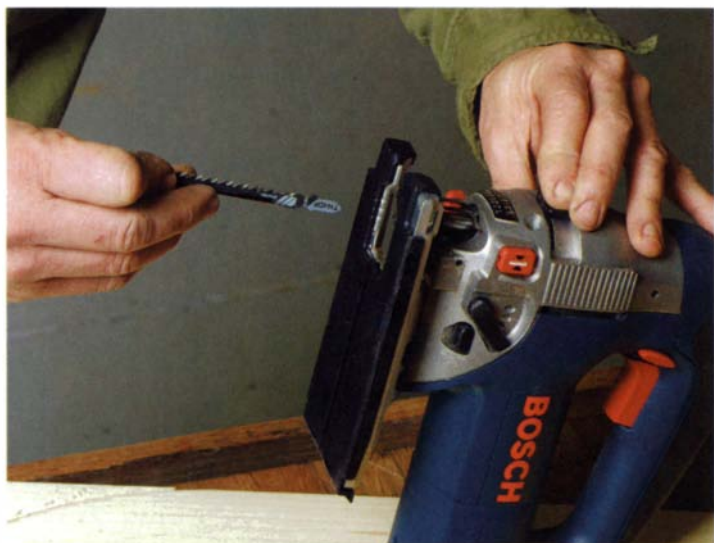
No-fuss blade changing. It's quick and easy to change blades on Bosch's new 1590EVSK jigsaw.
