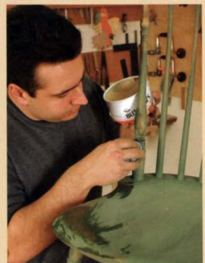
Rub off the loose paint. Use a green abrasive pad to smooth the whole chair and remove loose paint from areas that were waxed (above). Rewax the same areas as before, but allow the wax to cover a slightly larger area so that some of the green paint will be revealed under the second coat of paint.
