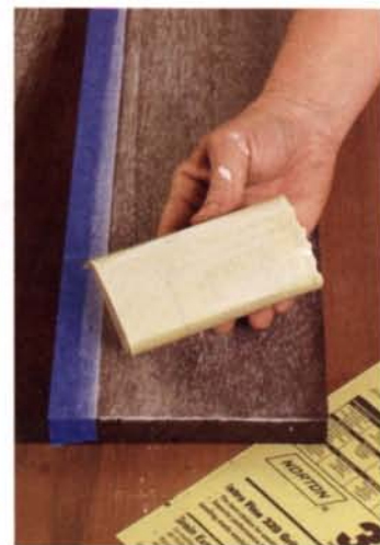
Norton's 3X paper is better. This piece of 320-grit paper is still sharp and displays no evidence of clogging, even after sanding a 6-in. by 30-in. section of a board.
