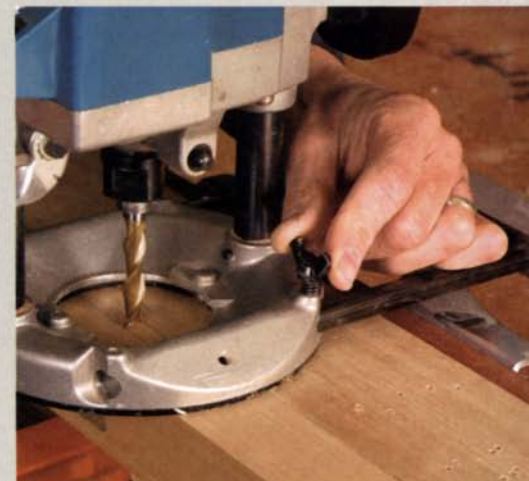
Center the bit. After marking the location of the mortise, adjust the edge guide to center the bit in the mortise.
