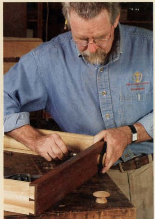
Cross-grain knobs. Use a screw with the same threading as the one used to mount the knob in the faceplate.
