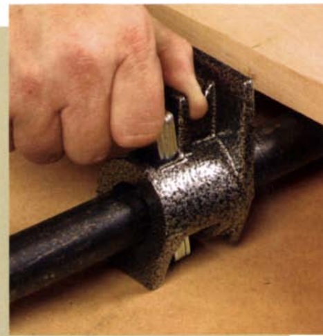
Columbian/Wilton's tail problem. When used on a benchtop, the tail on this pipe clamp is very difficult to disengage. Albers had to reach under the clamp to unlock the clutch plates.
