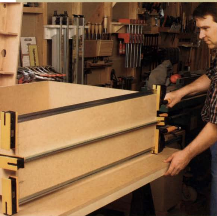
Parallel clamps offer long, accurate jaws. For some glue-ups, this means fewer clamps are necessary to apply even pressure along the glue joints.
