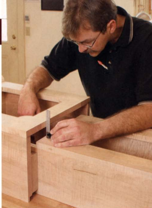
Attach the waist to the base. Where the waist sides extend down into the base cabinet, use plenty of glue and screws to secure the two cases to one another. Position them carefully before driving the screws through the waist sides into the glue blocks in the base. Once the glue sets, the waist and base become one cabinet. The bottom cove molding will conceal the gap between the two components.
