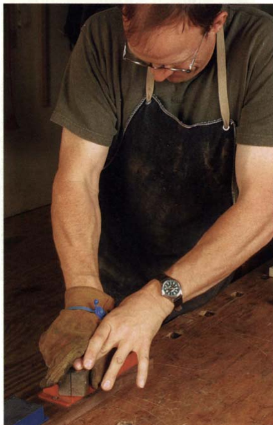
Hone the edges. A guide block helps hone the edges of the scraper 90° to the sides. The scraper should fit loosely enough that it can be pushed onto the sharpening stone.
