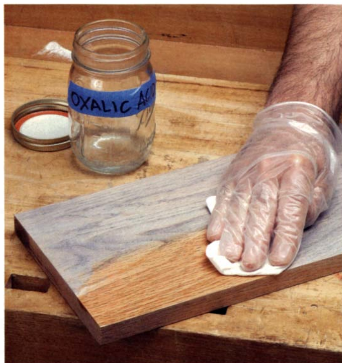
Oxalic acid will remove the blue stain. This piece of oak, which was wetted to raise the grain and then rubbed down with steel wool, has turned blue. To get rid of the stain, apply a solution of oxalic acid.
