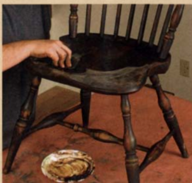
Set fire to your finish. Prepare a 1-lb. cut of shellac (above). Brush it on and have a friend immediately set it on fire (top right). The alcohol will burn off in a few seconds and leave the paint oxidized and aged-looking. Then rub a mixture of paste wax and roofing cement over the whole chair (bottom right) to complete the aging process.
