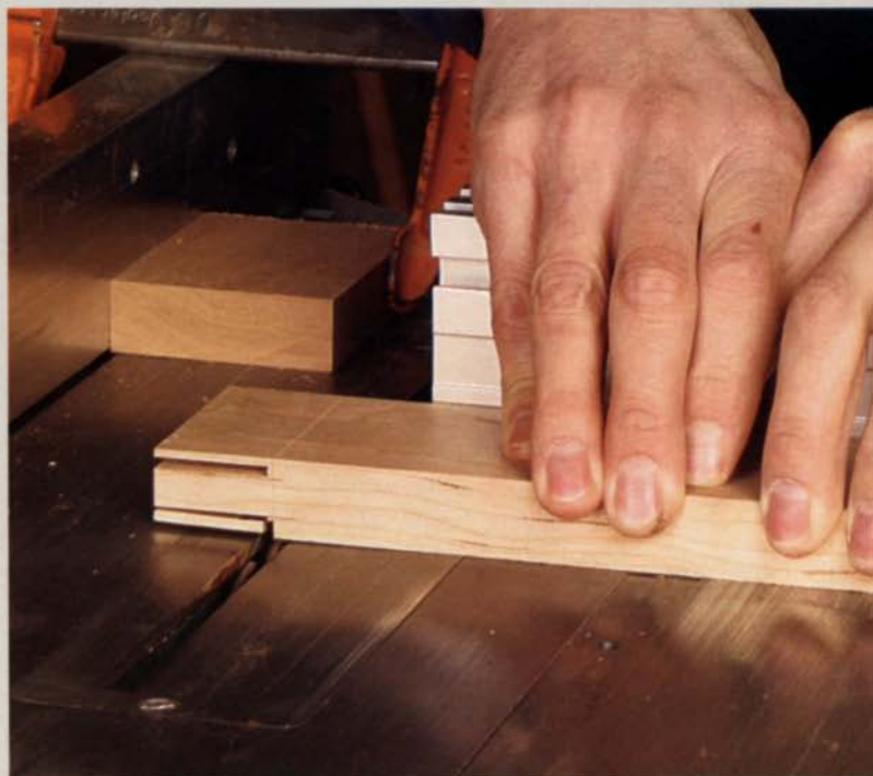
Use the miter gauge and a stop block. For consistent tenon shoulders, clamp the stop block to the rip fence and make the shoulder cuts using a miter gauge.
