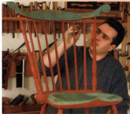
Secret to making an ancient-looking crackled finish. Apply hide glue or Antique Crackle to small areas only. Then apply wax and the last coat of paint.
