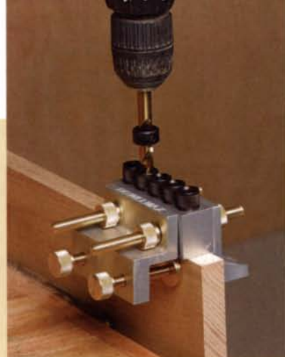
Upscale doweling jig. The Dowelmax jig produced precise dowel joints for our reviewer.
