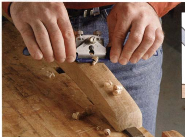
Spokeshave cuts with a chisel edge. The angle of the blade allows it to slice wood as a handplane does.
