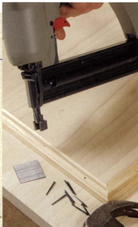
Small nails driven with a nail gun leave holes similar in shape to those left by cut nails driven with a hammer.
