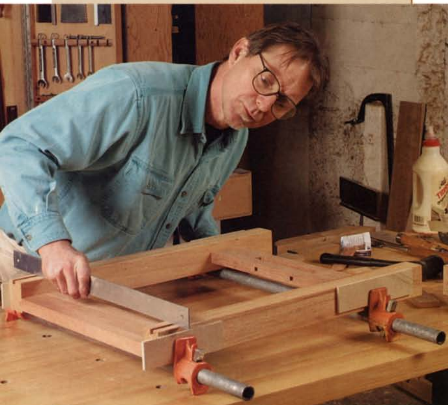
Assemble the table sides. Apply glue to the tenon cheeks and the mortise walls and then assemble each side separately, checking to make sure they go together square and true.
