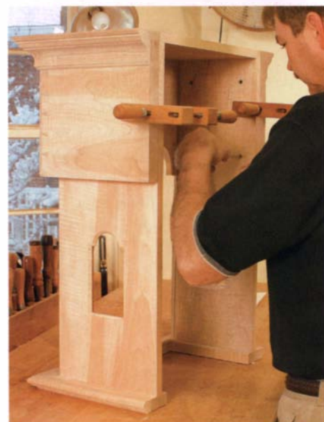
Screw the pediment to the hood. Because of the cross-grain construction, do not glue the pediment assembly to the hood. Instead, use screws through large pilot holes, which will allow some seasonal wood movement.
