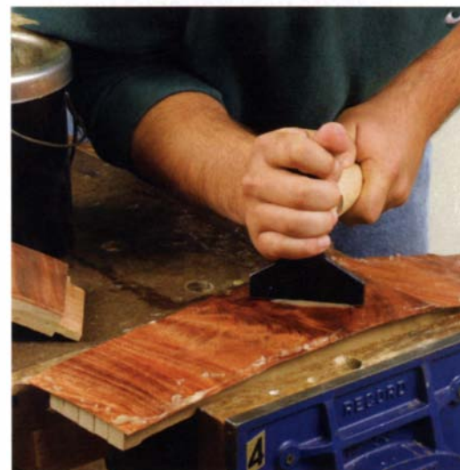
Scuff the surface and apply glue size. Rough up the substrate with coarse sandpaper. Then brush on a size, a watered-down coat of hide glue, and let it dry.
