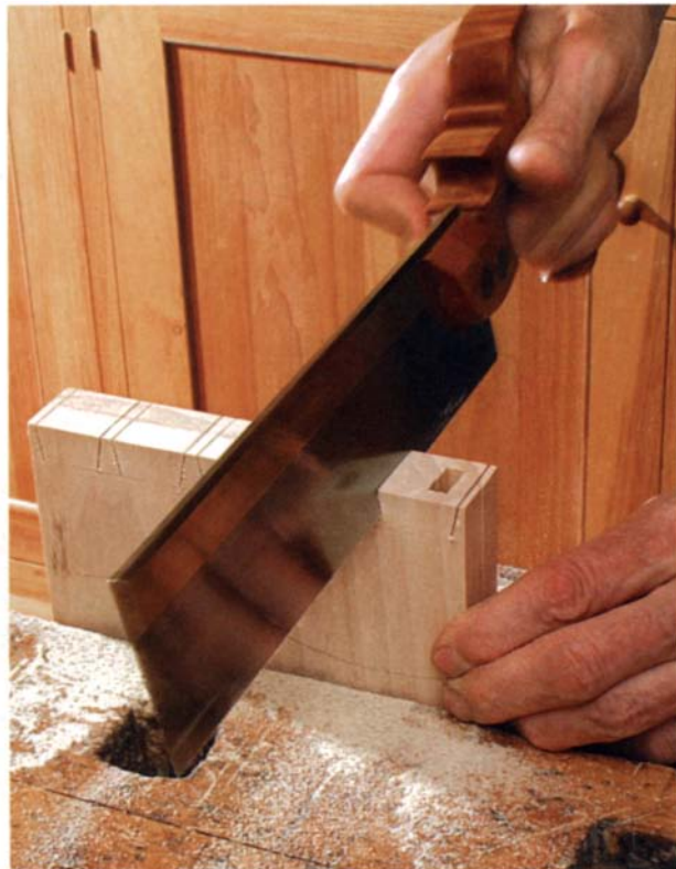
Make the tail cuts in both workpieces. By cutting the tails in both pieces at the same time, it's actually easier to maintain the sawkerf at 90° to the face of the boards.
