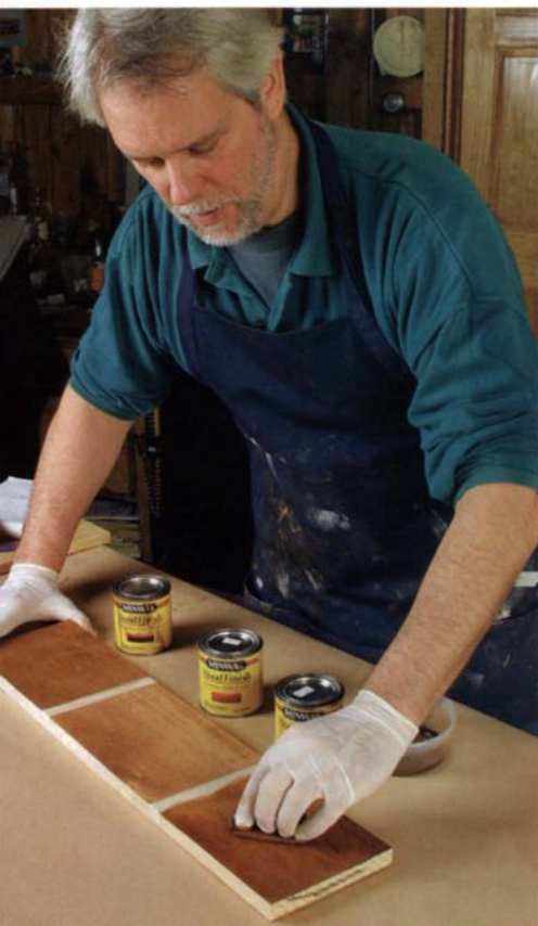
Always make a sample board. When mixing colors, it is important to test them on scrap-wood before applying them to the workpiece.
