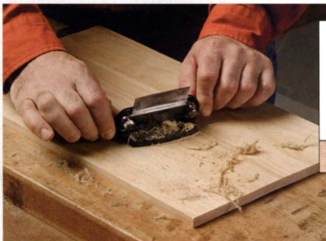
Scraper cuts with a burr. A scraper plane holds a blade at an angle that causes a scraping action from the burr of the blade.
