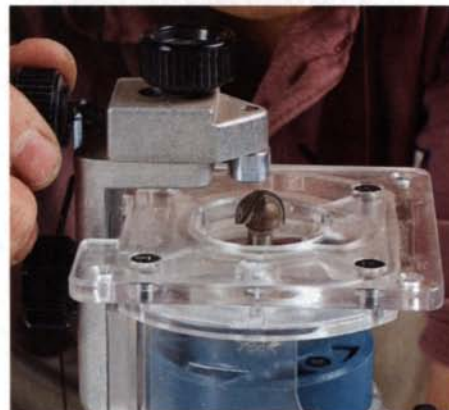
A better view. A clear plastic base and sub-base and lights built into the motor housing improve your view of the cutting action.
