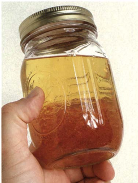
Shellac shelf life can vary. If dry shellac gets old or is packed poorly, it will polymerize, leaving an undissolved glob in the bottom of the jar.
