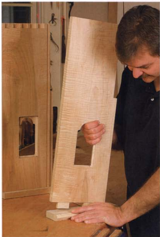
Dry-fit the hood parts before final assembly. The hood sides anchor to the base frame with two through-mortises per side. Cut the mortises before assembling the three-sided base frame, and test the fit of all the hood pieces before gluing them together.
