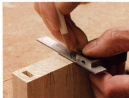
Transfer the tail marks. Use a pencil and a small square to lay out the tails across the ends of a pair of drawer sides.
