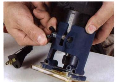
Locking in the vertical adjustment. The motor is secured to the base with a wing nut that can be difficult to tighten.
