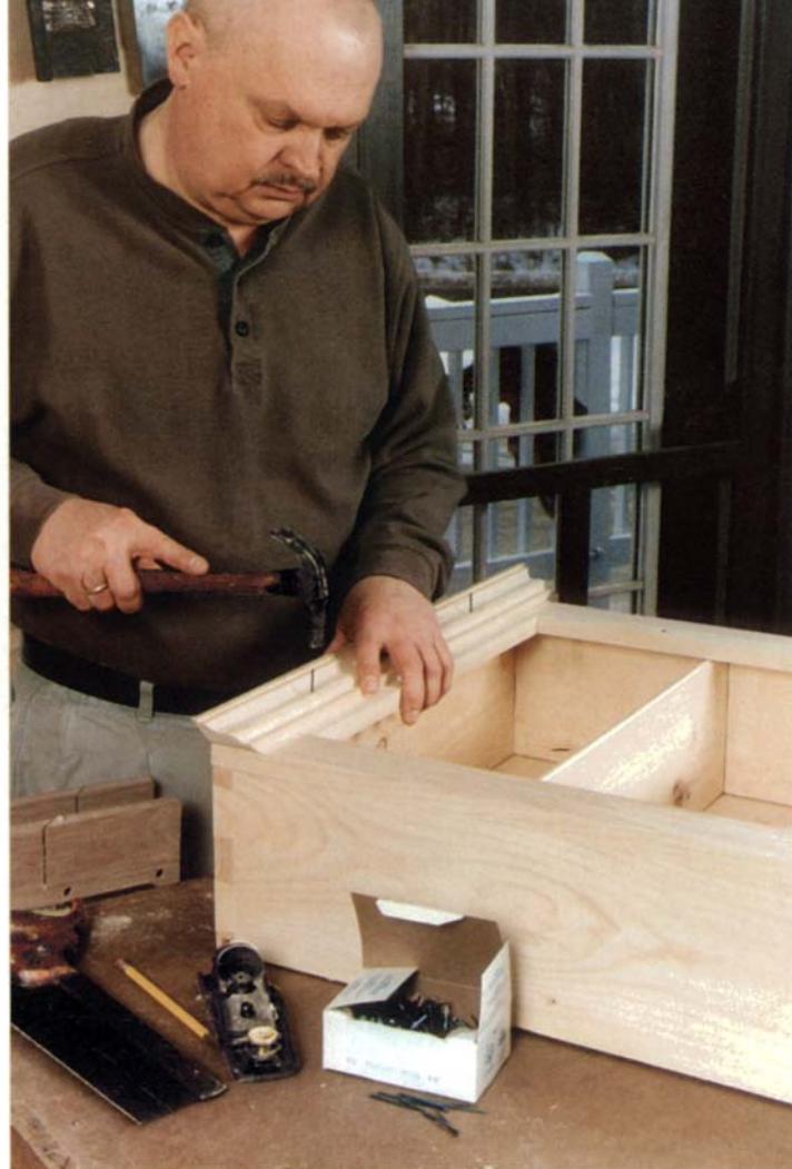
Nails hold moldings in place while glue dries. Using only nails on the side moldings allows the case sides to shrink and expand.
