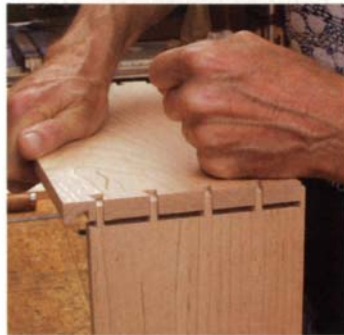
Test the fit. Use your fist to engage the two workpieces, and then pull them back apart.
