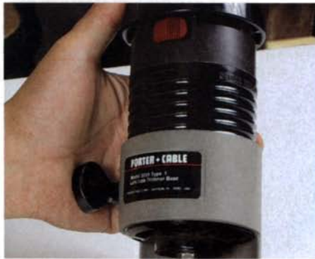
Right-handed bias in the design. The knob that secures the motor to the base makes the tool difficult to use for left-handers.
