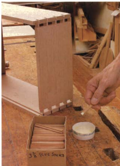
Glue sticks galore. Becksvoort keeps a supply of small sticks on hand. Dipped in glue, the sticks make it possible to get adhesive into all the crevices of the dovetail joints.
