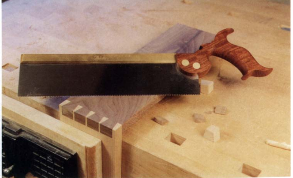
Smooth-cutting handsaw. Clean, smooth cuts were the norm with this small (12-in.) tenon saw from Adria Toolworks.
