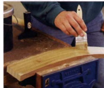
Scuff the surface and apply glue size. Rough up the substrate with coarse sandpaper. Then brush on a size, a watered-down coat of hide glue, and let it dry.
