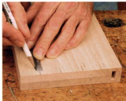
Mark the layout on the face of only one piece. Use a chisel to mark the cutouts where the pins will go, then use the same chisel to chop out the waste.
