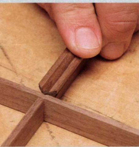
Eight miters for each intersection. Four muntin faces join together over each half-lap joint of the lattice grid.
