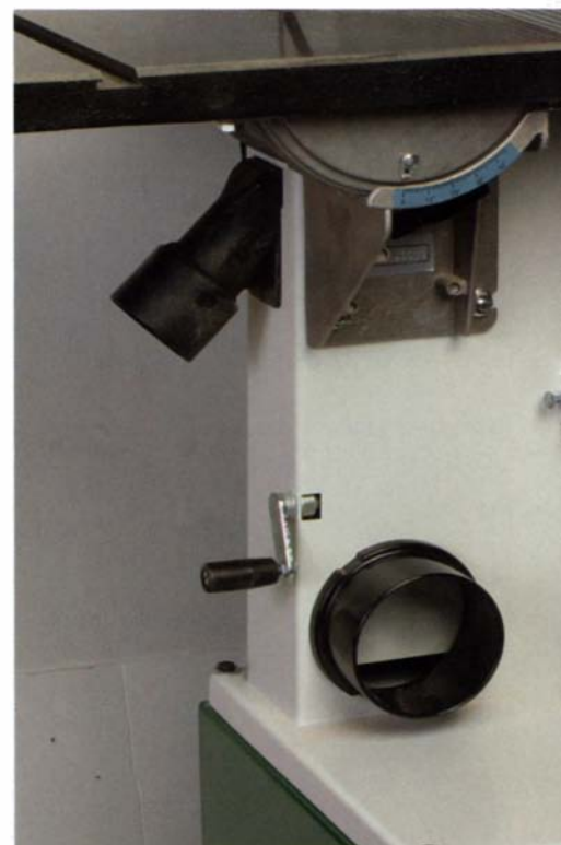
Rikon includes a pair of dust-collection ports. The top port accepts hoses from most shop vacuums. The bottom port works with larger dust-collection systems.
