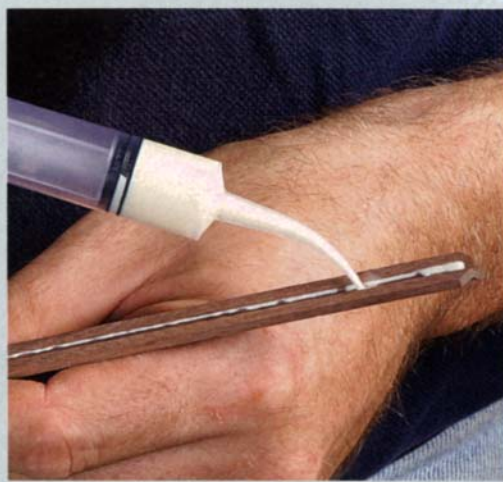
Don't use too much glue. A syringe is ideal for applying glue to the small muntin face pieces. (One source is Lee Valley, 800-871-8158.) Any excess glue should be removed before it dries.
