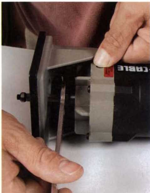
Securing the bit. To change bits on this Porter-Cable trimmer, you need only one wrench because you can lock the spindle by pushing a button on the side of the motor housing.
