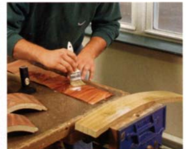
Now paint hide glue onto all surfaces. Apply full-strength glue to the substrate and the underside of the veneer.
