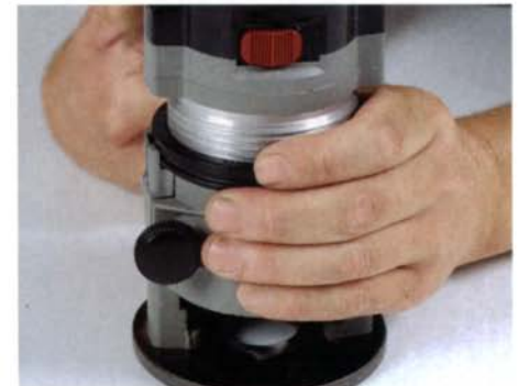
Precise vertical adjustments. The PC 310 trimmer has an adjustment ring that allows you to fine-tune the depth of cut.
