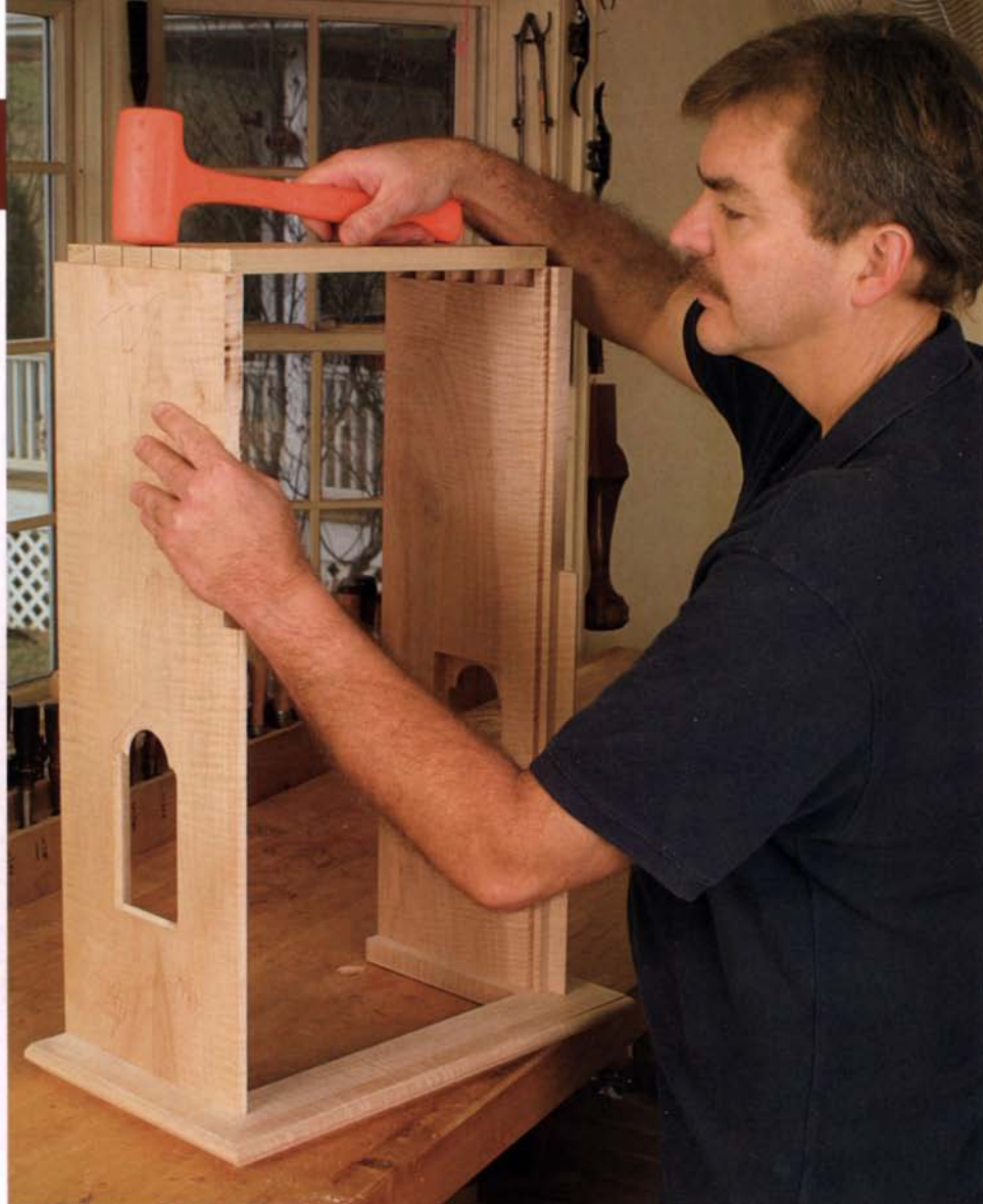
Dry-fit the hood parts before final assembly. The hood sides anchor to the base frame with two through-mortises per side. Cut the mortises before assembling the three-sided base frame, and test the fit of all the hood pieces before gluing them together.
