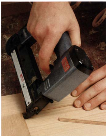
Headless nails are easy to hide. Senco's new pin nailer drives small headless pins, leaving holes that hardly can be seen.
