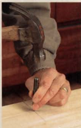
Before drilling, mark and center-punch. The dimple punched into the workpiece will guide the bit.
