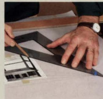
Push-pin pivot. Stick a push pin into each vanishing point and use it to pivot a straightedge to draw accurate vanishing lines.
