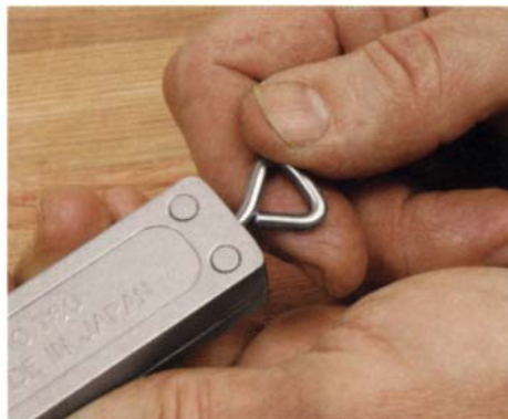
End screw. To allow the body to lie flat on both sides, Shinwa (shown) and Bridge City lock the blade from the end of the body.
