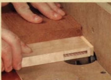
Rout dovetails on the front and back stretchers. Use the same bit that was used for the slots in the case. A horizontally mounted router allows the workpiece to remain flat on the router table.
