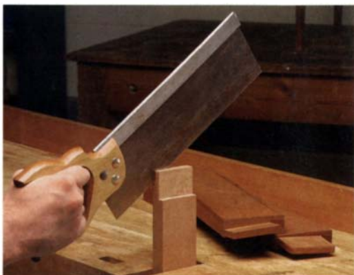
A rip saw cuts tenon cheeks. Cutting the cheeks (or faces) of a tenon is done most efficiently with a rip saw because they are cut with the grain.
