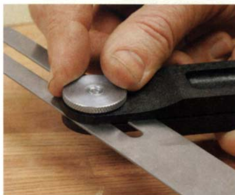
Knurled knob. On several sliding bevels (Craftsman is shown), the blade is locked by tightening a knurled knob.
