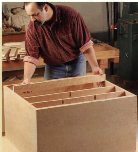
Installing the drawer frames. Begin by gluing the front stretchers in place (left). Then flip over the case and insert the runners into the front stretchers, applying glue only at the front tenons (right). Finally, glue the back stretchers into place.
