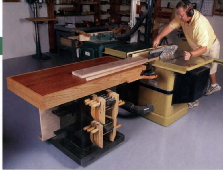
A multipurpose support table. This table can be wheeled to support operations at the tablesaw or the jointer, while the base stores clamps and jigs.
