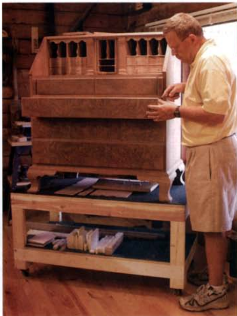
A secretary on the move. This rolling cart allows Lyons to move work around the shop easily. It also keeps a piece at a comfortable working height, with access to all sides.
