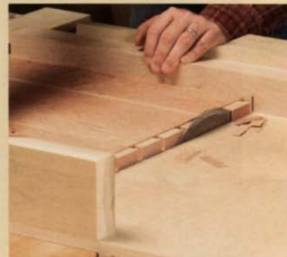
Finally, trim \frac{1}{8} in. from each end of the case bottom. Shorter tails are necessary for the half-blind dovetail joint at the bottom of the case.
