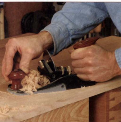
Scraping plane tames figured wood. When it comes to smoothing highly figured grain, the nearly square cutting angle on the Veritas takes light shavings with no tearout.
