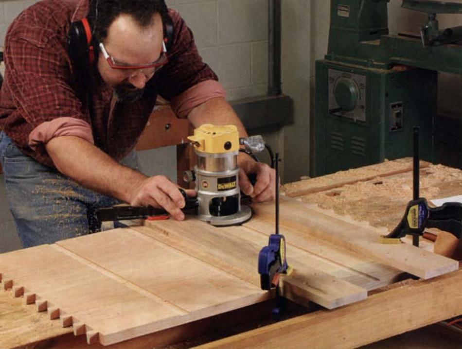
Router jig aligns carcass dados. The simple jig made from 3/4-in.-thick poplar is sized to fit your router's base. Align the jig with layout marks on the case side and clamp it securely. Use a 3/4-in. straight bit to rout the 1/8-in.-deep dados for the drawer runners.
