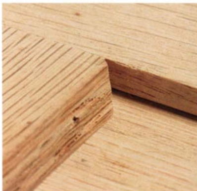
Headless nails are easy to hide. Senco's new pin nailer drives small headless pins, leaving holes that hardly can be seen.
