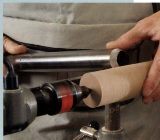
Vacuum while you turn. The Vacuum Gouge from CleanTurn Tools is both a turning gouge and vacuum port, so chips are sucked up right at the source.
