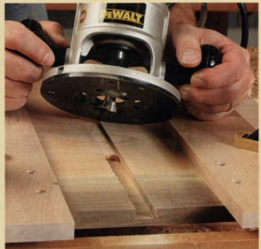
The same jig is used for dovetailed slots. After routing all of the dados, use a 3/4-in. dovetail bit to cut slots for the front and back drawer stretchers.
