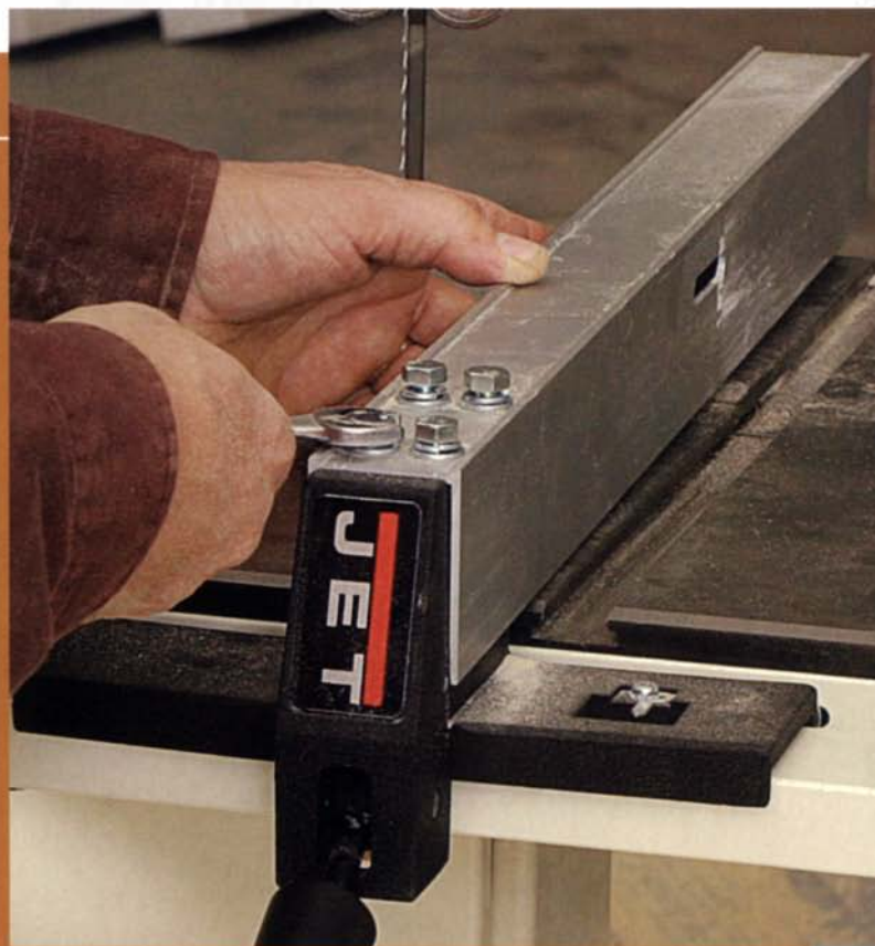
Dealing with drift. To adjust the Jet and Rikon rip fences for blade drift, you simply loosen four bolts.
