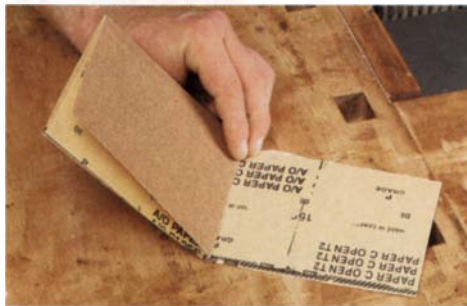
Then fold and tuck into the adjacent crease. Continue to fold and tuck in either a clockwise or counterclockwise direction.
