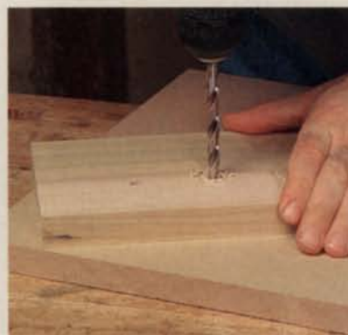
Position a sacrificial board underneath the workpiece. When wood fibers are supported, they don't tear as the bit exits the workpiece.
