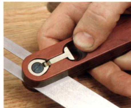
Cam lock. Veritas builds a cam lock into the body, a system that holds the blade securely.
