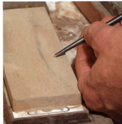
Refine the point. Use a benchstone, sandpaper, or other abrasive surface to smooth and sharpen the point.
