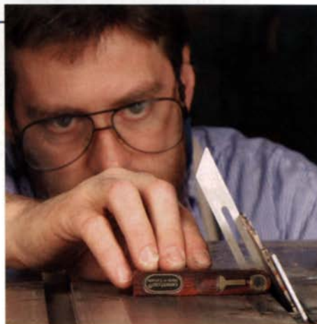
Set an angle on the table saw. With the tongue of a sliding bevel butted against a saw blade, it's easy to set the blade angle.
