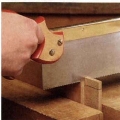
A crosscut saw is best for shoulders. A 14-tpi crosscut saw produces a clean, accurate cut across the grain.
