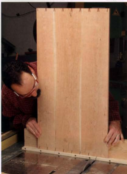
The table saw saves time. The tails on the top and bottom panels are cut using a table saw blade with the teeth ground to the angle of the dovetail.
