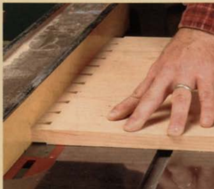
Rabbet helps align the dovetails during marking and assembly. The \frac{1}{8} -in.-deep rabbet extends to the baseline of the tails.
