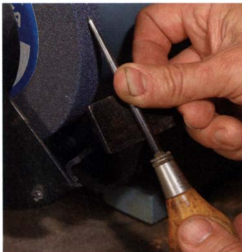
Keep the tool moving. For a balanced grind, roll the tool under your thumb as you hold it against the wheel.
