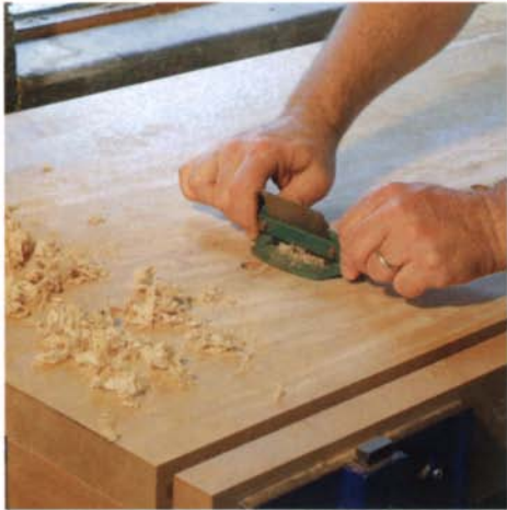
Scrape first. On a used bench, scrape away any dried glue before applying a new coat of the wipe-on finish.
