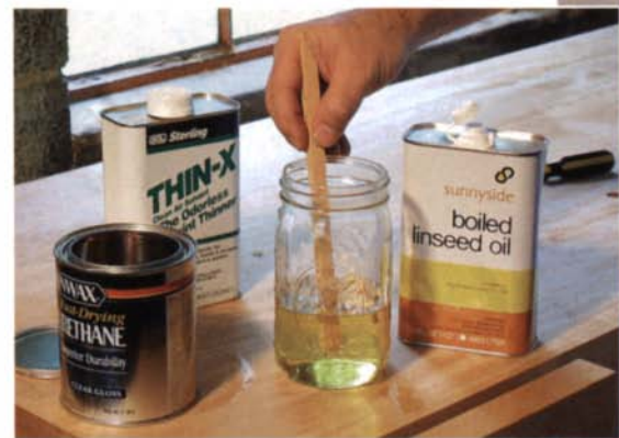
Mix the finish. Minick's mixture of oil, varnish, and paint thinner contains a higher proportion of resin than most Danish oils to give the bench greater protection.
