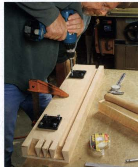
Attach the large vise nuts to the back of the end cap. Also, finish cutting and fitting the dovetails.
