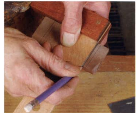
Fit the blade to its holder. After marking the width of the blade on the blade holder, draw another pair of lines ⅛ in. inside to outline the throat opening.
