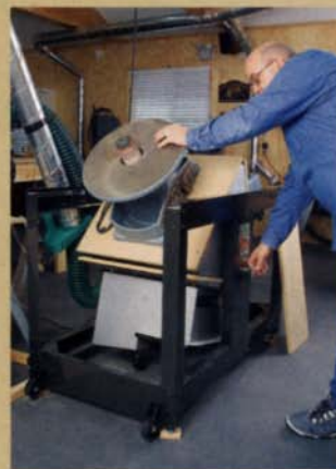
Space-saving stand. A Sears/Craftsman revolving workstation holds three benchtop machines: a spindle sander, a benchtop planer, and a pocket-hole cutter.
