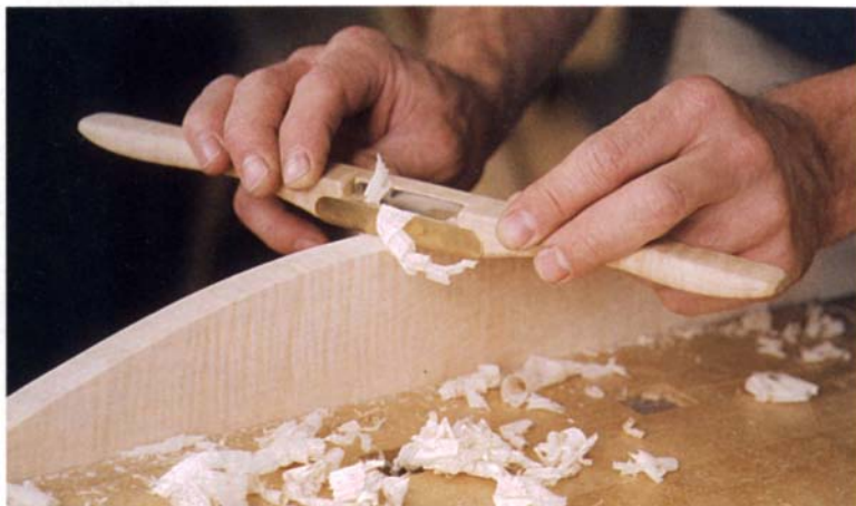
Smooth surfaces on curved work. The new standard scraper from Woodjoy will appeal to those who demand a blemish-free finish on sculpted or contoured work.
