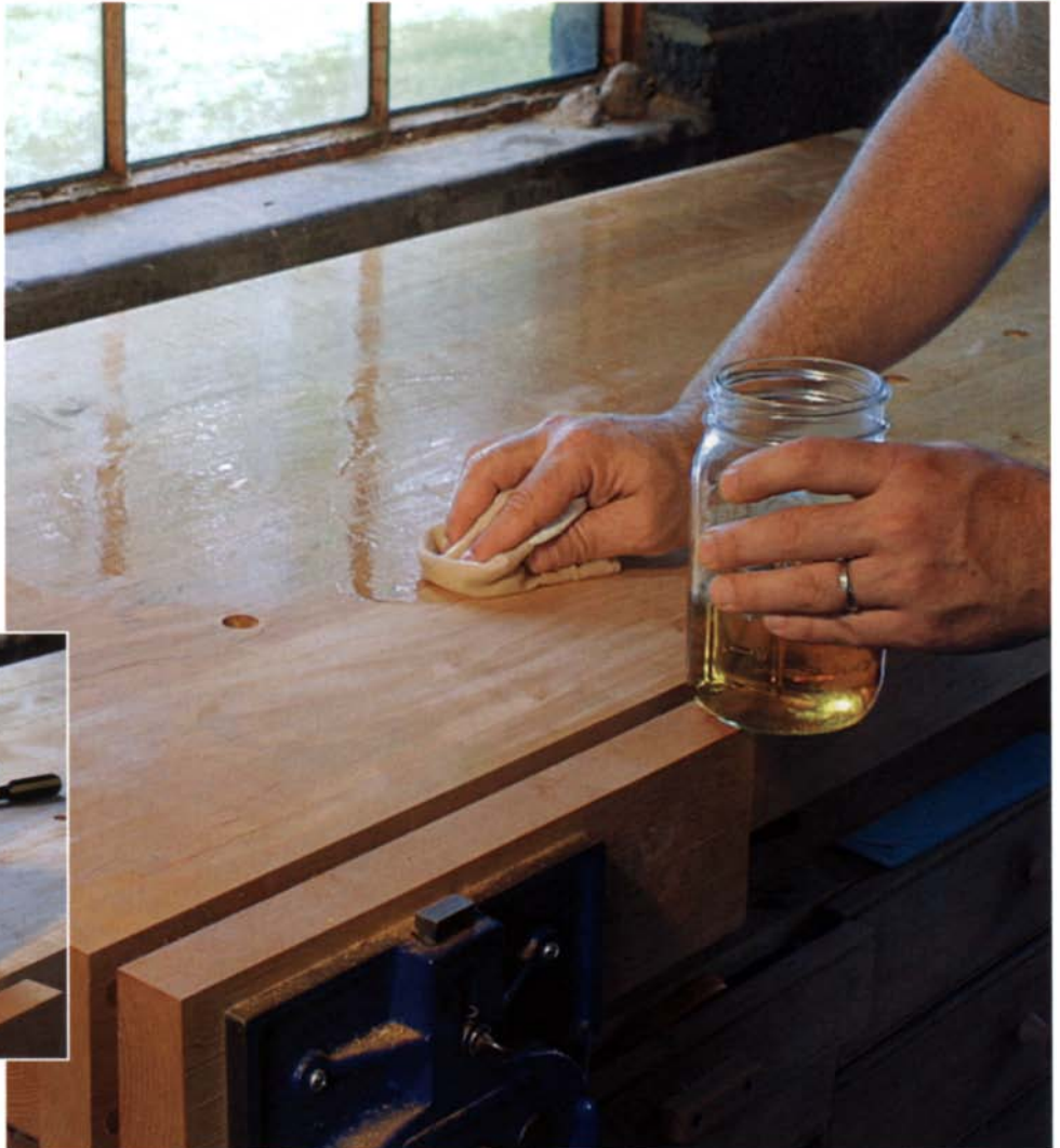
Lay it on heavy. Apply the oil-varnish mixture liberally and allow it to soak in for 10 minutes before wiping off the surplus with a clean cloth.
