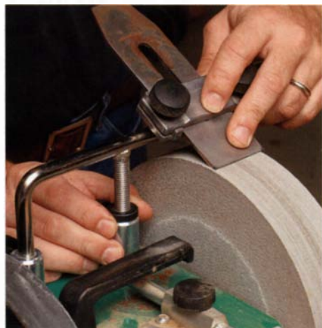
Micromanagement. Setting the height of the support rod on the Tormek is easier thanks to a new micro-adjust feature.
