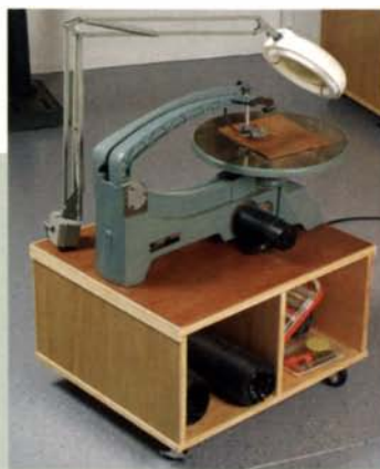
Scrollsaw sits at a comfortable height. The scrollsaw is mounted to this low rolling cabinet so that it can fit below the workbench when not in use. However, it's just the right height to use while sitting comfortably in a chair.
