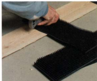
A rubber doormat sliced into small pads and placed under the feet of a machine can significantly reduce the vibration transferred from the shop floor to the framing in the rest of the house.
