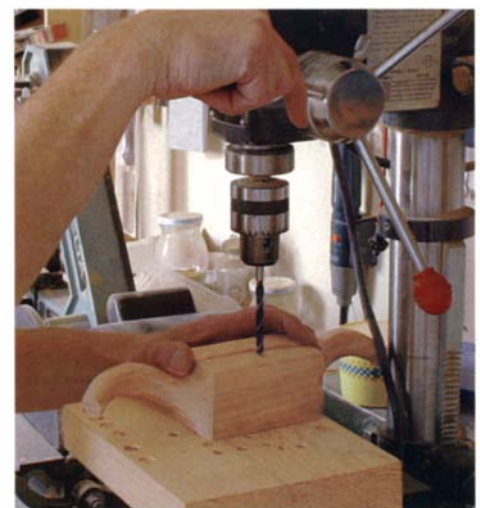
Drill the hole. With the 85° bevel side of the scraper body facing down, use a drill press to make the hole for the thumbscrew.
