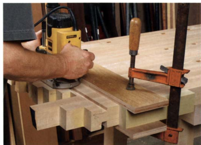
Use the simple two-fence jig shown. Rout deep slots in both sides of the slab, then use a jigsaw to cut off the waste, leaving square shoulders and a tongue that will fit into the end caps.
