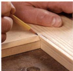
The upper face-frame stiles require a stopped chamfer. Dry-fit the frame and mark the end of the chamfer (left), then plane the chamfer to within an inch or two of the stop mark. A drawknife will give you a smooth edge (center) as you cut away the remainder of the chamfer. Dry-fit again and finish the corner with a chisel (right).
