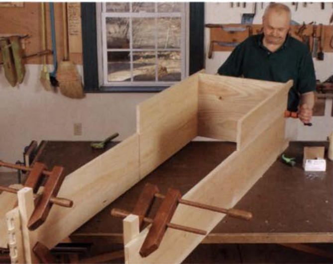
Assemble the carcass. The first step is to glue and clamp the case bottom to the cupboard sides.
