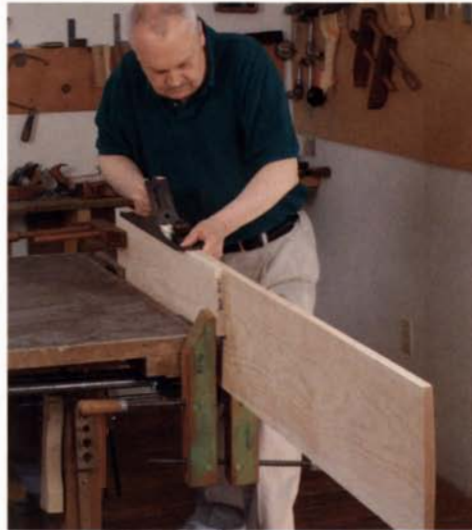
Joint the edges. By clamping the face of the short board to the face of the case where they meet, both boards may be planed simultaneously, ensuring that they will meet up perfectly.
