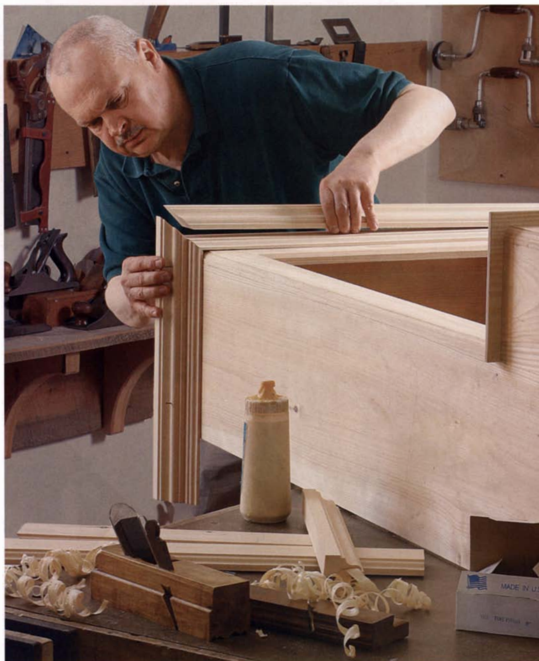
Secure the lower stiles to the case. Use 4d headless cut brads through the molding into the sides and 6d cut nails into the bottom.
