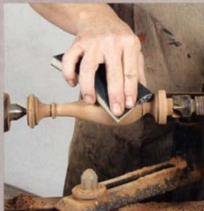
Sanding sponges protect fingers from friction heat. They're also flexible, which allows them to enter coves without dulling crisp shoulders.
