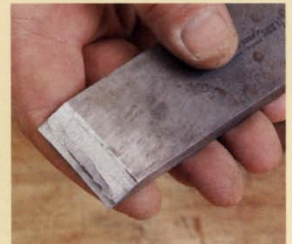
Getting there. With rust and dried glue ground away, this bevel is ready for abrading on the stone.
