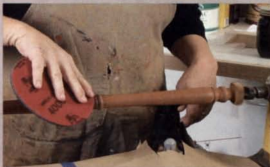
Grain filler can be colored. Use a cloth to apply the filler to the spinning wood (above), forcing it into the grain and removing any surplus. Smooth the surfaces with a 4,000-grit Abralon pad (left) before moving to the next finishing step.
