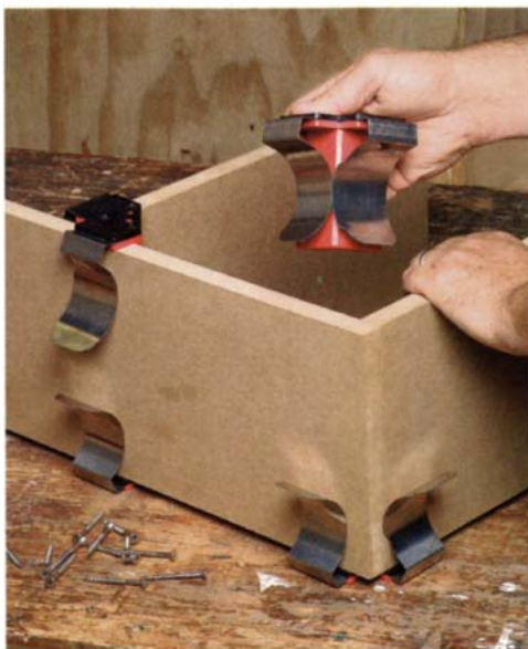
Clever clamps lend a hand. Slip one of these clamps onto a pair of butted boards, and the boards stay put until you're ready to add a clamp or drive a screw.
