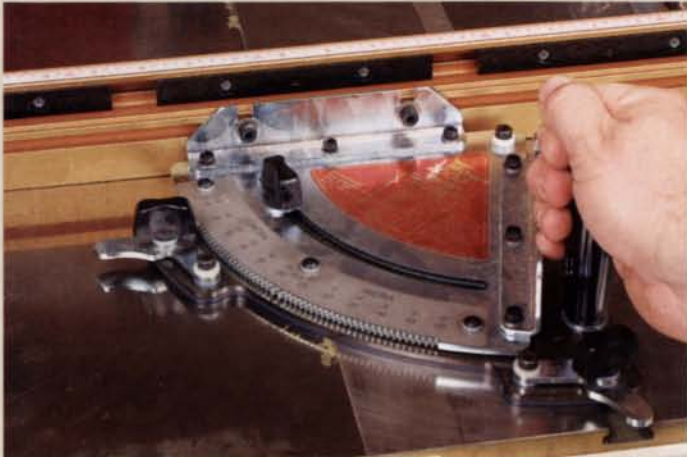
The Incra 2000 can go out of square. If the large black handle loosens with time and use, the fence-support plate will shift slightly left or right.
