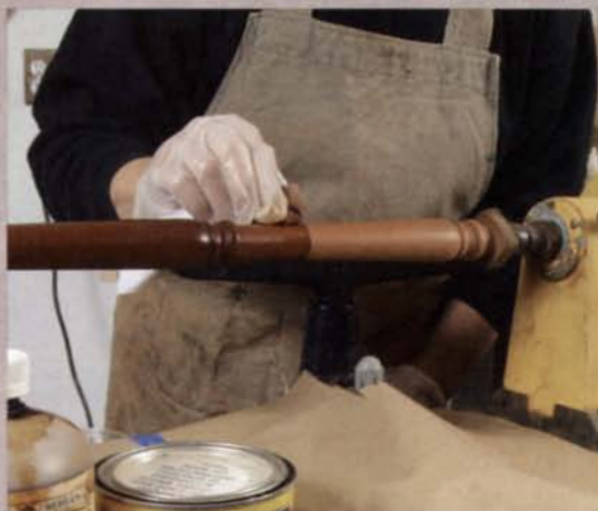
A moving stain. An alcohol-based dye or a pigmented oil stain is applied to the spinning workpiece in thin coats with a clean cloth.
