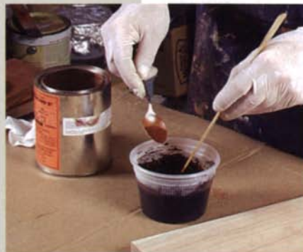
Prepare the dye. Stir 1 tsp. of dye powder into 8 oz. of warm distilled water to create a dye that is double the normal strength.
