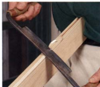
The upper face-frame stiles require a stopped chamfer. Dry-fit the frame and mark the end of the chamfer (left), then plane the chamfer to within an inch or two of the stop mark. A drawknife will give you a smooth edge (center) as you cut away the remainder of the chamfer. Dry-fit again and finish the corner with a chisel (right).
