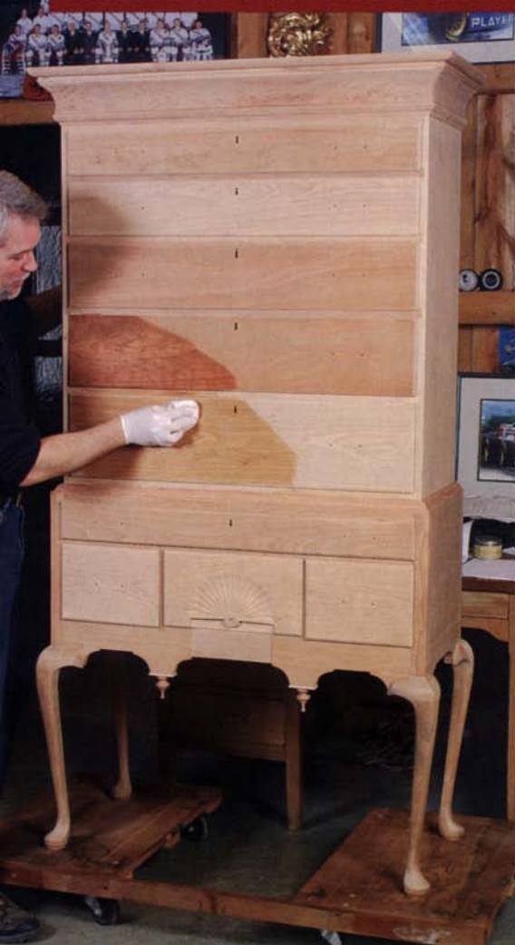
Prepare the dye. Stir 1 tsp. of dye powder into 8 oz. of warm distilled water to create a dye that is double the normal strength.
