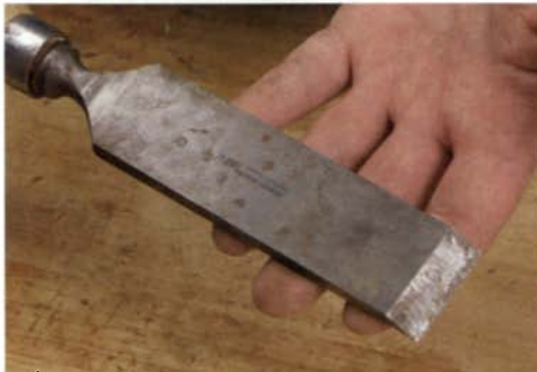
Before. This mortise chisel, covered with glue globs and rust and as dull as a butter knife, has seen better days.
