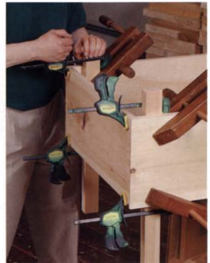
Clamping the top to the sides. Clamp blocks, positioned with wooden hand screws, provide gripping surfaces for the clamps to pull the dovetail joint tight.
