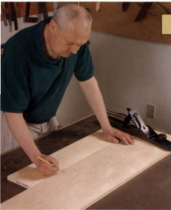
Form the step-back profile. The base is built up by adding a short board to each case side.
