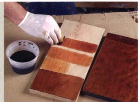
Adjust the tone. On a sample board, the first swatch was too dark, the second too light, and the third had the right depth but was too orange. Some black was added to adjust the tone.
