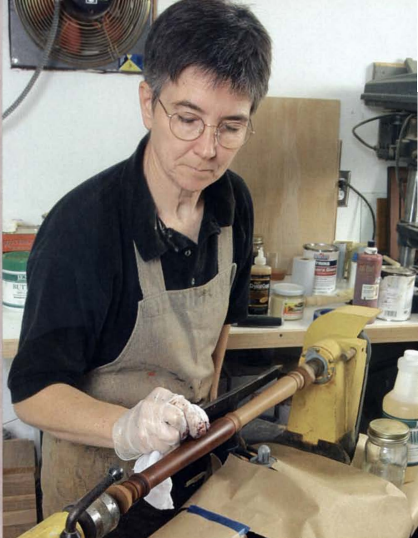
Grain filler can be colored. Use a cloth to apply the filler to the spinning wood (above), forcing it into the grain and removing any surplus. Smooth the surfaces with a 4,000-grit Abralon pad (left) before moving to the next finishing step.
