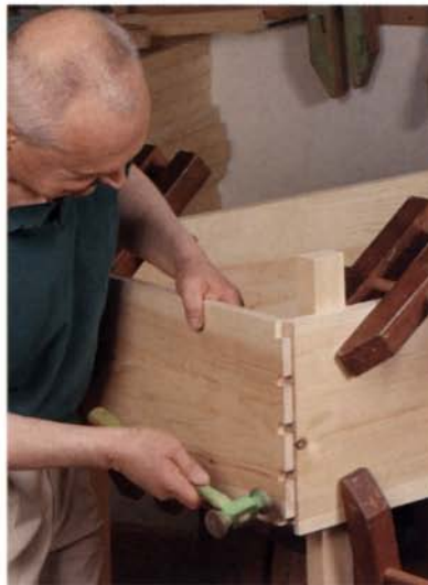
Join the dovetails with gentle force. With the bottom securely in place, apply glue to the dovetails and tap the top board into place.
