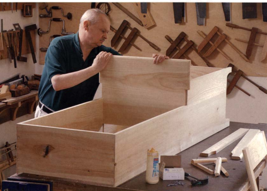
Slide the work surface into the dadoes. The cupboard work surface should fit tightly in the dadoes cut into the cupboard sides. It is secured in place with glue and nails. The dadoes are hidden by the front of the work surface.
