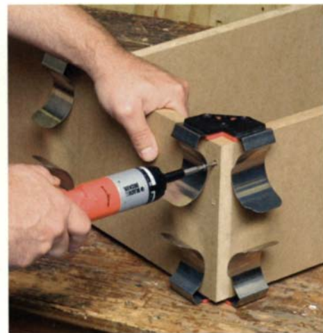
Clever clamps lend a hand. Slip one of these clamps onto a pair of butted boards, and the boards stay put until you're ready to add a clamp or drive a screw.
