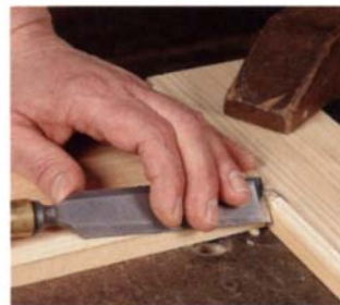
The upper face-frame stiles require a stopped chamfer. Dry-fit the frame and mark the end of the chamfer (left), then plane the chamfer to within an inch or two of the stop mark. A drawknife will give you a smooth edge (center) as you cut away the remainder of the chamfer. Dry-fit again and finish the corner with a chisel (right).
