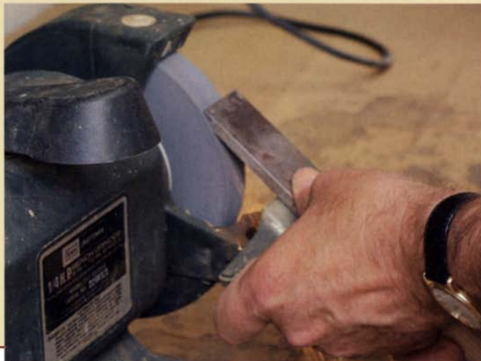
Getting there. With rust and dried glue ground away, this bevel is ready for abrading on the stone.
