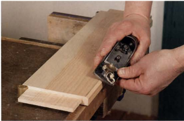
The upper face frame gets a chamfer on its inside edge. Scribe the width with a marking gauge and use a block plane to bevel the inside edge of the top rail.
