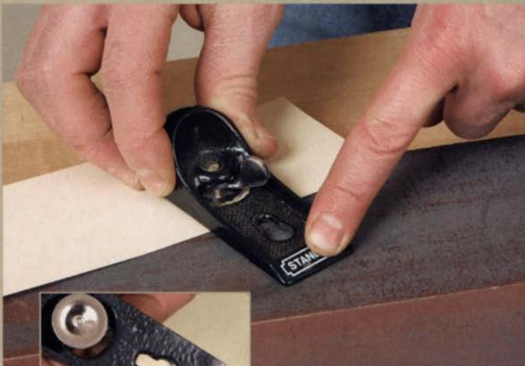
Tune the lever cap. While protecting the back of the cap assembly with a piece of paper, sand the paint off the front edge for a snug fit with the blade.
