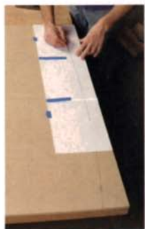
Transfer half of the curve to paper and make a half template. Using a half pattern will ensure symmetry. Cut out the template on the bandsaw. Then sand with a flexible batten to maintain a fair curve.
