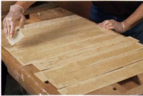
Spread the glue. Use a notched piece of credit-card size plastic or wood.
