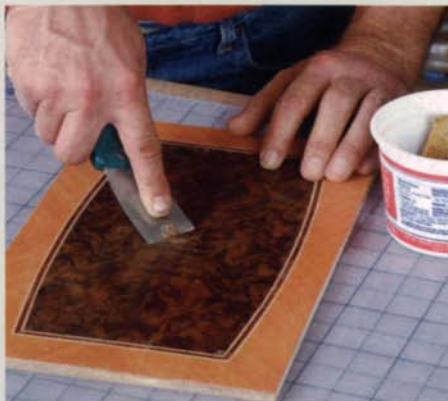
Wet the surface to scrape away the last bits of tape. The moisture also serves to reveal any air pockets beneath that must be repaired.
