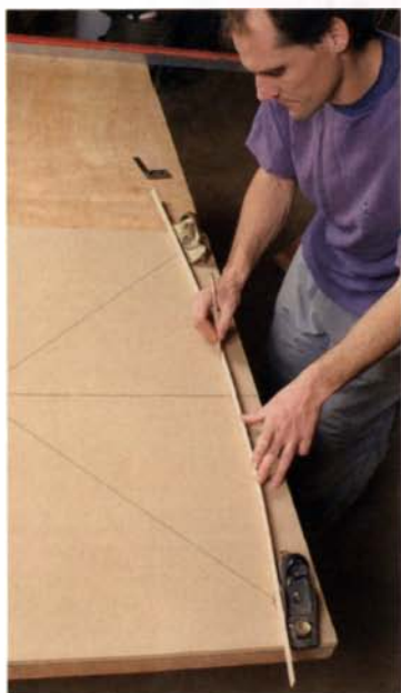
Start by finding a pleasing curve. Mark diagonals to locate the corners and use a batten to trace the desired curve.
