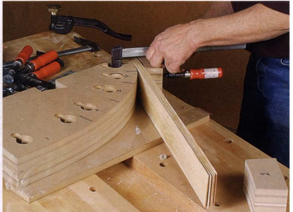
Add the first clamp. After placing the stack of plies in the form, install the first clamp while making sure all edges of the plies stay reasonably flush.
