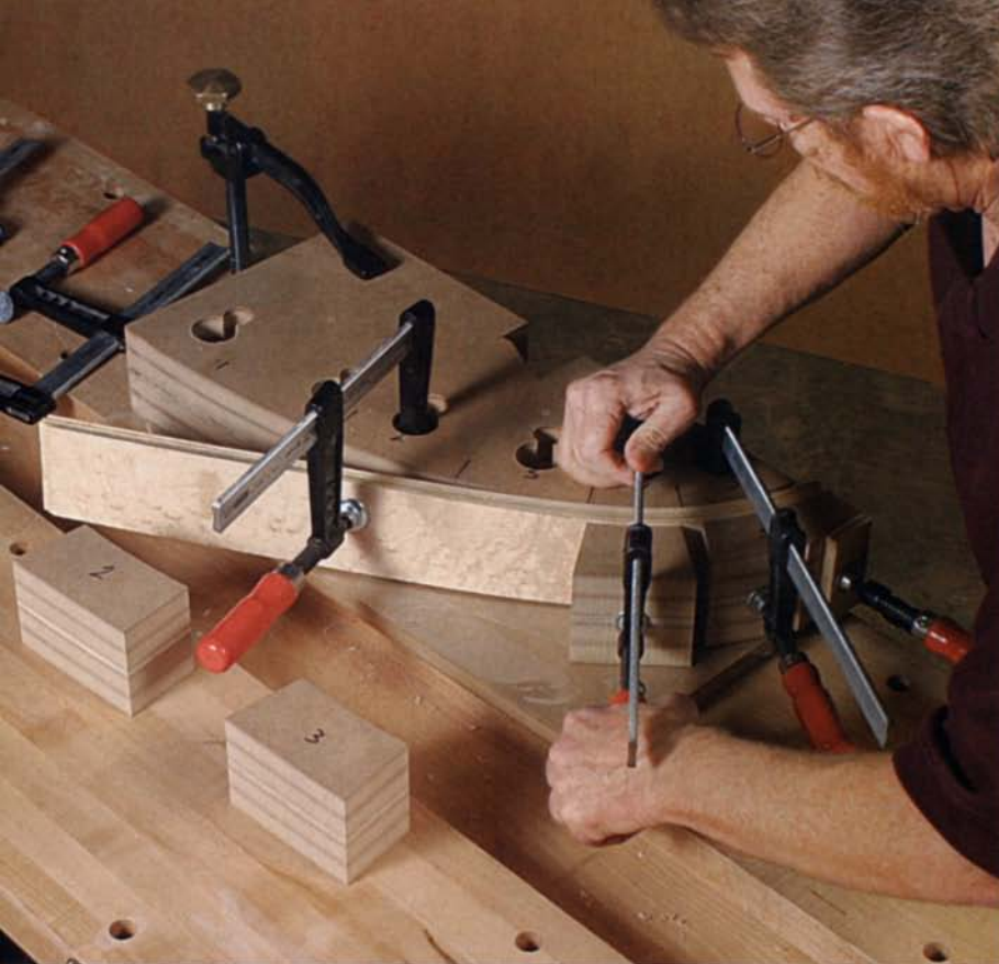
Once the first clamp is on, add the remaining clamps in sequence. Schleining always leads with a loosely tightened temporary clamp to get the bend started.
