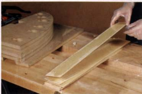
Stack the plies. With the glue applied, the plies are stacked with all of the edges flush.
