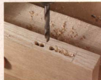
Do not overlap the holes. The drill bit needs the surrounding wood as support so that it can bore straight.
