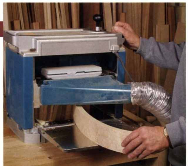
The other edge is smoothed by the thickness planer. After the first edge has been handplaned reasonably smooth and flat, the opposite edge is planed using a thickness planer.
