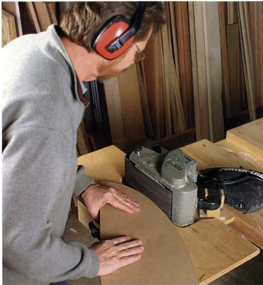
Smooth the curve. With a belt sander on its side and secured in place, Schleining smooths the curve of the core of the form.
