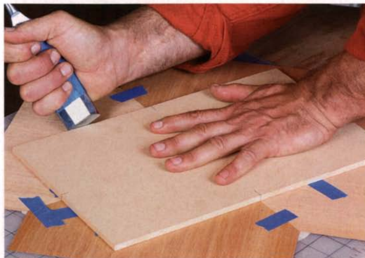
Lay down the substrate and trim around it. Use center marks to align the MDF substrate with the pattern's center seams.
