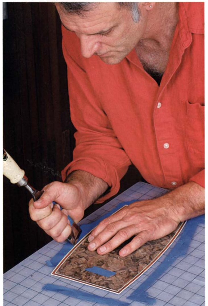
Trim away the overhanging tape. The chisel technique makes it possible to cut right to the banding without damaging it.
