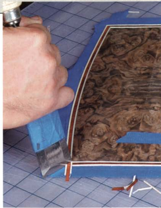
A perfect miter. Overlap the ends and make a parcelling (chopping) cut. Then align the chisel blade with the two corners and press straight down.
