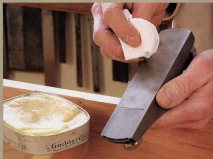
Wax the sole. This protects the plane from rust and makes for smooth sliding action.
