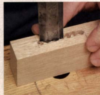
Clean up with a chisel. Pare the walls of the mortise smooth.
