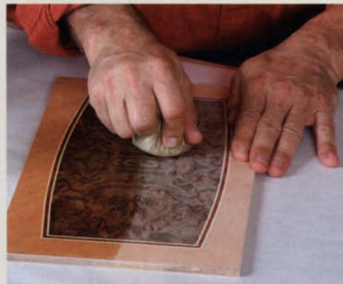
Wipe on a thin coat of shellac before filling and finishing. Schürch uses colored, acetone-based wood filler to fill the small voids in the burl or elsewhere. The acetone won't dissolve the shellac, which protects the workpiece.
