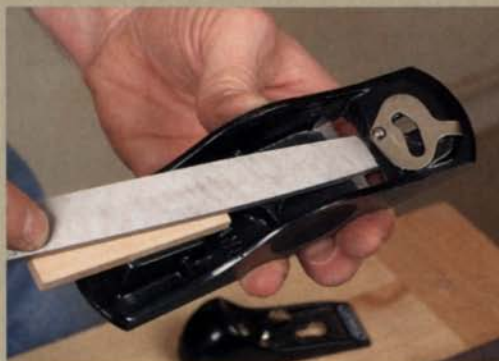
Tune the lever cap. While protecting the back of the cap assembly with a piece of paper, sand the paint off the front edge for a snug fit with the blade.
