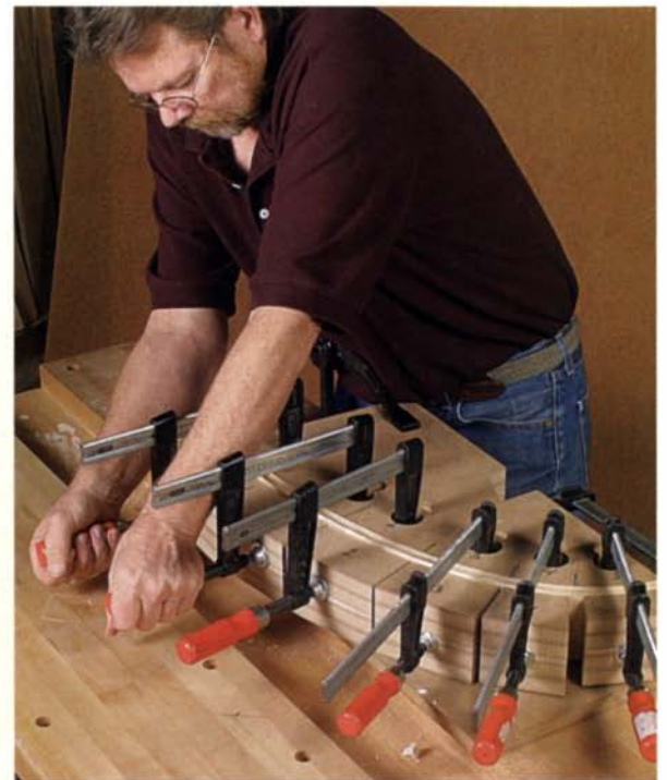
Tighten the clamps. After adding the final clamp, give them all a final check for tightness.
