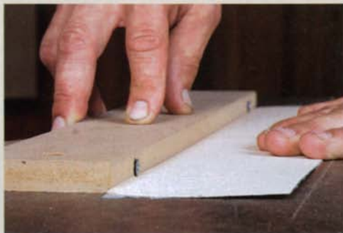
Slide the veneer against the simple jig. The thickness of the stringing will be determined by how much the screw heads protrude from the edge of the jig. Again, place gum tape on the back of the veneer to prevent splintering.
