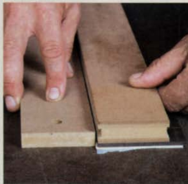
Set a thick straightedge onto the veneer against the screw heads. Sandpaper under the straightedge keeps the veneer in place.
