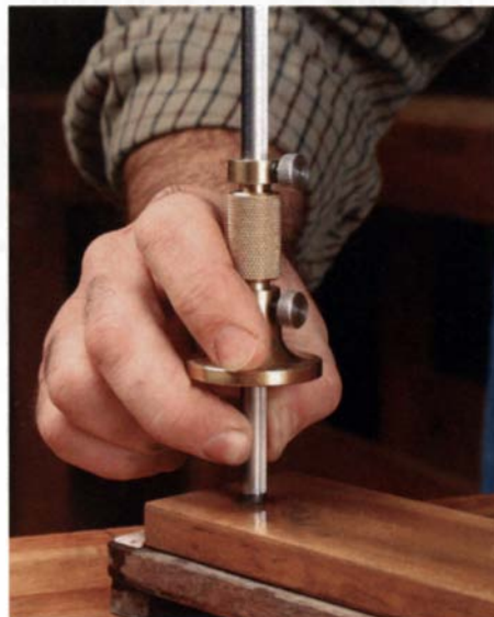
Wheel sharpener. With the beam on end, the cutter on a Tite-Mark gauge is sharpened easily on a fine-grit stone.
