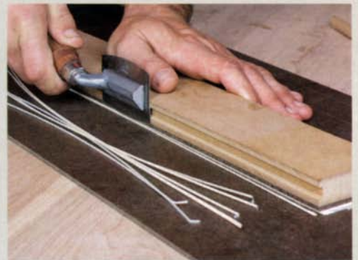
Cut away each strip with a sharp veneer saw. Pulling the saw straight back, make a light pass to start, then make firm passes until the strip is severed cleanly.
