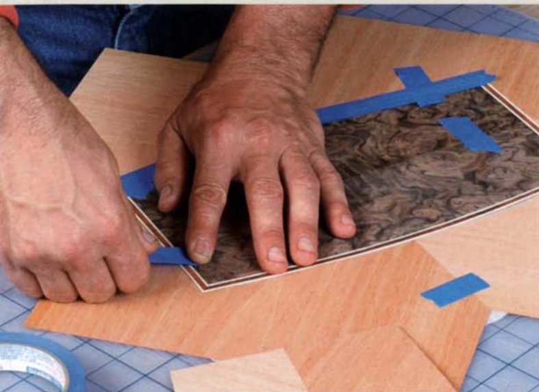
Lay the center section into the border and tape it. Again, use blue tape first on the glue face, then gum tape on the show face.
