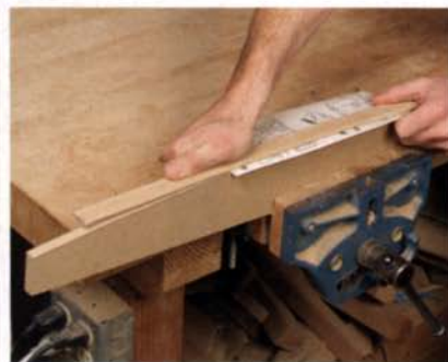
Transfer half of the curve to paper and make a half template. Using a half pattern will ensure symmetry. Cut out the template on the bandsaw. Then sand with a flexible batten to maintain a fair curve.
