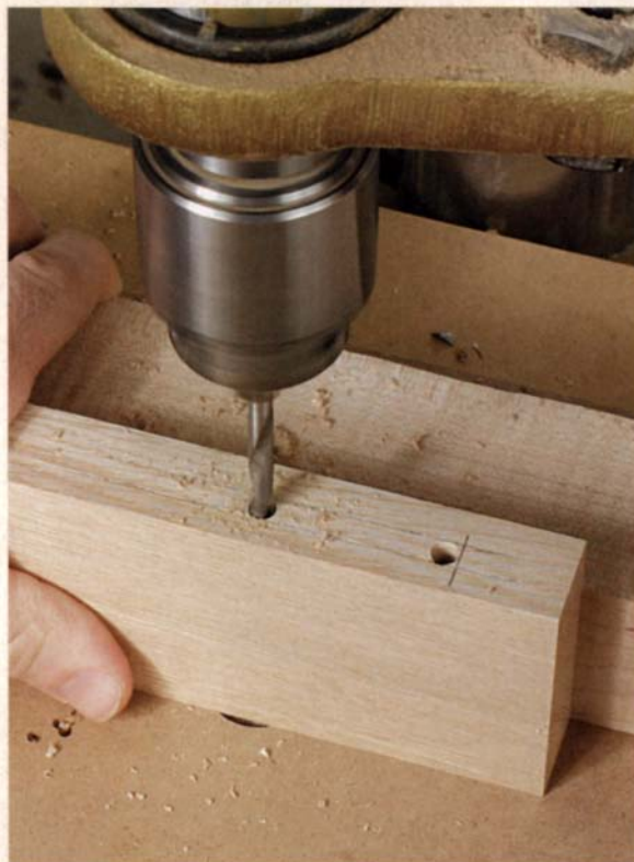
Drill the ends of the mortise first to give the tip of the bit solid footing. Square ends are critical to a strong joint, so it's important to eliminate bit deflection at the ends.
