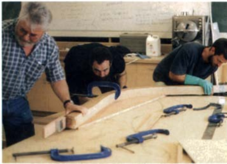
Master class. David Livermore (left) teaches steam-bending to Ross Annels (center) and James Curtis.
