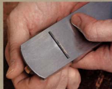
Adjust the throat. A small gap in front of the blade supports the finest cuts; a larger gap is required for heavier cuts.
