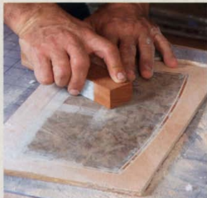
After the glue sets, sand away most of the gum tape. Use a sanding block and stay away from the edges to avoid sanding through them.
