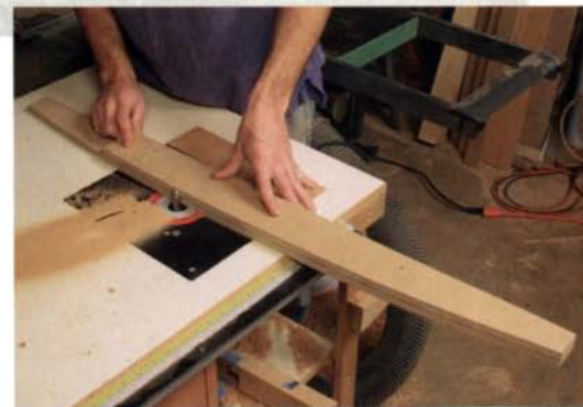
Use the half template to rout a full-length master template. Use a flush-trimming bit. This master will be the reference for both the panel and the edge-band templates.
