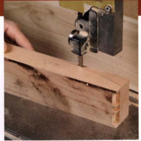
Cut the front curve on the bandsaw. Cut right to the line, then smooth the curve with a block plane and sandpaper.
