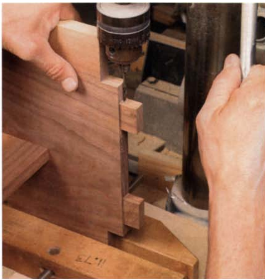
Drill a hole to prevent the tenon from splitting. Clamp the workpiece vertically in a handscrew. Then drill a hole through the width of the tenon.
