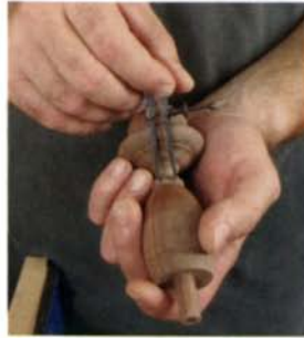
Divide to conquer. Mark out six points at the flame base with a pair of dividers.
