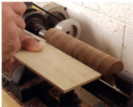
Dimension the turning. First turn the blank to the largest diameter. Then use a story stick to mark out the dimensions.
