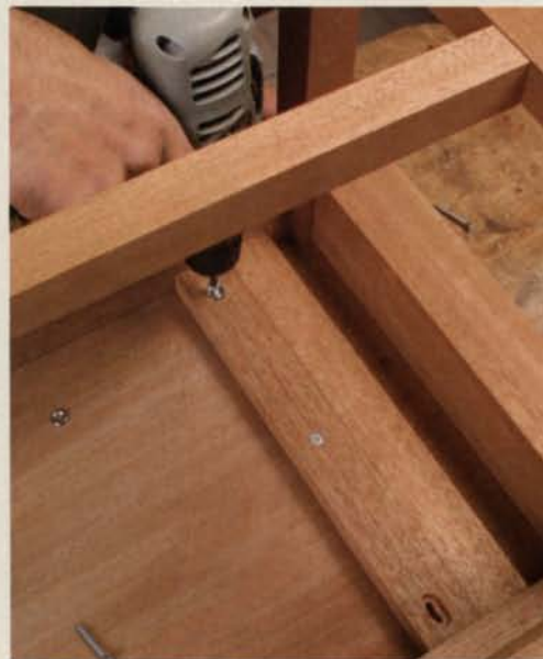
Meeting on the bevel. Slide the second cleat against the first one and screw it to the tabletop. The center screw can be fixed, but screws closer to the edges should be in slotted holes to allow for wood movement.
