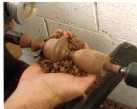
Smooth things out. Burnishing the completed turning with chips closes the grain and gives it a nice, natural polish.
