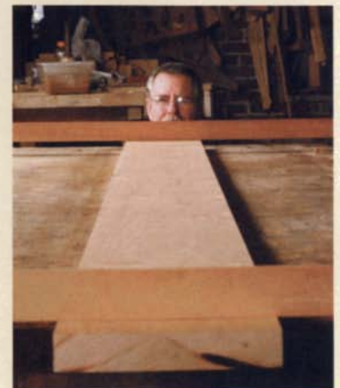
Twist detective. Winding sticks laid across each end of a board magnify any twist in the board.
