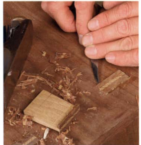
A trick for a clean, flush joint. To prevent tearout when planing a tenon flush, score a line around the base of the tenon.
