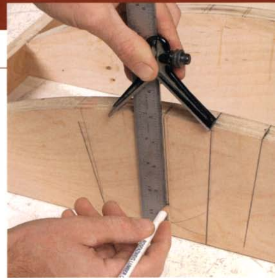
Figure out sections and angles right on the form. Use a center divider to draw lines straight down from each division.
