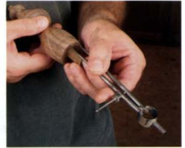
Locate the flame tips. Step off and mark nine equal spaces with dividers at the top.
