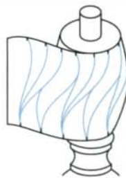
Divide to conquer. Mark out six points at the flame base with a pair of dividers.
