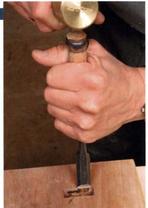
Lay out the offset of the angled mortise. After determining the offset at the top of the mortise, scribe lines to indicate where the angled cuts begin (above). Work steadily back toward the scribe line (right) and down toward the bottom edge of the mortise.
