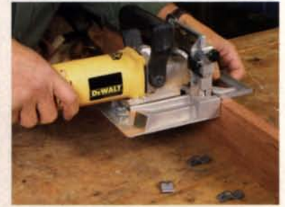
Grooves or slots. The clips are installed in grooves cut on the tablesaw or in slots cut with a biscuit joiner.
