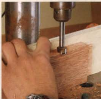
Precision drilling. The recess for twin-circle, or figure-eight, clips, should be close to the inside edge of the rail to allow for movement.
