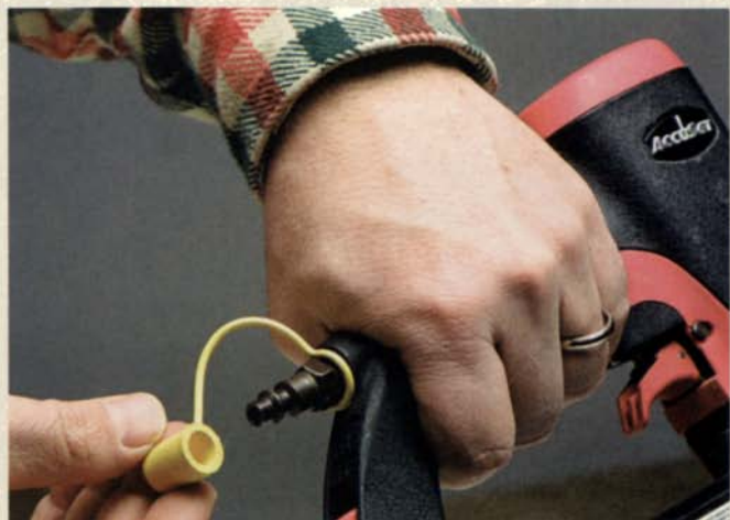
Cap keeps out crud. The Intacap helps prevent contaminants from getting into the intake connector of a pneumatic tool.
