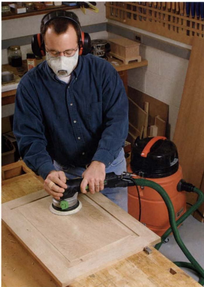
Cancer-fighting tools. Sanders create the very fine dust particles that penetrate deepest into the lungs. But the use of shop vacuums and dust masks can reduce breathable particulates to negligible levels, a government report says.
