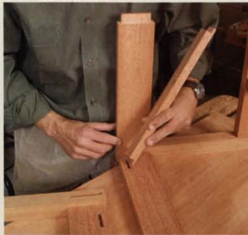
Tenons slide in to the grooves. One cleat sits in grooves in the side rails. The wide side of the board should be against the tabletop.
