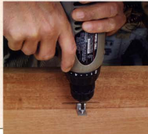
Grooves or slots. The clips are installed in grooves cut on the tablesaw or in slots cut with a biscuit joiner.
