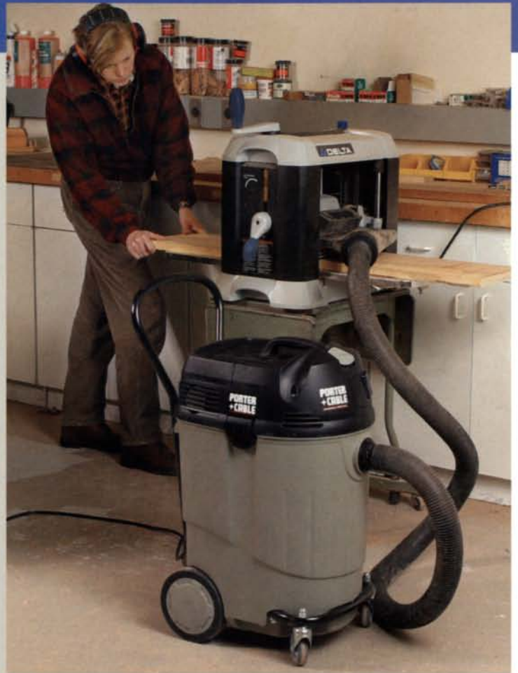
The shop vacuum also serves as a portable dust collector. Depending on the shop, it may be the only means of dust collection or it may be a backup to a larger system.
