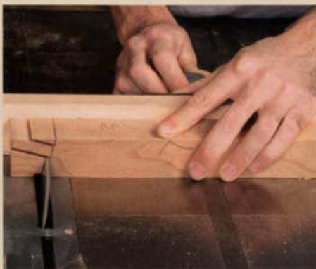
Cut the tenons on the rails while the stock is square. Make the cheek cuts first (left), then make the shoulder cuts (above).
