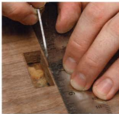
Lay out the offset of the angled mortise. After determining the offset at the top of the mortise, scribe lines to indicate where the angled cuts begin (above). Work steadily back toward the scribe line (right) and down toward the bottom edge of the mortise.
