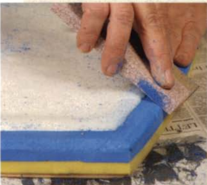
First, ease the edges of the dense outer band. This material is easily machined, sliced and sanded.
