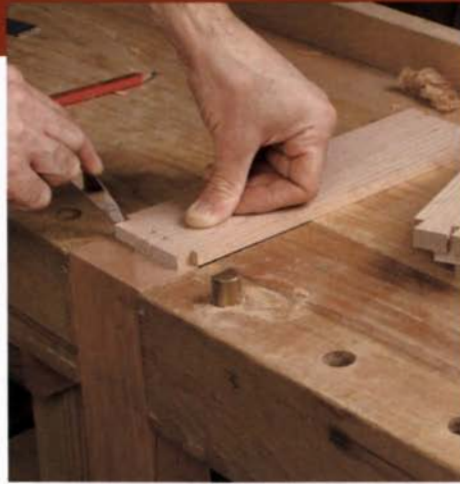
Cut all of the tails, then transfer the layout to the drawer front. Clamp the drawer front flush with the benchtop.
