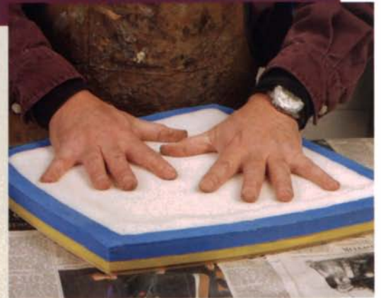
Last, press down the center section. Working from the edges toward the center, compress the softer, oversize center section as evenly as possible.
