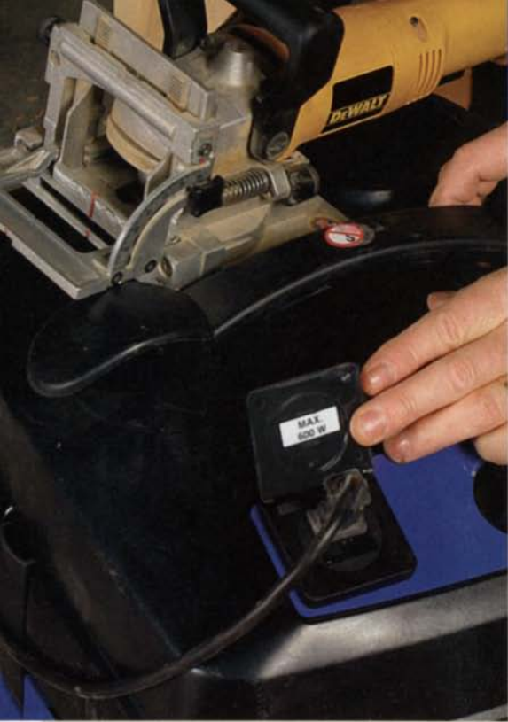
Plug into auto start. A receptacle right on the vacuum will turn the machine on and off in concert with the tool.
