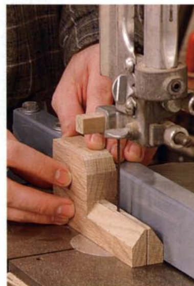
Narrow bandsaw kerf is just right. Split the body of the scratch stock down the middle but stop the cut 1 in. shy of the end. The cutters are pinched in the kerf and held in place with two machine screws and nuts.
