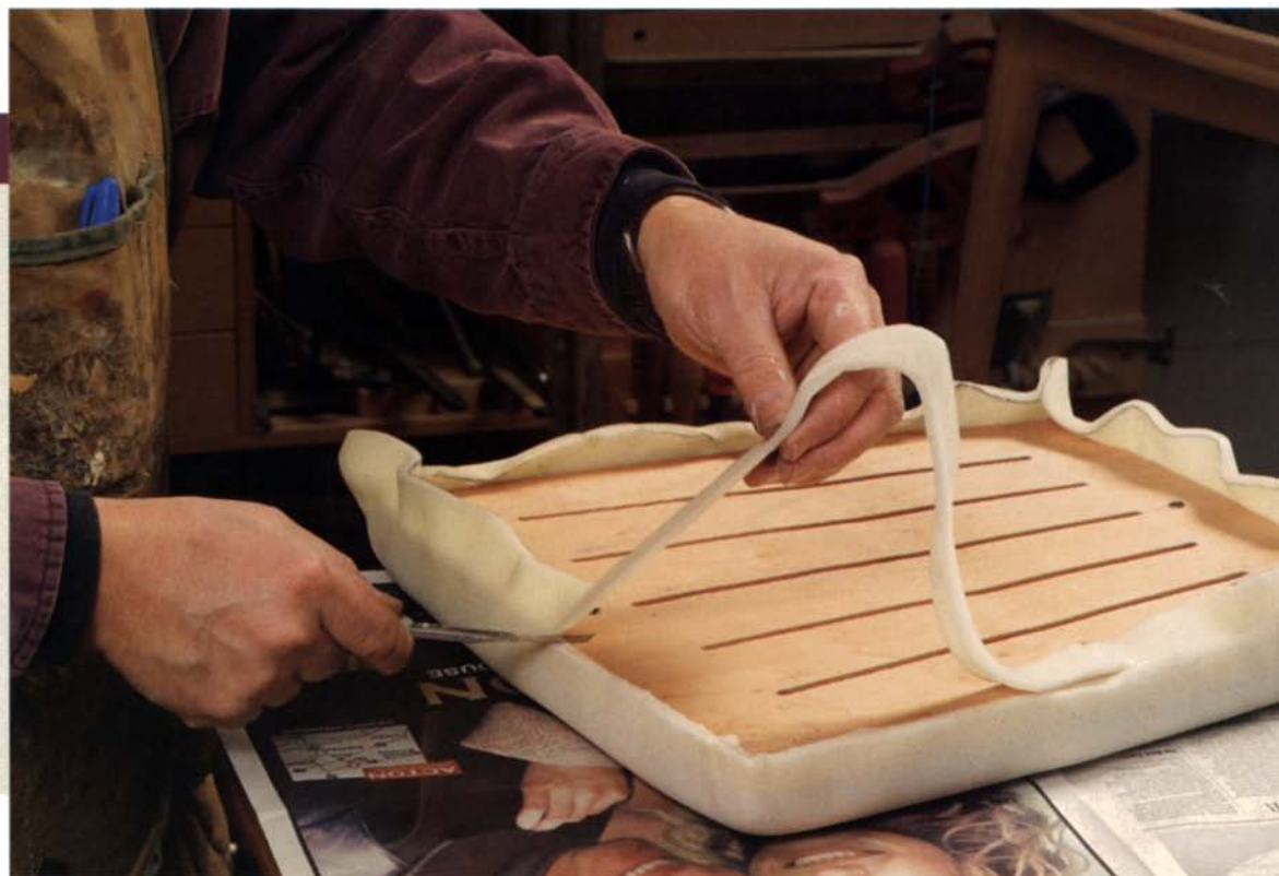
A final layer of foam smooths the bumps. Lay the seat platform upside down on ¼-in.-thick low-density urethane foam. Apply glue only along the sides of the platform and the exposed foam. Then pull up the foam evenly against the sides, being careful to avoid bumps and gathers.
