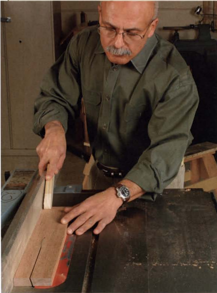
One cut makes two cleats. Select a piece of wood 3 in. wide and a little longer than the end rails of the table. With the blade at a 15° angle, rip the board in half.
