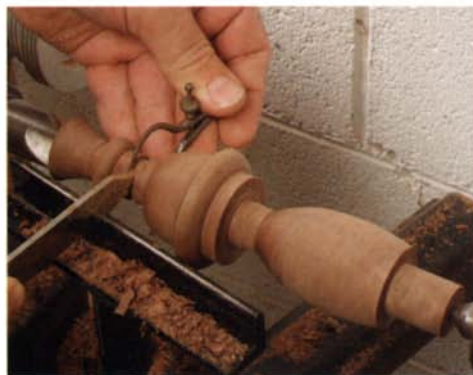
Form the flame and urn. Complete the turning of the finial, leaving a tenon at each end. The tenons will be used later to secure the work during carving.
