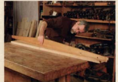
No bow here. To test whether a board is bowed, use a straightedge that is longer than the board.
