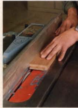
Grooves or slots. The clips are installed in grooves cut on the tablesaw or in slots cut with a biscuit joiner.
