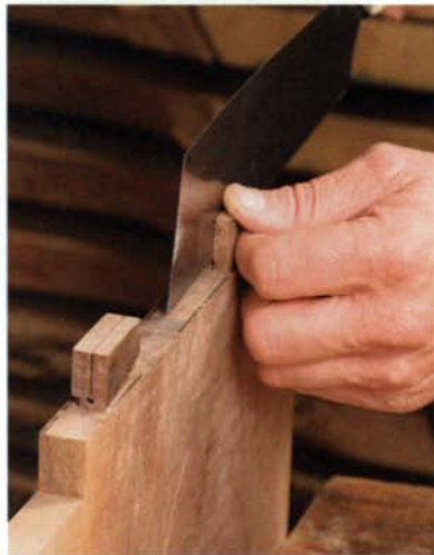
Saw a kerf down to the hole. A hand-saw leaves an appropriately narrow kerf in the tenon.
