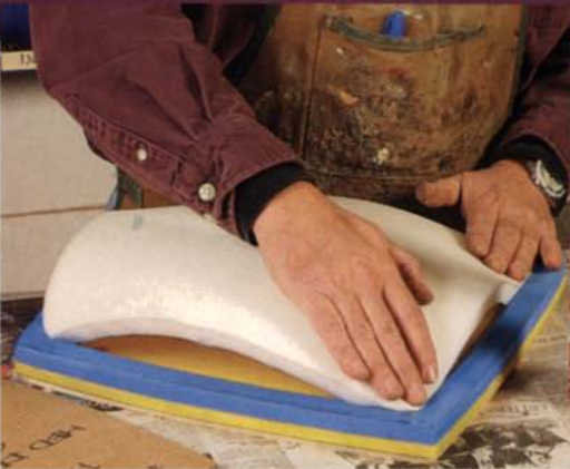
Start at the corners. Using spray adhesive on all of the mating surfaces, attach the corners of the center section of medium-density foam to the corners of the high-density outer band.
