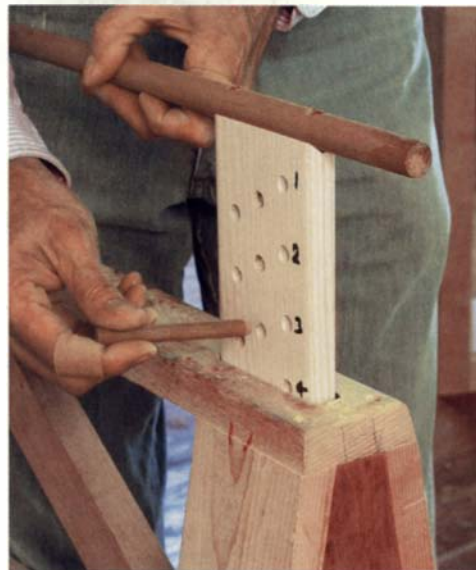
Ad adjustable-height sawhorses are versatile. Avoid back fatigue by raising the work up to a comfortable height.
