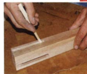
You don't need a lot of glue. With snugly fitting mortise-and-tenon joints, a thin layer of yellow glue spread evenly is all you need for a good bond.
