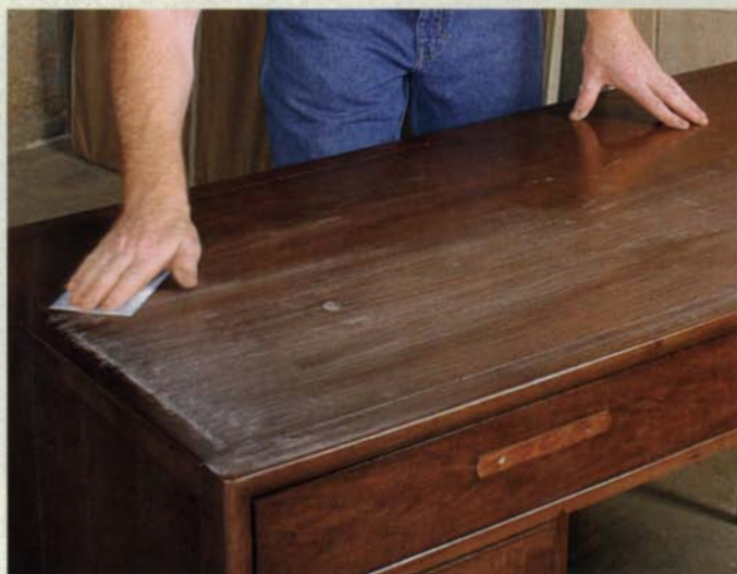
Sand before the final coat of lacquer. After the previous coat has dried, lightly sand the surface with 320-grit paper.
