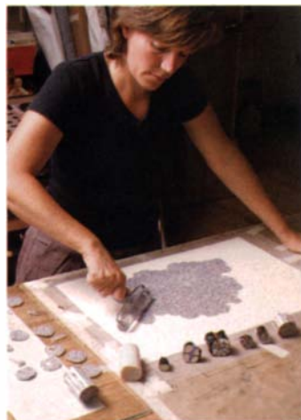
A step-by-step process. Single colors are rolled into canes, which resemble jelly rolls. The canes are combined and rolled into more complex canes, from which thin slices are taken. Last, the slices are lined up and flattened into continuous patterns.
