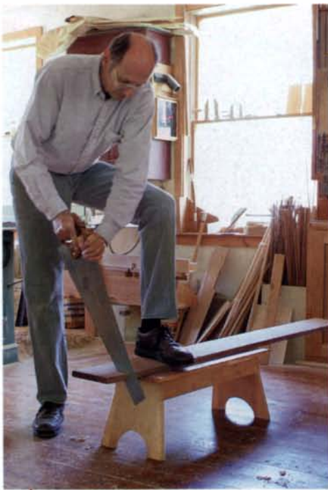
Stepping up for crosscuts. The 1-ft.-tall horse raises the workpiece so that you can use a crosscut saw comfortably.
