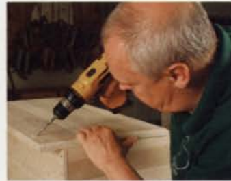
Drill holes for the legs. The angled holes in both the lid and the rear of the chest receive the two legs of each snipe hinge.
