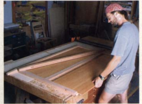
Assemble the back. The two back panels are slipped into the grooves in the frame parts and then clamped.
