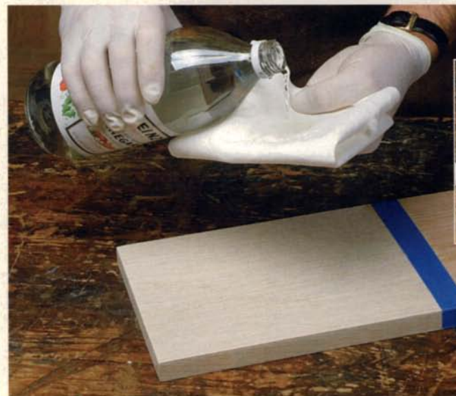
Start with two-part bleach. Some manufacturers say to mix the chemicals together; others say to use them separately.
