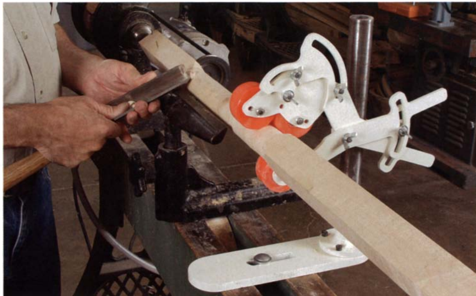
Steady as she goes. Oneway's new lathe steady rest sets up quickly, adds plenty of support and makes it easy to add or remove a workpiece.
