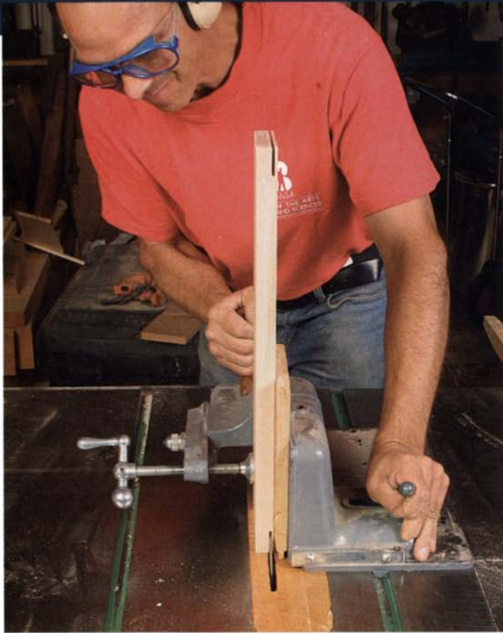
Tenons on the tablesaw. With the workpiece firmly clamped against this tenoning jig, the tablesaw can cut tenons cleanly and accurately.
