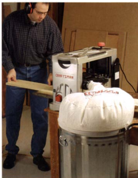
Can it. The Craftsman 21743 benchtop planer has a built-in dust collector that feeds chips into either a 30-gal. trash can or a 30-gal. plastic trash bag (cans and bags are not included).
