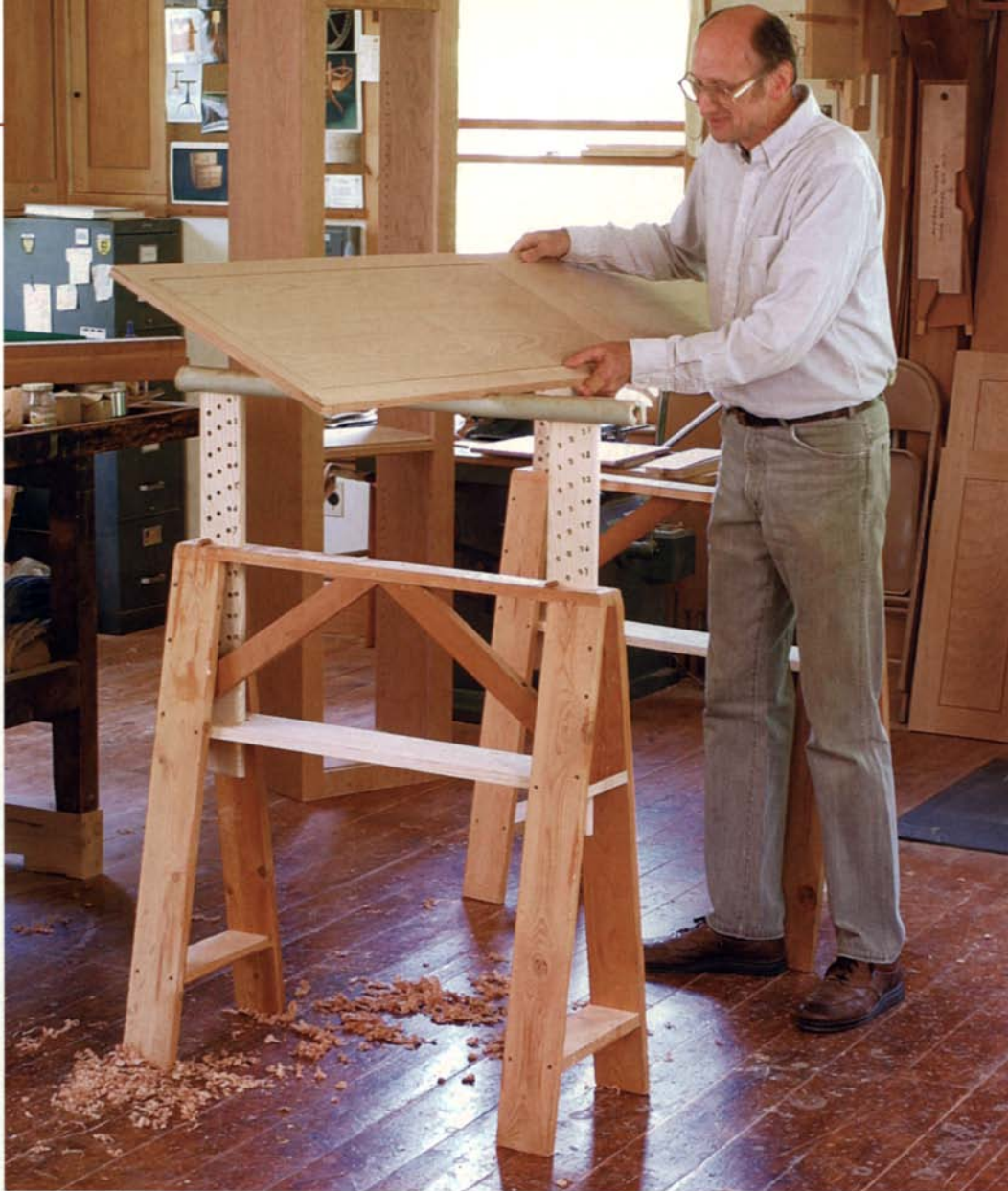
Ad adjustable-height sawhorses are versatile. Avoid back fatigue by raising the work up to a comfortable height.
