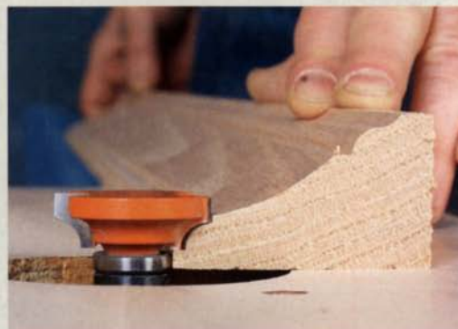
These bits were designed for use in a router table. The bearing is located between the shank of the bit and the cutter. The design makes it easy to apply a shaped edge to the molding.
