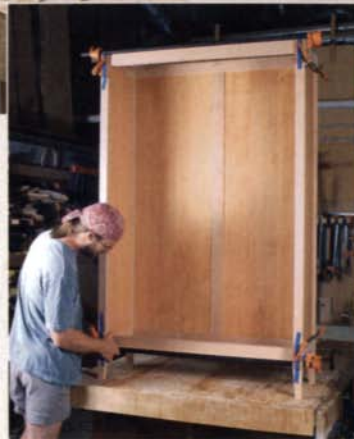
Add the remaining frame-and-panel parts. Once the back glue-up has dried, the remaining frame-and-panel parts are added in one big glue-up. First, the lower front rail is assembled to the two lower side rails, and then all four of the side rails are added to the back posts. Following in quick succession are the side panels, front posts and the upper rail (above). An assortment of clamps keeps the joints tight until the glue sets up (left).
