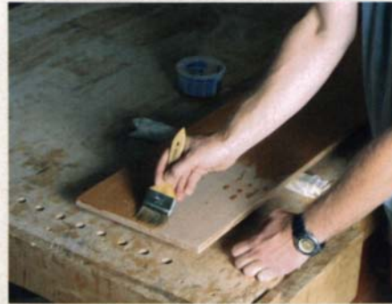
Finish the panels. Before assembly, the panels are finished with four coats of tung oil.
