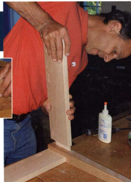
You don't need a lot of glue. With snugly fitting mortise-and-tenon joints, a thin layer of yellow glue spread evenly is all you need for a good bond.
