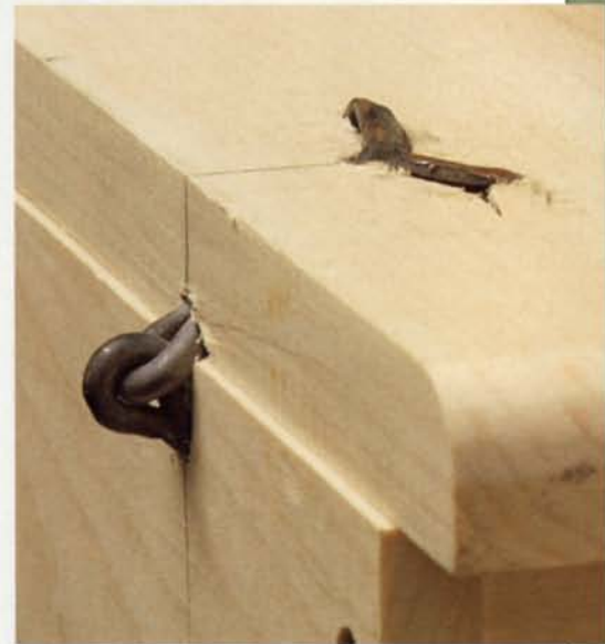
Completed snipe hinge. Pound the bent legs flat with a hammer, then file them flush with the surface. They will be barely visible under a coat of paint.
