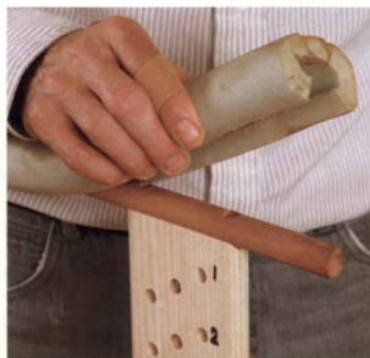
Pad the crossbars to protect your work. Foam pipe insulation works well and easily slips on and off the top.
