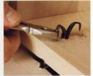
Make fish hooks. Pry apart each pair of soft iron legs with a screwdriver. Then use pliers to bend over the point 180°.
