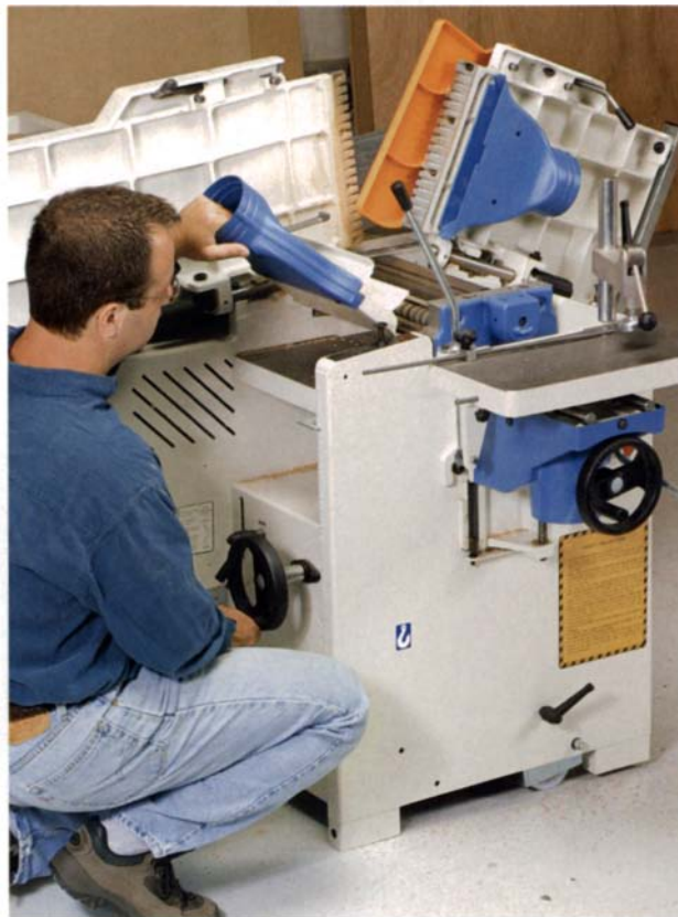
Quickest planer-jointer conversion in its group. As on the Knapp (p. 59), the planer dust hood is smaller, meaning the planer bed does not have to move as far during the changeover. However, the rip and jointer fences have to be moved or removed.
