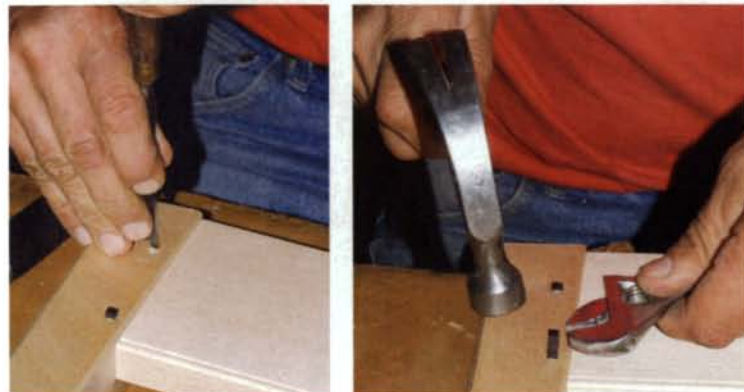
Pins are an insurance policy. Small hardwood pins will hold the joint tightly, even if the glue fails. Hack leaves the outside end of the pin square and holds it with a wrench as he hammers it home.
