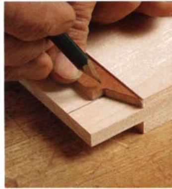
Trim tenons to size and shape. A matching template made to the negative shape of the one used to check mortises shows where to cut the angled haunch on the tenons. The first cut is made with a stop block on the miter gauge.
