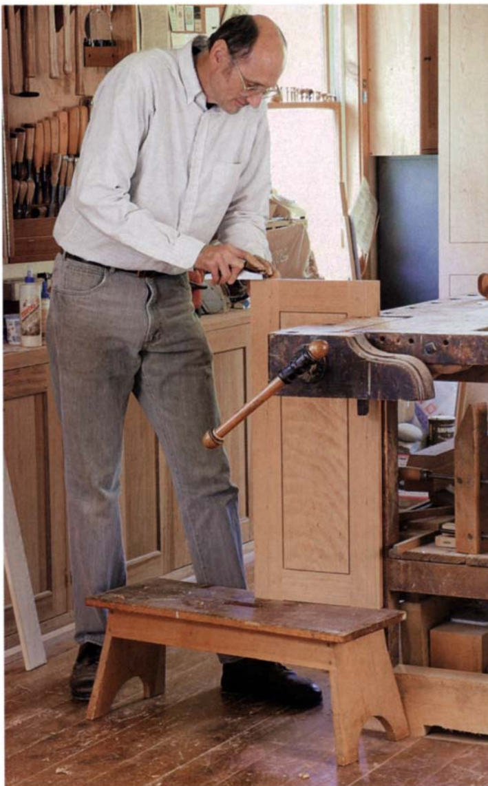
Use horses in conjunction with your bench. While a workpiece is secure in the vise, the short horse provides solid support from below.
