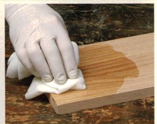
One application is usually enough. To remove all of the color from a piece of lumber, a second application may be necessary.
