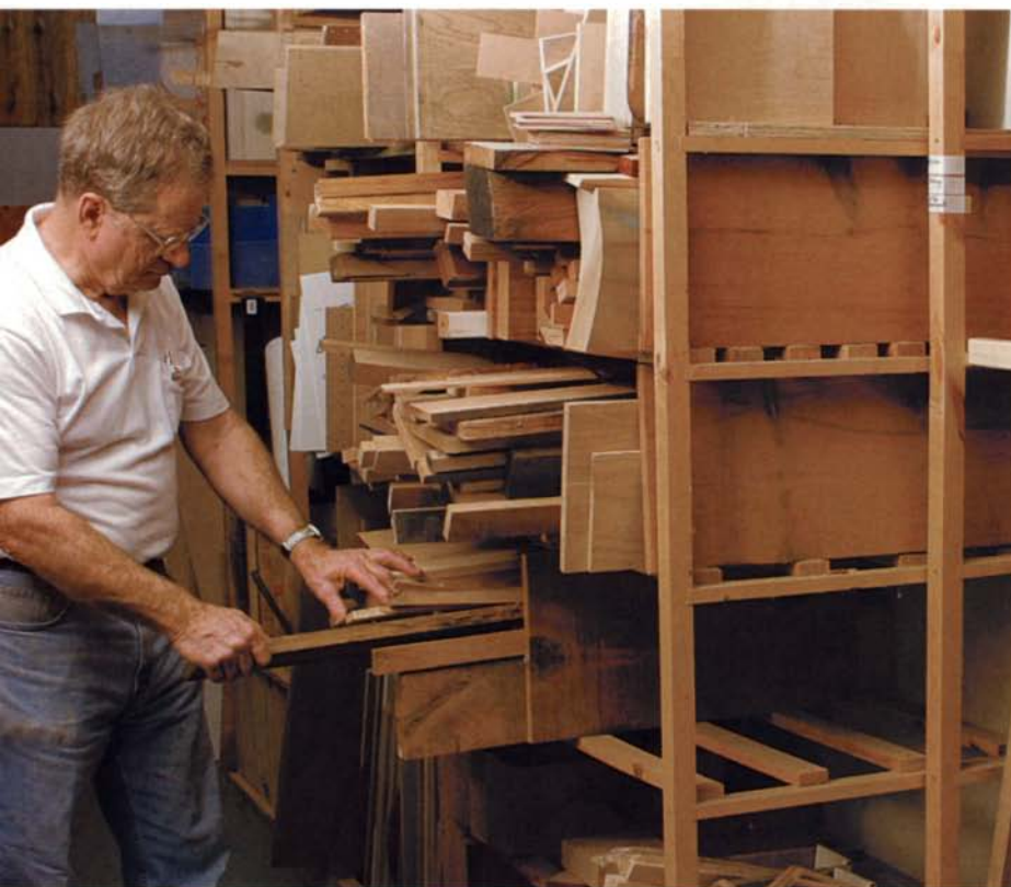
Adjustable wood storage rack. The rack is converted from horizontal storage to vertical storage by simply removing the cross pieces.
