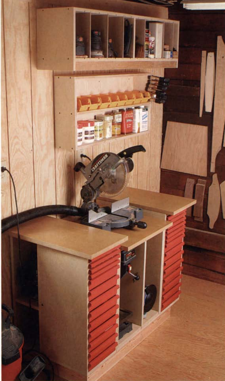
A well-thought-out corner of the shop. The chop saw station not only provides good outfeed support for the saw, but it also stores the grinder and the drill press and houses two banks of drawers.
