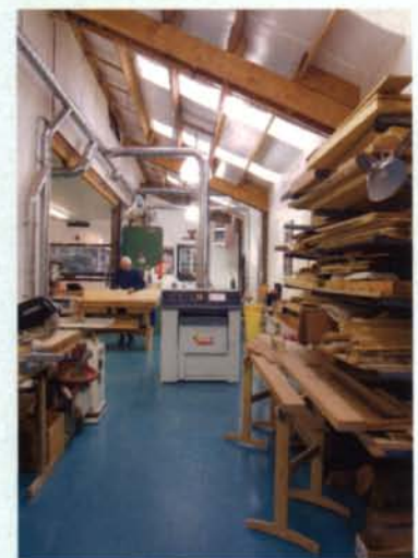
Efficient layout. Machines are arranged so that wood progresses in logical order from the lumber rack through all of the workstations.
