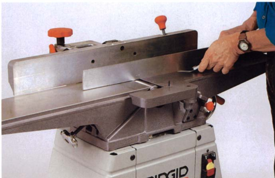
Are they flat? Shop manager John White checked the grinding job on infeed and outfeed tables with a straightedge and feeler gauges and used a machinist's level to measure the diagonal twist. Most of the measurements fell well within accepted tolerances.
