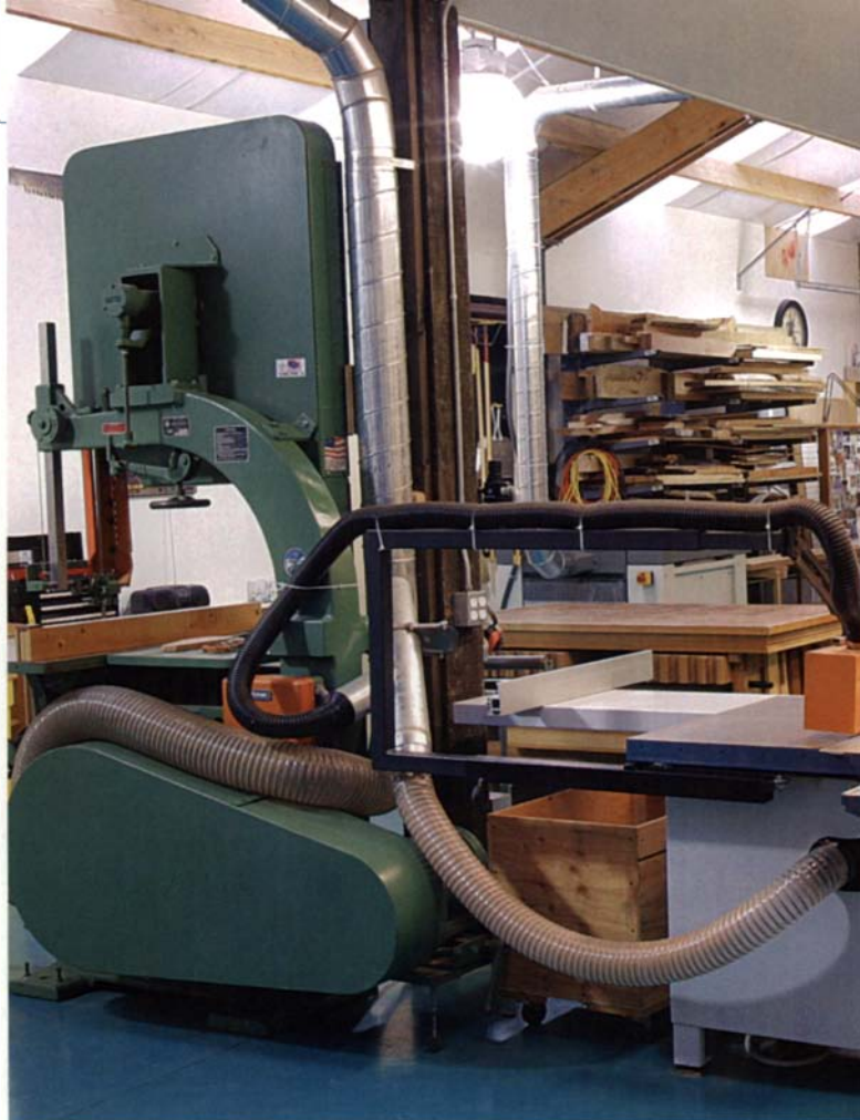
Dust collection for large machines. The 36-in. bandsaw and sliding tablesaw are grouped together so that they can share a duct for efficient dust collection.
