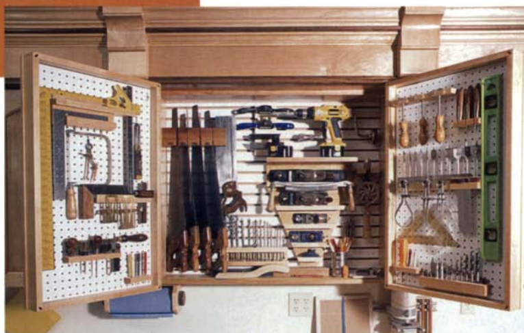
T-slotted panels, common in retail displays, are used inside the cabinets. Custom-made tool holders fit into the slots. The backs of the doors are fitted with Peg-Board.
