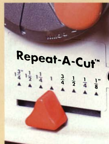
Gauge shows depth of cut. Some of the planers feature a gadget that quickly lets you see how much stock the next cut is going to remove.
