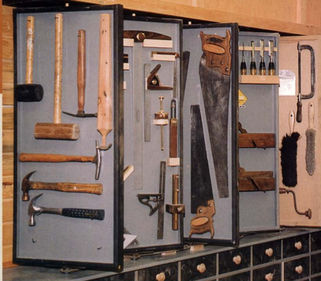
Five-panel tool rack revolves. Johns' tool rack provides about 40 sq. ft. of storage while taking up only 15 sq. ft. of wall space.
