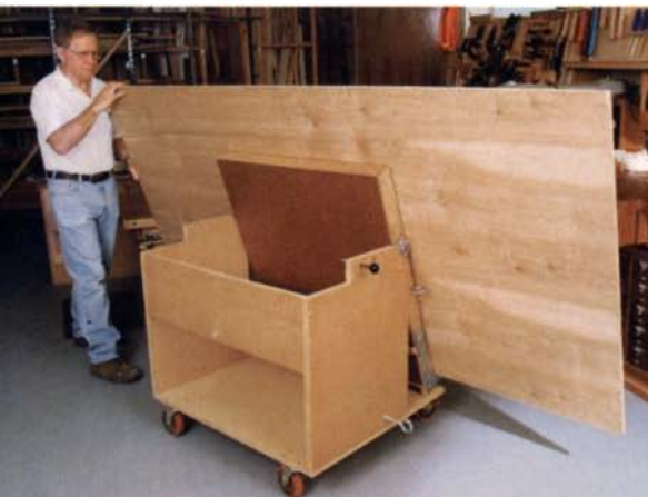
The L-shaped tilting top holds several sheets of plywood. A pin locks the tabletop in the horizontal position. Large locking casters can handle bumps in the concrete without stalling. Pillow blocks make for a smooth pivoting action.
