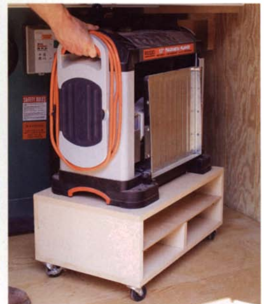
Or make one yourself. Teague's planer base is nothing more than an MDF box with locking casters screwed to the bottom, and it includes shelves as well.
