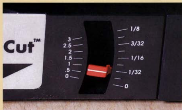
Gauge shows depth of cut. Some of the planers feature a gadget that quickly lets you see how much stock the next cut is going to remove.
