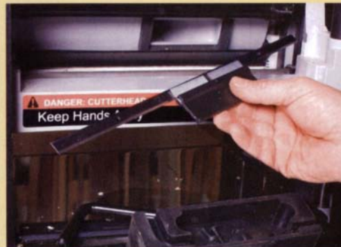
Changing knives shouldn't be a chore. Depending on the machine, the job can take anywhere from five to 25 minutes.
