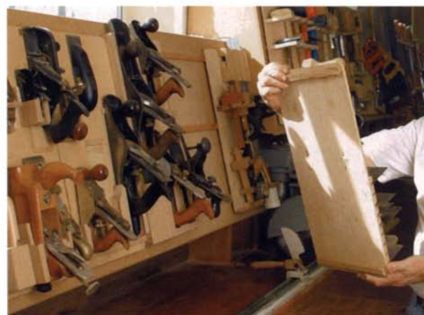
Angled tool racks are placed above the bench. Individual tool holders are attached to the rack with French cleats.
