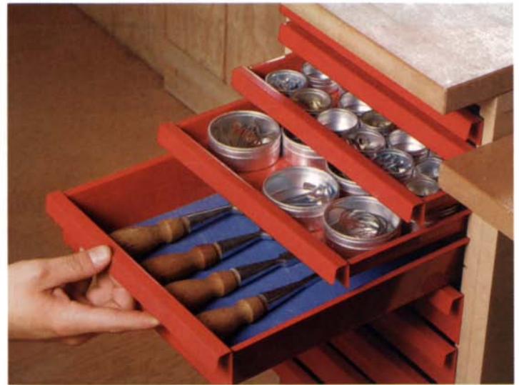
Drawers are like clamps—you can never have enough. Metal drawers slide in sawkerfs in the carcass. Hardware and fasteners are stored in watchmaker's cases. Drawers for cutting tools are padded.
