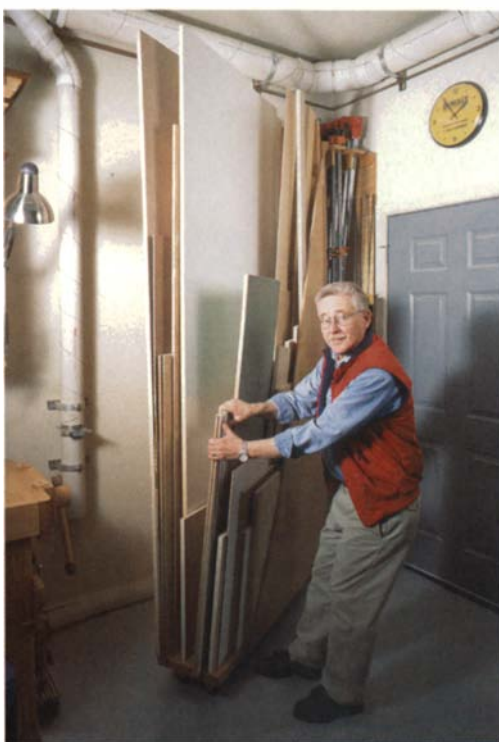
Swiveling vertical storage unit. One edge is fastened to the wall with heavy hinges, and casters underneath allow the unit to pivot for easy access.
