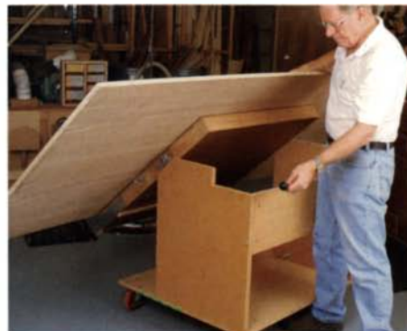
The L-shaped tilting top holds several sheets of plywood. A pin locks the tabletop in the horizontal position. Large locking casters can handle bumps in the concrete without stalling. Pillow blocks make for a smooth pivoting action.
