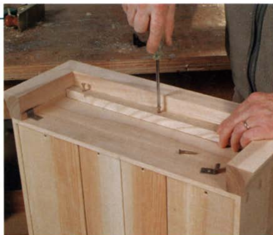
Attach the cornice to the case. The front cornice piece is screwed through the cleat. The side pieces are attached with buttons, which allow for wood movement.
