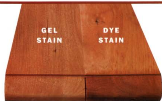
A tale of two stains. The gel stain on the left imparts an even color over the whole piece of wood. The dye stain on the right creates a blotchy finish on the face grain and an ugly, dark end grain.
