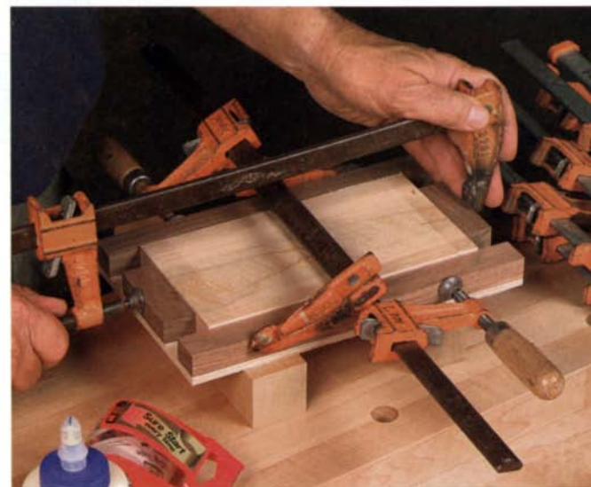
The guide blocks are glued to the base of the jig. Clamp the guide blocks both to the set-up block (center) and to the top face of the jig. Thin packing tape on the set-up block makes it easier to remove after glue-up.
