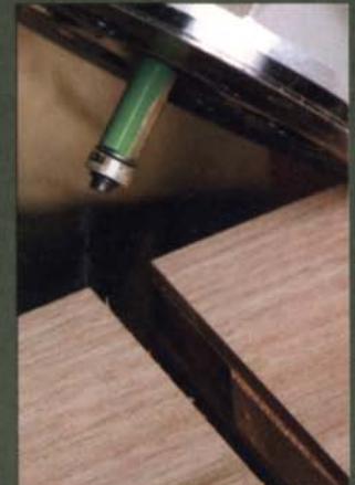
Clean up the sabersaw cut. Use a router equipped with a bearing-guided, flush-trimming bit.
