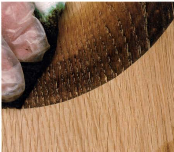
Due to surface tension, water has trouble penetrating the pores of open-grained woods. As a result, specks of unstained pores are left across the surface.
