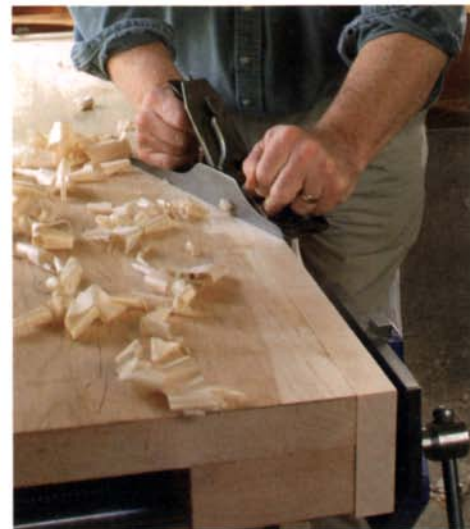
Plane the top edge of the face. A sharp handplane is all it takes to get the face flush with the top of the bench.
