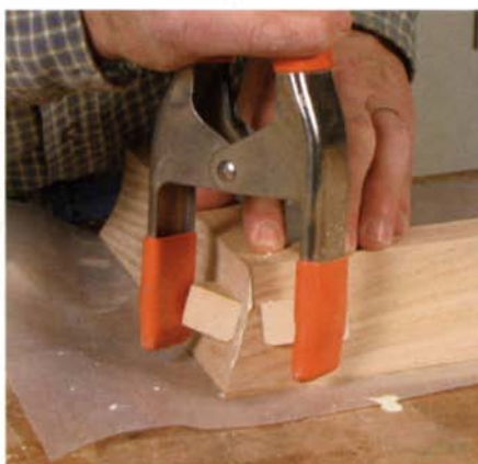
Triangular blocks add bite to spring-clamp jaws to close up miters. Attach the blocks with hot-melt glue, and chisel them off after the cornice is dry.
