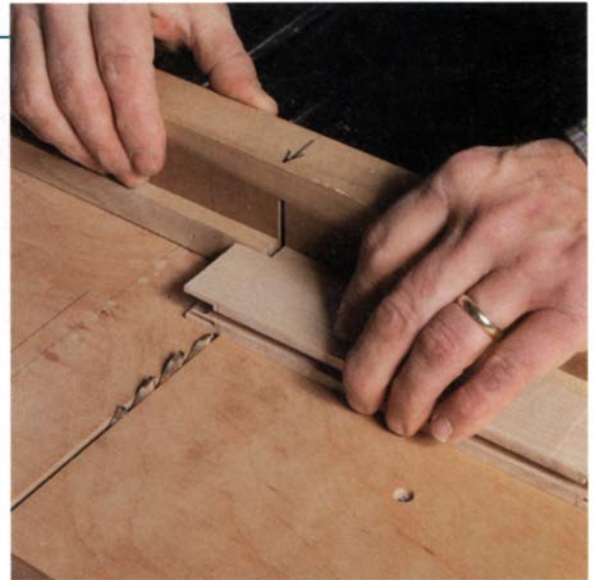
Trim the tapered shoulders on a sled. Nail offcuts from the stiles to a tablesaw sled or miter gauge. The offcuts will provide the correct shoulder angle.
