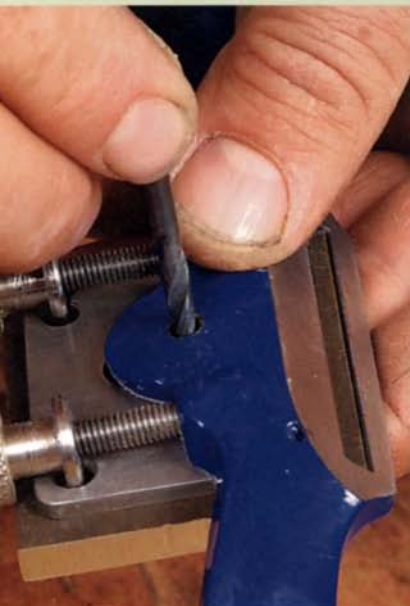
Next, mark for the center hole. This simply is a clearance hole for the center screw, which threads into the body of the tool.
