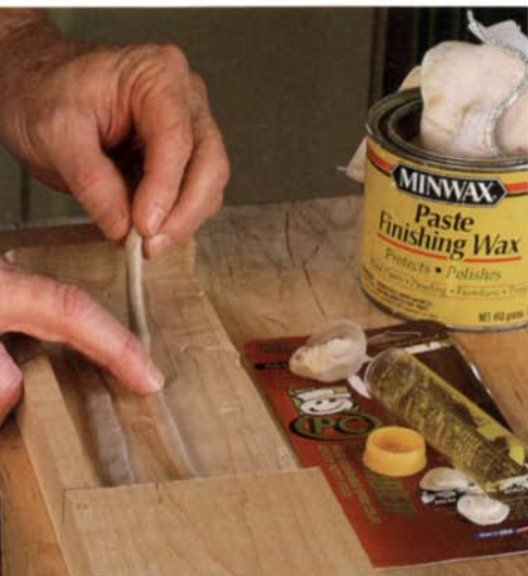
Attach the back face to the edge of the benchtop. To fill in the gap between the back face and the back jaw of the vise, add a couple of strips of epoxy putty to the mortise just before applying the face to the bench (left). After coating the jaw with paste wax, attach the face with a few wood screws driven into counterbored holes (right).
