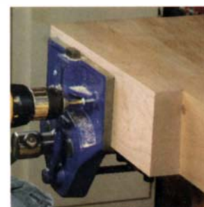
Add the front face. Like the back jaw of the vise, the front jaw is tapered. To minimize the effect of the taper, you can bevel the outside surface of the front face slightly. Then attach the face by driving two screws through predrilled holes in the jaw.
