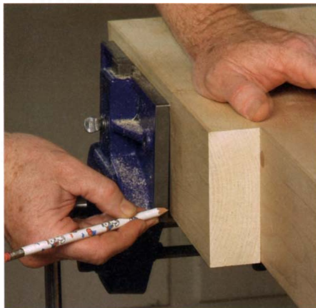
Add the front face. Like the back jaw of the vise, the front jaw is tapered. To minimize the effect of the taper, you can bevel the outside surface of the front face slightly. Then attach the face by driving two screws through predrilled holes in the jaw.
