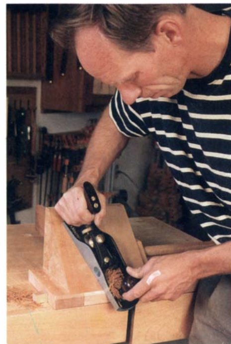
A smooth smoother. The plane was comfortable in most assignments, whether working end grain, long grain or miters.
