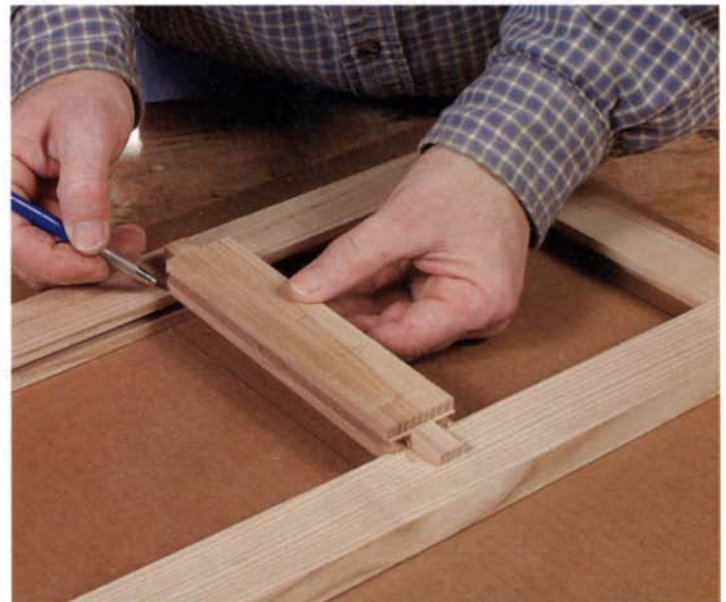
Fit the middle rail. Dry-fit the door frame and fit the middle rail to the piece, using a full-sized drawing as a guide.
