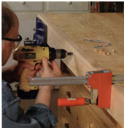
Attach the back face to the edge of the benchtop. To fill in the gap between the back face and the back jaw of the vise, add a couple of strips of epoxy putty to the mortise just before applying the face to the bench (left). After coating the jaw with paste wax, attach the face with a few wood screws driven into counterbored holes (right).
