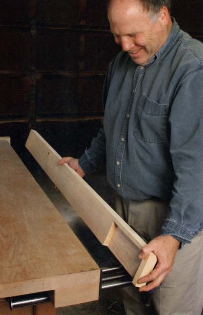
A long face. A mortise in the back face accepts the back jaw. The face extends the full length of the benchtop, which will make it easier to clamp long boards.
