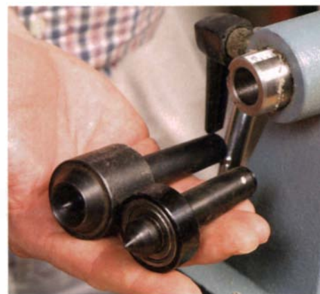
Better and best. Only the Nova uses a live single-point center (right) in the tailstock; the other midis use a live cup center (left). The students favored the live-cup version.
