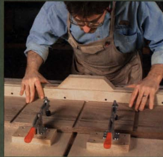
Dado one side at a time. After setting the blades to the right height, make all of the dado cuts on one side of the verticals. Transfer the cut lines for the dados on the second side with a square and a sharp pencil.
