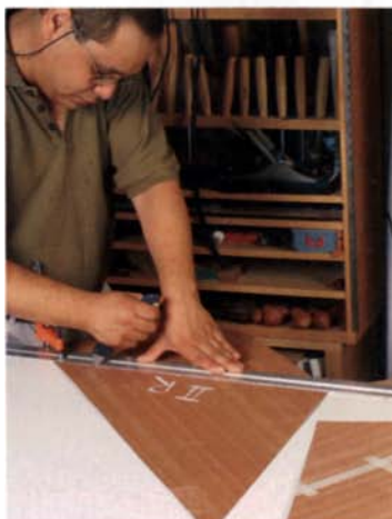
Cut triangles off the top. Use a straightedge and mat knife for quick, clean cuts.
