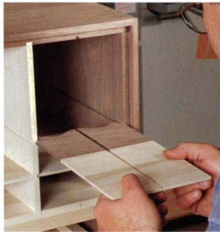
Horizontal dividers are next. To prevent binding during assembly, glue is added only along the front edges of the joints.
