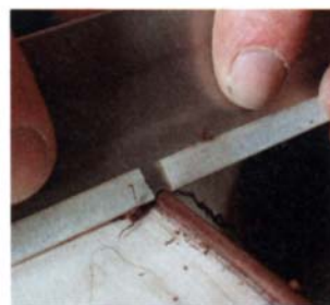
A shopmade scratch stock. O'Malley filed a notch into a scraper to make a scratch stock. Masking tape protects the apron.
