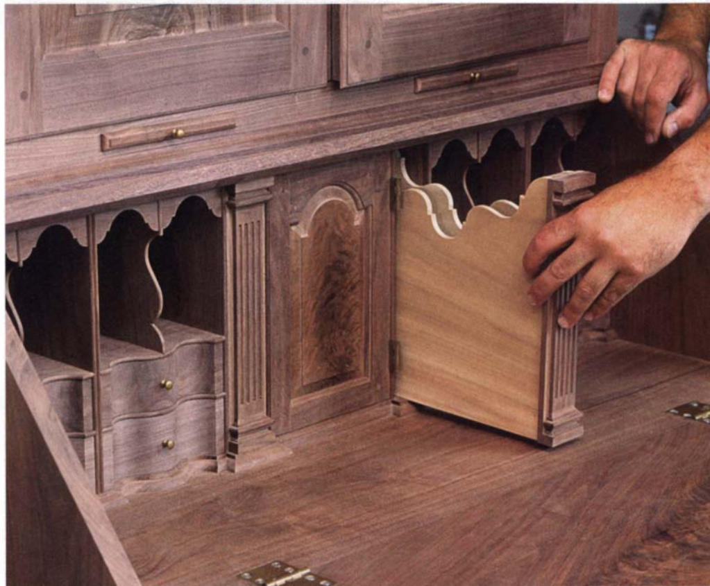
Installing a desk gallery, p. 66
