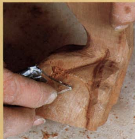
Clean up carvings. A piece of glass with a sharp point gets into tight corners, such as those found on carvings.
