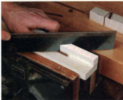
Hand tools are safer. Although these small pieces of beading can be mitered on a chopsaw, it is safer to use a backsaw with a shopmade miter box.
