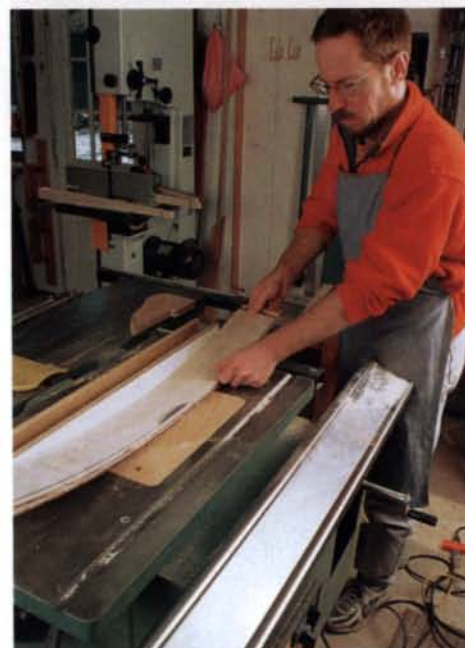
Cut the front apron to width. Before making the actual cut, practice sliding the curved apron past the stationary blade. Maintain a steady angle at the cutting point.
