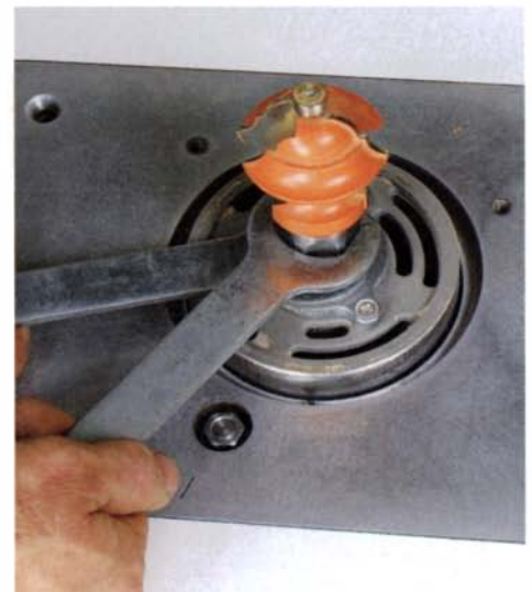
Above-the-table bit changes. Both ProLift models let you raise the router collet above the table, so bits can be changed from on top.
