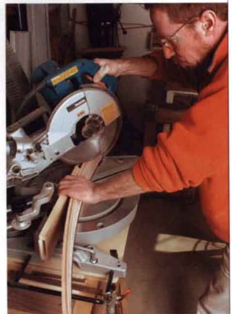
Trim the front apron on a chopsaw. The false drawer front is cut at an angle to preserve the seamless appearance of the apron.
