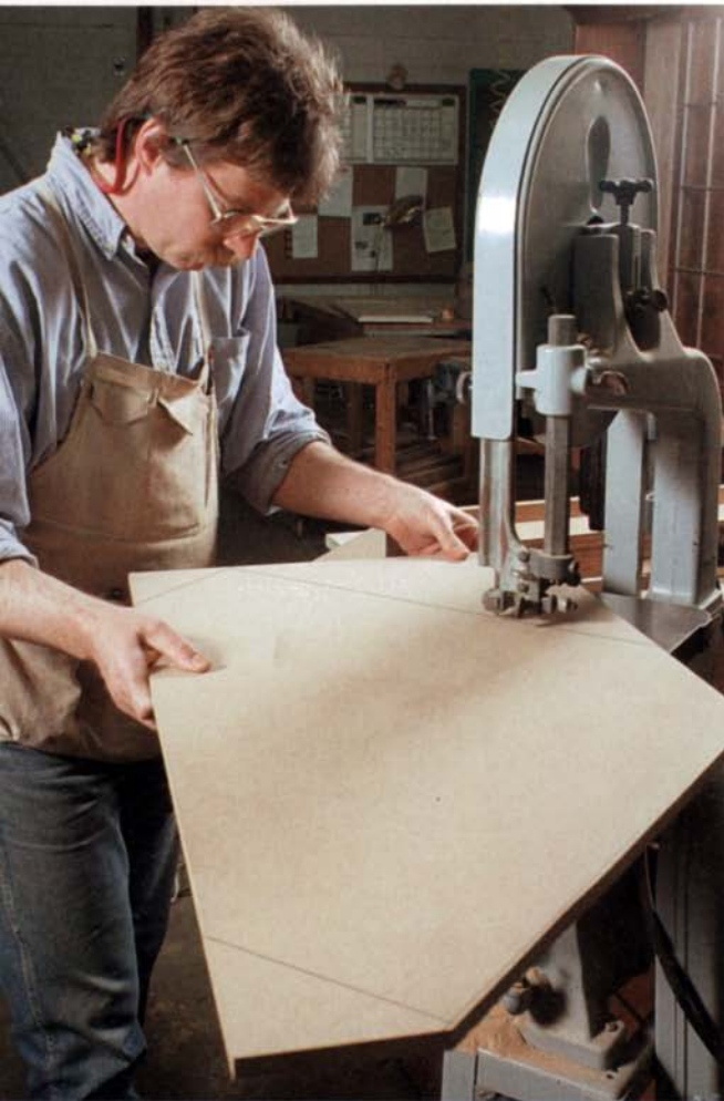
Odd shapes are no problem. After drawing a pattern on MDF for a corner-cabinet shelf, Latta rough-cuts the waste on a bandsaw, staying about \frac{1}{16} in. off the line.
