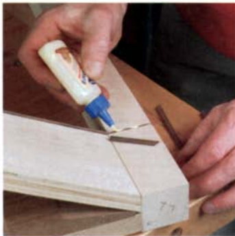
Fit the beads. The lower beads are best fitted before table assembly. Those near the top must wait until the front apron is attached.
