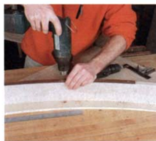
Screw the bead to the underside of the front apron. Avoid the area where the drawer will be cut and in the center where the fingerhold is routed.
