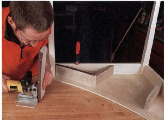
Biscuits join the apron to the drawer rails. The sharp angle at the end of each front rail demands care when using the biscuit joiner.
