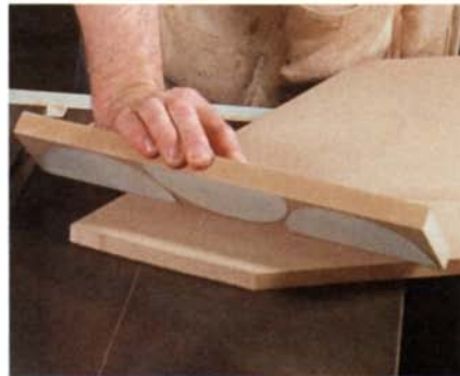
Make a push stick from MDF. Attach sandpaper to the underside of the push stick for a secure gripping surface.
