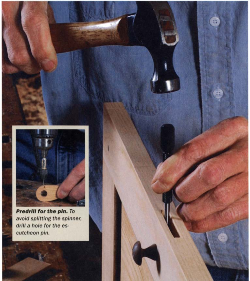
Secure the spinner and knob with a pin. Instead of glue, use a small brad or escutcheon pin and drive it in using a nailset.
