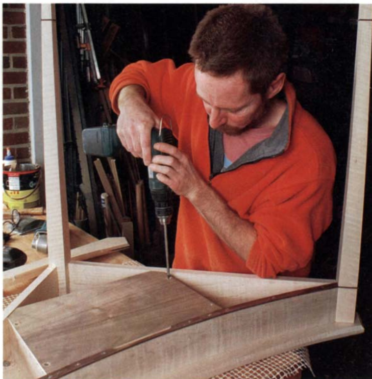
The drawer panel serves as a runner for the drawer. It also adds rigidity to the structure.
