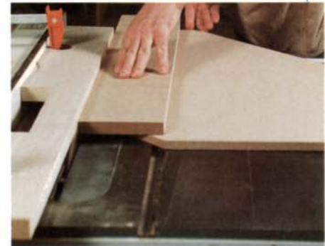
Place the push stick directly on a layout line. Press the stick firmly against the auxiliary fence and the pattern to prevent slipping during the cut.
