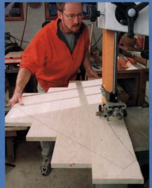
Rough-cut the tabletop after tracing the template. Minimize the waste of wood by stepping the glue-up to create a semi-triangular shape.
