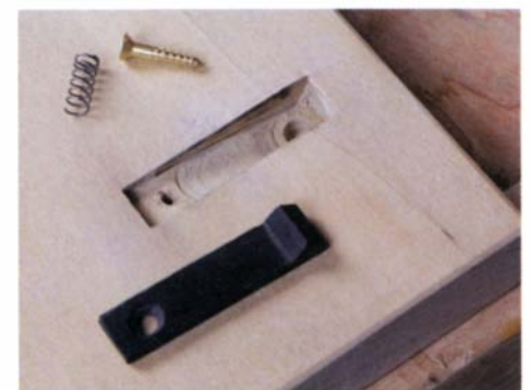
Assemble the catch. The spring sits in a hole bored in the deep end of the mortise.
