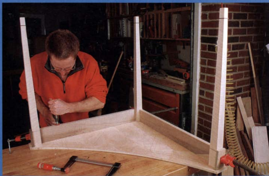
Assemble the rear of the table. After the legs and the side aprons have been cut, glue them together using the template as a guide to squaring them up.
