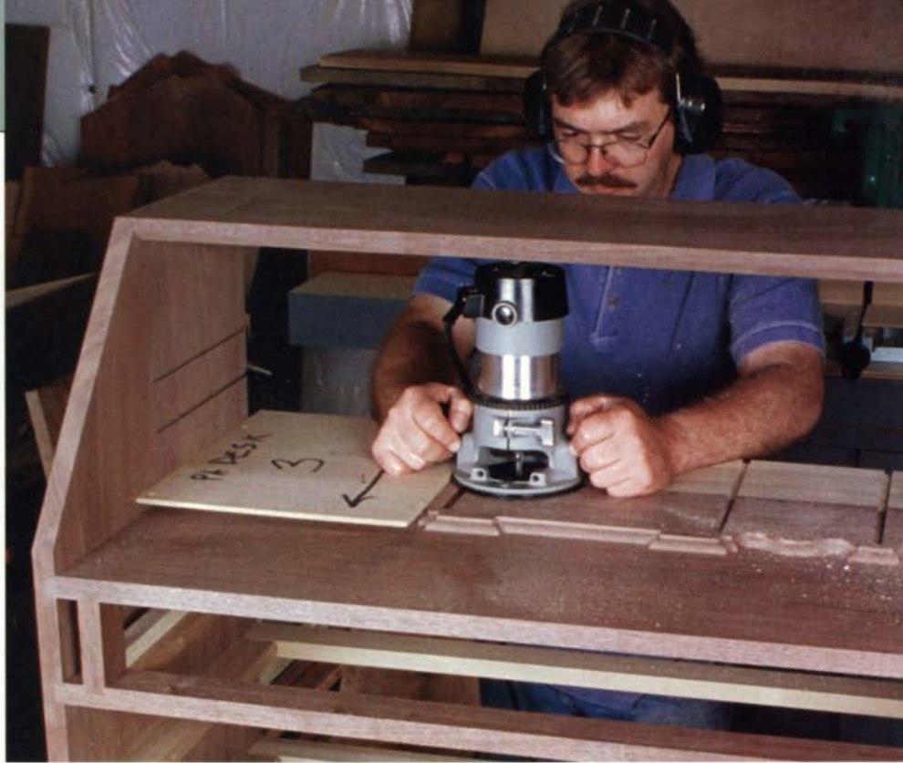
Dado the seat board and the case. Once the seat board has been set into place, use a straight bit to rout the dados. Templates ensure that all corresponding dados align.
