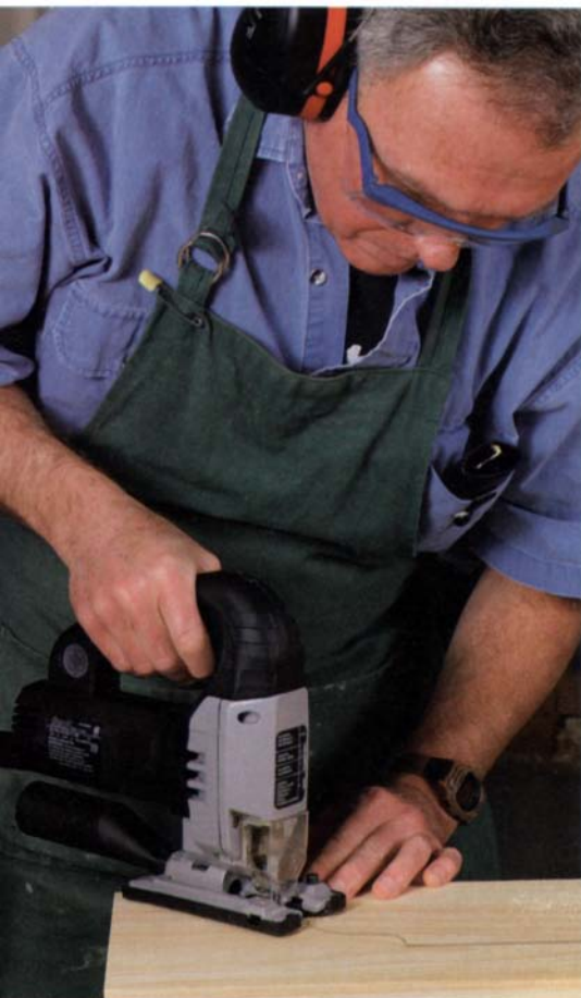
A jigsaw with cruise control. Freud's new jigsaw has a unique electronic feature that maintains the blade speed, even when the blade runs into a hard material like a knot.
