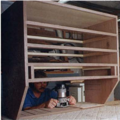
Dado the seat board and the case. Once the seat board has been set into place, use a straight bit to rout the dados. Templates ensure that all corresponding dados align.
