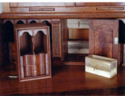
Hidden away. The gallery features a tombstone prospect door that opens to reveal a prospect box. The box can be removed to reveal three hidden drawers.
