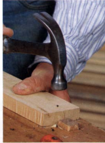
Planing thin, curved stock. A brass escutcheon pin tacked into a flat board serves as a ministop for smaller workpieces. Because brass is soft, it won't damage your tools if you run into it.
