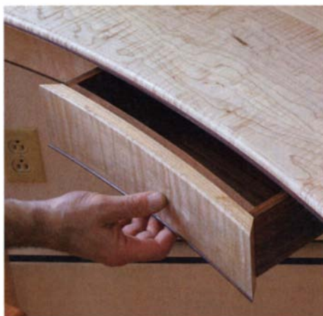
A place for your stuff. The drawer blends in with the front apron, making it nearly invisible. A fingerhold in the false front is easy to grab.
