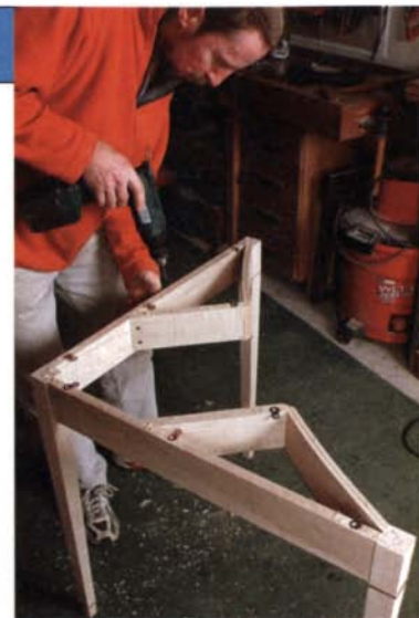
Firm yet flexible. The tabletop is attached with figure-eight fasteners, which allow for seasonal movement.
