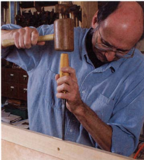
Chop out the mortise. Becksvoort chisels out the mortise by hand.
