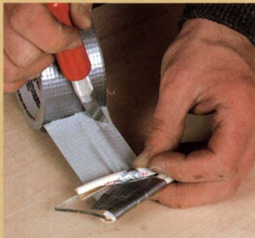
For safety, wrap the three unused sides of the scraper with electrical cable insulation. Secure it with duct tape.
