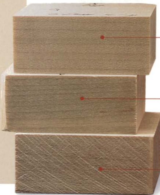
A RIP-CUT SURFACE AFTER HANDPLANING
