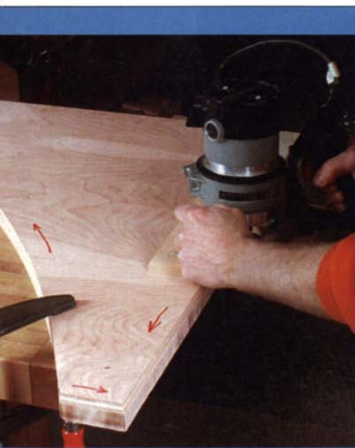
Flush-trim the edges. Using the template as a guide, flush-trim the edge of the tabletop. The arrows on the template indicate the routing direction to minimize tearout.
