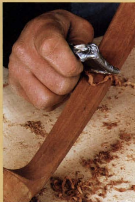
The scraping cut. Angled slightly forward from the vertical, the scraper removes stock quickly over curved surfaces.
