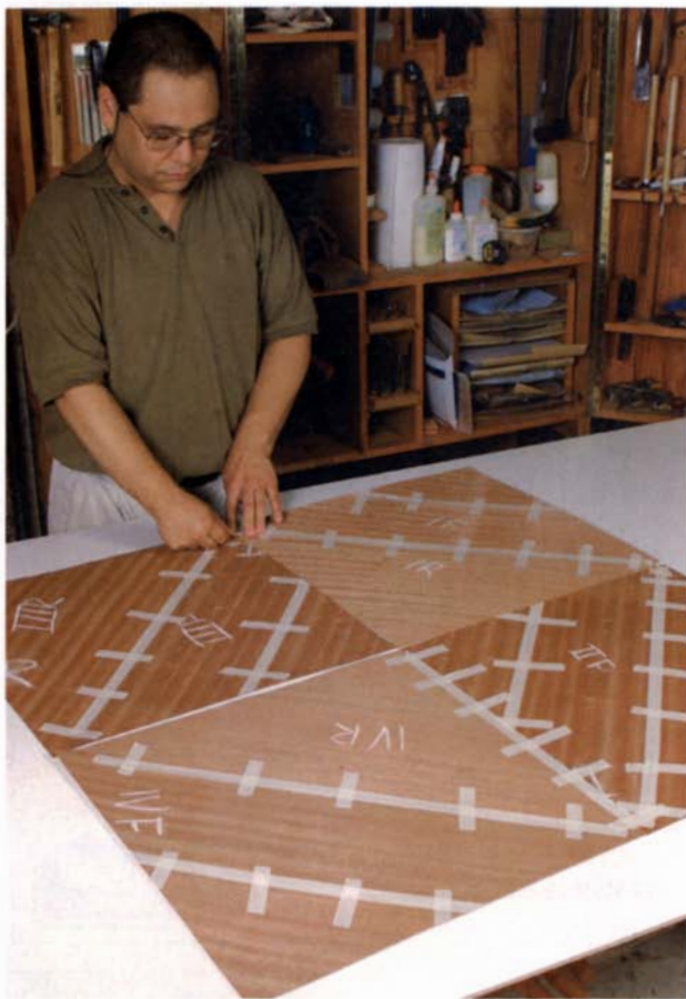
Join the rectangles to form a diamond pattern. Tape the new seam temporarily and then create the reverse-diamond pattern as shown at right.
