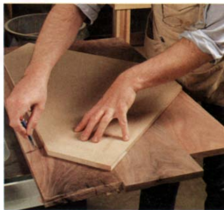
The pattern has two purposes. Trace the shape onto the workpiece for rough-cutting on the bandsaw. Then use it as a template for final trimming on the tablesaw.
