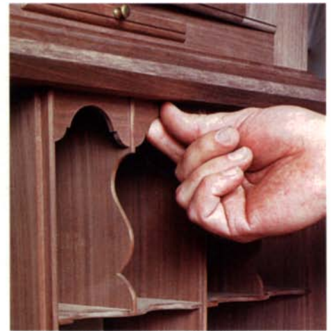
Valances are a nice touch. Bird glues them to the tops of the pigeonholes. He adds glue blocks later for additional support.
