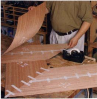
Book-match the rhomboid shapes into pairs. Tape these seams temporarily to keep track of the orientation.
