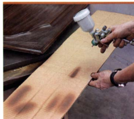
Before spraying a shading finish tinted with color, use a scrap of cardboard to set the size of your spray pattern.
