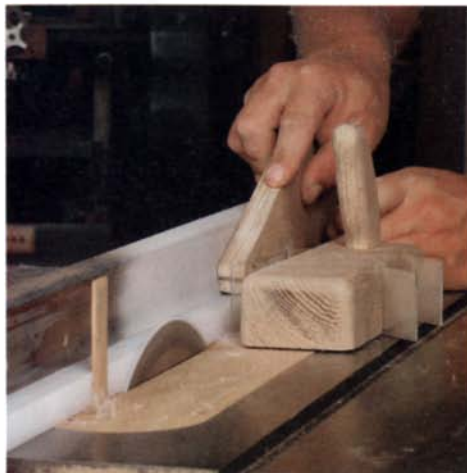
Rip the plastic runners. A combination blade makes a smooth cut in UHMW plastic.
