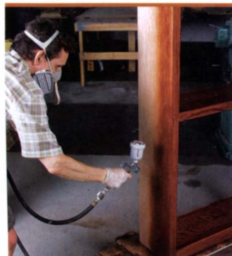
With a touch-up gun you can apply stains fast and evenly. Here, Jewitt uses the gravity-feed touch-up gun with a plastic cup to spray a water-based dye stain on an oak bookcase.
