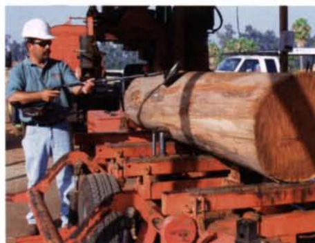
Metal detection. A common problem with nonforest logs such as this redgum is the risk of them containing nails, bits of fence wire and other blade-damaging objects.
