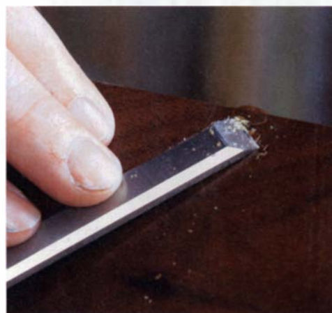
Shave off surplus filler. A few strokes with a sharp chisel pare away most of the filler that is proud of the wood. A smooth finish is achieved with 600-grit wet-or-dry sandpaper wrapped around a block of wood.
