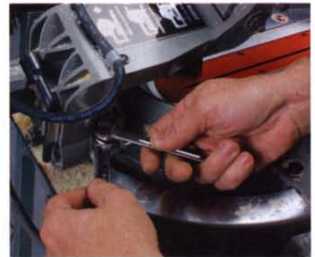
Two wrenches required. To adjust the 45° and 90° stops, you may have to tilt the saw head to access the bolts and locknuts.
