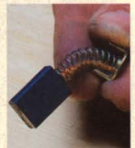
This brush is still in good shape. Worn-out brushes can lead to sparks coming from the motor, and they can indicate a loss of power. Replace brushes when they get too worn, which would be about half the size of the one shown here.
