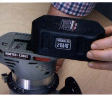
Easy on and off. The battery slips easily onto the motor housing and locks in place. Push a release button, and the battery will slide right off.
