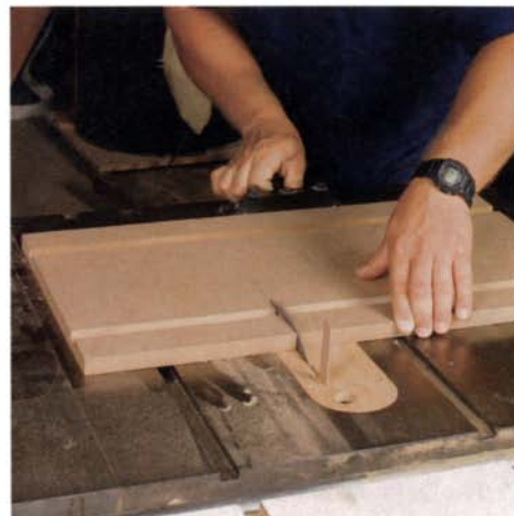
Cut the blank in two. Crosscutting the blank provides stock for the base and platform.
