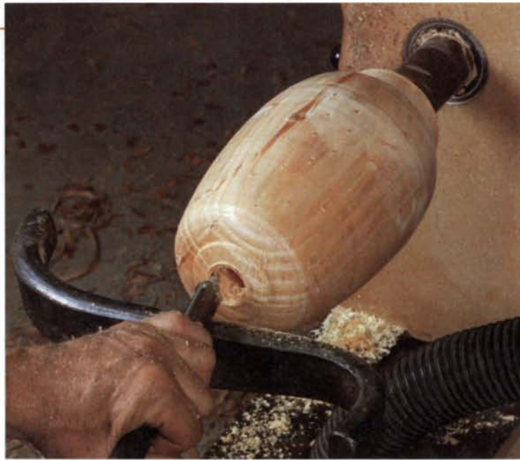
Open the entrance. This is done with the articulating tip of a boring bar set in a straight position.
