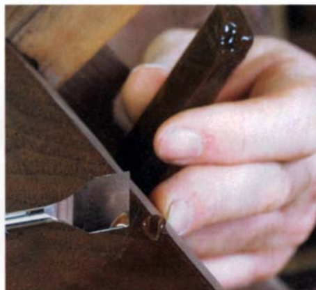
Apply the burn-in material to the cavity. Don't worry about forming a smooth surface. The first step is to fill the void.
