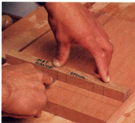
Mark the outlines and spacing of the mortises in the top. With two lines already scribed to mark the thickness of the mortises, use the layout gauge to mark the other edges.
