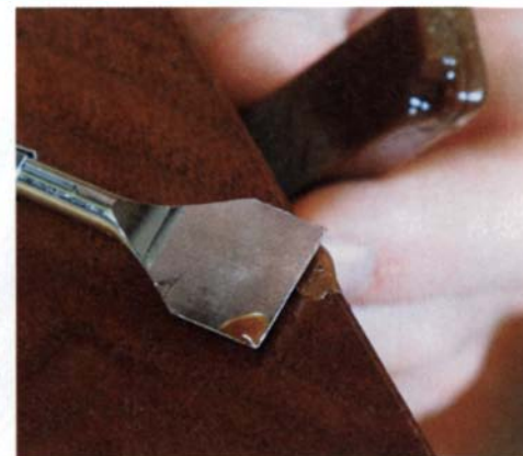
Smooth and compress the filler. Drag the hot knife across the surface to level the shellac with the surrounding wood.
