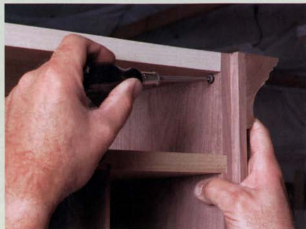
Attach the molding. While traditional period pieces were often face-nailed, Bird installs the crown molding using unseen screws set into elongated holes.
