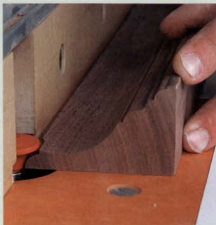
Finish the job at the router table. Once the cove has been cut, an inverted cutter trims the top profile in a single pass. A small lipped roundover finishes off the crown molding.
