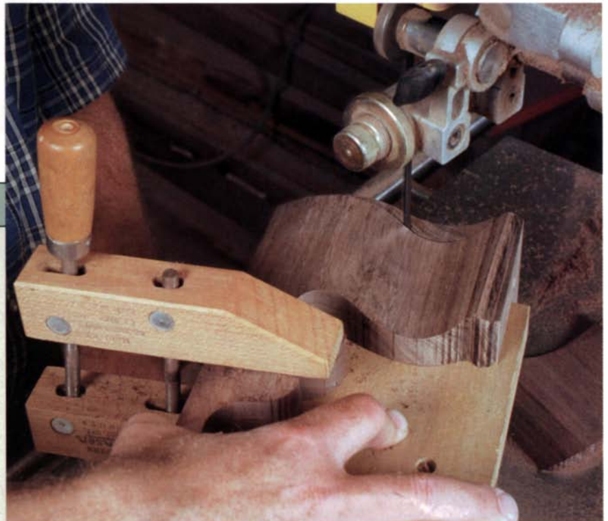
Follow the glueline. Once the first profile has been cut, simply follow the exposed glueline to make sure the two sides match.
