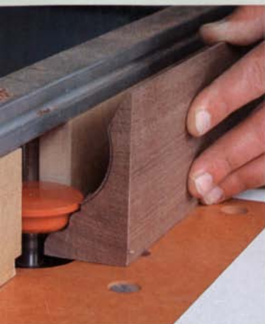
Finish the job at the router table. Once the cove has been cut, an inverted cutter trims the top profile in a single pass. A small lipped roundover finishes off the crown molding.
