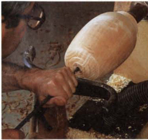
Drill a deep hole to establish the final depth. Lewin uses a long drill in a handheld chuck, supporting the bit on a tool rest. He pauses every 1 in. or so to clear chips, and he checks the depth frequently near the bottom.
