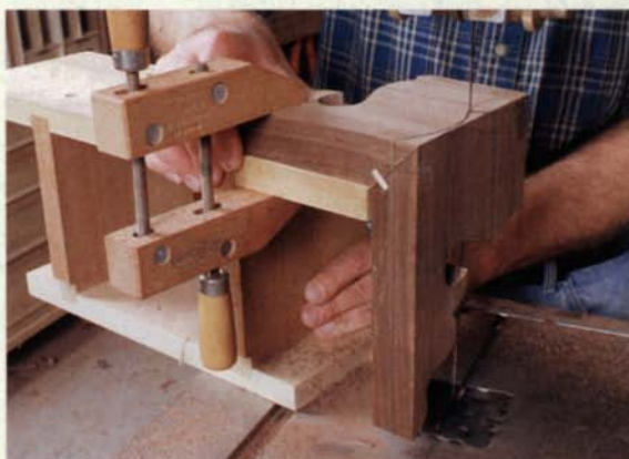
Quick jig helps profile the feet. With the feet clamped to an elevated jig, rough out the side profile of the feet on the bandsaw.
