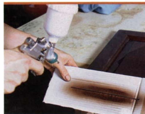
A mask makes a cleaner touch-up repair. A piece of posterboard with a sawkerf cut through it limits the amount of stain and finish applied to an edge on which the color has been rubbed through and removed.
