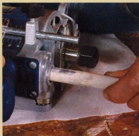
Work on the bores. A cleaning stick, made from a piece of paper towel wrapped around a dowel, is used to clean out the holes that accept the guideposts.
