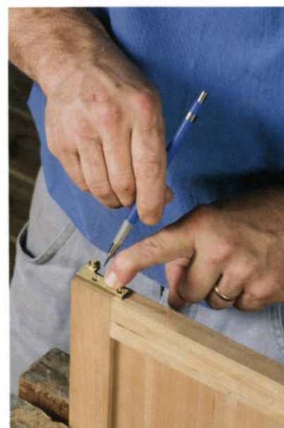
Mark the location of the door hinges. Layout is done after the doors have been fitted to the case opening.
