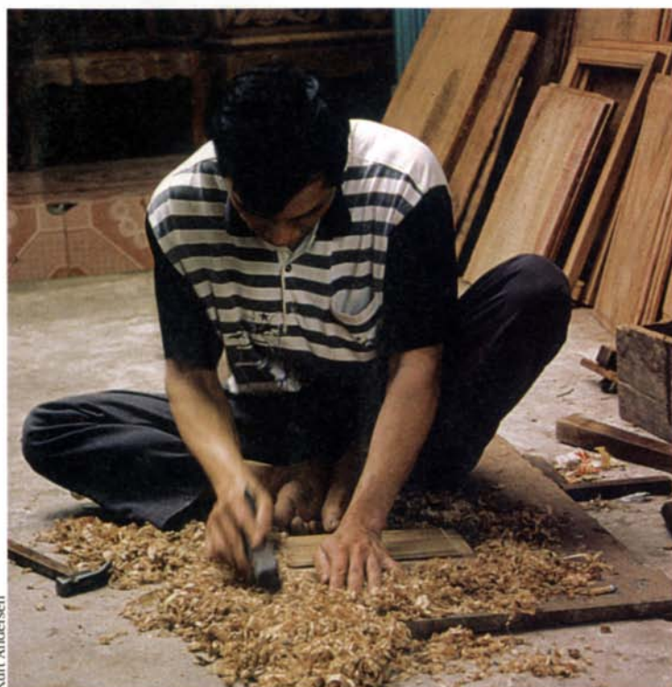
A footrest and a hand tool. Andersen never saw a bench or a vise in the village, but much of the hand-tool work is of a very high standard.
