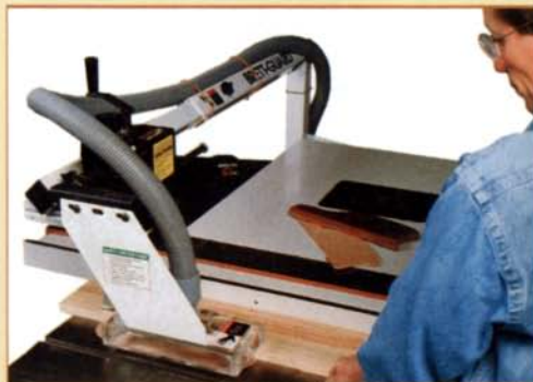
The Brett Guard is heavy duty and easy to use. But using a splitter with it is problematic.
