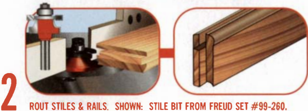
2 ROUT STILES & RAILS. SHOWN: STILE BIT FROM FREUD SET #99-260.
