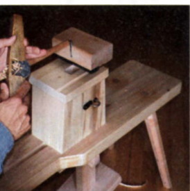
Puppet system. The optional puppet system lets you clamp a workpiece between centers. That way you can work the entire length of the piece.
