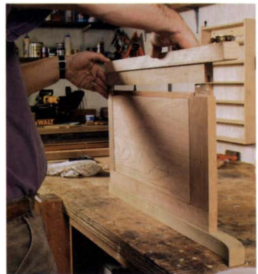
Complete the side. Finish by attaching the other stile and leg, which have been biscuited. Glue and clamp horizontally.
