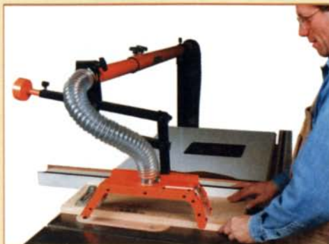
The Exaktor blade cover is similar to the Excalibur. However, the flat front on the cover doesn't ride up and over workpieces, and the extension arm is difficult to adjust.
