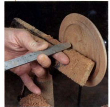
The two sides of the wax cup. Turn the piece on a screw chuck and refine the inner and outer surfaces with a scraper.
