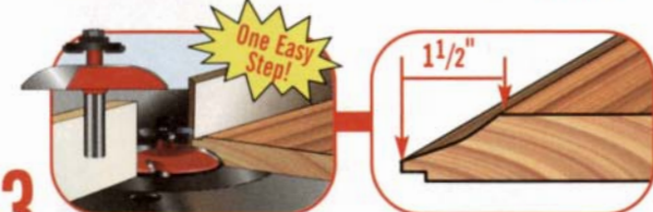
3 IN ONE STEP, ROUT DOOR PANEL PROFILE AND BACK CUT.
