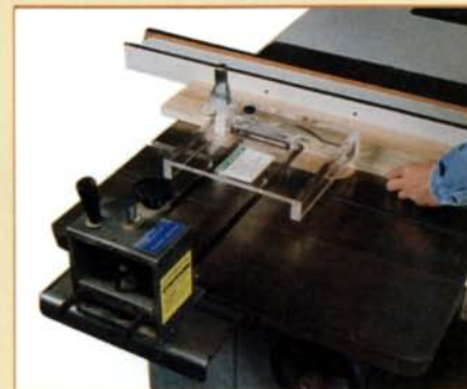
The original Brett Guard mounts on the saw's left edge. It can be added to any saw, but its position limits cutting capacity on the left side of the saw table.
