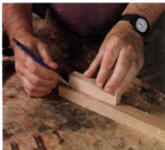
Lay out and install the hinges before glue-up. Use a piece of scrap the same thickness as the door to locate the door's rear edge on the stretcher.
