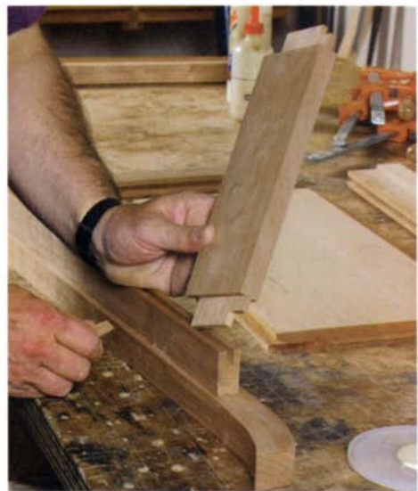
Attach the rails. Once the leg-and-stile assembly has dried, insert the bottom and top rails of the frame and panel.
