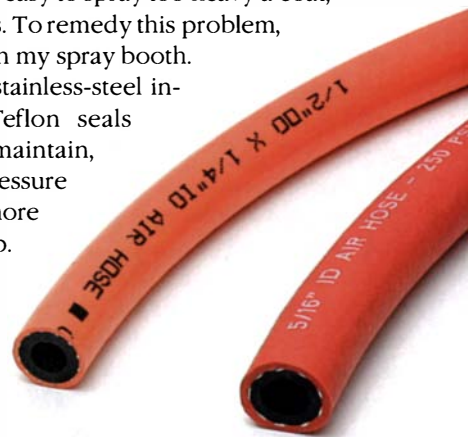
Hose sizes make a difference. LVLP spray equipment needs at least 5/16-in. inside diameter hose (right) to function properly. The 1/4-in. hose (left) cannot deliver sufficient air to prevent pressure drops in the system that will adversely affect the spray patterns.
