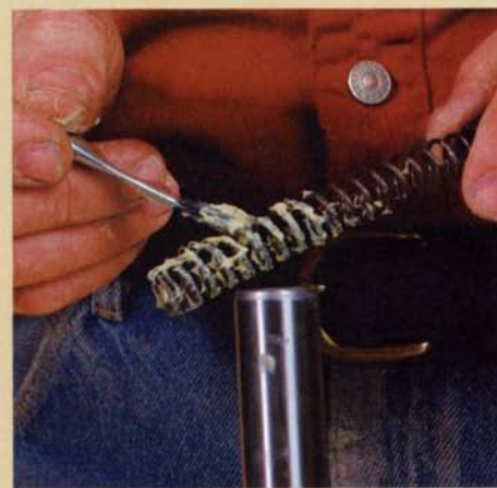
Brush on some grease. Give the springs a generous coating of lithium grease before re-installing them in the guideposts.
