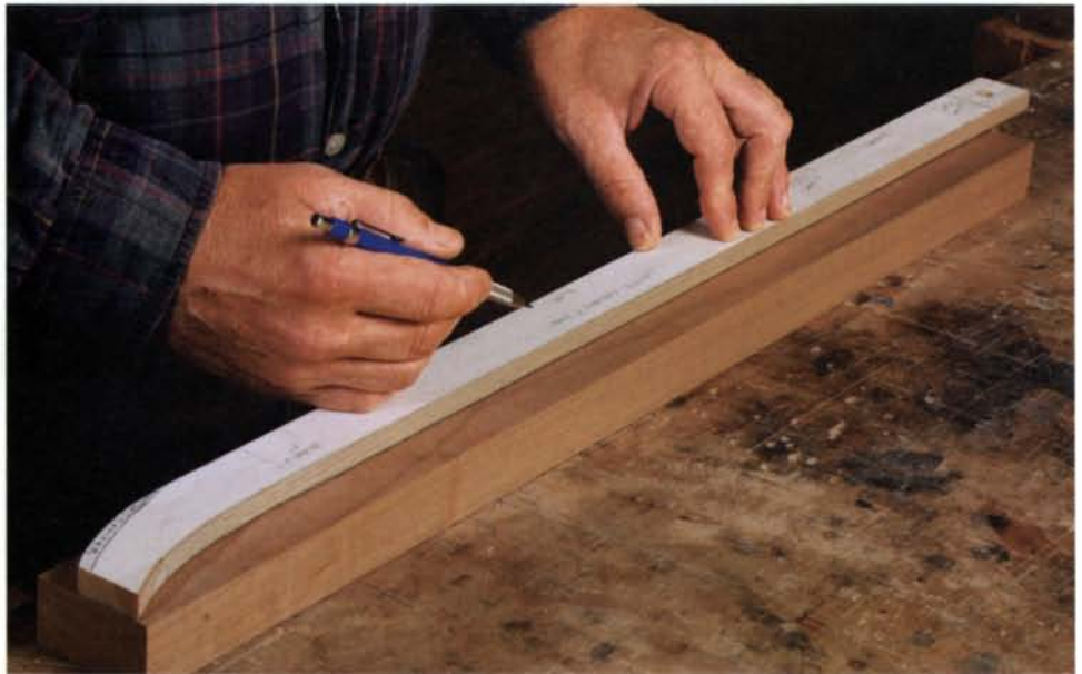
Story stick aids leg layout. To ensure consistent leg form, shape a single template to trace the layout of all four leg blanks. The same template can be used for marking out the mortises.
