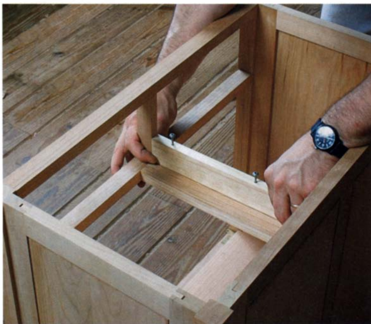
Not quite a sliding dovetail. The drawer divider is joined with a dovetail only half the thickness of the rail so that rail strength is not compromised.
