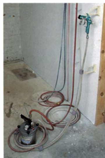
A separate pressure tank is ideal. This small pressurized fluid tank delivers the finish material to the gun effectively. Fatigue is reduced because the operator is spared the additional weight of a cup of finish, and the spray gun is easier to handle.
