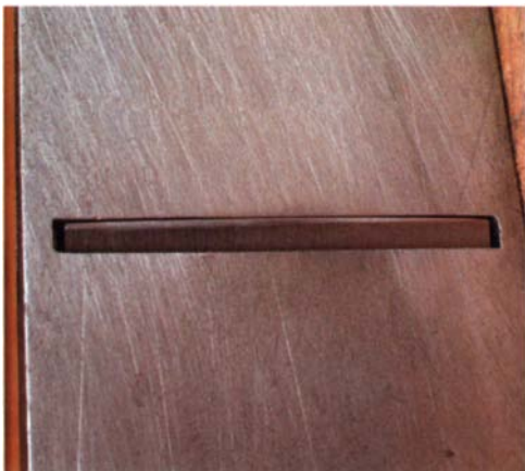
A slightly crowned plane blade won't dig in at the corners. Grind and hone a gentle curve across the entire width of the blade, with the corners about \frac{1}{4} in. back from the center.
