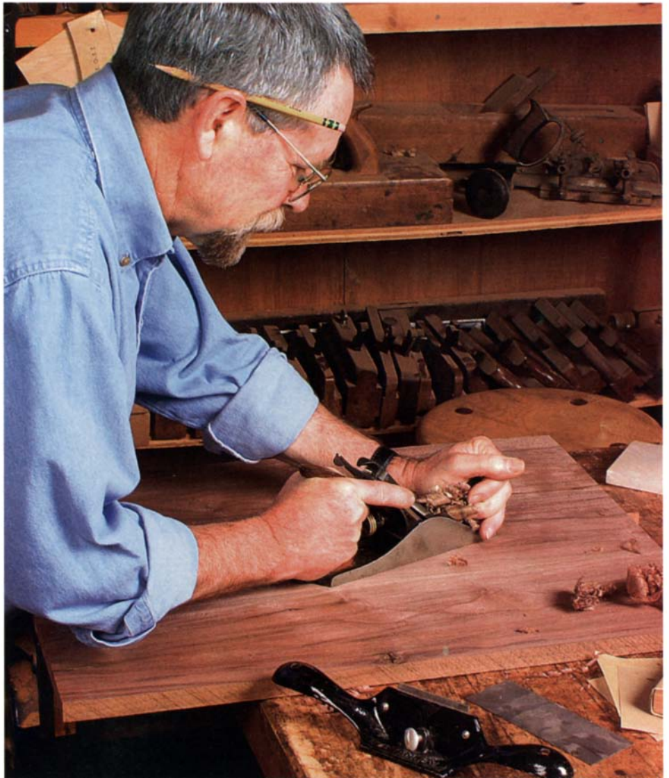
Handplaning is the most important step. A well-tuned smoothing plane will flatten the surface quickly and slice below the "compression layer" left by planer blades. To make the job easier, rub some paraffin on the sole and skew the plane slightly to create a shearing action.
