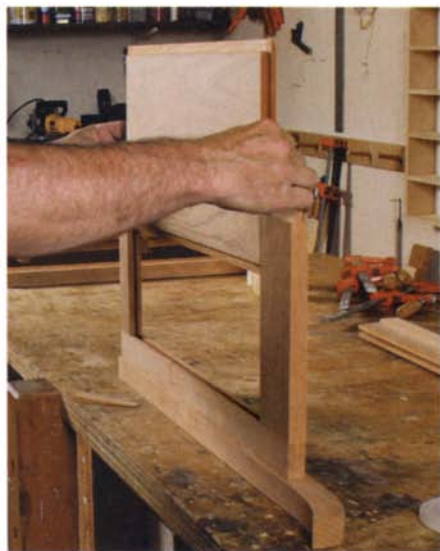
Drop the panel in place. Gibson prefinished the rabbets on the panel so that he wouldn't have to squeeze finish into the small gap between the frame and the panel.
