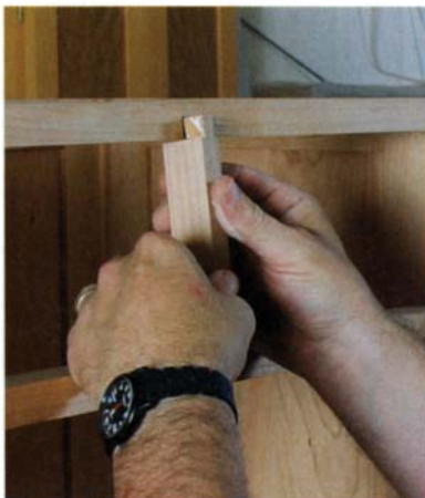
Not quite a sliding dovetail. The drawer divider is joined with a dovetail only half the thickness of the rail so that rail strength is not compromised.
