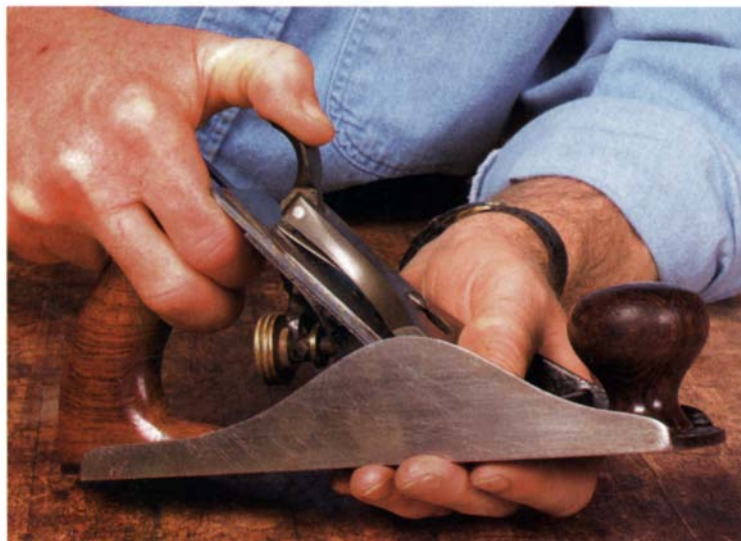
Handplaning is the most important step. A well-tuned smoothing plane will flatten the surface quickly and slice below the "compression layer" left by planer blades. To make the job easier, rub some paraffin on the sole and skew the plane slightly to create a shearing action.
