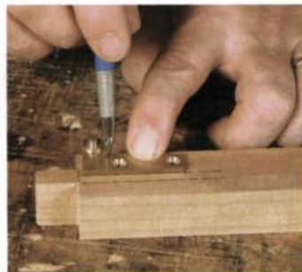
Use the hinge as a template to mark the mortise. The hinge should be centered in the door area of the stretcher (see the drawing above).
