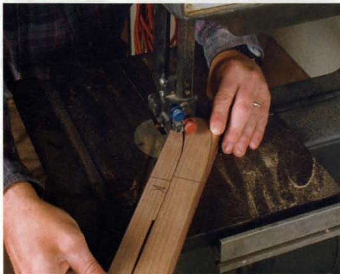
Finish on the bandsaw. Cutting from the bottom of the leg, finish the sweep of the foot on the bandsaw.
