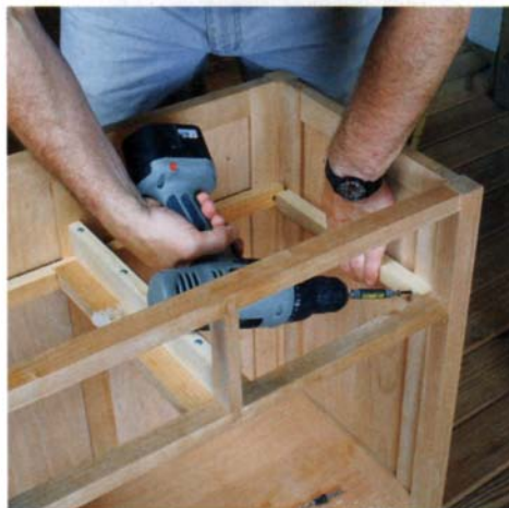
Runner fits flush with rail. Screwed in for strength, the runner lines up with the back guide and the front rail.
