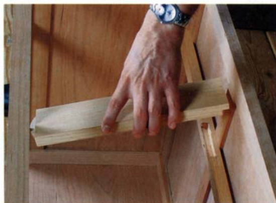
Fit the center runner. For ease of assembly, the back is rabbeted and drops into a notch in the ledger. The front is biscuited into place.
