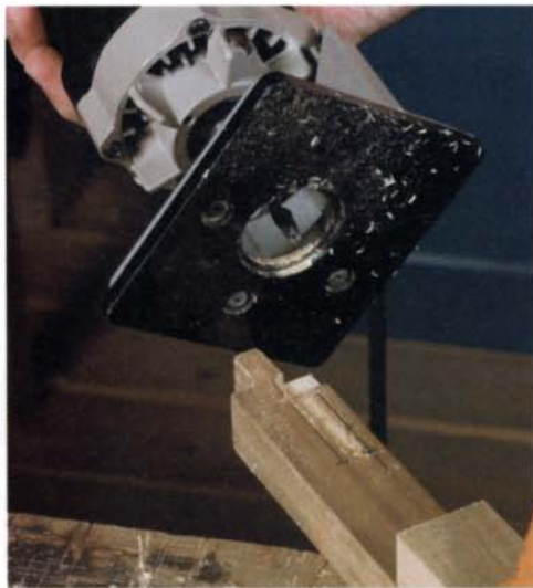
Lay out and install the hinges before glue-up. Use a piece of scrap the same thickness as the door to locate the door's rear edge on the stretcher.
