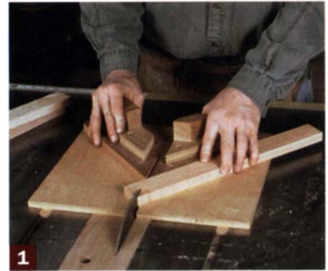
1 The first cut is made on the left-hand side of the jig. If the work slips, it will do so away from the blade.
