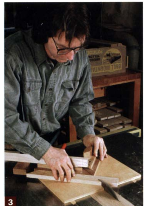
3 Make the second cut on the right-hand side of the jig. With the stop block in place, you are assured of consistent cuts.
