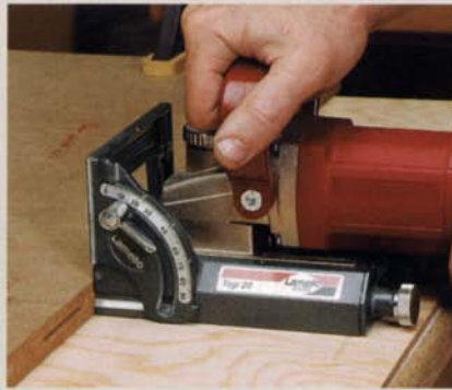
Testing for parallel. For the first test, the adjustable fence supports the joiner (left). The base of the joiner serves as the fence for the second test (right).
