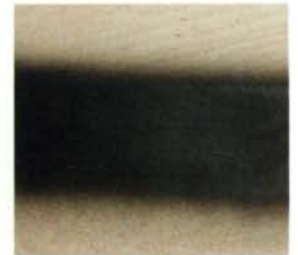
See how it runs. The top bar of black lacquer had fast-evaporating acetone added. The lower bar was thinned with slow-evaporating lacquer thinner, giving the finish time to run before it could dry.
