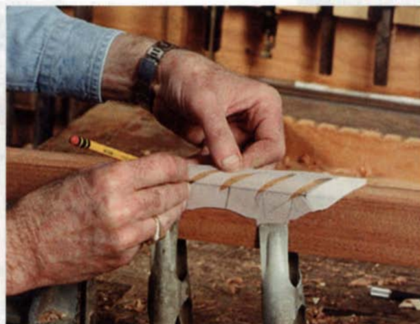
A template made of thin plastic or cardboard simplifies layout. The carving along each apron should begin and end with the same element.
