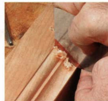
A custom scraper makes short work of tool marks. It would be very difficult to sand this profile, but the scraper smooths the surface and leaves crisp edges.
