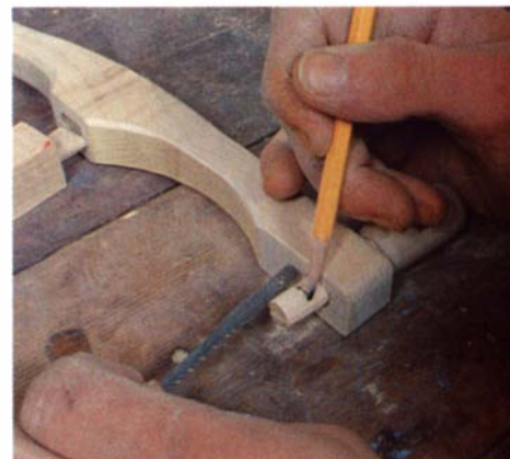
Mark the holes for the blade pins. Use the blade to determine the exact locations of the holes on the shanks.
