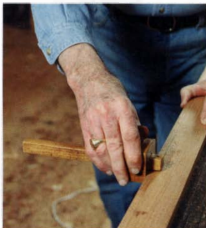
Scribe the carving stock \frac{1}{2} in. from the edge. Use straight-grained wood about \frac{1}{2} in. thick.
