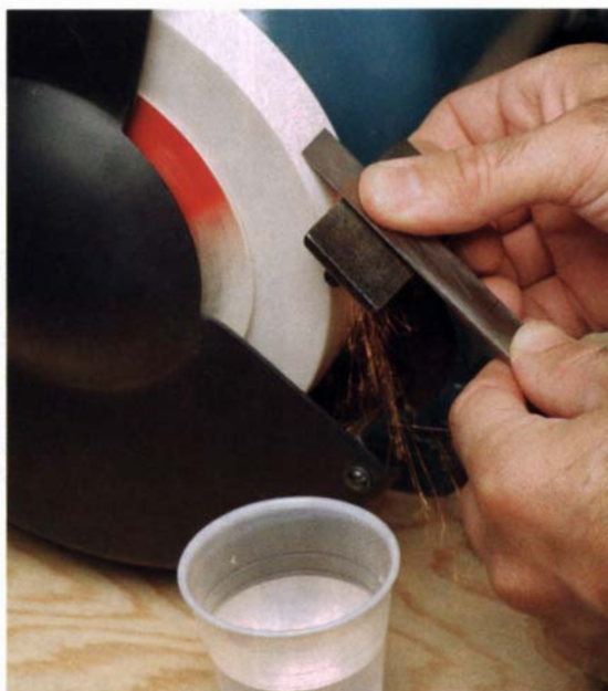
The key to grinding metal is to keep it from overheating. Use a light touch and pause often to dunk the tool in water. Aluminum-oxide wheels, usually white or pink, produce less heat than standard-grit gray Carborundum wheels. Slow-speed motors also help.
