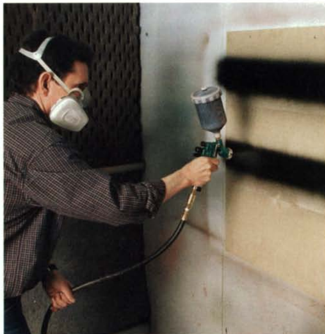
Adjust your lacquer for every occasion. When spraying a vertical surface, it is important that the finish dries before it has a chance to sag and run.
