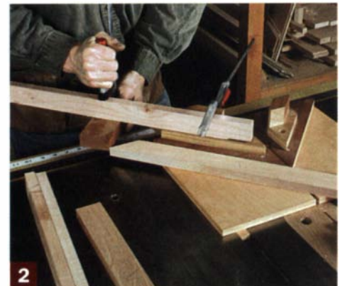
2 Uniform length. Mark the length on the workpiece and on the right-hand fence. Clamp a stop block against the mitered end.
