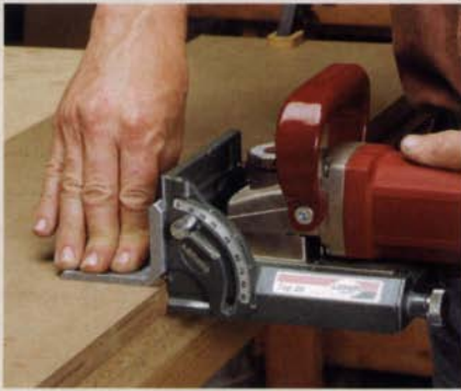
Testing for parallel. For the first test, the adjustable fence supports the joiner (left). The base of the joiner serves as the fence for the second test (right).
