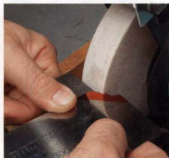
Grind close to the line. Set the tool rest perpendicular to the grinding wheel, and use the corner of the wheel to reach into concave areas of the profile.
