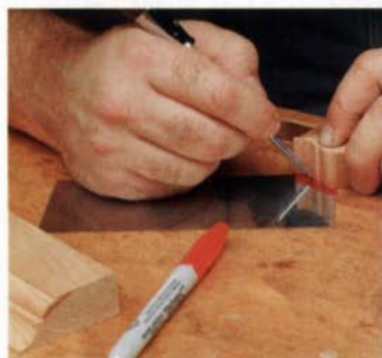
Lay out the profile. Paint the scraper stock with a permanent marker, then scribe around a cut-off of the molding. An awl will leave a sharp, precise line.
