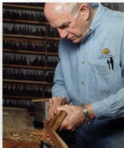
Radius the edge of the stock to the scribe line. Most of the carving is done along this radiused edge.
