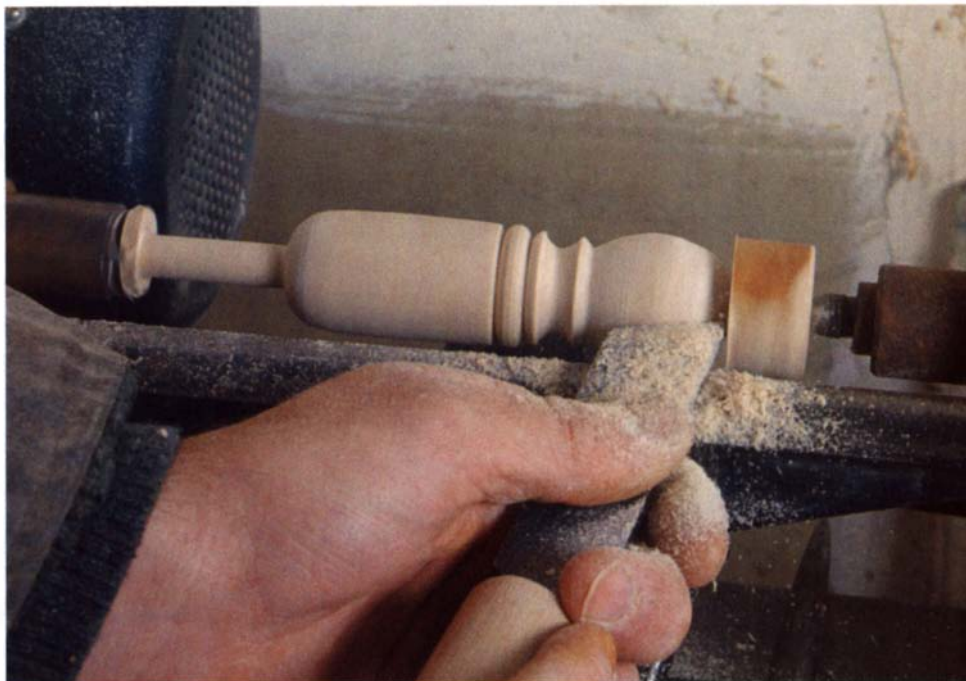
Shape it on the lathe. Once a blank for the handle has been mounted in the lathe, it takes just a few minutes to turn a profile that's both interesting and comfortable.
