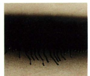
See how it runs. The top bar of black lacquer had fast-evaporating acetone added. The lower bar was thinned with slow-evaporating lacquer thinner, giving the finish time to run before it could dry.
