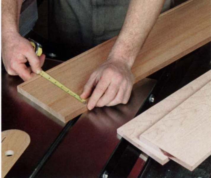
Each part determines the size of the next one. Lay out the groove in the drawer front directly from the bottom assembly. Then measure to the groove in the drawer front to determine the height of the drawer sides.
