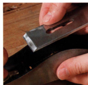
This side up. On a block-style plane, the bevel of the blade faces up.
