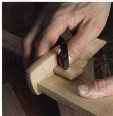
Shopmade marking gauge, p. 80
