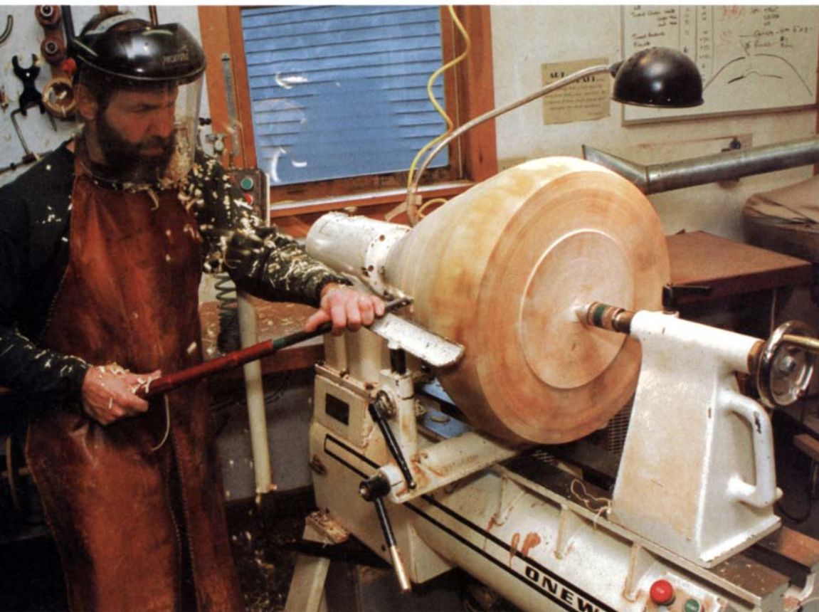
A large blank of aspen. The delicate lampshade begins as a blank of green aspen (left) weighing up to 200 lbs. Each finished piece has a unique pattern, but they all cast a soft, warm light.
