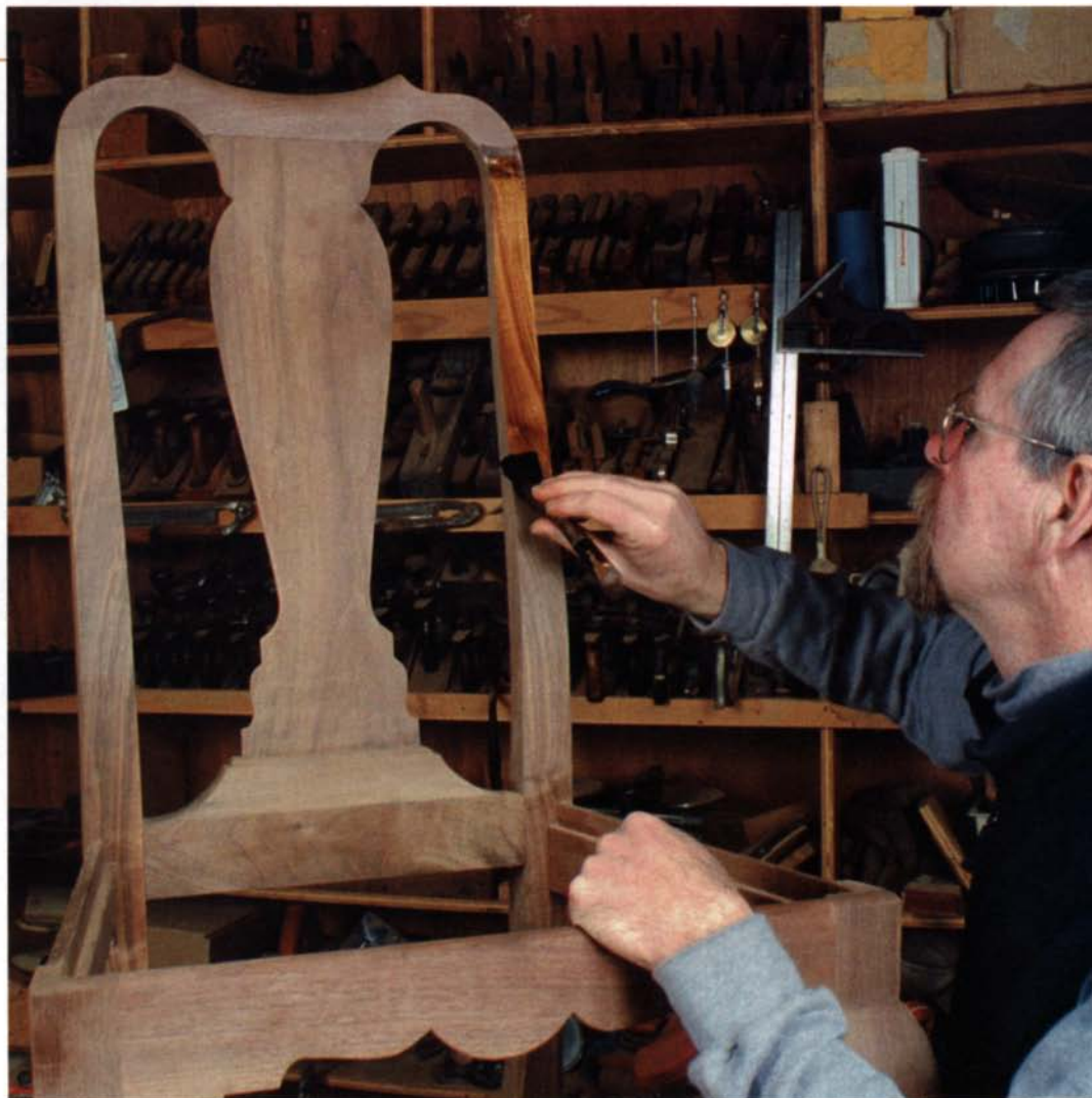
A shellac for every wood. The slightly greenish hue of buttonlac combines with the purple hue of walnut to yield a rich, brown color.
