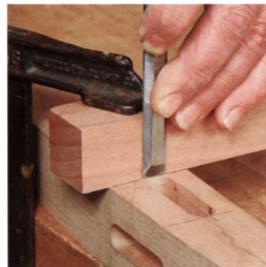
Squaring up mortises. When squaring up a machine-made mortise, a block of wood clamped to the workpiece can act as a guide.
