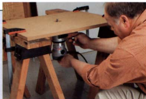
Router-table mock-up. To judge accessibility, each router was mounted to a piece of MDF clamped to a pair of sawhorses.
