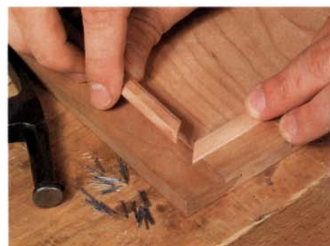
An applied molding holds in the panel. The thin strip, called a bolection molding, also hides the panel edge. A plywood panel, glued in place, is recommended for this door.
