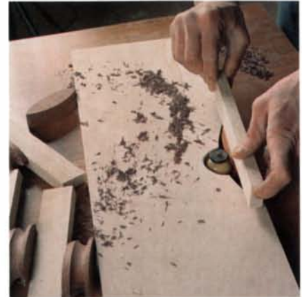
Keep fingers away from blades. A scrap of wood glued to the top of a pull blank keeps fingers above the spinning cove bit on the router table.
