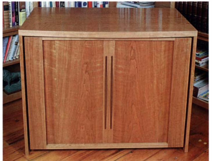
The finished cabinet appears to have solid-wood doors. The panels on both edges conceal the parting of the slats as the doors are opened.
