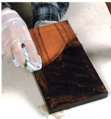
Wipe off the filler. With a clean cloth, wipe off the filler by moving across the grain. A cloth moistened with naphtha removes any dried excess glaze.
