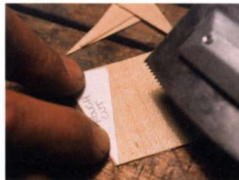
Rough cut. With a veneer saw and the single-segment template, cut out the segments and several extras.
