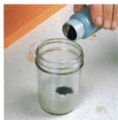
Apply the pore filler. The author adds dry pigment to a glaze to create a pore filler. Brush on the colored glaze generously to ensure that all of the pores are saturated.
