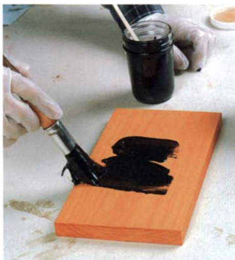
Apply the pore filler. The author adds dry pigment to a glaze to create a pore filler. Brush on the colored glaze generously to ensure that all of the pores are saturated.
