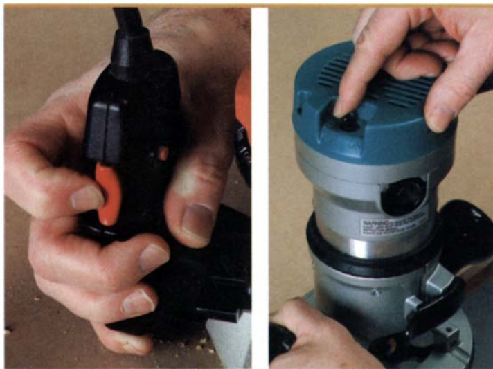
A trigger switch on the handle, like the one shown here on the Craftsman 17506 (left), is simple to use. Both of the Makita routers have the switch on top of the motor, so you have to let go of one of the handles to reach it.
