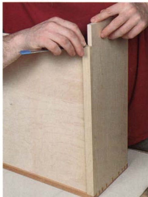
The drawer side is set in from the bottom runners and the sides of the drawer front (above). When laying out the half-blind pins, set a marking gauge about \frac{1}{16} in. heavier than the thickness of the drawer sides.
