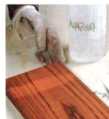
Wipe off the filler. With a clean cloth, wipe off the filler by moving across the grain. A cloth moistened with naphtha removes any dried excess glaze.
