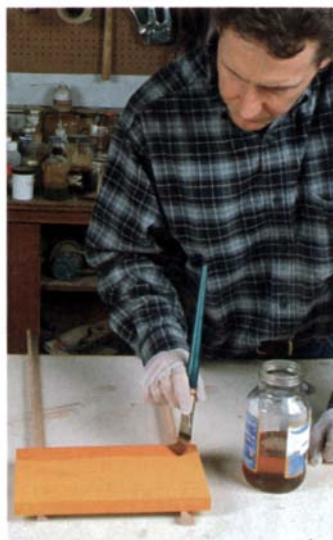
Seal in the dyed wood. The author uses a 1½-lb. cut of super-blond dewaxed shellac, but most clear finishes will work.
