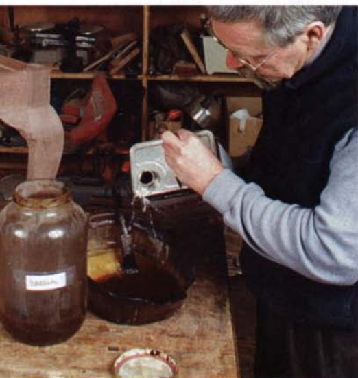
The first coat goes on thin. To allow for greater penetration of the first coat, Lowe thins the shellac with additional denatured alcohol.
