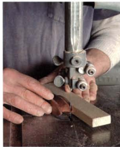
Curved shapes are softer. After routing, the scrap is cut away on the bandsaw and sanded to a curved shape. The author uses a balloon sander.
