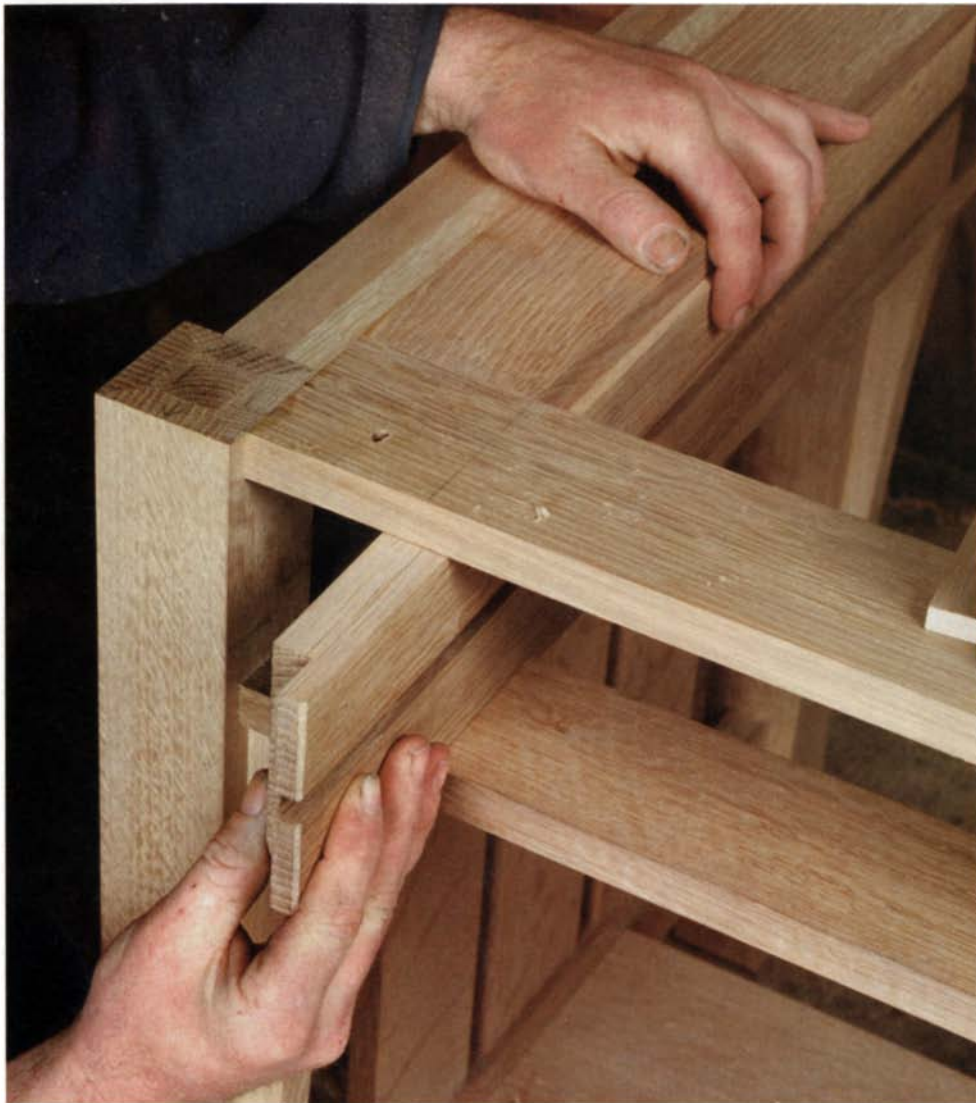
Block out the ends. The ends of the table are blocked out with a board grooved to accept the drawer glides.
