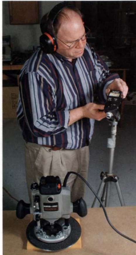
Noise test. To record the sound level of each router, a decibel meter was mounted in a tripod and placed in about the same height your ears would be if you were using the router.
