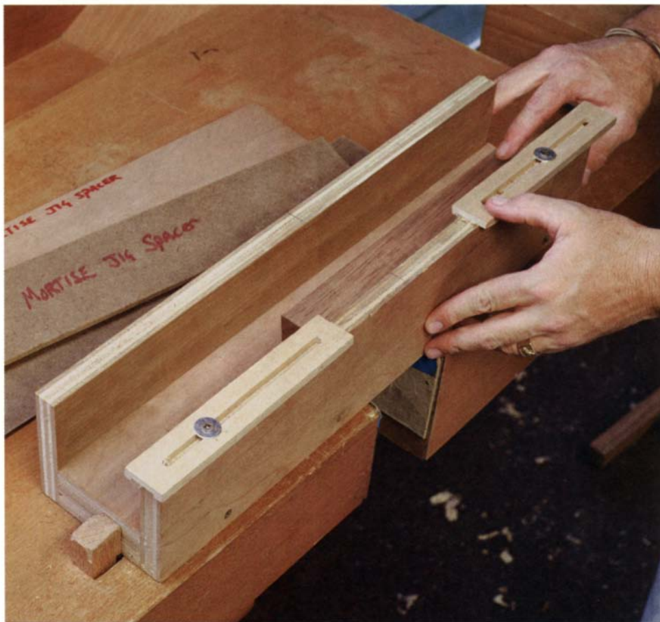
This jig has an important feature. Adjustable stops on this mortising jig limit the distance the router can travel and keep the length of all of the mortises consistent.
