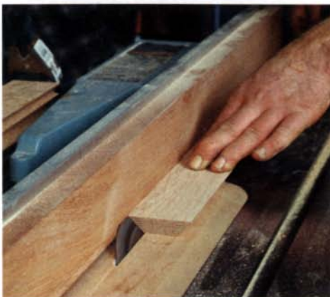
Four mitered pieces are required for each leg. Choose quartersawn stock with matching fleck patterns, then miter both edges.
