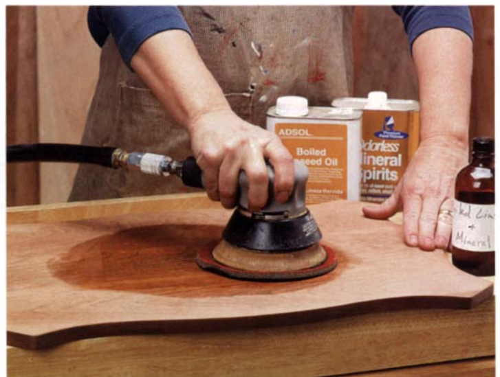
Fill the pores first. Sand the surface with a 500-grit Abralon pad lubricated with linseed oil and mineral spirits. The resulting slurry fills pores, burnishes the surface and adds depth.
