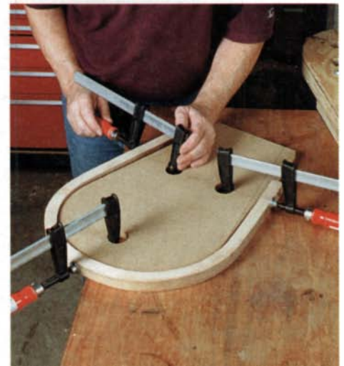
Cooling forms save space. Once the bend is complete, a cooling form, made of MDF, is a good way to store the piece for cooling overnight. Using cooling forms also enables you to bend other blanks almost immediately.
