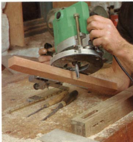
Rout the mortises. Using an edge guide on a plunge router, drop the bit a little at a time until you reach the desired depth.
