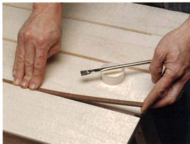
Add the inlay. Thin strips of cherry fill in the grooves, producing tight joint lines along the full length of the bench.
