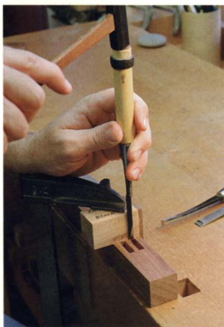
Help with the handwork. A thick block of wood clamped firmly to the workpiece serves as a guide to chisel the ends of the mortises true and square.
