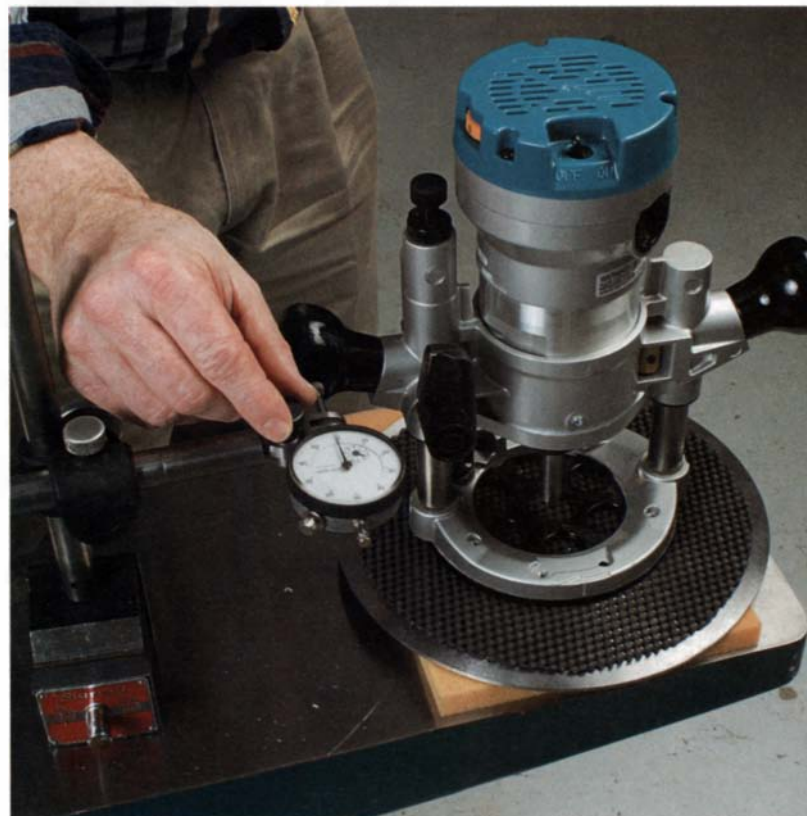
Good vibrations. With the router running, a dial indicator was used to measure the vibration at the handles.
