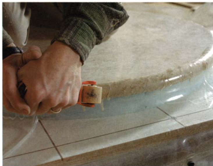
Start the vacuum pump, but shut it off when the veneer just starts to bend. Massage away the wrinkles along the top edge using a wallpaper roller. Run the pump a little more, stop it and roll over the wrinkles. Repeat as needed.
