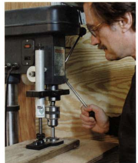
Yes, sir, it works. The Drill Sargent automatically exerts pressure upon the workpiece as the quill is lowered.
