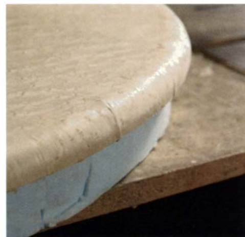
A few wrinkles are inevitable. They may be sanded away, leaving the edge smooth.
