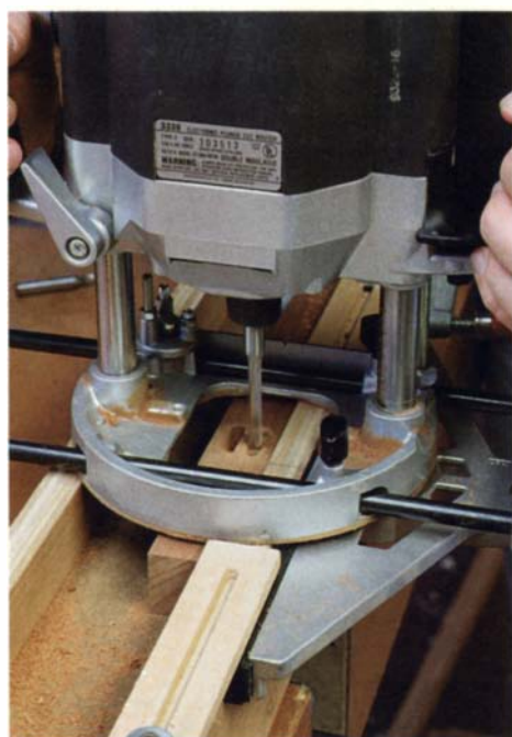
Steady as she goes. The router base sits firmly on the top of this jig as the router fence indexes the location of the mortise.
