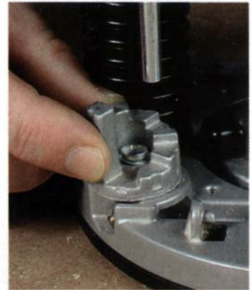
Stepped stops. The Bosch turret, with eight equally spaced steps, works with a minimum of fuss.
