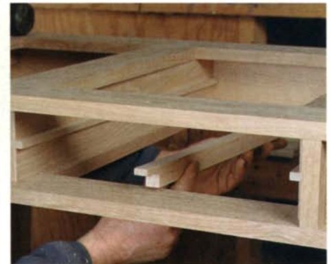
Insert the drawer glides and install the center glide. Glue the drawer glides in place and mount the center glide on the lower drawer frame. The center glide ensures that the drawer tracks correctly.
