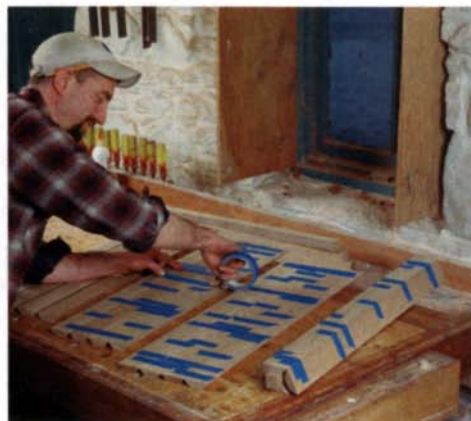
Strips of masking tape act as clamps. Set the mitered edges of the legs tightly against each other, then tape them together.
