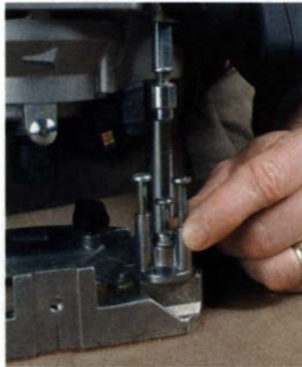
Three-step turret stop. The Festool has a turret stop with three adjustable steps.
