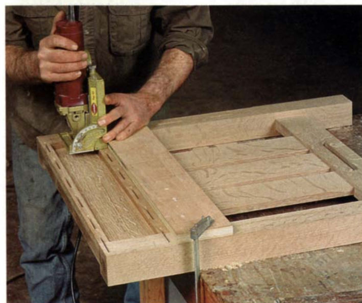
Assemble the ends. First fit the slats to the apron and lower rail, then set the assembly into the mortises on the legs.
