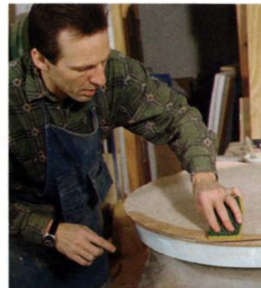
Place the workpiece on a piece of rigid foam. Dampen the veneer along the edge and slide the assembly into the vacuum bag.
