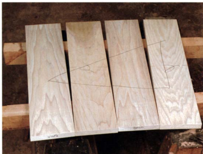
Panel boards are matched for appearance. A large triangle records the order and placement. When gluing up multiple panels, use different marks to distinguish them.
