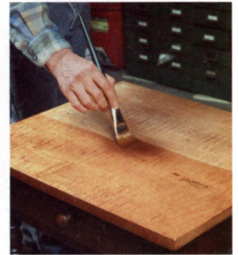
Fill fine scratches with more finish. Fix small scratches in lacquer and shellac by painting in the proper finish with a small artist's brush. Then lay on a coat over the entire surface.
