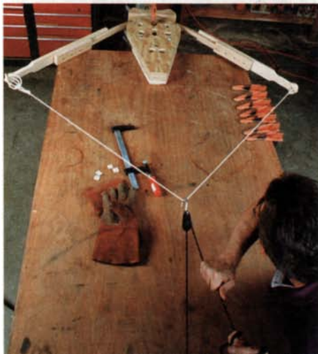
Pulley system lends a hand. Because the author typically works alone, he gains leverage by using a pulley system, made from an inexpensive block and tackle bought from the hardware store.
