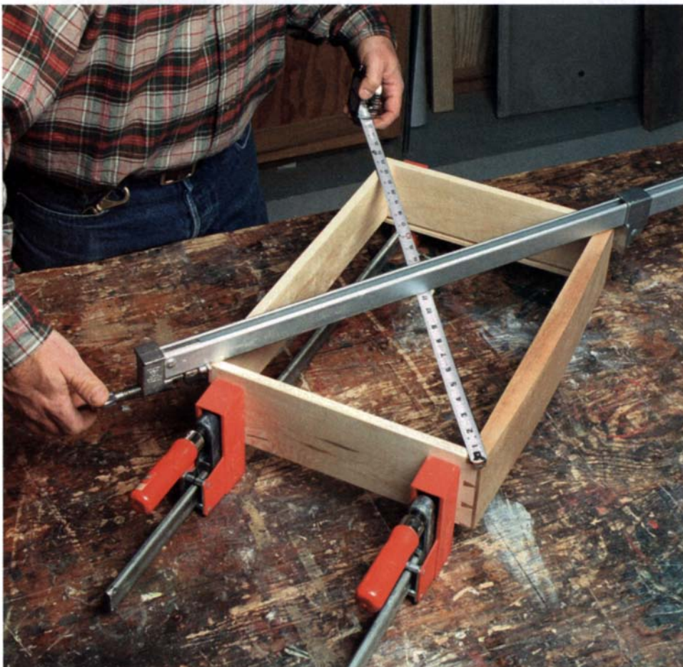
Be careful not to overcorrect a glue-up that measures out of square. The workpiece often continues to move for several minutes after clamping pressure is applied, carrying it beyond square in the other direction.
