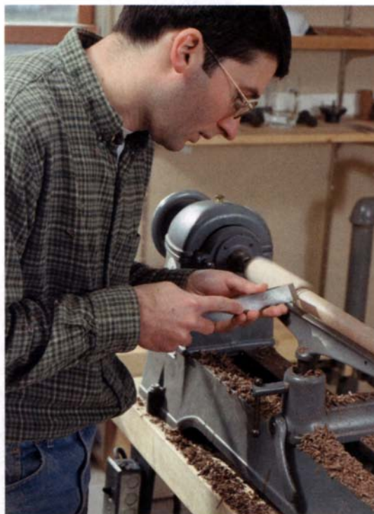
1. Make a series of grooves. Use the long point of the skew chisel to define the valleys between the beads.
