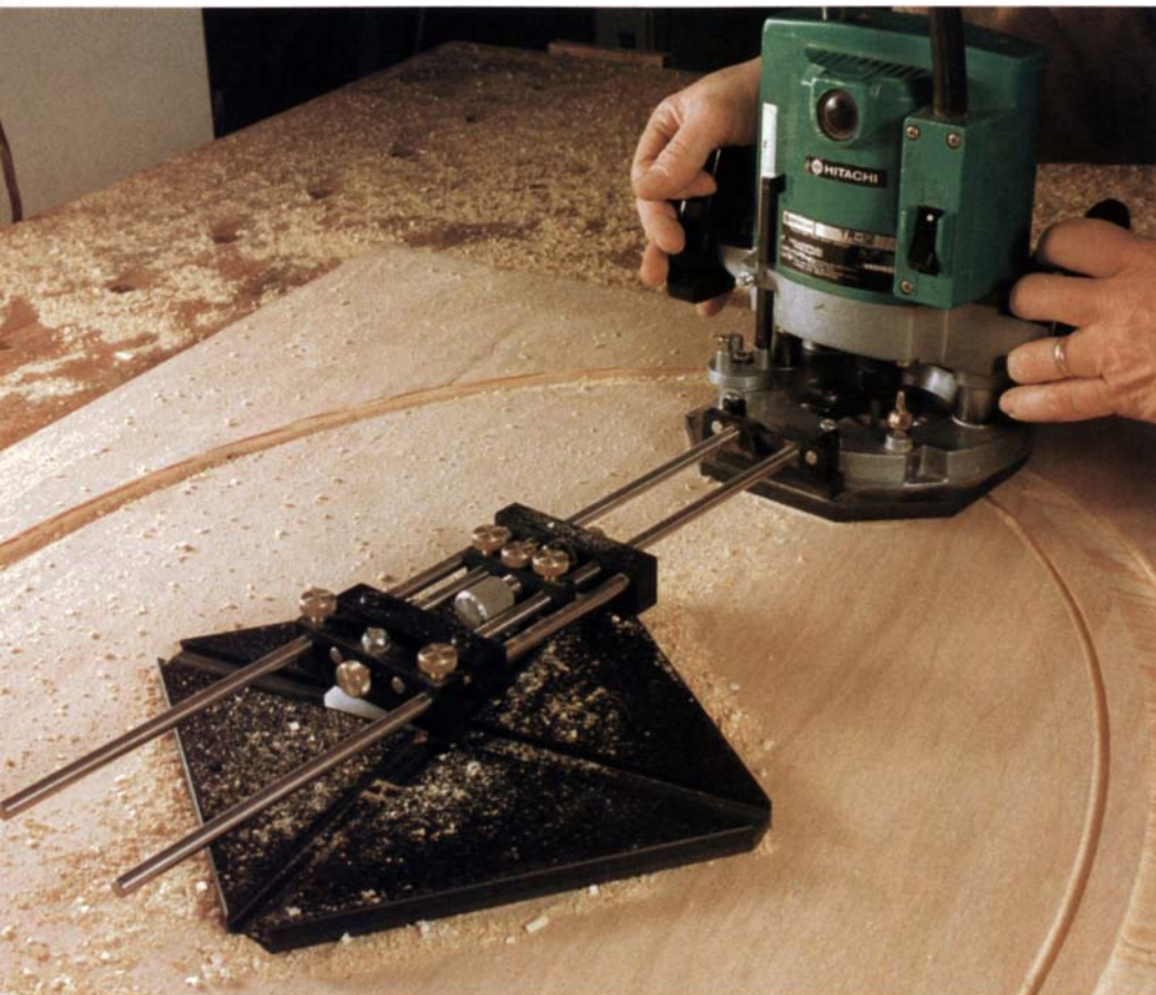
Perfect ellipse every time. The router pivots around an axis plate, cutting a perfect ellipse.
