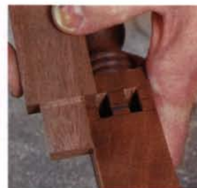
Check the fit by holding the rail against a leg. The edge of the rail should meet the edge of the mortise.
