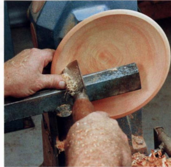
Scrapers refine turned surfaces, p. 56
