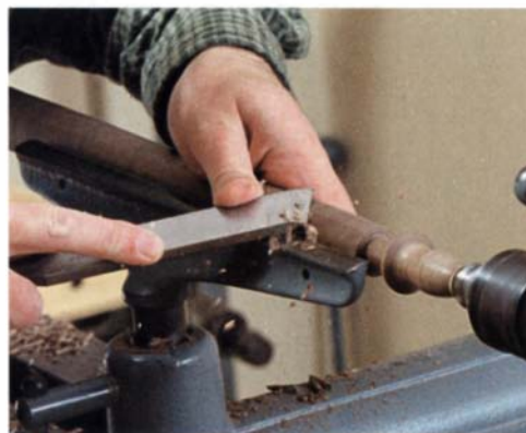
1. Shape the valley of the foot beginning with a gouge. Then switch to a skew chisel to make the soft convex curve.
