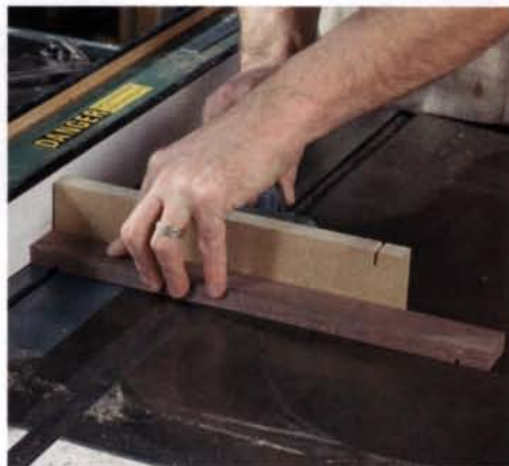
Crank up the blade to \frac{1}{8} in. Score the bottom face and front and back edges of the upper rail.
