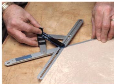
Set. As the outside legs of the Multifix are adjusted to match the desired angle, the center leg automatically slides to the miter angle.
