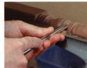
3. All cove cuts are made using a narrow gouge. Cut into the valley from both sides to avoid catches.
