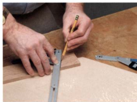
Scribe. With the outside legs separated, use the center leg to scribe the miter angle directly to the workpiece.
