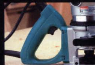
D-handle models have a locking trigger switch for operator control and comfort
