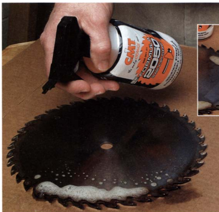
Spray and wipe. Resins and gums loosen a few minutes after Formula 2050 is applied. The dissolved residue simply wipes off.
