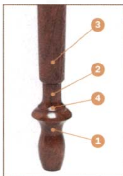
1. Make a series of grooves. Use the long point of the skew chisel to define the valleys between the beads.
