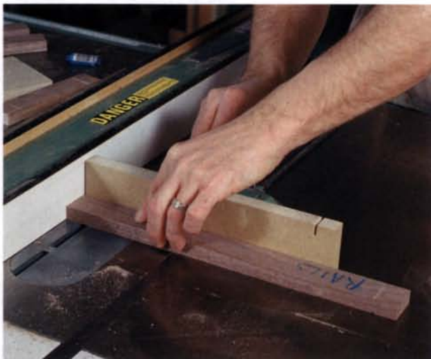
For the first cut, raise the blade just a hair. Make the first cut on the top and bottom faces of the lower rail, just scoring the stock.
