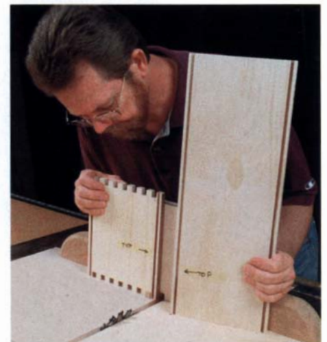
Box joints on the tablesaw, p. 60
