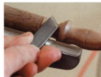
4. Define the collar at the base of the cuff using the corner of a skew. Fine details such as this should be consistent from leg to leg.
