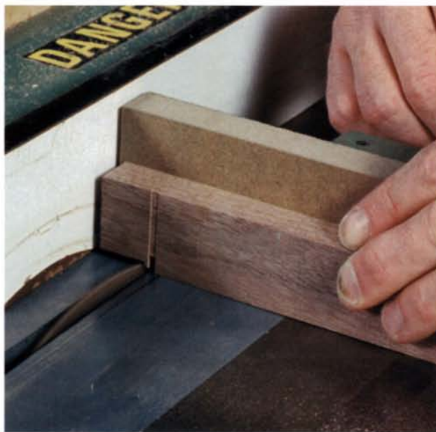
Raise the blade to almost \frac{1}{4} in. Cut the front and back edges of the lower rail, then nibble away at the edges.
