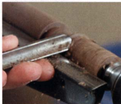
1. Shape the valley of the foot beginning with a gouge. Then switch to a skew chisel to make the soft convex curve.
