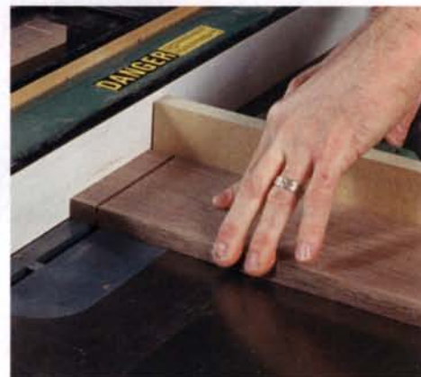
Raise the blade to \frac{3}{8} in. Cut the shoulders on the faces of all the aprons. The stock left between the kerfs should be \frac{1}{4} in. thick.
