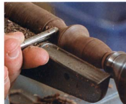
2. Work on the cuff, which is mostly straight. Both the flat and concave sections are cut using a gouge.
