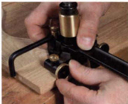
Machine-screw fence. A pair of knurled, brass machine screws serves as the fence.
