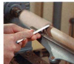
2. Roll the uppermost bead first. It is the most difficult to turn because of the sharp corner. Then turn the others.
