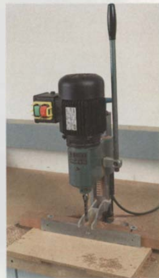
Multico brought us the benchtop hollow-chisel mortiser. Before Multico, these machines were large and heavy. Now there are many sizes and brands from which to choose.
