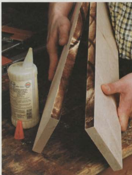
Burned wood makes a poor glue joint. Remove the charred surface before glue-up.
