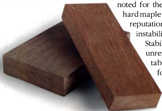
Dimensional stability. Walnut and mahogany are known for their dimensional stability, a very desirable property.
