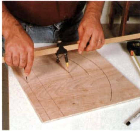
Scribe the arcs. Establish the upper and lower edges of the cutout by scribing the arcs with a compass.
