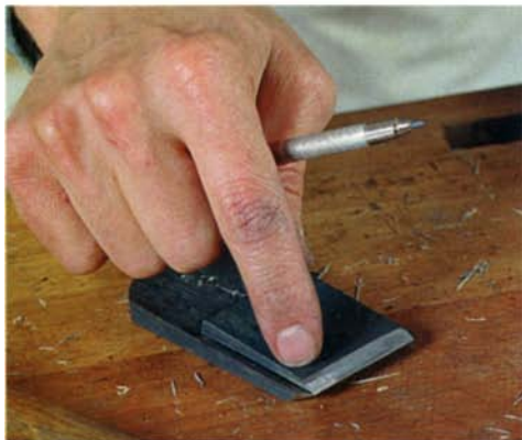
Check that the chipbreaker is flat. Position the chipbreaker over the iron and tap on the corners to see whether it rocks.
