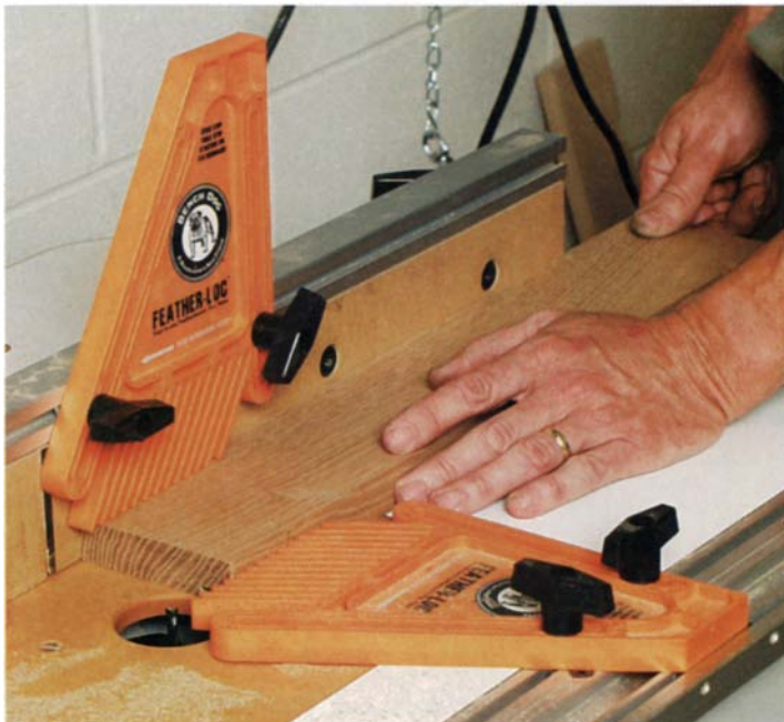
Bench Dog featherboards are quick and easy to set up. They can be used horizontally or vertically; they also work as stops.
