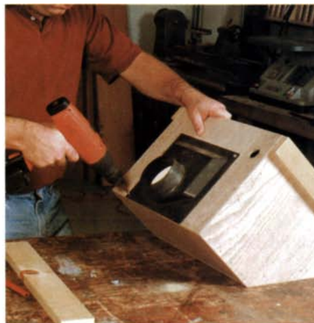
The dust port goes on back. A plastic dust port provides an easily accessible attachment point for the dust-collector hose.
