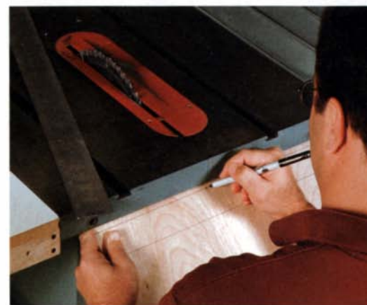
Transfer the mark. Slip the back plate under the top of the saw to transfer the center point of the arc from the saw to the plate.
