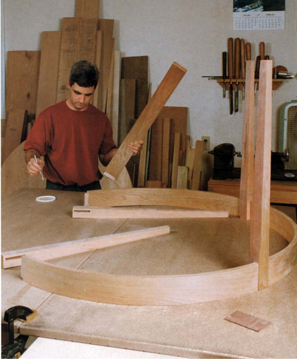
Gluing up the base assembly. Use a flat, level surface to lay out and glue up the legs to the aprons. Any misalignments need to be adjusted before tightening the band clamps.
