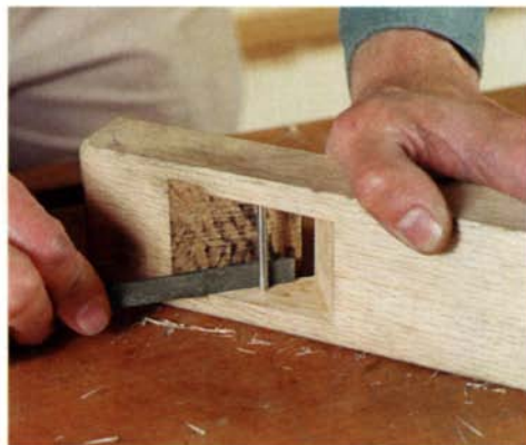
Hammering the chipbreaker may not be enough. The metal retaining pin may have to be filed down until the chipbreaker fits.
