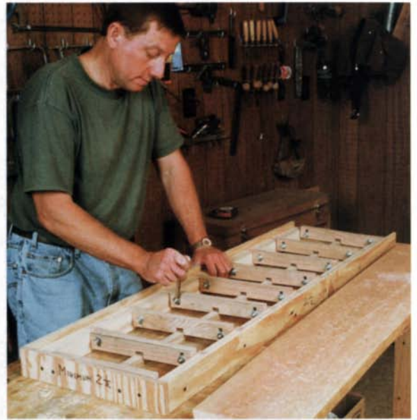
Remove the board temporarily. And tighten down all of the bolts.
