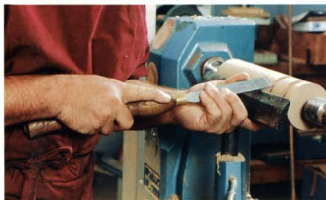
Underhand grip. The forward hand grips the shank from underneath, with the forefinger hooked under the tool rest.
