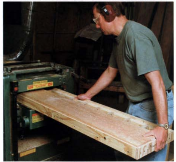
The entire sled goes through the planer. Multiple passes will probably be necessary to produce a flat side.
