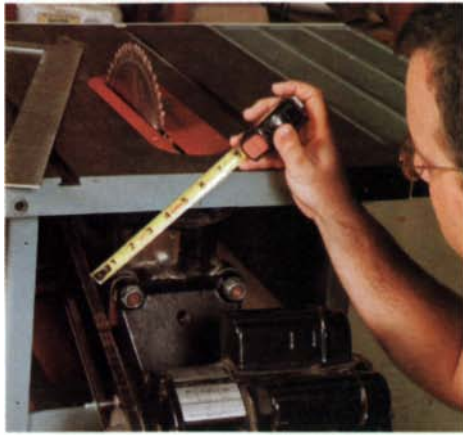
Measure the belt in the raised position. Take the first measurement with the sawblade in its highest position.
