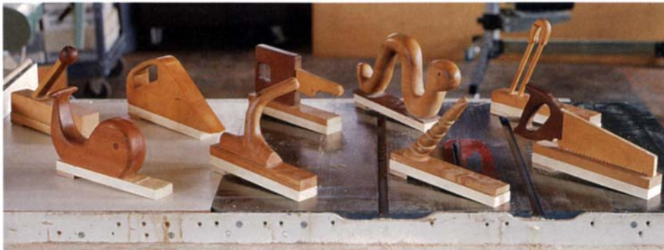
Pick a push stick. All of these student-designed push sticks vary in artistic style but share the functional characteristic of having a disposable sole and heel held on with hot-melt glue.
