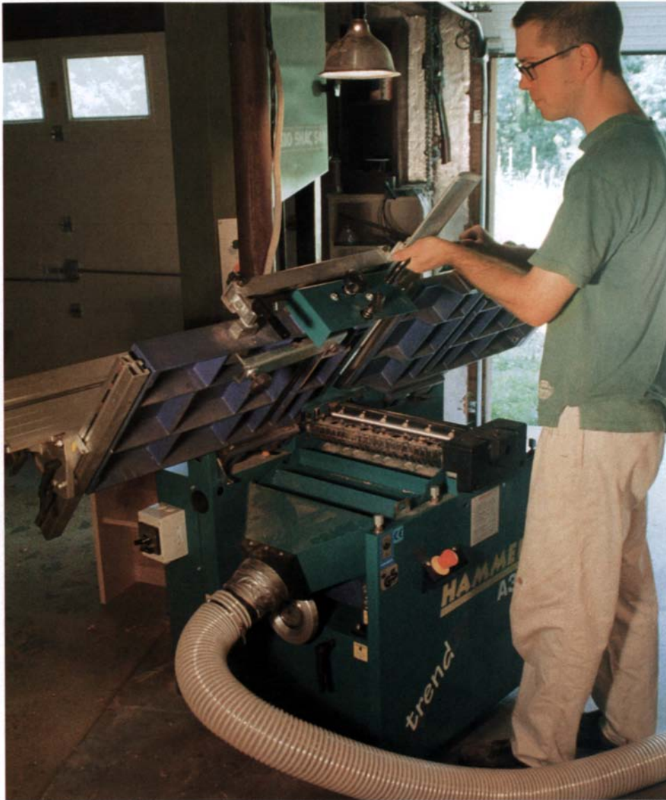
Switching from planing to jointing takes only a couple of minutes. In planing mode, the jointer tables are swung up and out of the way.
