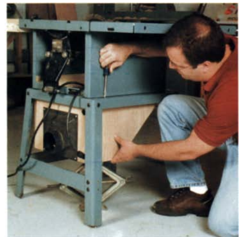
Jack it up. An old scissors jack holds the dust box in place when driving home the sheet-metal screws.
