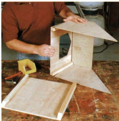
No fancy joinery required. The author uses ring-shank nails to join the dust-box parts.
