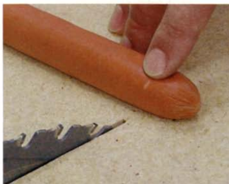
SawStop could save your finger. The SawStop senses when flesh touches the blade and, within milliseconds, stops the rotation.
