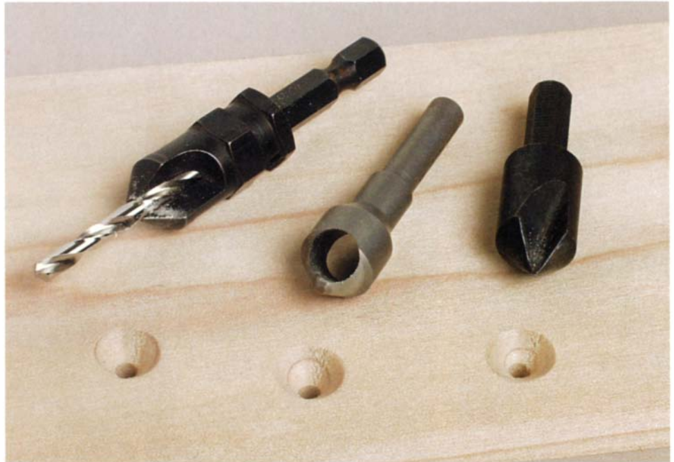
Accurate countersinking in wood. The first rule is to use a bit that is designed for wood. Avoid multilipped countersinks. The combination drill/countersink at left will guarantee a countersink that is concentric with the hole. The Weldon-style countersink (center) and single-lipped type also work well in wood, but the workpiece should be clamped to a drill-press table so it won't shift between drilling and countersinking operations.
