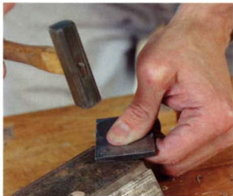
Flatten (or roll over) the corners of the iron to correct for rocking. Use the same hammer and anvil used for bending the iron.
