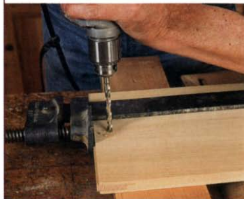
Clamp down the cleats into their grooves, and drill for their retaining pins. A contrasting wood is used here for the pins, but the pins could be disguised by choosing the same wood used in the door.
