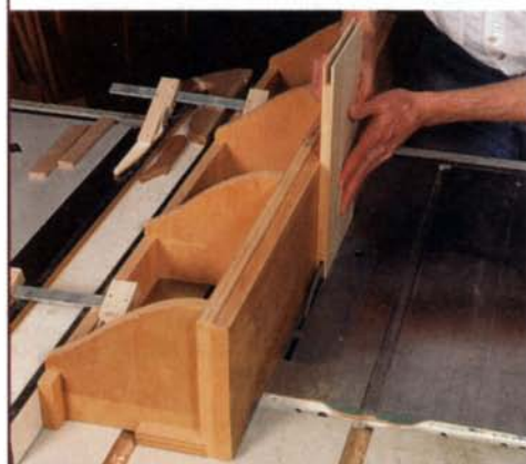
Cutting the grooves. An auxiliary fence is taller and gives additional support.
