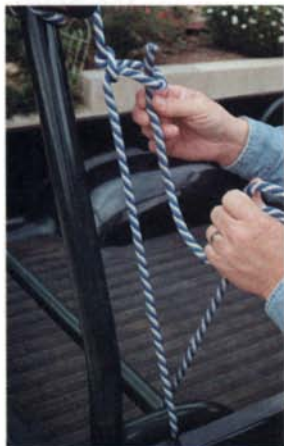
3. Bring the end down under a hook or bar on the truck and back up through the loop of the slipknot.
