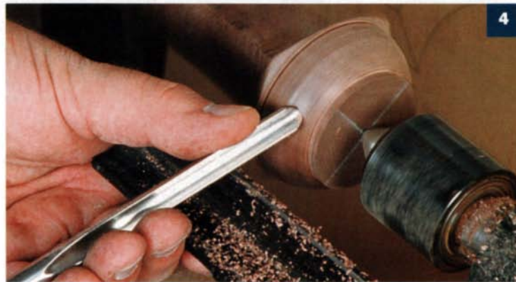
4. Round from the bottom up. Working up from the bottom of the pad, use a gouge to ease the transition from the top.
