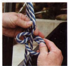
6. Then grab another loop of the loose end and tie a half hitch. This locks the tie-down. Because you made the half hitch with a loop, you can untie it simply by tugging on the end.
