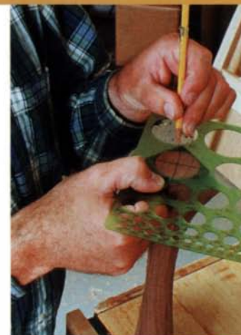
Templates help lay out the pad. Use a circle template to position the circle at the bottom of the pad.
