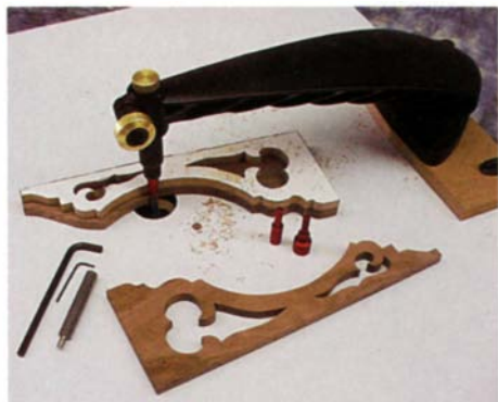
Turn a router table into an inverted pin router. The Veritas pin-router arm is perfect for intricate template work.
