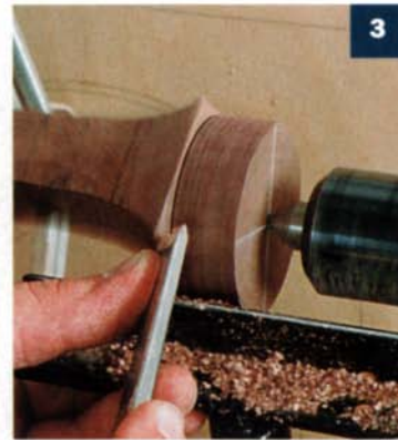
2. Forming the pad. A gouge rounds the pad at its widest dimension. Check frequently with calipers until you reach final width.
