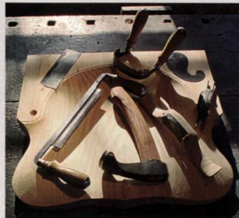
The tools in question. You don't have to spend a fortune on tools to get started. Clockwise from top center are inshave, goose-neck scraper, two bottoming shaves, gutter adze, drawknife and card scraper.
