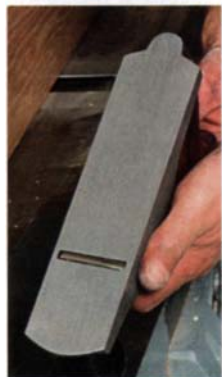
Truing a plane. To flatten a plane's sole, the author glues aluminum-oxide sandpaper onto the bed of his jointer (top), then works the plane back and forth until the scratches cover the entire sole (bottom).
