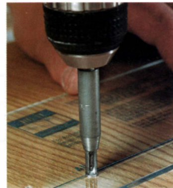
Pilot holes should be centered. Self-centering bits guarantee accurate placement.
