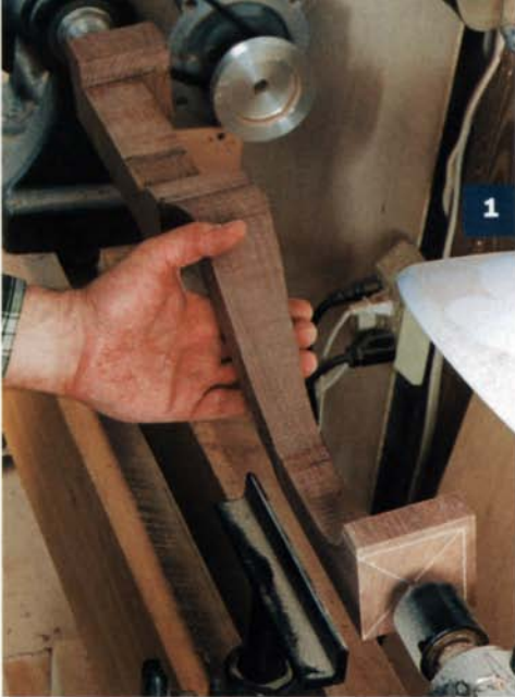
1. Blank is mounted off-center. Position the leg in the lathe using the pad centers you drew out earlier.
