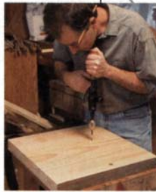
Quick depth gauge. Two holes drilled 1 in. deep provide the main points of reference for carving out the seat.
