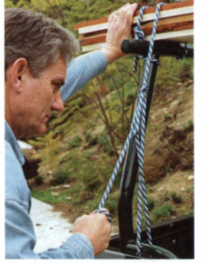
4. Then pull down hard. Try to move the lumber sideways; if it moves, pull harder on the rope.
