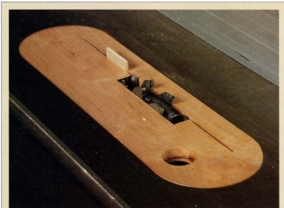
Safer dadoing. The riving knife, or fin, is set into a wooden throat plate and is located even with the right side of the dado cut, just lower than the blade height. The riving knife should contact the shoulder of the dado cut that is closest to the rip fence, preventing the workpiece from rotating away from the fence and kicking back.
