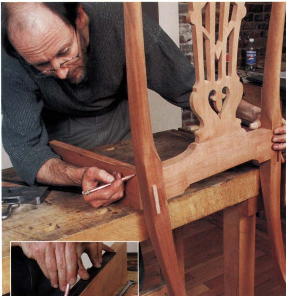
Establish layout lines. Connect the bottom line of the wind with the bottom front corner of the rail. Planing to this line gives you an even wind and lets the rail meet flush at both the front and back legs.
