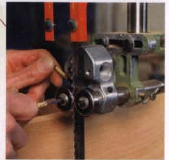
Fine-tuning. Raise the upper guides to cutting height before setting the bearings. The roller bearings should be set just aft of the blade's gullets.
