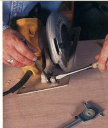
Parallel base and blade. Use a dial indicator to check that the blade is parallel to the edge of the saw base. Adjust the base to correct any error.
