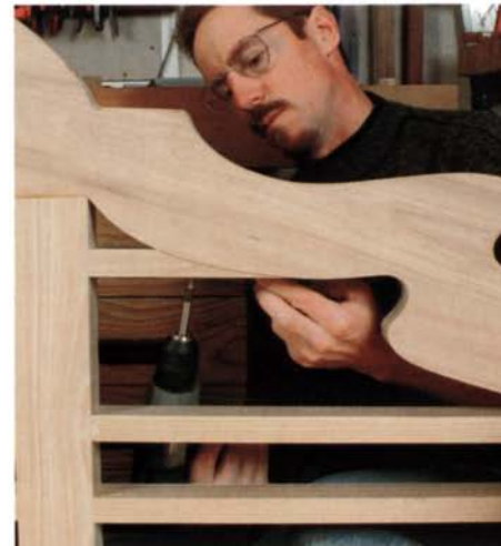
Scribing the back slats. The upper slats on the back are scribed for a tight fit. A bandsaw is used to cut them to shape, but final shaping is done with rasps and sanding machines. The shaped ends of the slats are screwed into place from underneath.
