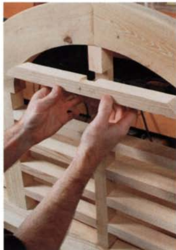
A smooth fit. Using a dado set on the tablesaw, the two top slats are notched to fit over the center stile.
