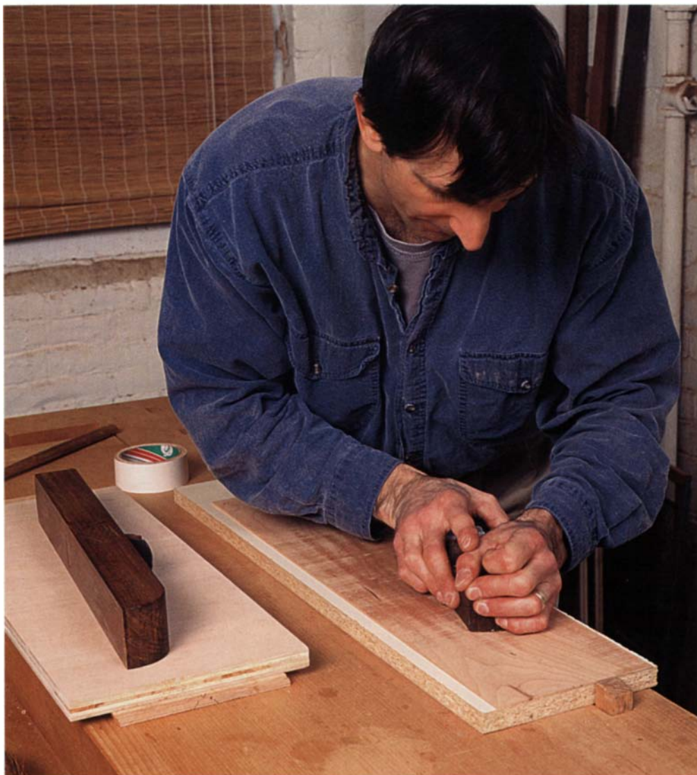
Smoothing after sawing. Double-stick tape keeps a sheet of veneer still for a quick smoothing with handplanes. At \frac{1}{16} in. thick, the veneer can be planed and worked like solid wood.
