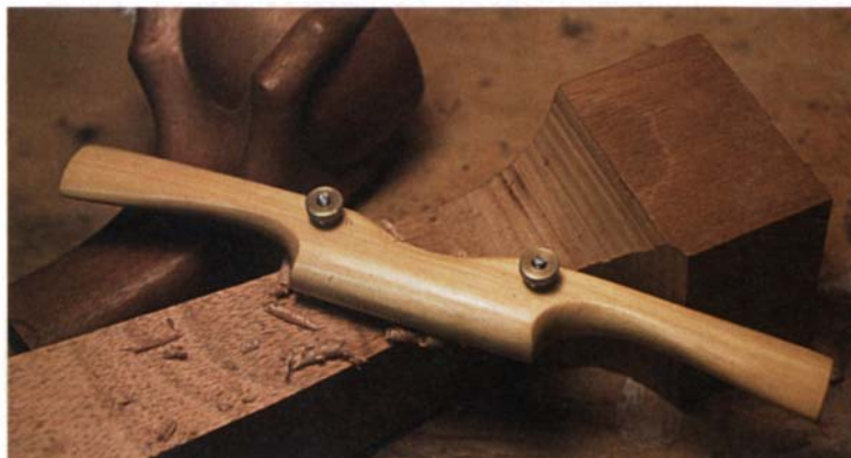
Classic wooden spokeshave. Dave's Shaves have their blades angled at 25°, which helps prevent chattering.
