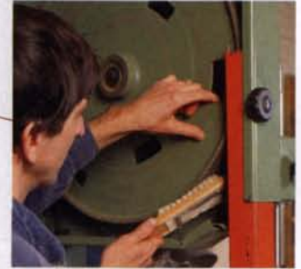
Keep it clean. For best tracking, brush the bandsaw's tires regularly and start a veneer-cutting job with a fresh blade.
