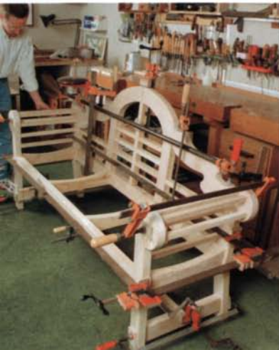
Finishing the back. After the main components of the bench have been glued up, the smaller slats can be set into place.
