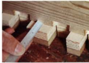
Mark the offset on the tails template. A backer board is attached at the mark (see the chart on the facing page).
