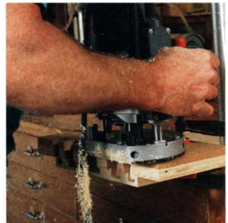
The pins stock is clamped facedown to the template. Rout the pins from above using a router bit with a bearing and stop collar.
