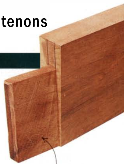
A compound-angle tenon is the best way to join a side seat rail to a chair's back leg.
