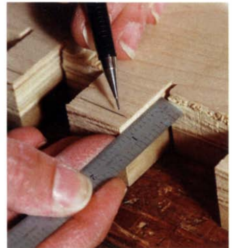
Use a ruler to mark the offset. The pins offset will depend on the thickness of the stock used (see the chart below).
