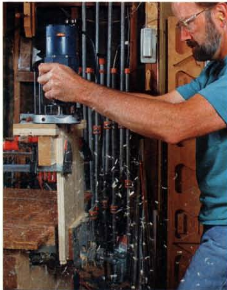
The tails are routed with the stock clamped vertically. The backer board positions the stock and prevents tearout.
