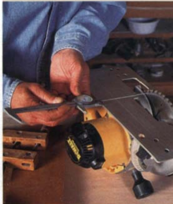
Parallel base and blade. Use a dial indicator to check that the blade is parallel to the edge of the saw base. Adjust the base to correct any error.
