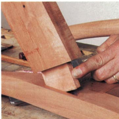
Take it slow. The author uses a shoulder plane to trim the cheeks, checking the tenon frequently against the mortise until he has a tight fit. He then trims to the layout lines with a shoulder plane.
