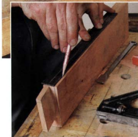
Establish layout lines. Connect the bottom line of the wind with the bottom front corner of the rail. Planing to this line gives you an even wind and lets the rail meet flush at both the front and back legs.
