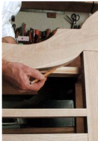
Scribing the back slats. The upper slats on the back are scribed for a tight fit. A bandsaw is used to cut them to shape, but final shaping is done with rasps and sanding machines. The shaped ends of the slats are screwed into place from underneath.
