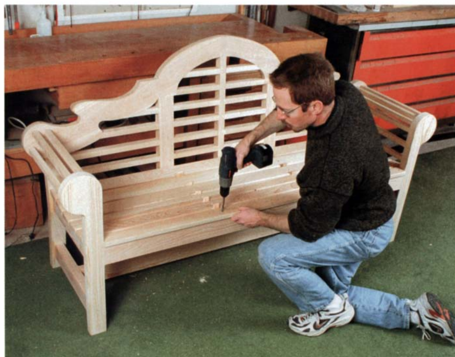
The last touch. Working from the back toward the front, the author uses spacers and screws down the seat. Once in place, bungs are epoxied into place over the countersunk screws.
