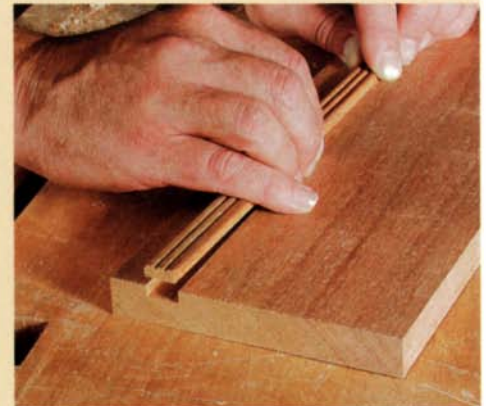
Set the beading in place. The beaded stock is glued into a groove ripped on the drawer front.
