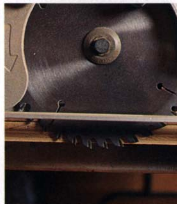
Don't worry about what's below. Set the depth of cut so that a full tooth of the blade extends below the workpiece. You'll be cutting right into the surface of the sacrificial table.
