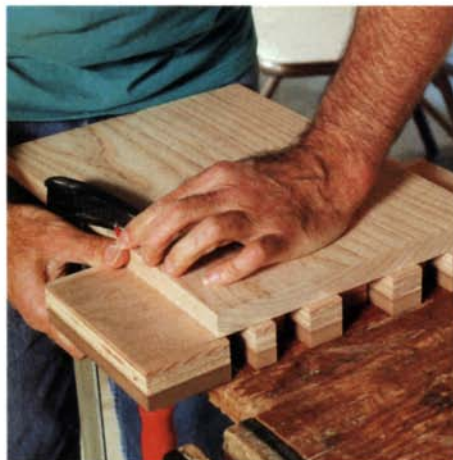
The pins stock is clamped facedown to the template. Rout the pins from above using a router bit with a bearing and stop collar.
