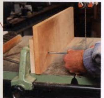
High fence provides full support. The auxiliary fence should be at least as high as the veneer will be wide.
