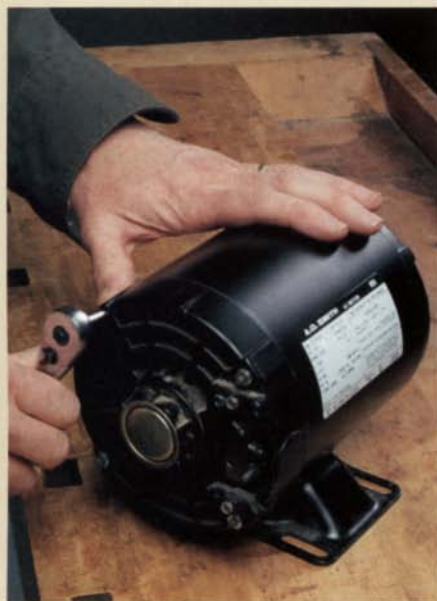
Open up. The end plate is removed to access the centrifugal switch.
