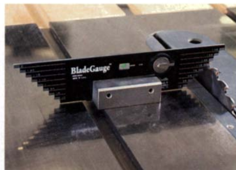
BladeGauge uses simple electronics to indicate blade height. When the blade touches one of the contacts, placed at ⅛-in. increments, an LED lights up.
