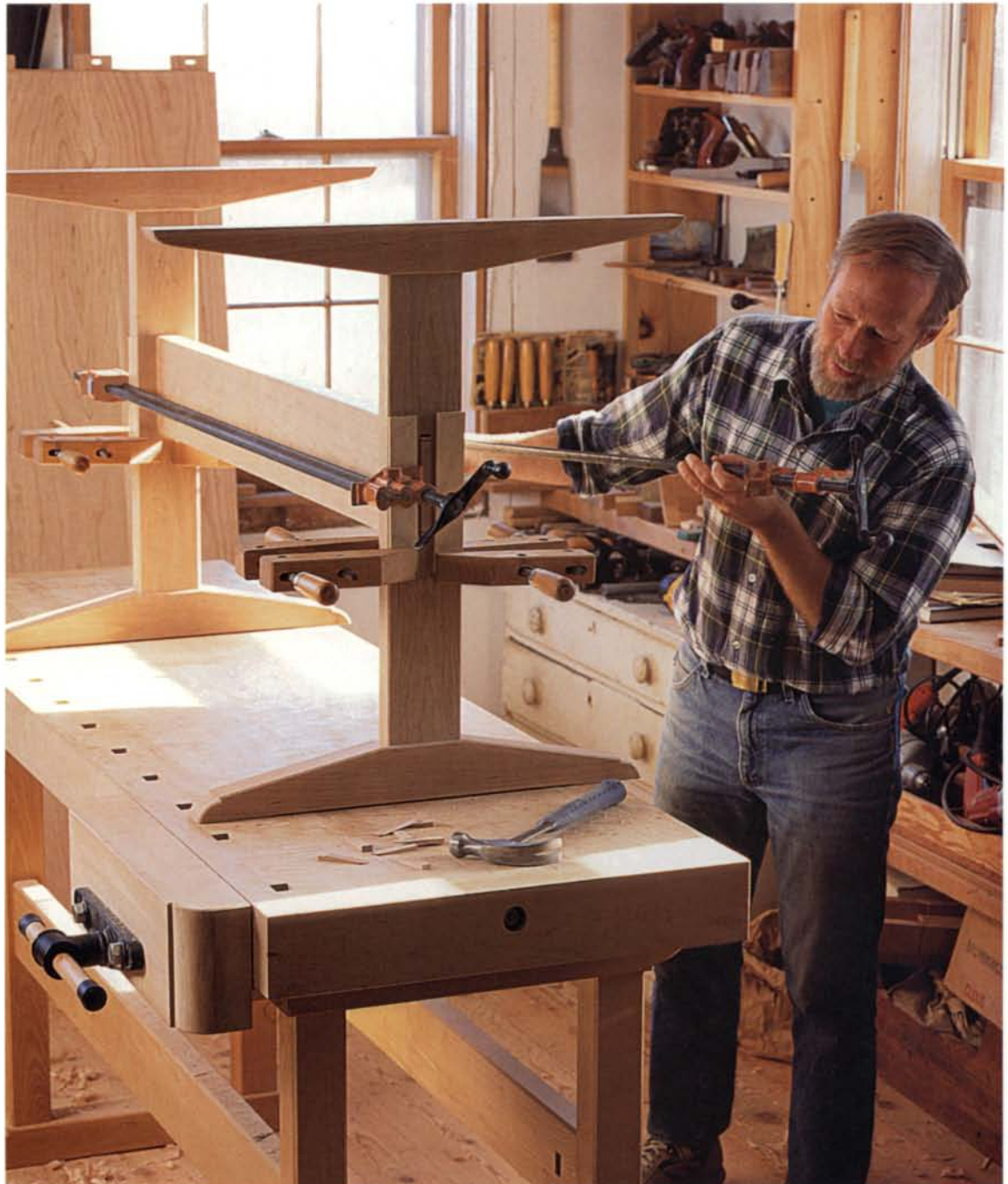
Trestle table with breadboard ends
