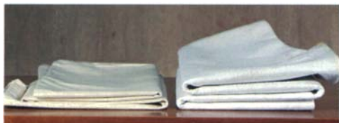
Fabric vs. felt. A fabric bag, left, has less thickness and is more porous. Felt, right, does a much better job of filtering out very fine dust.
