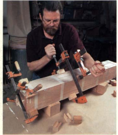
Shopmade blocks allow opposing clamps. Shop-built clamp blocks provide a perpendicular pad for the clamps. As opposing clamps are tightened, the box is pulled square.
