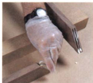
Two biscuits make a stronger joint. Biscuits provide ample gluing surface and keep the pieces aligned. Once clamps go on, check the diagonals to make sure everything is square.
