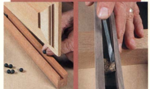
Cork cushions keep the panel centered but allow it to expand and contract. No glue is applied to the floating panel. Use a utility knife to cut cork slightly oversized. Space balls—perfect for \frac{1}{4} -in. dados—are hard rubber pellets designed to do the same job as cork (available from louis and company: 800-422-4389).
