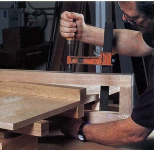
Tape and scrap make simple and effective deep-reach clamps. Tape a spacer between two stout scrap boards and slide the assembly over the cauls. Pressure applied near the edge is transferred to the middle of the panel.
