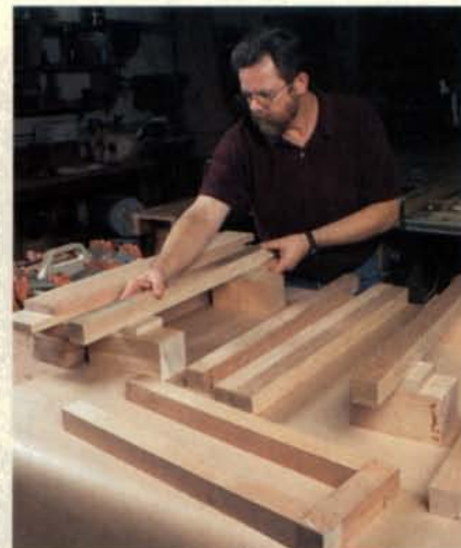
Raising the panel allows room for clamps. With glue and clamps at hand, begin by laying cauls on blocks so that it's easy to keep boards flat and in place.
