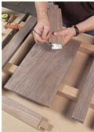
A little glue goes a long way. Apply glue only deep into the mortise and on the end of the tenon to keep squeeze-out to a minimum.
