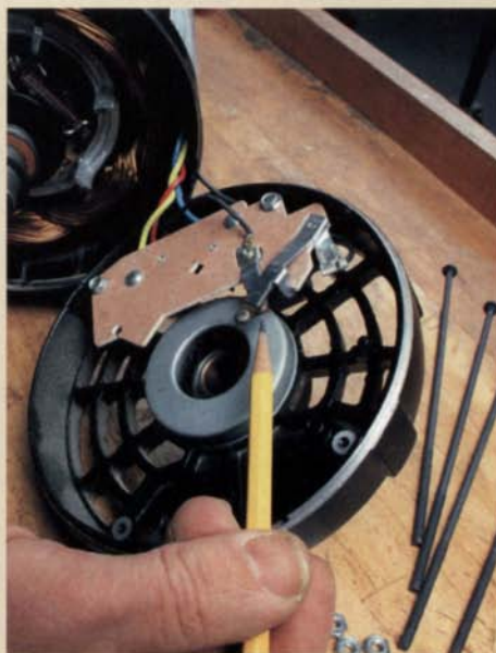
Check the contacts. With the motor open, inspect the contacts on the end plate.
