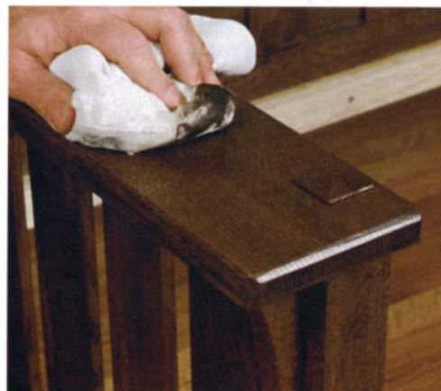
Black wax over shellac. The combination of these two finishes looks especially good when applied over fumed white oak.
