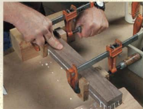
Clamping face-glued joint with cauls. First, use cauls to keep pieces aligned, then squeeze the joint together. Glue flows more easily when you start at one end and work toward the other.
