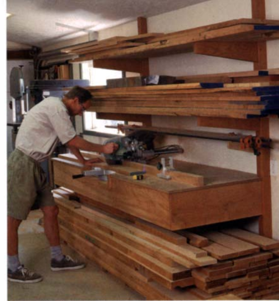
Lumber and a place to cut it. A system of cantilevered arms provides easy-access lumber storage as well as support for a chop saw table designed for rough-cutting planks.
