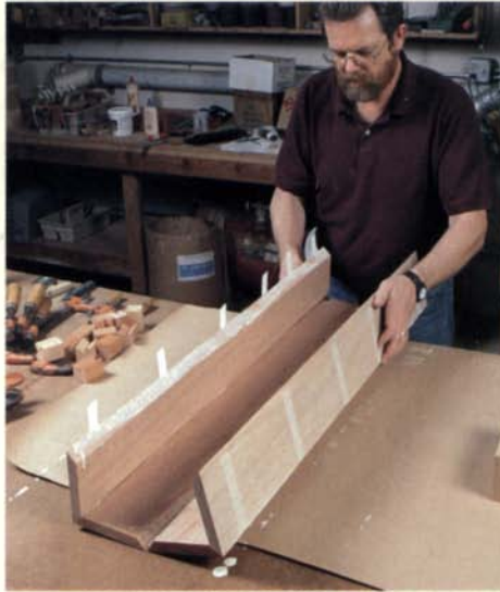
Mitered parts roll up to form a box. After the pieces have been turned over, glue is spread in the miters, and the box is rolled up.
