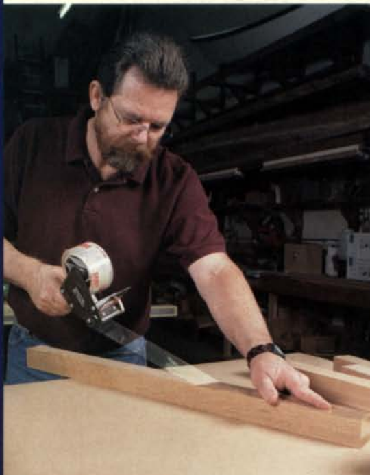
Raising the panel allows room for clamps. With glue and clamps at hand, begin by laying cauls on blocks so that it's easy to keep boards flat and in place.
