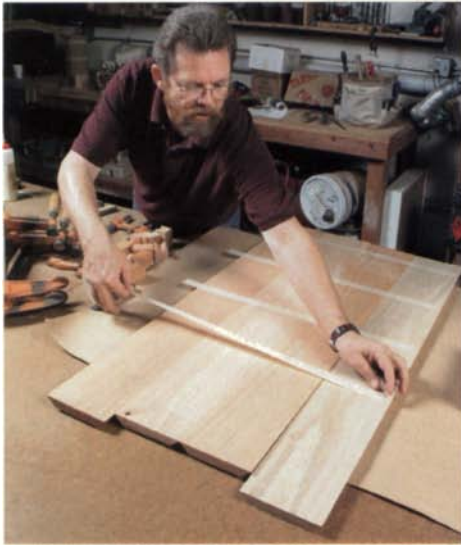
Packing tape binds the box. Stranded tape with imbedded fiber has tremendous strength. Strips of tape are laid on the face side of the box, keeping everything in place.
