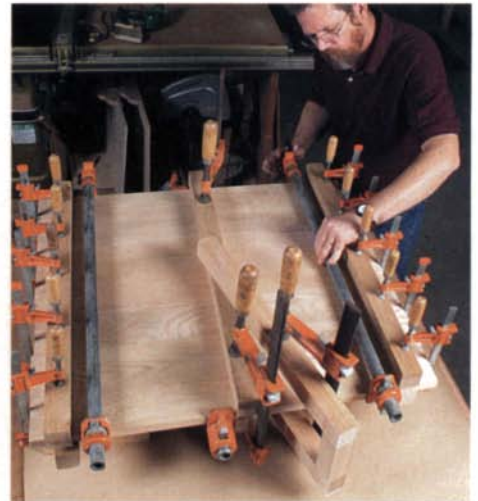
Bar clamps squeeze the joints together. Apply just enough pressure to close the joints—too much pressure will force glue out. Keep the bar clamps above the surface because black marks will appear everywhere the clamps touch the wet glue.
