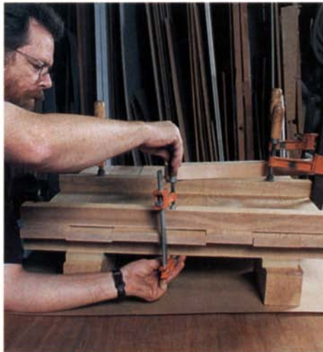
Cauls keep edge joints aligned. As the cauls are clamped together, the boards are pulled into perfect alignment. After the cauls have been firmly clamped in place, use bar clamps to pull the joints together.
