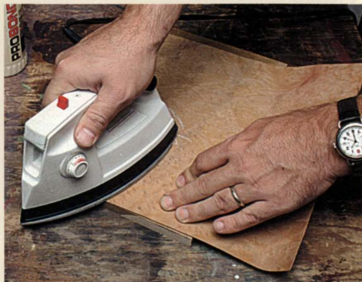
Shrinking the veneer. Pre-ironing dries and shrinks veneer, lessening the chance that it will buckle when glue is applied.
