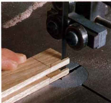
An easy but refined door detail. With the rail grooved and the mortise cut, a bandsaw trims away the inside edge to accept the stile.
