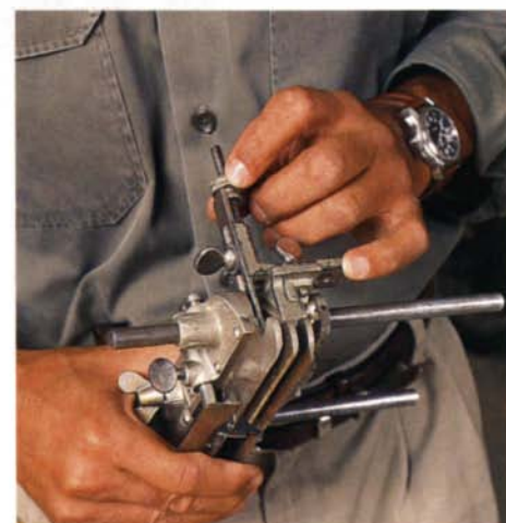
Adjust the auxiliary skate. An auxiliary skate can be attached to the sliding section for additional support. It can be adjusted laterally as well as vertically.
