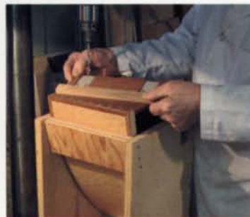
A cork-lined plywood cradle held the triangular side drawers so Lonson could drill accurate holes for the hinges.
