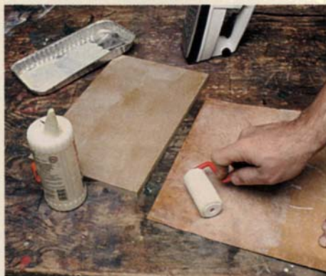
Laying on PVA. Using a small paint roller with a short nap, coat both the veneer and the substrate with PVA glue.
