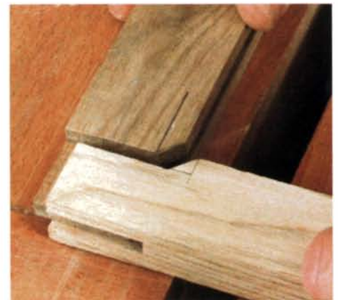
A perfect fit. It's best to work out any problems before you begin glue-up. A dry run ensures that everything fits and that the bridle joints pull tight.
