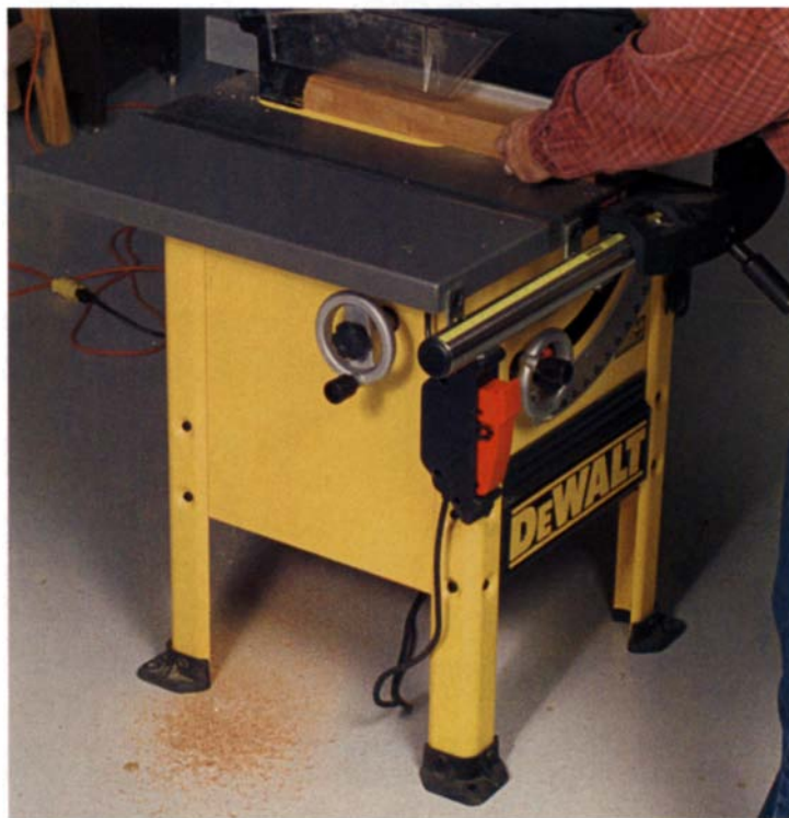
A well-designed contractor's saw. DeWalt's 1½-hp saw is compact and solidly built.
