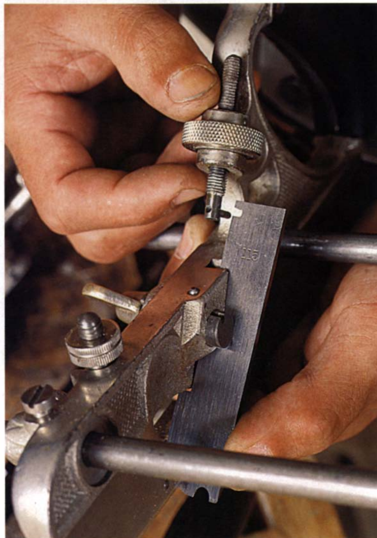
Engage the cutter. A notch at the top of the cutter engages a post on the adjusting knob's threaded shaft.
