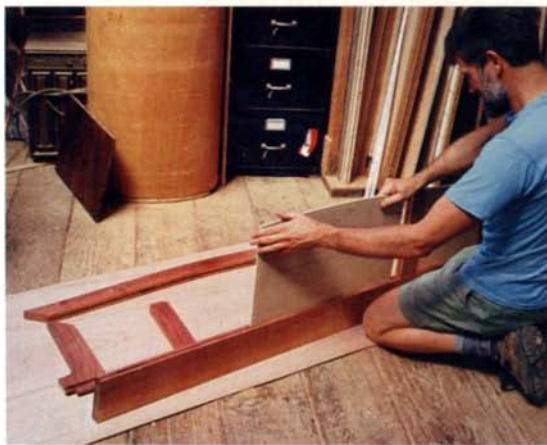
Dry-fit the headboard to determine the size of the panels. The author makes panel templates out of MDF.
