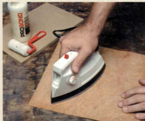
Shrinking the veneer. Pre-ironing dries and shrinks veneer, lessening the chance that it will buckle when glue is applied.
