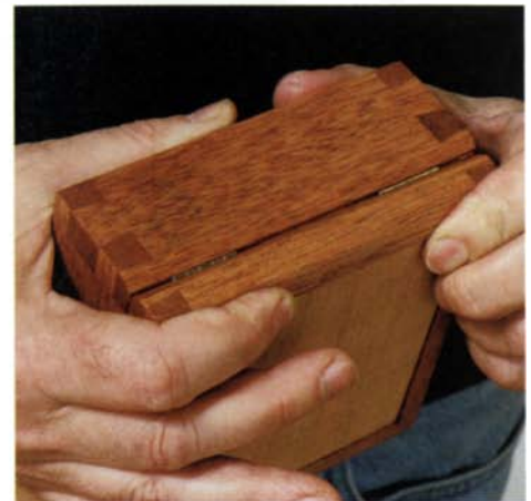
been pressed together. Simply slide the lid side to side (right) to make it line up perfectly. However, unlike other hinges, these barbed hinges cannot be removed without tearing out the wood around the slots.
