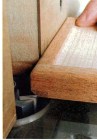
Cut the rabbet. After cutting the chamfer, cut a rabbet slightly more than \frac{1}{2} in. deep on the carcass and lid to make room for the \frac{1}{16} -in.-dia. hinge barrel.
