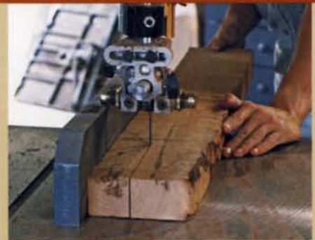
The right blade for hardwoods. Ripping hardwoods on the bandsaw is easy with a 1/2-in.-wide, 4-pitch blade.
