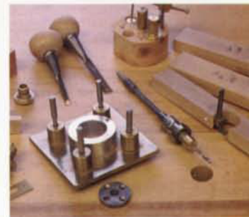
For many tasks on the commodes, Lonson made custom tools. The short, ball-topped chisels chopped mortises in tight spaces.
