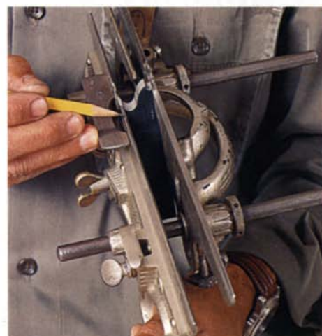
Line up the skates. To provide maximum support during the cut, get the skates in line with the high points of the cutter's contour. Set their heights just below the cutter's.
