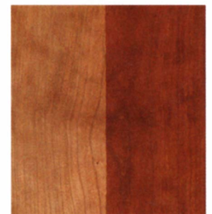
Aged cherry in no time. Potassium dichromate ages cherry better than any pigment or dye stain, without the inevitable blotches.
