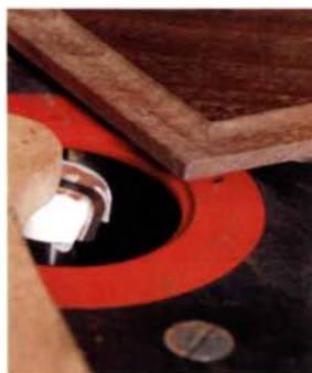
The walnut panels for the headboard are shaped on the router table. A bowl bit is used to detail both faces of each panel.
