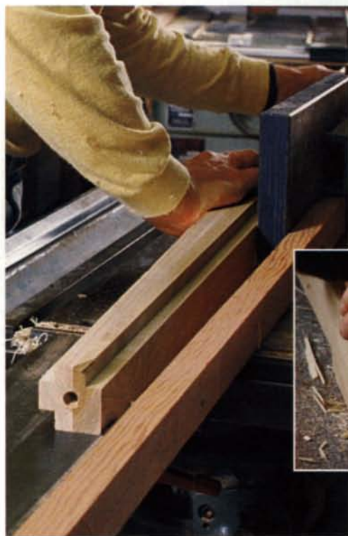
The upper portions of the posts are tapered. The author uses a shop-built tapering jig and a 12-in. table saw with a 14-in. blade. The blade guard is removed for this operation.
