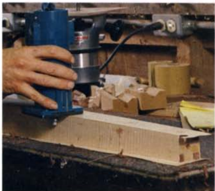
Veneers are trimmed flush using a laminate trimmer. Black acacia veneer will be glued over the maple veneer shown here. The walnut corner blocks are already in place.
