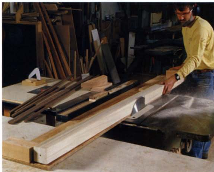
The upper portions of the posts are tapered. The author uses a shop-built tapering jig and a 12-in. table saw with a 14-in. blade. The blade guard is removed for this operation.
