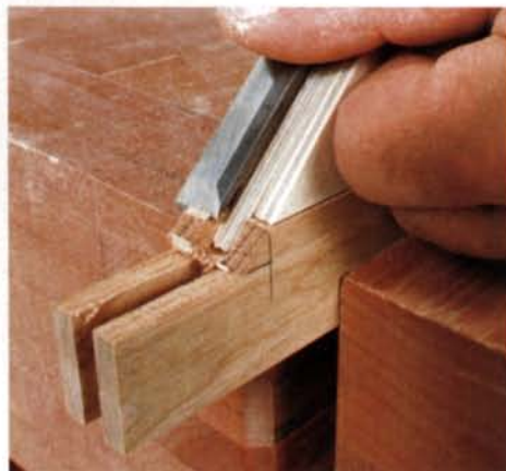
A mitered door joint. With a 45° miter jig clamped to the rail, a chisel pares to the line. This simple detail lends a framed and finished look to the door.
