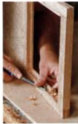
Rear wall of groove is removed to accept glass (above).
