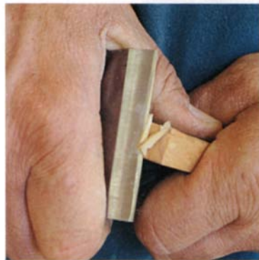
If a blade can shear the end grain of soft pine without tearing or crushing the fibers, it is truly sharp.
