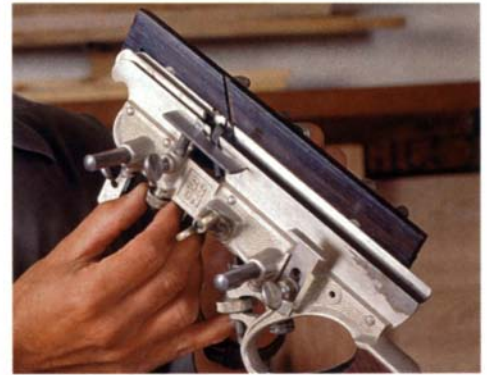
Set the depth stop. Depth of cut can be controlled by one or both of the 55's two depth stops.
