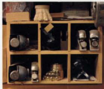
Lonson had brass lion's feet cast from a wooden copy he carved of the original foot. The lion's-head pulls came from England.
