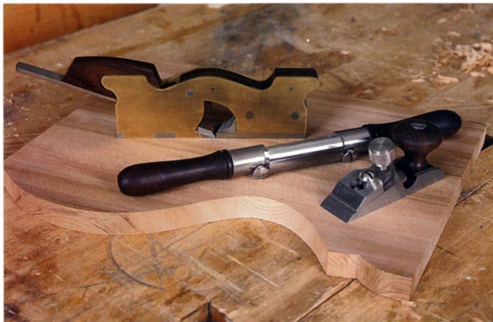
Hand-crafted hand tools. The Kelly Tool Works line includes (from left) a shoulder plane, a spokeshave and a chisel plane.
