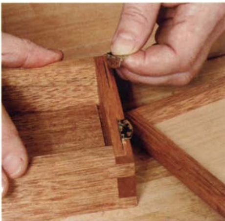
Finish the box before assembly. After the finish has cured, insert the hinges into the carcass (left photo), then the lid (middle). If necessary, you can easily make minor adjustments after the lid and carcass have
