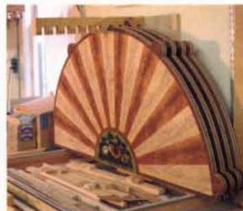
Lonson veneered the satinwood and mahogany sunburst over shop-made bass lumber core. He also made his own edge-banding.
