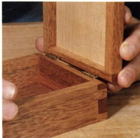
Finish the box before assembly. After the finish has cured, insert the hinges into the carcass (left photo), then the lid (middle). If necessary, you can easily make minor adjustments after the lid and carcass have
