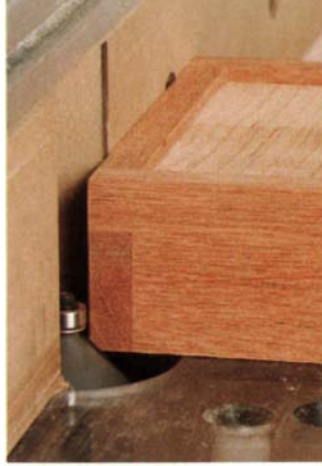
On the router table. Cut a 45° chamfer on the carcass and lid. The chamfer should end no more than \frac{3}{16} in. from the outside edge of the slot.
