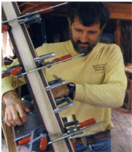
Walnut corner blocks are clamped into the rabbeted sections of the posts. The walnut strips are proud of the blank and flush-trimmed once the glue cures.
