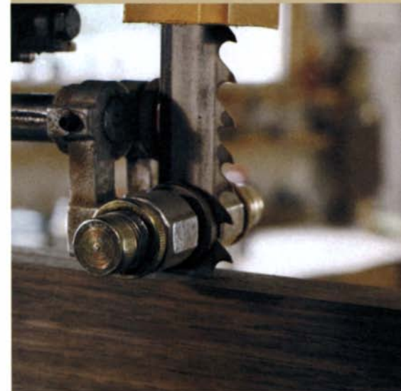
Smooth operator. A variable-pitch, hook-tooth carbide blade cleanly slices 1/4-in.-thick veneer from this crotch walnut plank.
