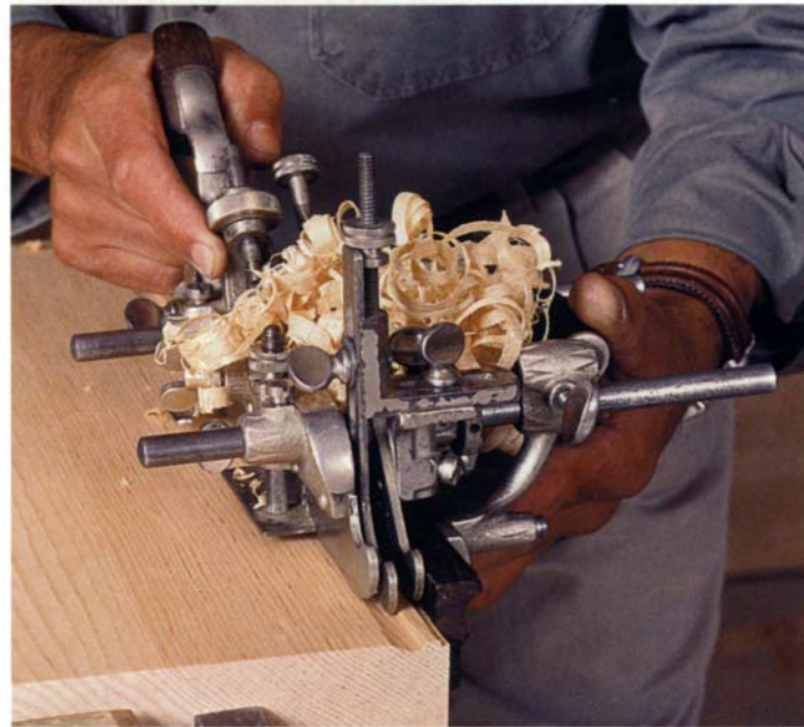
Fix the fence. The fence slides along the arms and can be positioned in height as well.
