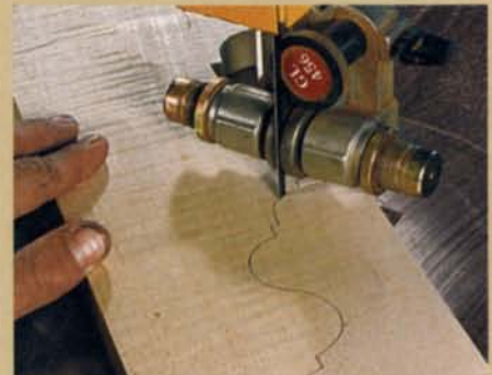
Good for most curves. A 1/4-in., 6-pitch blade can cut most contours, but a 10-pitch blade leaves a smoother surface.
