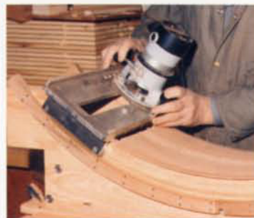
A passionate jig-builder, Lonson made this one to smooth curved core stock for drawer fronts. A convex jig smoothed the outer face.
