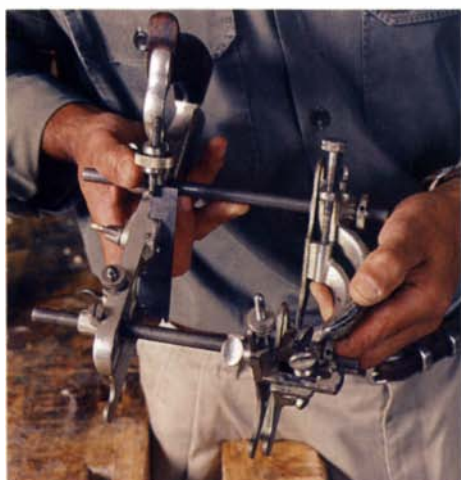
Fit the sliding section. The sliding section snugs up to the main body. With skates that adjust up and down, the sliding section separates the 55 from all other multiplanes.
