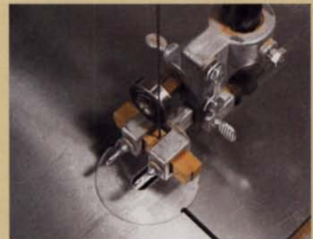
Tight curves, clean cuts. A 1/16-in., 24-pitch blade cuts intricate scrolls with little or no cleanup required.
