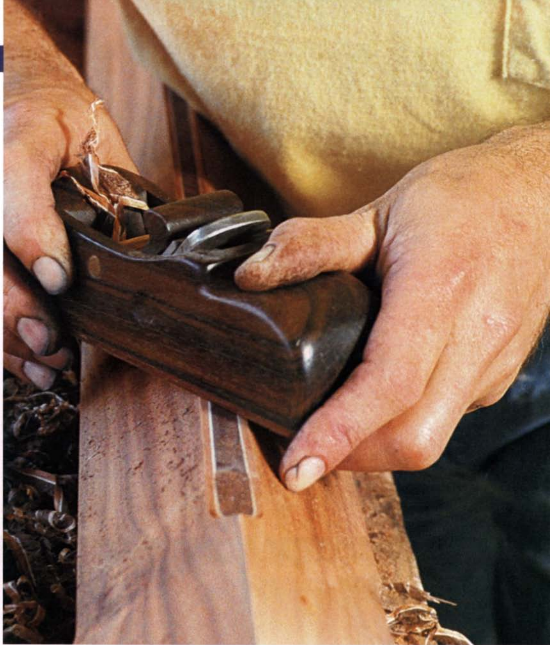
Chamfers, cut with a tilting-head shaper or router, expose the maple veneer, which looks like stringing. A handplane tapers the chamfers, which are widest at the lower portions of the posts.
