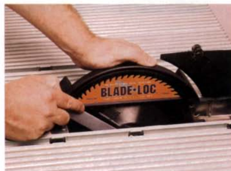
An easier way to remove a table saw blade. The Blade-Loc holds a sawblade securely while wrenching the arbor nut.
