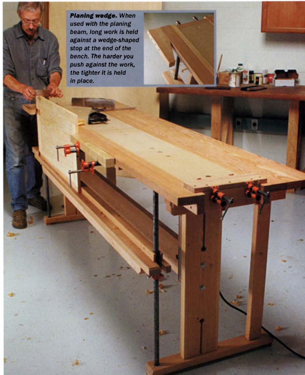
Sliding height adjustment. Pipe-clamp tailpieces slide on cast-iron pipes held captive in the top and bottom of the bench. A T-shaped Douglas fir planing beam rides on the clamps.
