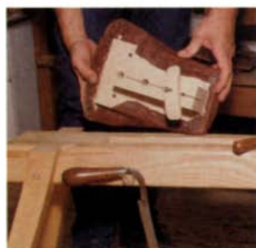
For a more ergonomic seat, you can glue wedges to the underside that raise the back 1 in.
