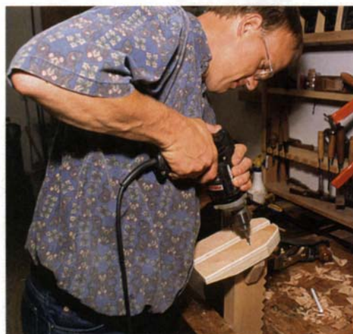
Go deep. Be sure the screws through the lower jaw are amply countersunk.
