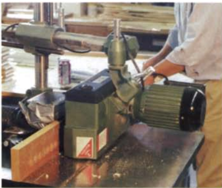
Power feeders are commonly used with shapers. Shapers may require large feeders, such as this ½-hp model (above), which is mounted sideways for this application.
