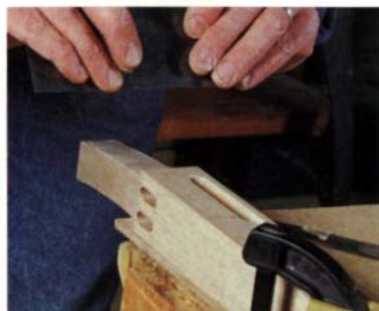
After cutting the mortises, shape the feet. The feet are cut out on the bandsaw, then cleaned up with a scraper.
