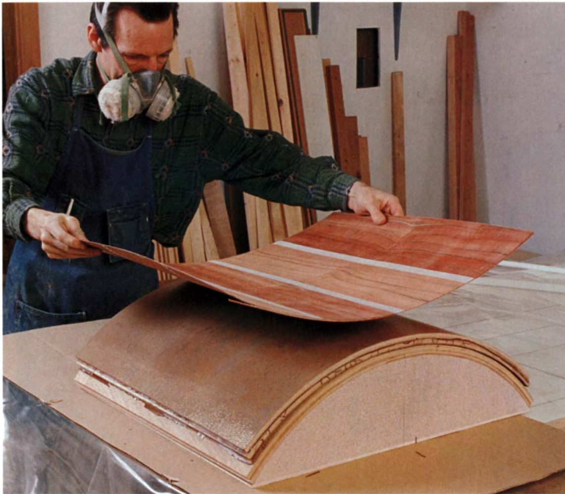
Two layers of veneer (two-ply) glued cross-grain to each other are used on both faces of the core.
