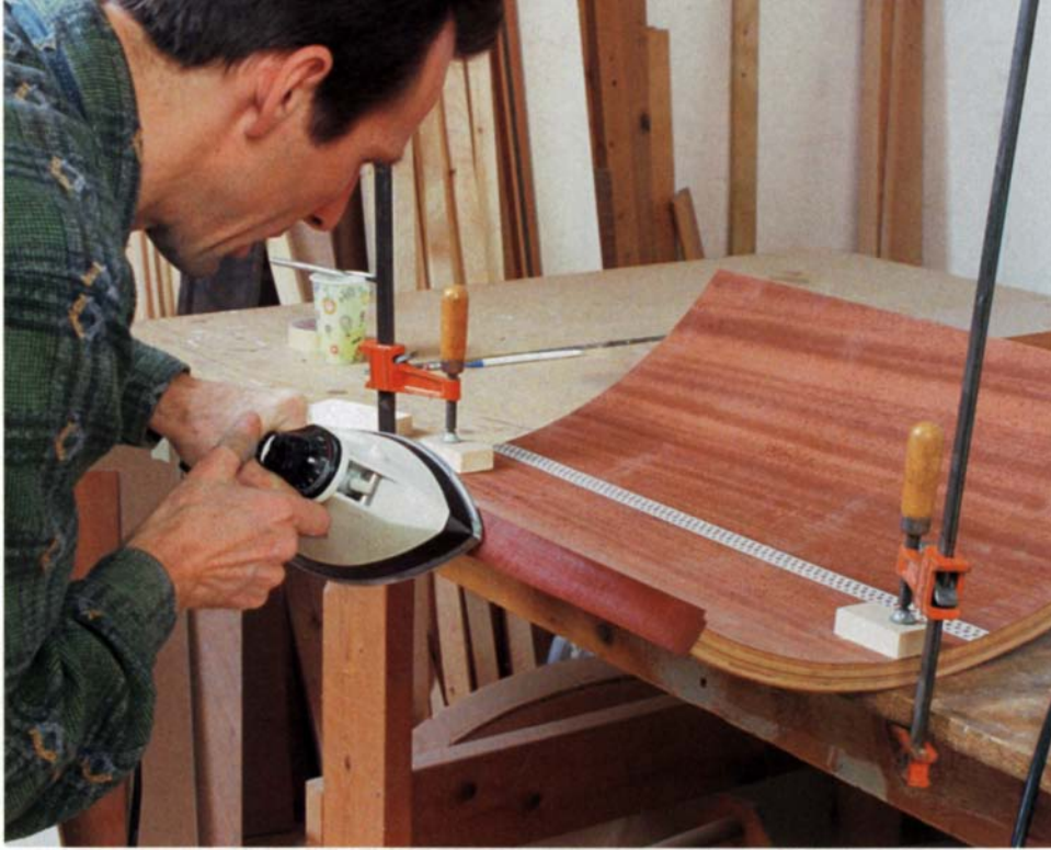
Edge-banding can also be ironed in place. Coat the edges of the core and veneer with yellow glue and let them set for an hour before ironing.
