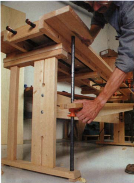
Sliding height adjustment. Pipe-clamp tailpieces slide on cast-iron pipes held captive in the top and bottom of the bench. A T-shaped Douglas fir planing beam rides on the clamps.
