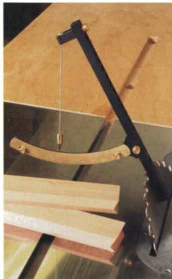
Angle-setting gauge from the Beall Tool Co. The Inclinometer attaches to the sawblade with strong magnets. It can also be used to set a jointer fence.
