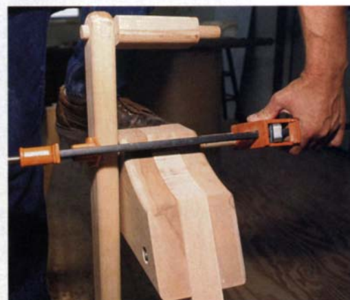
Watch that squeeze-out. Glue the ends of the treadle pivot pin but not the middle. Minimize squeeze-out and thoroughly wax the center portion of the pin.
