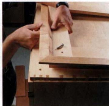
Removable molding. It's much easier to protect the molding if it can be wrapped separately when transporting the case.
