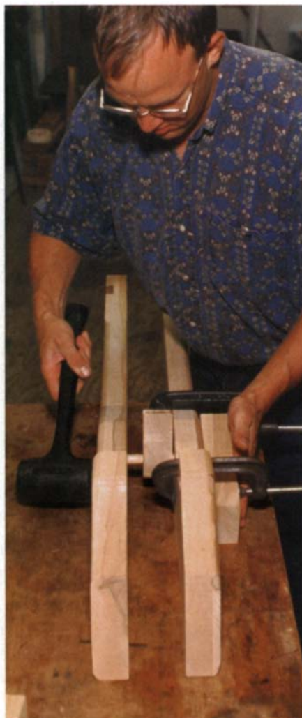
Don't glue me in. The whole length of the ratchet-key pivot pin is waxed before assembly. If the rubber tension strap ever breaks, the pin can be knocked out and the key removed for the repair.
