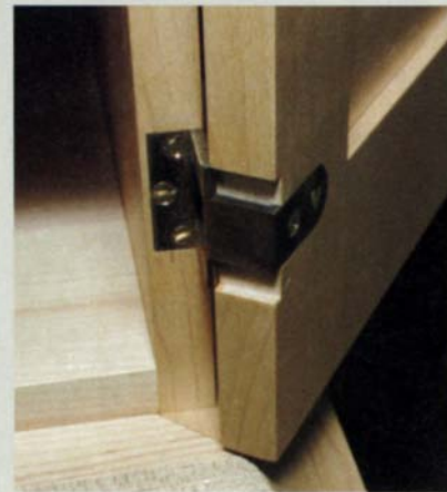
Cranked hinges allow doors to open wide. Mortises must be cut in the doors and the front edge of the case.
