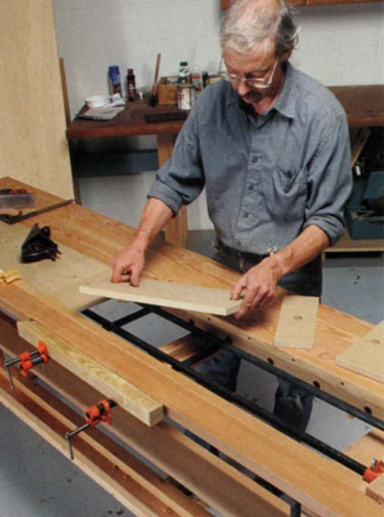
Lift-out MDF panels. The panels, cut in different lengths from MDF scraps, make a durable yet disposable center surface for the bench. The panels get removed when the tail-vise pipe clamps are in use.
