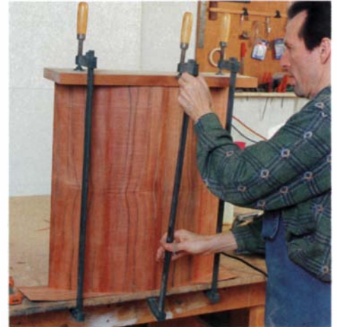
Clamp edge-banding veneer onto the ends of the workpiece. The author clamps directly to his workbench.
