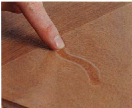
How much glue is right? A finger swiped across the glued surface should produce a shallow ridge.
