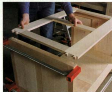
The top of the lower case is a simple frame without panels. Double dovetail joints are used at each corner to ensure the case won't bow.
