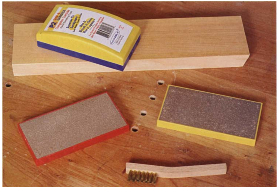
Sup-R-Sander blocks come in three grits. Tungsten-carbide particles are brazed onto a thin steel base, which is glued to the block's plastic body.
