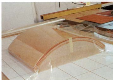
In the bag. A vacuum press simplifies the job of building forms and clamping curved parts during glue-up.
