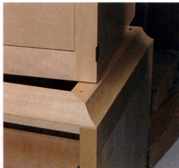
Upper and lower cases can be separated for ease in moving. Threaded inserts and bolts are hidden from view but make a strong connection.
