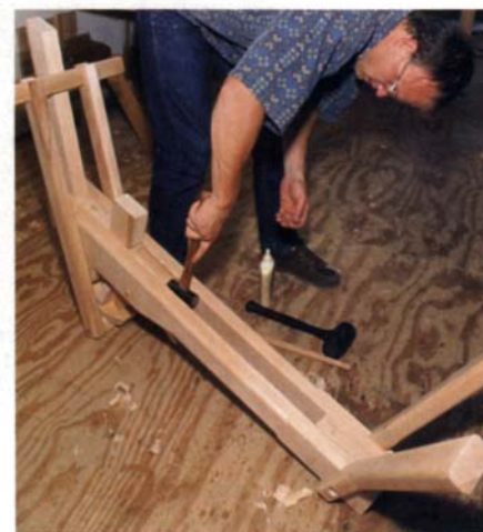
Wax and rap. With the ratchet riser in place and well waxed, coat the sides of the riser support block with glue and tap it up against the riser.
