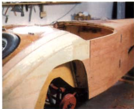
Skinning the body. The mahogany skin was fastened to the plywood body with epoxy and wood screws. The screws were later replaced with copper nails, for a more refined look.
