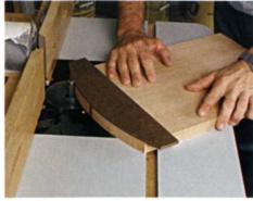
Trim the panel flush. Tack the template in place and trim the panel flush on the router table using a straight bit with a pilot bearing.
