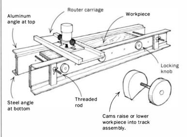
For the woodworker in a small, low-budget shop, Tim Hanson's router-surfacing fixture (*FWW* #77, pp. 42-43) offers the advantages of simplicity, accuracy and small storage requirements. When I set out to build Hanson's fixture, I couldn't find some of the components he used, so I revised the design as shown above.
