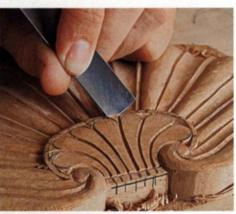
Chop the tops. After defining the tops of the petals using a gouge with a tight sweep, the author uses a shallower gouge to remove the triangular chip between petals.
