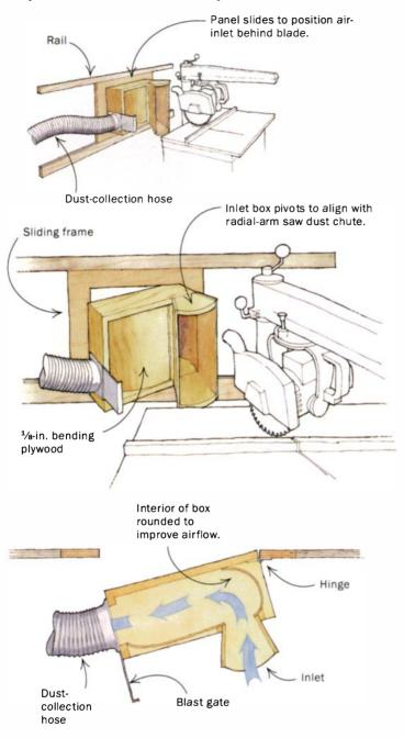
Collecting sawdust from a radial-arm saw is difficult because the sawdust is thrown in different directions, depending on the angle of the cut. Here's a solution that has considerably reduced cleanup at my saw (see the drawings at left). The device is a movable dust-collection port that can be swiveled to catch dust at just about any angle the saw can throw it.
