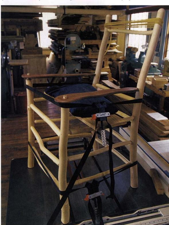
and rear panels (see the photos on the facing page). Brush a slow-setting epoxy in the mortises and use padded clamps to pull each panel together. Padded bar clamps work fine, but I often use my tail vise and some extralong wooden benchdogs covered with bicycle inner tube to avoid denting the chair parts. Once the front and rear panels have been pulled together, I glue in the side stretch-
