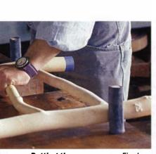
Putting the squeeze on. Final assembly begins with the front and rear panels. The author uses a slow-setting epoxy and pulls the joints home with his bench's tail vise and some extralong benchdogs (above). Elbow grease and a rubber mallet are used to drive the tenons of the side rungs and armrests home. Then band clamps hold them in place and a bag of sand across the seat rungs keeps the chair from twisting (right).
