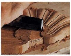
Shape and shave the rosette field. Using a gouge with a shallow sweep, the author defines the narrow, curving rib at the rim of the rosette. Then, after he chops in the volutes, he uses a wide chisel to angle the whole field of the rosette, ramping it downward from the rim toward a line between the volutes drawn 3/16 in. below the high point.
