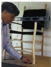
One last thing. With the chair on a flat table, place shims beneath the chair's legs until it is stable and level; then mark the legs at one height and trim them.
