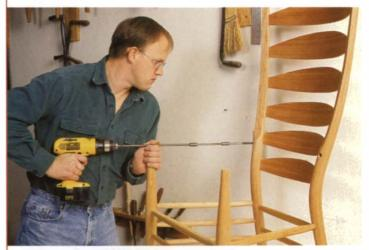
Handy for freehand drilling. The author uses a Powerbore bit for freehand drilling in cross-grain on rounded parts. The long center point of the bit holds its place positively, and the single-spur-and-lip design permits the user to start slowly, speeding up only when the bit is fully engaged in the hole.
