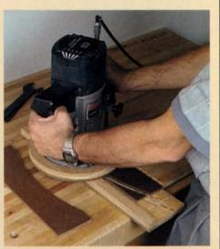
A matching pair. Once the radius has been adjusted, tack a Masonite blank onto the iig's well. Cut the panel template with the router in a single pass.
