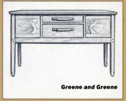
Ebony splines and details, rounded corners and carefully recessed legs can be used to build in a softer Arts-and-Crafts style.
