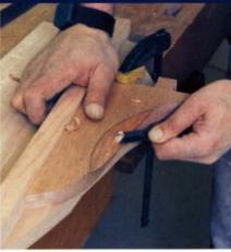
Fingerhold is cut with a gouge. The swinging leaf support, cut on the end with a gentle cyma curve. nests against the apron end, which gets cut with a slightly more exaggerated curve. The back of the support is relieved with a gouge to provide a fingerhold for opening the support.
