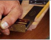
Hinge pivots at the roundover fillet line. Transcribe a line on the underside of the tabletop equal to the setback of the vertical fillet on the rule joint.
