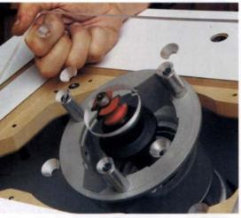
Replacement router collet works without wrenches. Because of the PowerCollet's large size, spacers must be used between the router and the baseplate.
