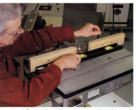
A fence should be square to the table and easy to adjust. A split fence, which is found on many benchtop models, such as the Woodstock Rebel, must be realigned each time it is moved, a time-consuming process.
