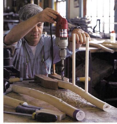
Dowel sighting. When cutting mortises with a hand drill, you can ensure that the holes are in the same plane by filling them with dry-fit dowels as you go and then sighting along the drill bit and the dowels.
