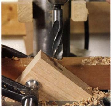
Moderate angles are no problem for a brad-point bit. Angles like this can be handled by a brad point because the spurs and center point are engaged before the lips begin cutting. The Austrian double-margin brad point (shown here) has separate margins for its spurs and its lips.
