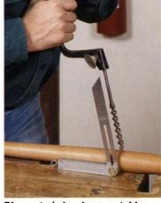
The auger's lead screw guides the cut. With its threaded lead screw pulling the bit into the cut, the auger bit requires very little feed pressure. The user can concentrate instead on getting the angle of the hole right.
