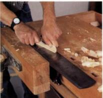
Jointer plane for straight edges. The longest of the steel-body planes, a jointer plane, with its 22-in.-long sole, cuts straight edges on long boards (above). Clamped upside down in a vise (left), a jointer plane works well for planing small or odd-shaped pieces of wood.
