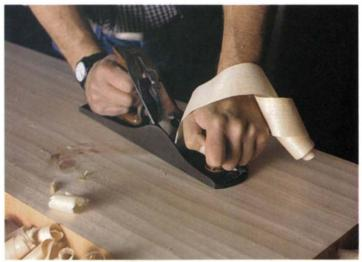
Face-planing starts with a jack plane. A jack plane, sharpened with a slight crest in the iron, makes quick work of dressing a roughsawn board. The telltale scalloped surface is a sure indication of handwork.
