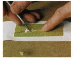
Using hide glue, tack the stack-cut parts onto white paper. The gaps left by the blade's kerf will be filled later with dark wax, which creates a sharp, thin outline.
