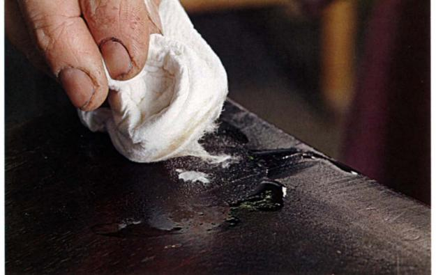
The tissue test. You can easily identify an unknown clear finish by dabbing it with different solvents and testing each patch with a piece of tissue to see if it sticks.
