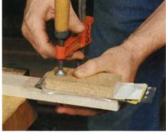
Gluing and clamping. After gluing a piece of onion-skin or tracing paper to the face of the partially completed oval, clamp it between blocks of wood. Veneers come in many thicknesses. To even out the pressure when clamping mixed stock, use strips of newspaper.
