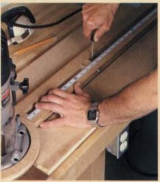
A slight adjustment. To cut the panel template, increase the radius on the jig's arm 1/2 in. to allow for the bit diameter and the panel tongue.
