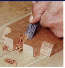
Knuckle relief. The back of the wood hinge knuckles are cut away at an angle so that the hinge can swing freely. If the knuckles were left square, their front sides would pinch one another as they swung.
