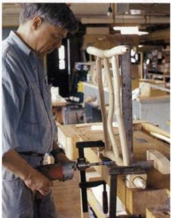
For angled mortises, tilt the frame, not the drill. To establish the angle for the side-stretcher mortises, tilt the chair's front frame forward (left). To help measure the tilt, use a framing square held upright in a kerfed block of wood. The author uses shopmade clamping blocks lined with leather to hold the work without marring it.
