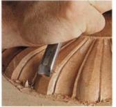
The ins and outs of lobes. Grain orientation on all but the center lobes will usually necessitate cutting toward the rosette on one side of the lobe and away from it on the other.
