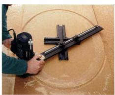
Master guide. The Ellipse Master accurately guides a router for cutting ellipses.
