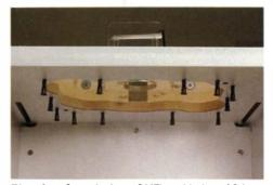
**The view from below.** CMT's table has 12 leveling screws, accessible from below. The Bench Dog router table has a similar setup.
