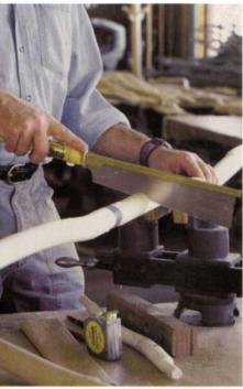
Don't try this on a tablesaw. A handsaw is the best and safest tool for crosscutting the irregularly shaped saplings. A Japanese dozuki saw, with its thin blade and fine teeth, is excellent for the job.
