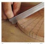
Two saws start things off. The author uses a bandsaw to make shallow kerfs that mark the transitions, or fillets, between concave and convex lobes. He follows up with a handsaw to carry the kerfs across the top of the shell. The deeper bandsaw kerfs are relief cuts at the ends of the concave lobes.
