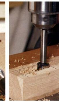
All-terrain bits. Steep angles, overlapping holes, very thin stock—none of these situations poses a problem for the Forstner bit, with its continuous rim guiding the bit. Unless the bit is backed out of deep holes every ½ in. or so, chips become impacted above it and can cause burning.
