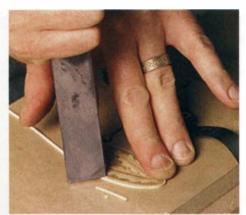
Wrap the oval with the holly. Cut the miter joint using a chisel held vertically. After applying glue, hold the stringing in place with tape.
