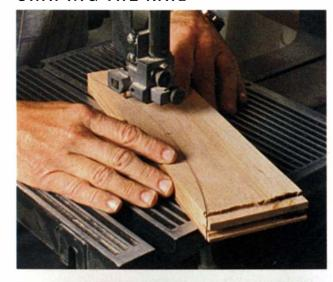
Roughing out the rail. Shape one end of the rail on the router table, then cut away the excess material on the bandsaw.
