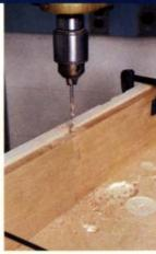
Fit to be drilled. Once the wood hinges have been pared to fit, clamp the pieces together against a backer board and drill a 1/8-in.-dia. hole through the hinge. A 1/8-in.-dia. steel rod is used as a hinge pin.
