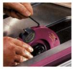
**Magic Molder** for tablesaws. Up to 70 cutter profiles are available. as well as blanks for making custom cutters.
