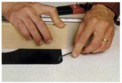
**Levelers are built into the Eagle America baseplate.** Six Allen screws are easily adjusted from above.
