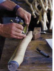
Marking for mortises. Working from rudimentary drawings, the author lays out centerlines for stretcher mortises. Because the materials in rustic work are unpredictable, the design of a piece changes along the way. So there is little value in precisely detailed drawings.
