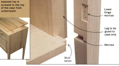
The dovetails that hold the case together are fairly easy to cut, either by hand or machine, but remember that the layout is different at each corner where a leg joins the case (see the top photos on p. 45). The top rear dovetails are cut narrow to make room for the back boards where the leg will be rabbeted. The case bottom has stub tenons that will be housed into the legs. These tenons are shouldered so that any later
