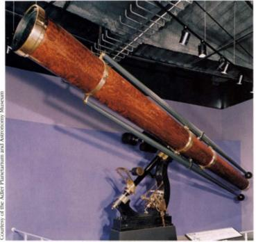
A wooden telescope. Multiple coats of varnish were dissolved off this 1863 Dearborn Telescope, but the original shellac was left intact.
