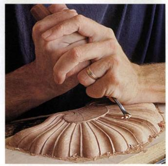
Giving convex lobes their curves. Convex lobes are shaped with gouges used bevel side up. A small backbent gouge is useful for the section near the rosette and for areas of tricky grain.
