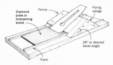
I was looking for a method to sharpen my plane irons that was quick, accurate and didn't remove too much metal. And I have an aversion to roller guides that are messy and push waste metal into the stone. I found the solution with this simple fixture.
