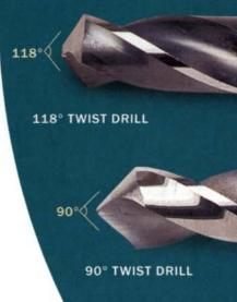
Best bit for end grain. A twist drill, which cuts like a ripsaw, bores into end grain beautifully. Brad-point and Forstner bits, which score the hole at the perimeter, act more like crosscut saws and perform better than twist drills in cross-grain but not as well in end grain.
