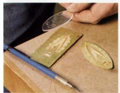
Mark the oval using a Plexiglas template. After cutting the oval, file the edges fair.
