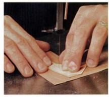
**Using clear tape, attach a vein to one half of a leaf.** Tilt the scroll saw's table to about 13°. Cut the first half of the leaf's vein. Bevel cutting will produce a very snug joint between parts.
