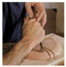
V-grooves start the fillets. After redrawing the fillet lines in the ramped area, a parting tool is used to establish each fillet with a V-shaped groove. The groove, centered on the line nearest to the convex lobe, should be about 1/8 in, deep at the rosette and deeper as it reaches the perimeter, where it should just erase the shallow bandsaw kerf.
