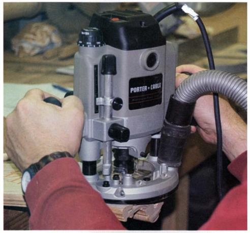
Midsized variable-speed router. When connected to a shop vacuum, the Porter-Cable model No. 7529 router, with its hollowed-out base, greatly reduces the amount of sawdust left behind.
