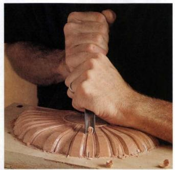
Concave comes first. Starting about a third of the way out from the rosette, the author cuts outward with a gouge of slightly smaller sweep than the widest point of the lobe. He takes increasingly deep cuts until the final pass cuts across the entire lobe, right up to the fillets. He cuts the center third with a smaller gouge, feathering its cuts into the larger ones. The last cut is made back toward the center, and a downward chop with a chisel relieves the waste.
