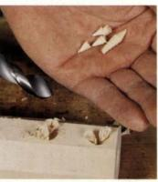
Long-point twist drill takes a sweet shaving. Ground to a 90° V-angle at the tip and sharpened properly, a twist-drill bit should cut cone-shaped shavings.
