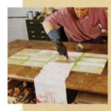
I put four different kinds of chemical strippers to the test on an old, painted piano bench. Using the tissue test, I found the top finish to be lacquer, but the tests for the paint underneath were inconclusive, so I assumed it to be an oil-based paint.
