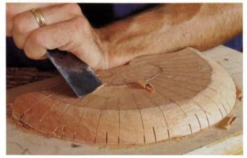
A gentle ramp. After defining the perimeter of the rosette at the center of the shell with 1/16-in.deep chops with a gouge. the author wields a straight chisel bevel side down to create a ramp, a slight rise from the rosette toward the perimeter.
