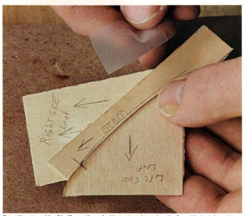
**Tape the second leaf half over the vein.** Veneer tape is used on the face side (not shown) to join the first two pieces together. All cutting and temporary taping is done on the back side (shown). The pencil lines denote grain orientation.
