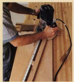
Making the rail template. With brads securing the template blank in place, a router outfitted with a 1/4-in. straight bit cuts a smooth arch in the rail template.
