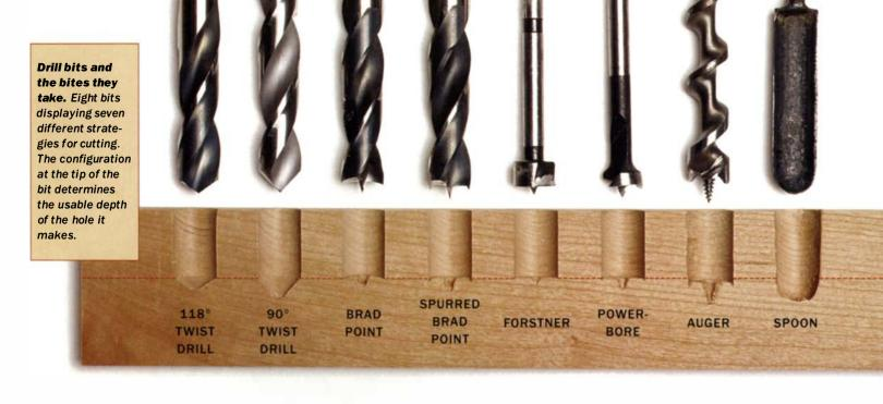
brad point. Also, the flutes clear the chips well enough that I can plunge to the bottom of a 1½-in.-deep hole in one pass without worrying about clogging.
