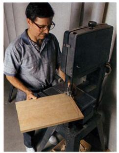
Cut the panel to rough shape. Trace the arc from the template onto the panel and trim the waste material away on the bandsaw.
