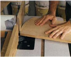
Raise the panel. When turning a flat panel into a raised one, you can make a safer cut by using both the fence and the pilot bearing.
