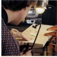
Cut carefully. Keep the fretsaw blade angled at about 13° and cut slowly and steadily, turning the stock as needed. Note the plywood support with a bird's-mouth cutout.
