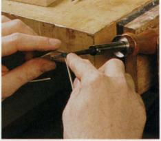
Bend the stringing using a soldering iron set on low. A feeler gauge helps nudge the stringing into shape. The author modified his soldering iron's tip by adding differentdiameter brass tubes slid inside each other.
