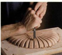
Open up the V-groove. A second pass with the parting tool flattens the V-groove on one side and establishes the fillet surface. The author rolls the parting tool toward the concave lobe and cuts that side of the V-groove so that it is at 20° or 30° rather than at 45°.
