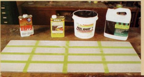
Before and after. The author tested four categories and brands of commonly available strippers. He checked and compared the results after 30 minutes, one hour, three hours and six hours.
