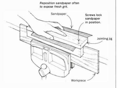
I designed the jig shown above for jointing edges when I was using thin, salvaged timber to be glued up into wide panels for cabinet doors. To get nearly perfect joints, I needed square, straight edges on the thin workpieces, and my cast-iron jack plane is too heavy and clumsy for such delicate work. The jointing jig I came up with is a bit slower than a plane, but the finished edges are square and smooth.
