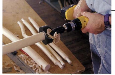
On a rustic chair, the only stretchers that need to be even vaguely straight are the ones for the seat. But when tenoning, you need to be sure that the stretcher is horizontal. Fit the stretcher in a vise, hold a long spirit level so that it rests on both ends of the stretcher and adjust the stretcher until you get a level reading (see the bottom photo on the facing page). If both tenons are cut on the same horizontal plane, it doesn't matter how curvy the wood between them is.
