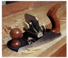
Big scraping plane from Lie-Nielsen. The No. 112 scraping plane weighs 4 lbs. and comes with a 27/8-in.-wide blade.
