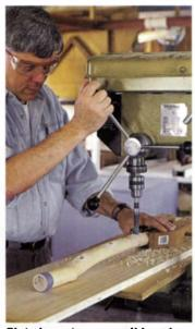
Flat clamp tames a wild workpiece. To make a curved chair leg fit for safe, accurate mortising on the drill press, attach a handscrew clamp to one end. The clamp holds the leg in register and provides a flat surface to mate with the table. To get mortises of the same depth, use the index on the collar of the drill-press arm.
