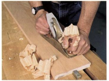
After the jack, use the smooth. A smooth plane is used for the final dressing of the face of a board. The plane is especially handy for removing the marks left by jointers and thickness planers.
