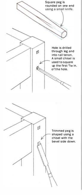
and rosewood. Ideally, the peg wood should be harder than the wood it will be driven into. Cut strips for the pegs first, then choose a drill-bit size just a trifle under the width of the pegs. Burnishing down a small square of masking tape prevents any fiber tearout when drilling the holes. Then square up the holes about 3/16 in. deep with a small chisel.
