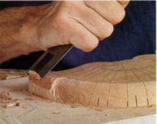
Rounding the rim. Starting in the center, the author uses bench chisels to turn down the perimeter of the shell (left). The shape he aims for is not an arc but a section of an ellipse: The curve begins gently and then accelerates. At both sides of the shell (right), he chops downward instead of slicing through side grain. A few strips of double-sided carpet tape secure the blank to a sacrificial backer board during carving.
