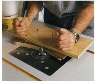
Cut the profile and curve in one pass. With the template tacked into place, use a railcutting bit to shape the profile and fair the edge.
