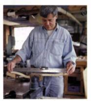
What's in the middle doesn't matter. Only the tenons on both ends of an irregular workpiece must be aligned for the joints to fit. That alignment starts with a level held to the stretcher.
