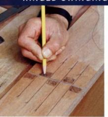
The drop-leaf supports swing on a wood hinge. Hinge knuckles-two on the support and three on the stationary pieceare 5/8 in. long. The width of each knuckle is determined by the width of the apron stock divided into five parts. A cyma curve on the end of each support adds a decorative touch.
