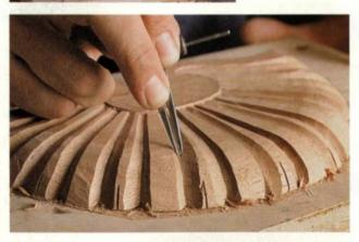
Finishing the fillet. With dividers or a compass set at 3/32 in.. the author scribes the width of the fillet from backer board to rosette (left). One leg of the dividers rides in the bottom of the V-groove, the other on the concave-lobe side of the V-groove. With the parting tool, he makes a shallow cut to the concave-lobe side of the line (below left). This cut both defines the fillet and starts the wall of the concave lobe.
