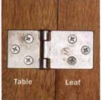
Looks like a butt hinge, but it ain't. A table-leaf hinge has leaves of different lengths, and the screw holes are countersunk on the sides opposite the barrel.
