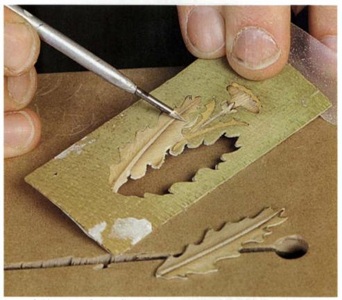
Leaves fall into place. Once the first leaf has been completed, place it in the background and secure it with veneer tape. Return to the pattern, align the second leaf and repeat the steps.
