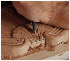
V-grooves stop at the bar. Parting-tool cuts define the petals of the rosette, starting at the rim and ending at a 1/s-in.-wide bar at the base of the ramp.
