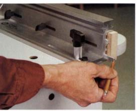
The Bench Dog has aluminum rods for shimming the outfeed fence. One face has been machined to square it up. Also, large knobs are used for all adjustments.
