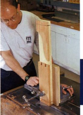
Table aprons are double thick. After the swinging leaf support has been cut, fit and drilled and the end of the apron is cut with a cyma curve, the primary apron pieces are glued to subaprons. Cutting tenons on the doubled-up aprons is straightforward. In the photo, the swinging support has been removed from the apron.
