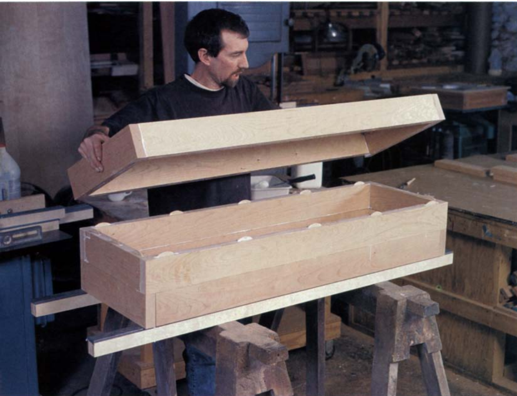
A race against curing glue. The cabinet must be glued up in one swift process. Four-board boxes are biscuited, coated in white glue, then set onto similar assemblies.
