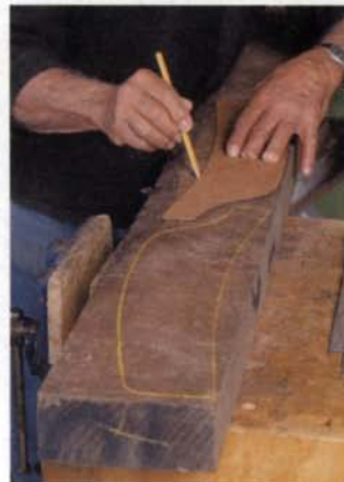
Interlocking layout. Tracing a plan-view pattern, the author lays out chair arms in a 12/4 walnut board. He flops the pattern and nests the layouts to get as many arms as possible from the board.
