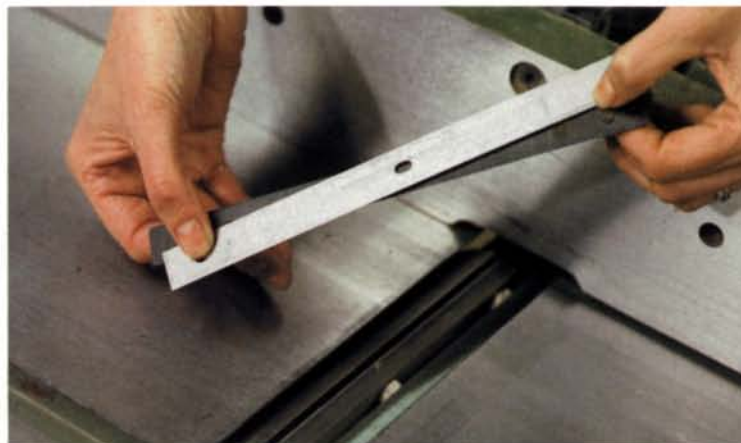
Esta disposable knives are available for most jointers. The retrofit kit includes all of the parts you need to simplify knife-changing.
