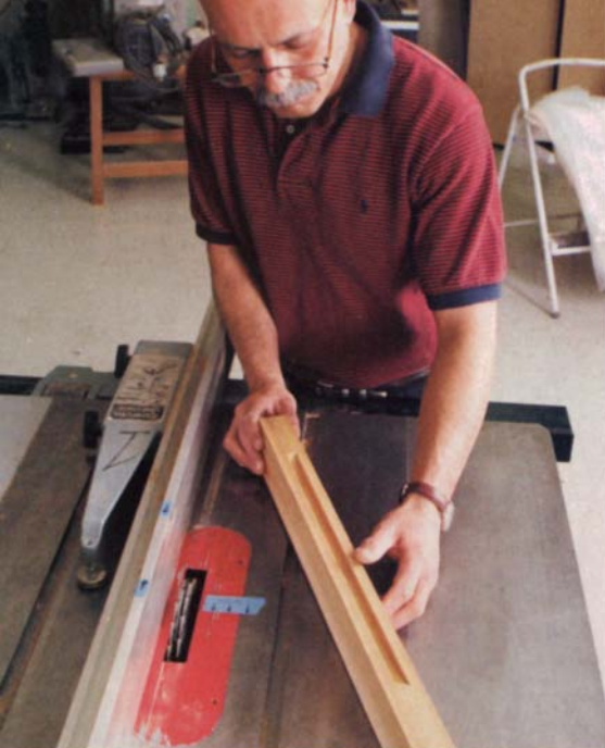
Grooves in the stiles are stopped. Use tape to mark the beginning, center and end of the cut. Lower the stock carefully onto the blade, cut the groove and lift the stock off the table.
