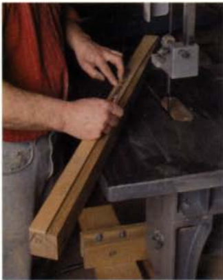
Template with a brain. Before bandsawing, the author traces the curve of the leg from a 1/4-in.-thick MDF template. The template is also a story stick, marked with the locations of all of the horizontal elements in the sideboard.
