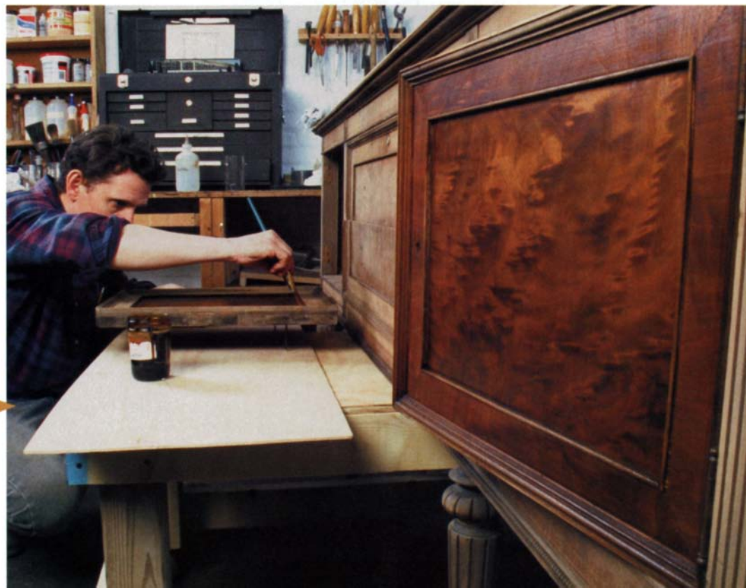
Two ways to finish both sides at once. The doors on this walnut sideboard illustrate two ways to finish both sides of a component: Either leave the door in place for finishing or take it off the cabinet and place it on a nail board for finishing.
