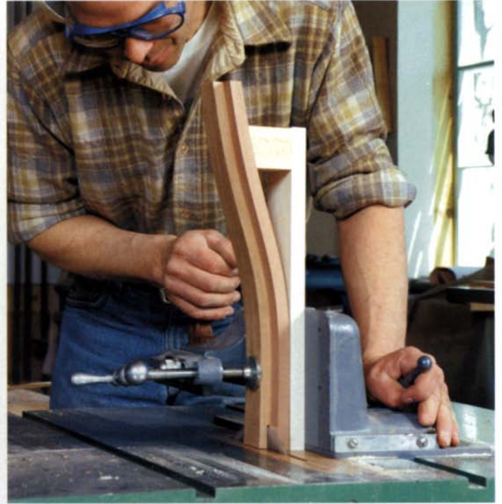
If parts are laminated or steam-bent, make a jig for a jig. A simple jig supports this curved piece at the correct angle and still makes it possible to use a tenoning jig.
