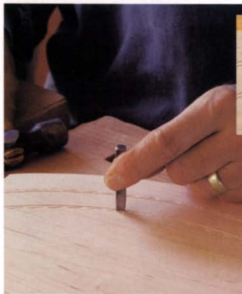
Filling in. With the grooves and the first stamp having established a framework, building the rest of the pattern is a matter of filling in.
