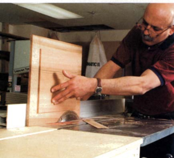
Cut the raised panels on the table saw. A shallow shoulder is cut 2 in. from the edge of the panel. Blade marks are cleaned up with a shoulder plane and then sanded.
