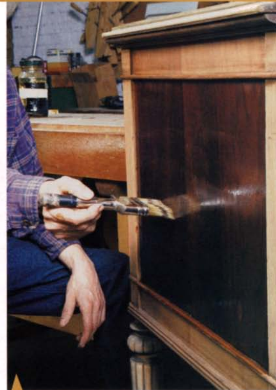
Tip it off top to bottom. Use only the very tip of the bristles of a good-quality varnish brush to even out a cross-brushed finish and to keep it from sagging.
