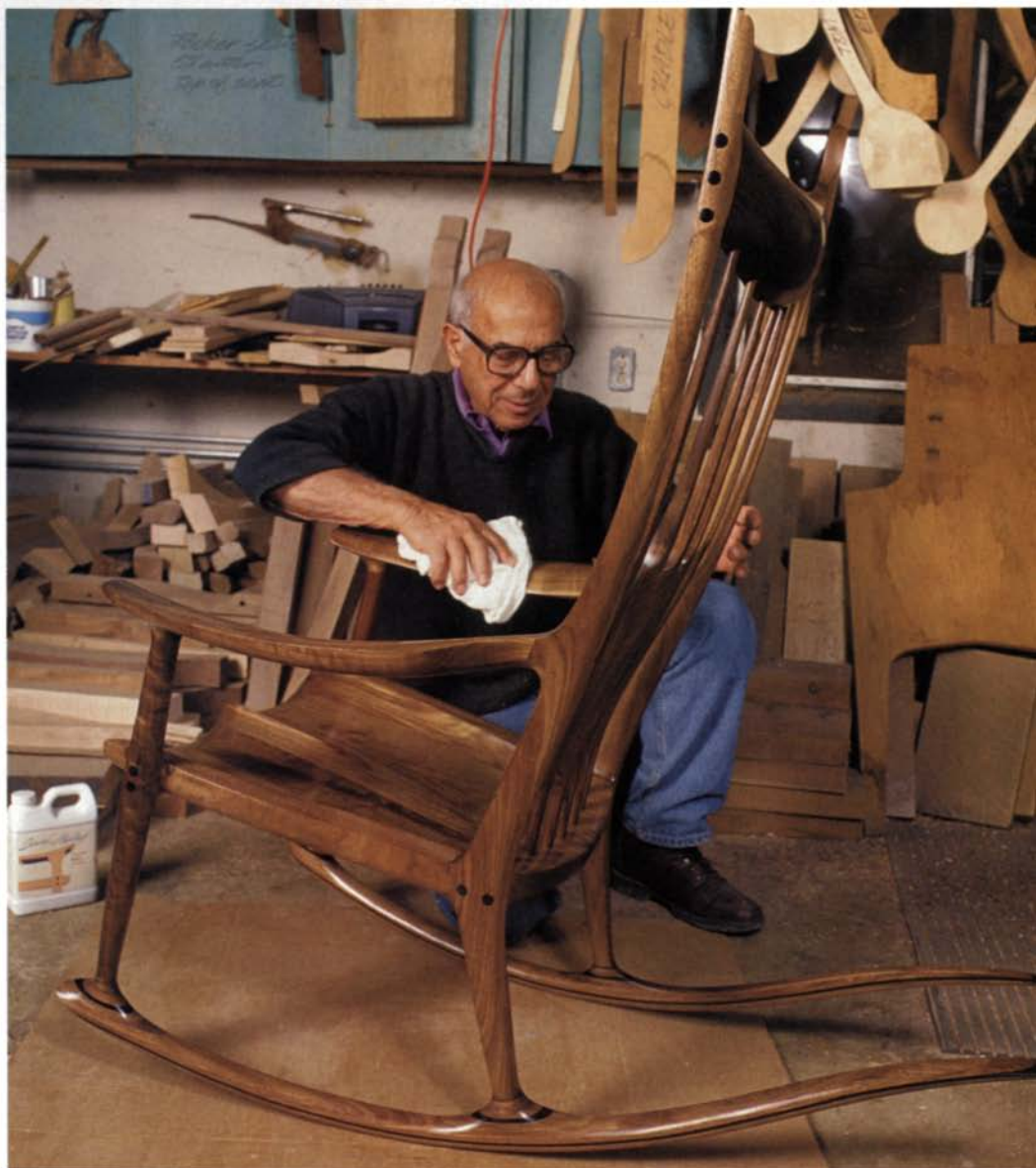
Rubbed the right way. The author's chairs get four coats of oil finish and two coats of wax, each coat thoroughly rubbed out.
