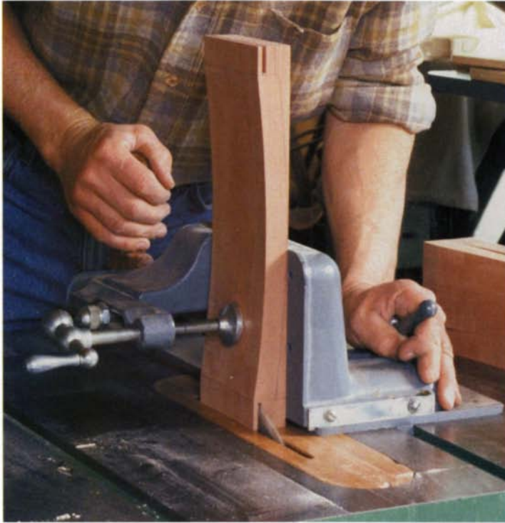
When possible, cut joints before cutting all of the curves. This chair rail still has one flat face, which goes against the tenoning jig. Bandsaw the convex curve after cutting the tenons.
