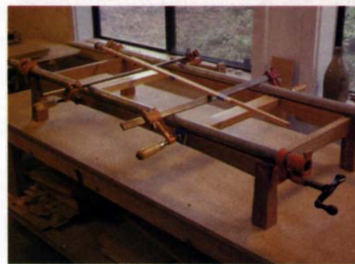
Slim but strong. To make a strong base without wide rails, the author made the rails \frac{15}{16} in. thick, added cross braces and notched the spline tenons for deeper penetration into the legs.
