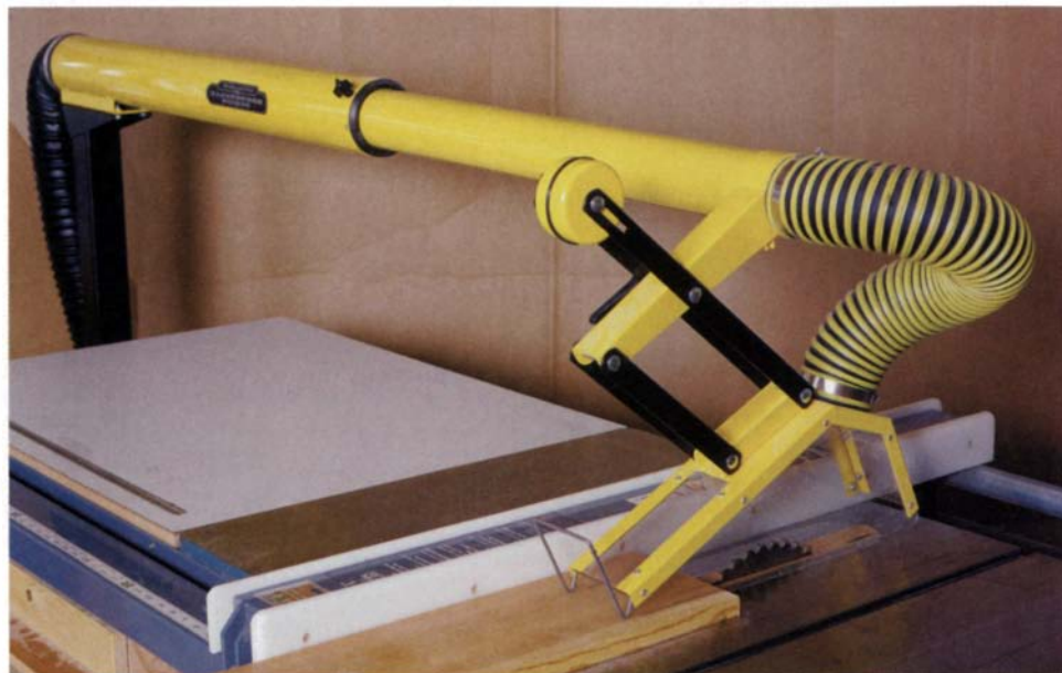
Bigger hose makes for better dust collection. The Excalibur EXBC overarm tablesaw blade cover by Sommerville Designs has a 4-in.-dia. hollow column that connects to a dust collector.
