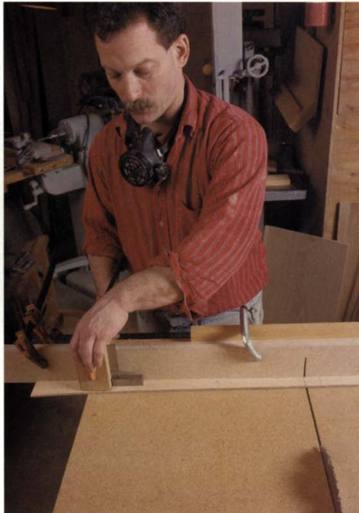
Don't move that stop block. After cutting the leg segments for the upper case, the author leaves the stop block where it is to cut the sides for the upper case.
