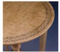
Begin with a V-groove. The author follows a pencil line with a V-parting tool to cut grooves that establish the radius of the pattern.
