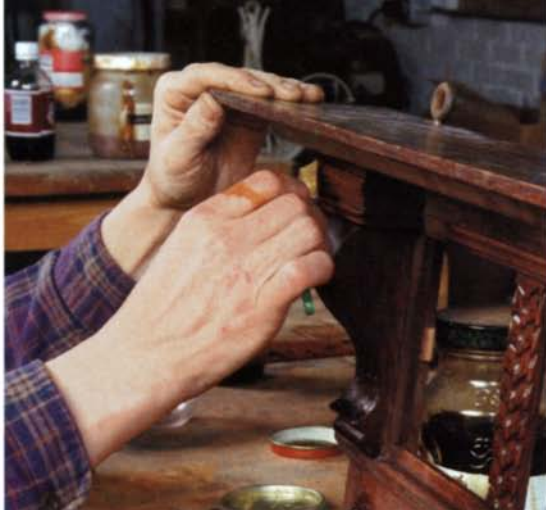
A toothbrush for tight crevices. For tight spaces and intricately molded shapes, apply a gel varnish with a soft toothbrush, then brush off the excess finish with a large, dry bristle brush.
