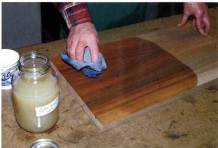
Applying a glue-size. A washcoat of hide glue, thinned to a liquid at room temperature, not only reduces blotches, but it also improves the finish surface of thirsty, fuzz-prone woods such as black willow (shown).
