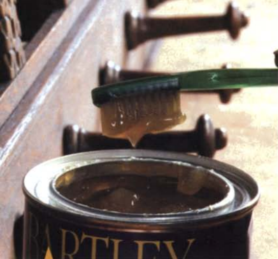
A toothbrush for tight crevices. For tight spaces and intricately molded shapes, apply a gel varnish with a soft toothbrush, then brush off the excess finish with a large, dry bristle brush.
