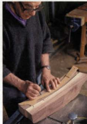
Adding another dimension. With the arm blank jointed and planed, the author traces a second pattern to establish the general contours of the arm's elevation.
