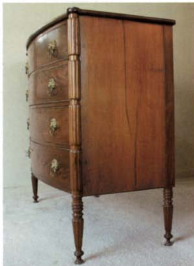
Floating panels don't split. These two bow-front chests are very similar in form and age but not in construction. The top chest, with a single-board side fixed to the legs, top and bottom, has cracked due to fluctuations in heat and humidity. The side of the chest in the middle—a floating panel held in stiles and rails—hasn't cracked.
