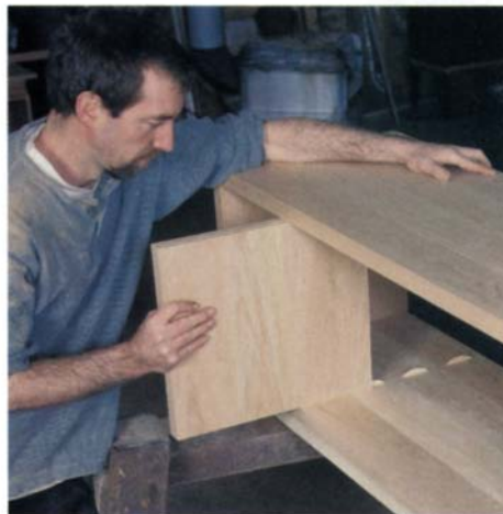
Like a hand in a glove. Biscuits are glued into the cabinet frame, then the grooved divider slides easily into place.
