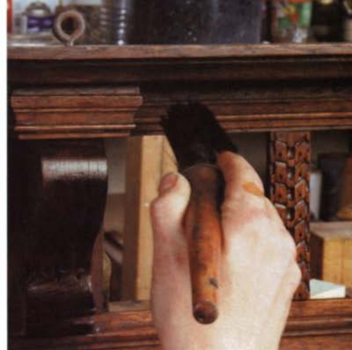
A toothbrush for tight crevices. For tight spaces and intricately molded shapes, apply a gel varnish with a soft toothbrush, then brush off the excess finish with a large, dry bristle brush.
