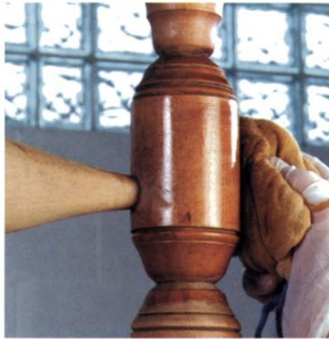
A pad for shellac. A wad of soft, absorbent, lint-free cloth is all you need to make a pad for applying shellac. You can use a plastic squeeze bottle to wet the pad or you can dip it into the finish. Wipe on the shellac in light, smooth passes.
