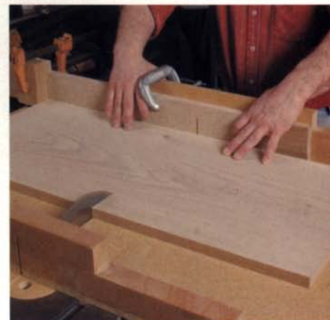
Don't move that stop block. After cutting the leg segments for the upper case, the author leaves the stop block where it is to cut the sides for the upper case.
