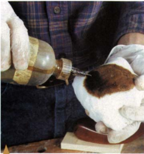
A pad for shellac. A wad of soft, absorbent, lint-free cloth is all you need to make a pad for applying shellac. You can use a plastic squeeze bottle to wet the pad or you can dip it into the finish. Wipe on the shellac in light, smooth passes.
