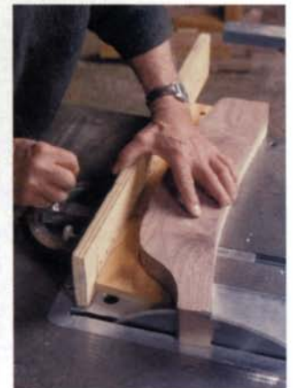
Good references. The compound angle where the arm will join the chair's back leg is cut on the table saw while the arm is still flat on the top and bottom. A simple, curved plywood jig steadies the curved side of the arm for the cut.
