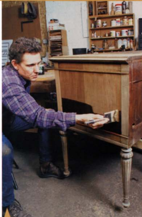
Lay it on left to right. Cross-brushing, which works best with varnish, starts with a horizontal application of the finish.
