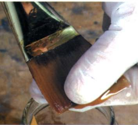
Storage trick prolongs brush life. Squeeze excess shellac from the bristles and let the remaining finish harden on the bristles. A dip into alcohol will make the bristles soft and supple again.
