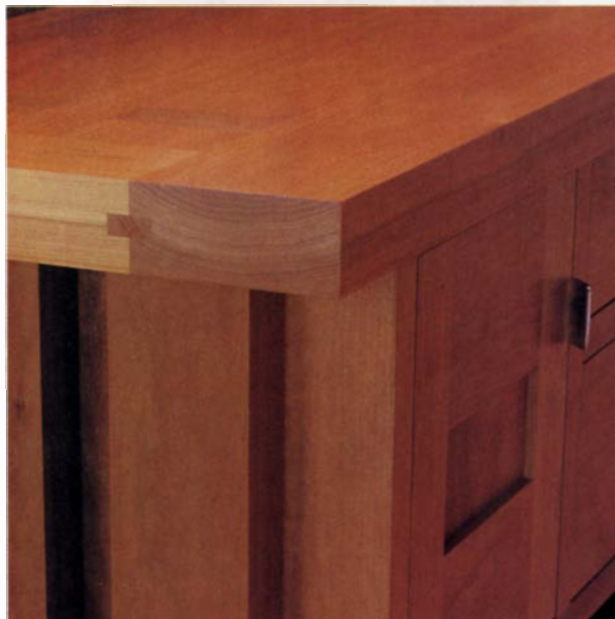
Breadboards with a twist. The unique breadboard design of the tabletop calls for the long side boards to sandwich the short end boards.
