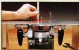
Once your router is clamped, you can easily prop up or flip the plate to adjust bits as shown.
