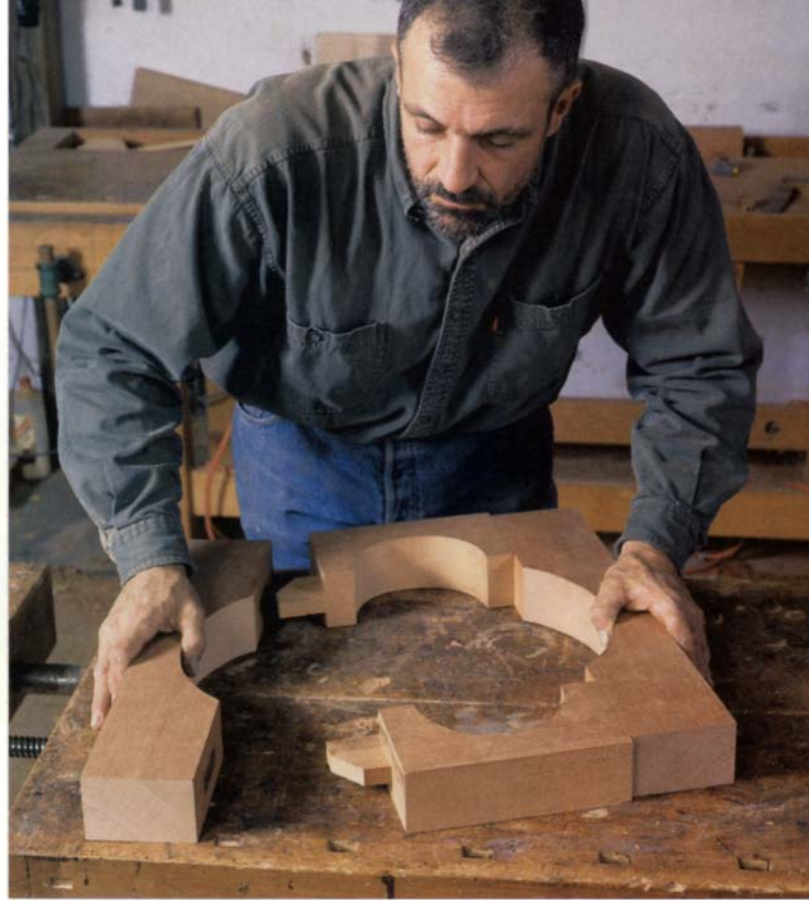
Assemble the frame. The bulk of the frame has been reduced by bandsawing arc-shaped segments prior to assembly.
