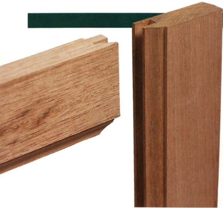
Cope-and-stick bits do most of the work. The sticking portion of the bit cuts the profile and groove in one pass. These bits are best suited for 3/4-in.- to 7/8-in.-thick stock.
