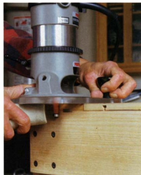
Edge trimming. Trim the platform edge parallel to the L-section face. The metal rails are set back from the face to prevent damaging the router. A vacuum hose catches the MDF dust.
