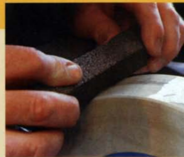
Silicon-carbide sticks produce a coarse dressing on well-worn wheels and cost from $2 to $10.
