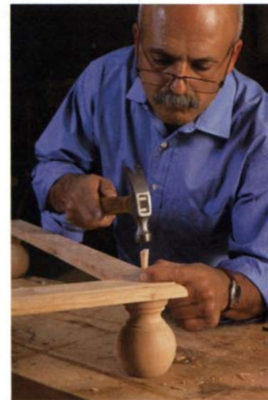
Footed frame. The round tenons of the bun feet are wedged to holes drilled in a molded frame. The frame is screwed to the bottom of the case.
