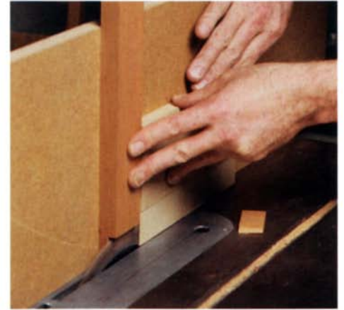
Cutting the cheeks without a tenoning jig. The rail is pushed along an auxiliary fence clamped to the tablesaw's fence. A backer block prevents tearout.
