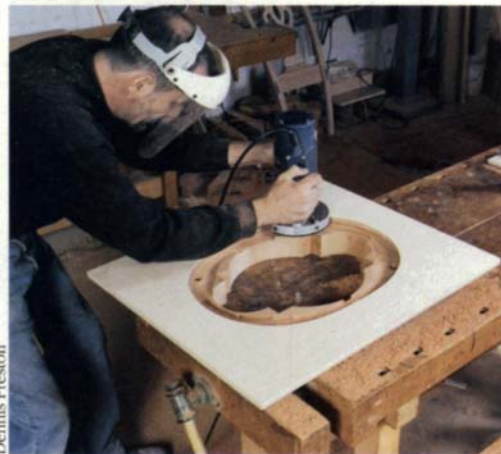
Assemble the frame. The bulk of the frame has been reduced by bandsawing arc-shaped segments prior to assembly.
