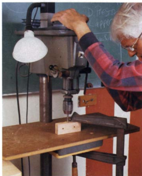
Tapping holes. Turn the drill-press spindle by hand. Once the tap engages the wood block, it self-feeds, cutting uniform threads.
