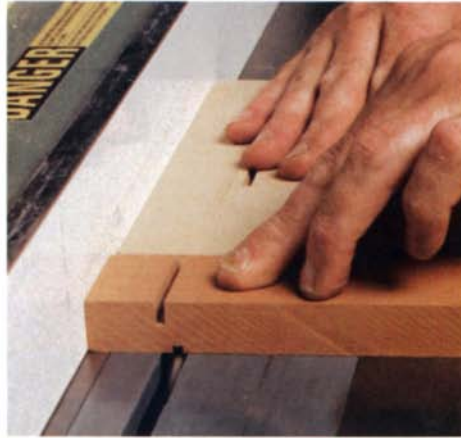
Rails must have offset shoulders. Guide the stock along the tablesaw fence and push it using a backer block for extra support.
