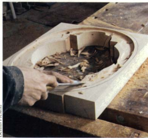
This gouge is good. To hog away stock the router couldn't reach, the author used a gouge.
