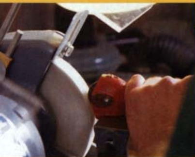
Simple steel (or “star”) wheel dressers sell for about $15. The wheels eventually wear out but can be replaced.
