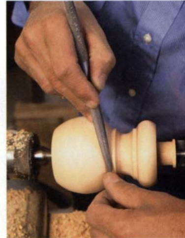
Finish with a rasp. Use a rasp with a light touch to smooth the bumpy surface left by the gouge and to finish shaping the bun foot.
