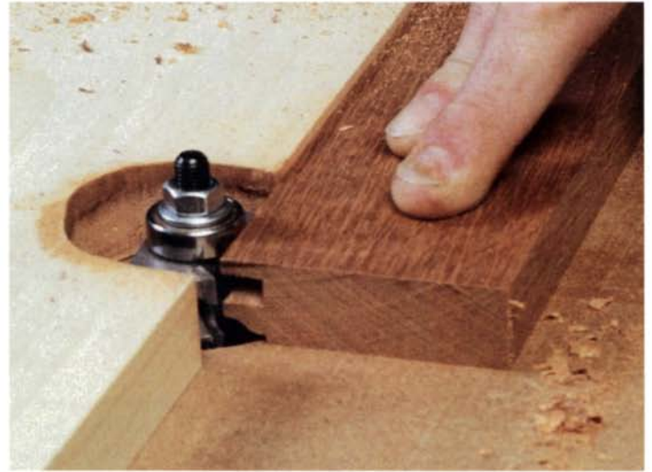
Cope-and-stick bits do most of the work. The sticking portion of the bit cuts the profile and groove in one pass. These bits are best suited for 3/4-in.- to 7/8-in.-thick stock.
