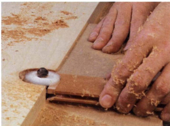
Rout the matching coping. Use a backer block when cutting the coping along the end grain of the rails.
