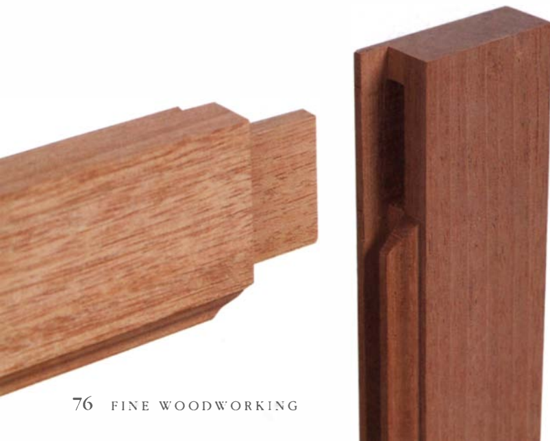
Make final adjustments using a chisel. The back wall of the groove on the stiles must be removed up to the miter. On both rails and stiles, use a guide block—a piece of scrap cut at 45° and clamped to the stock—to miter the inside corners of the profile.
