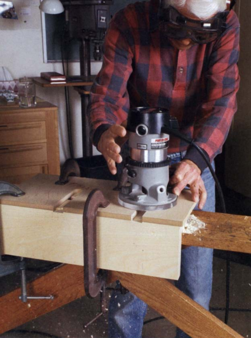
A template makes matched rail slots. Align the front edge of the template with the L-section. Repeating this operation on the platform ensures that the rails stay in alignment and that the jig operates smoothly. The cuts are made with a top-bearing pattern bit.
