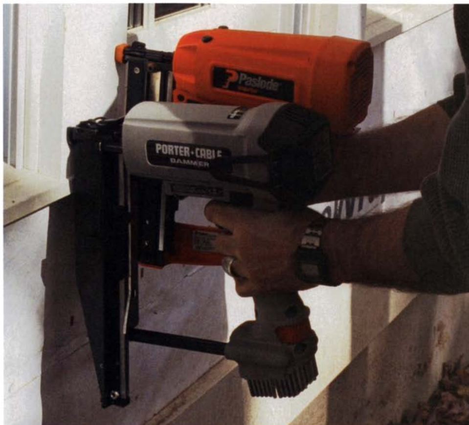
Fuel, not compressed air, powers these finish nailers. The Porter-Cable Bammer is the least costly of the two, but the Paslode Impulse nailer is easier to operate.
