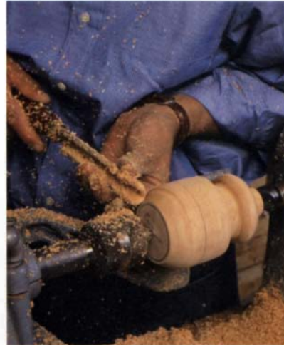
Bun foot starts with a gouge. Turn a rough cylinder, then use a pencil to mark out the major segments of the foot, including an equator for the foot's sphere.
