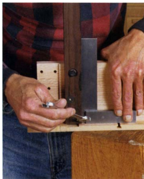
Square the fence to the platform. Tighten the two fence-mounting screws to lock the position. A slightly oversized hole allows the fence to be positioned at exactly 90°.
