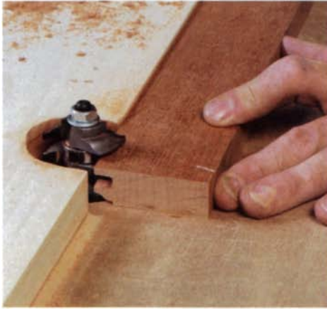
Shape the rails and stiles on the router table. The sticking portion of a cope-and-stick bit cuts the profile and groove in one pass. Set the fence flush with the bearing.
