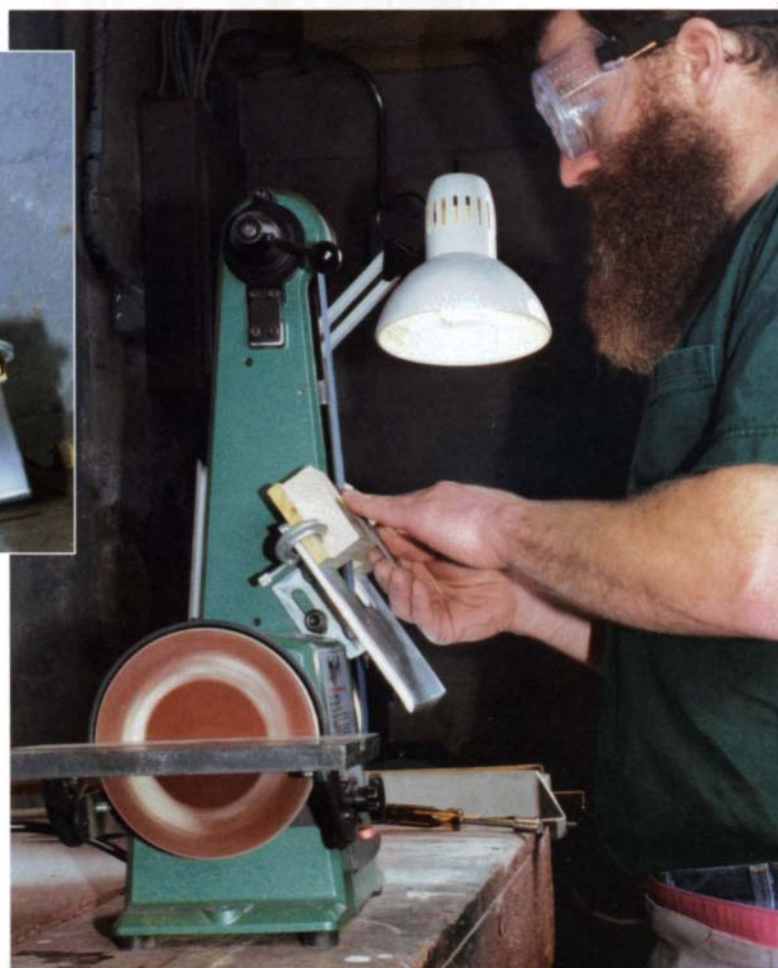
Customize the belt sander's tool rest for better performance. A block of wood, notched and back-beveled to clear the sanding belt, makes this machine more useful for a variety of blades.
