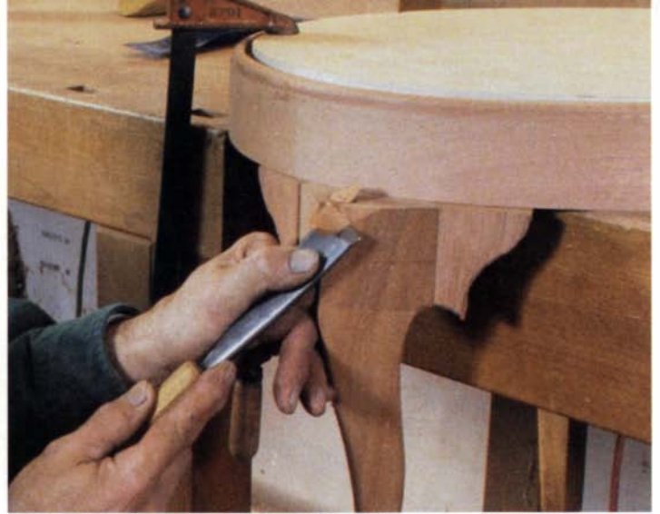
Knee work. With the leg dry-fitted, rough-shape the upper leg, blending the knee to the frame. Final fairing with a rasp is done after glue-up.
