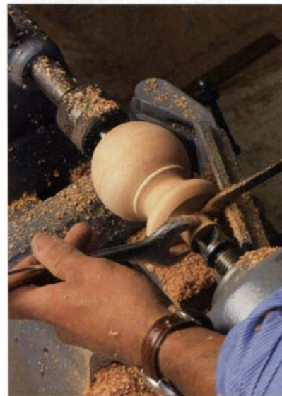
Wrenching accuracy. To size the round tenon on top of the bun foot, hold an open-end wrench against the back of the foot while cutting the tenon to size with a parting tool. When the wrench slips over the tenon, it's the right size.
