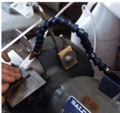
Turn your dry grinder into a wet one. Misting devices spray a steady stream of water to cool the tool and to keep grinding dust to a minimum. This one runs on a supply of water from a plastic jug and air from a compressor set at 80 to 90 psi.
