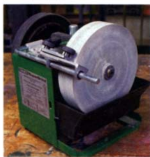
Sharpening a curved gouge on the Tormek. The carving-tool jig shown here steadies the blade of this curved gouge as it is rolled against the wet wheel.
