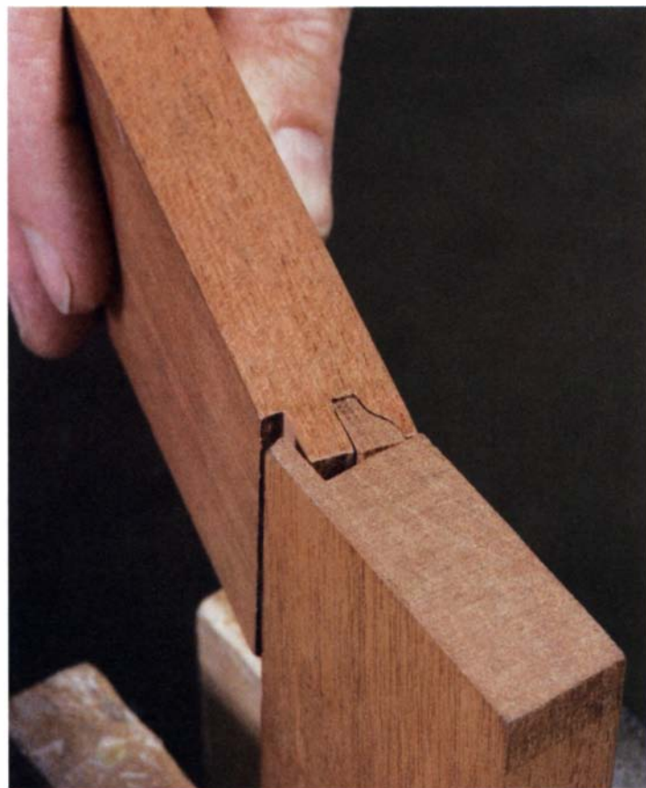
Where cope-and-stick joints fail. The molded edge, which has been reduced in thickness, is a weak spot in this joint. That's why it's a good idea to glue plywood panels into the grooves of the door frame, which will produce a much sturdier door overall.
