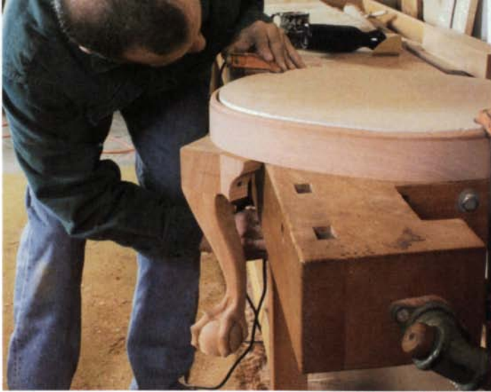
Temporary fixing. With the ball and claw complete, prepare to carve the knee by dry-fitting the leg to the frame. Use screws through the knee blocks to hold the leg in place.
