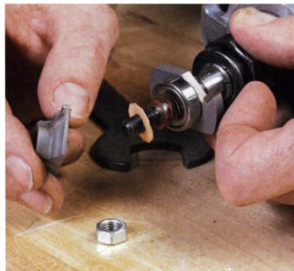
Reversible bits are adjusted by using shims. A good-fitting coping and snug-fitting stub tenon require some trial-and-error when adjusting the distance between the cutters.
