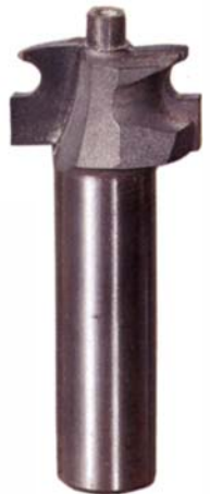
A finer quirk. The author honed the quirk cutter on the router bit at right to achieve a finer quirk.
