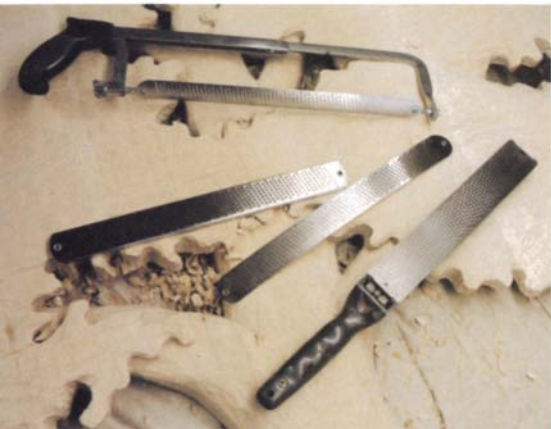
Microplanes cut and shape wood. Standard hacksaw frames and Surform handles will work with Microplane inserts.
