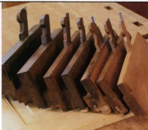
Beading plane. Antique beading planes are relatively inexpensive and widely available. They come in a range of sizes—one profile per plane—and cut straight runs of nearly polished beads.
