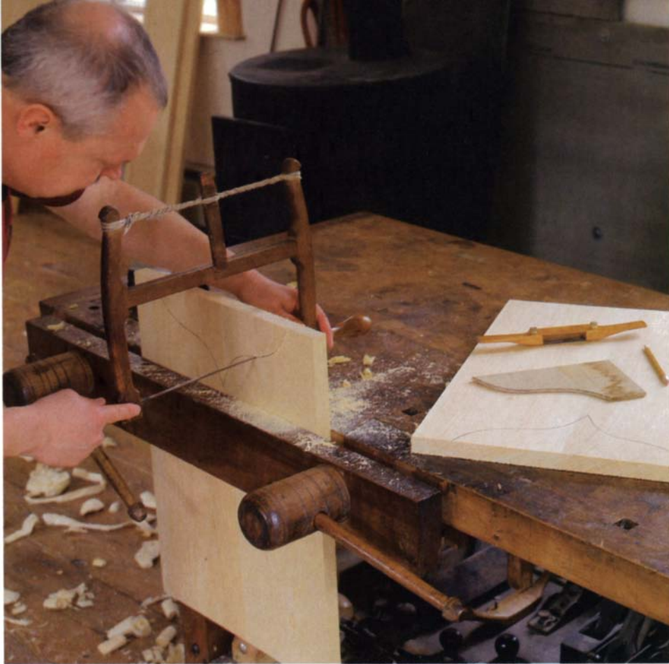
Bowsawed boot jack. A plywood half pattern, seen on the uncut panel, is used to trace the boot-jack end that forms the blanket chest's feet. If the bowsaw jams in the cut, pop out the waste piece with a chisel blow to the panel's end grain.
