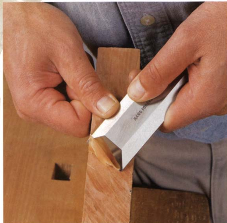
Polished to a mirror surface. Polishing both surfaces of a cutting edge eliminates minute scratches that will impair the edge's ability to sever wood fibers. Cutting end grain on old, dry cherry is a test for any edge.
