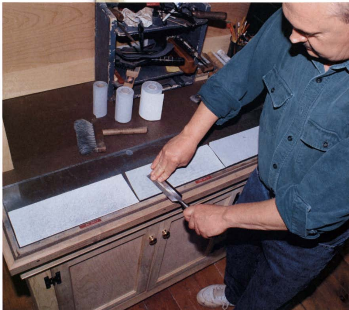
The author uses sandpaper and a piece of glass to sharpen his tools. It's imperative that both sides of a cutting edge get sharpened. Here, the author sharpens the back of a chisel.
