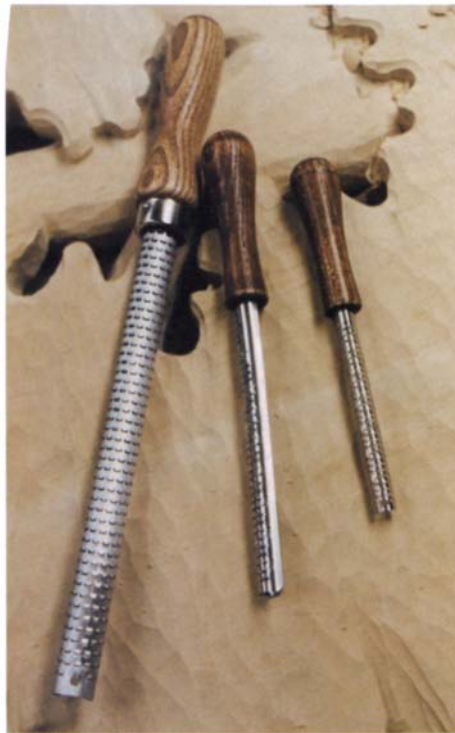
Quick-cutting rasps. Microplanes come in about a dozen shapes. They leave a finer surface than steel rasps do.
