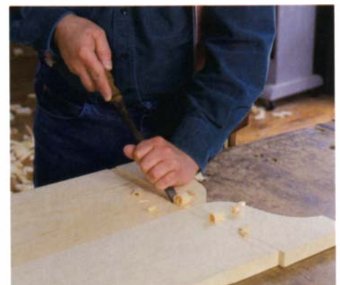
Scribe with a knife, then cut a dado with a chisel. Soft white pine, used for this chest and for thousands of similar antique versions, cuts easily with sharp hand tools. After a little chisel work, scribe again with the knife to cut cross-grain fibers until the dado is ½ in. deep.
