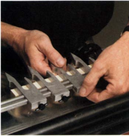
Porter-Cable's Omnijig has an optional variable-spacing template available. Adjustable fingers, which cut both pins and tails, slide along a pair of clamping bars.
