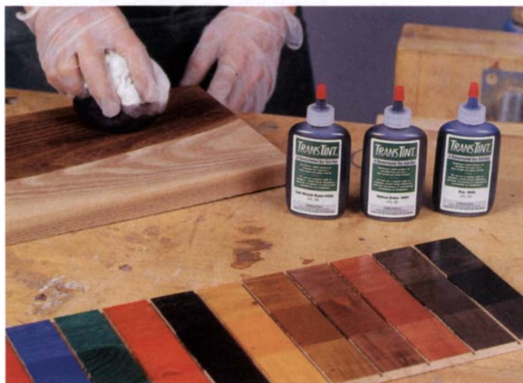
Liquid dyes. TransTint dyes, which are available in wood tones as well as in primary colors, resist fading.
