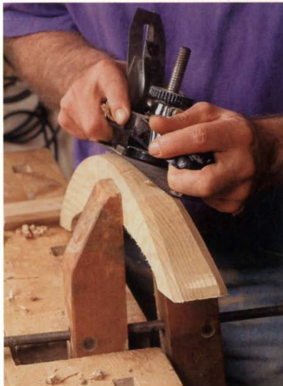
A little more sole. For cutting a true radius like this round tabletop, the compass plane is set very close to the radius of the circle and rides on more of the sole.
