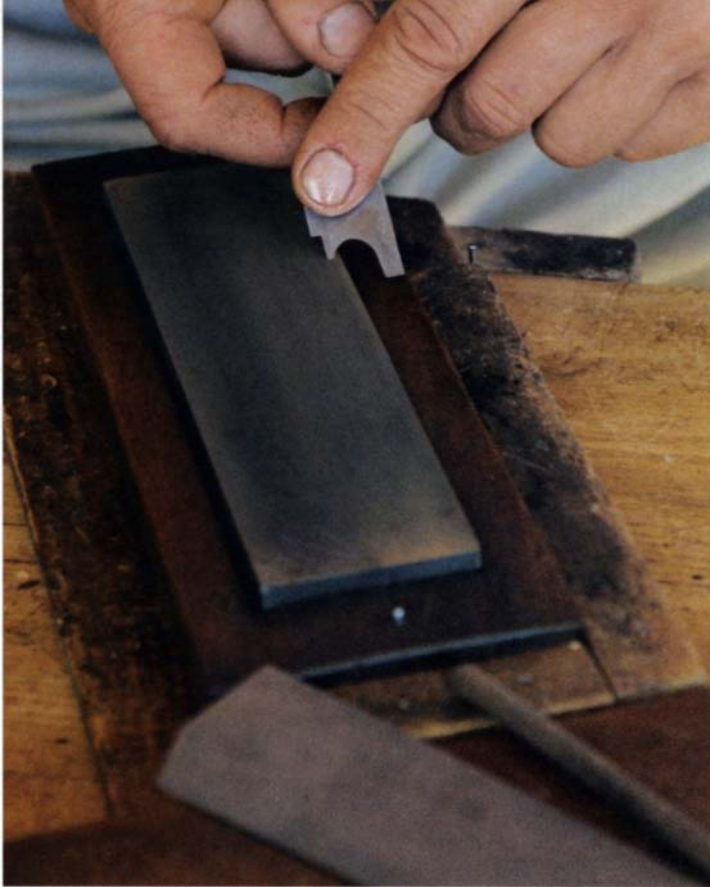
Think of a quirk cutter as a miniature plane iron. Sharpen the bevel of the quirk-cutting portion of the iron on a stone, as you would a plane. Sharpen the curved section that cuts the bead itself with round and knife-edged slip stones (bottom of photo).
