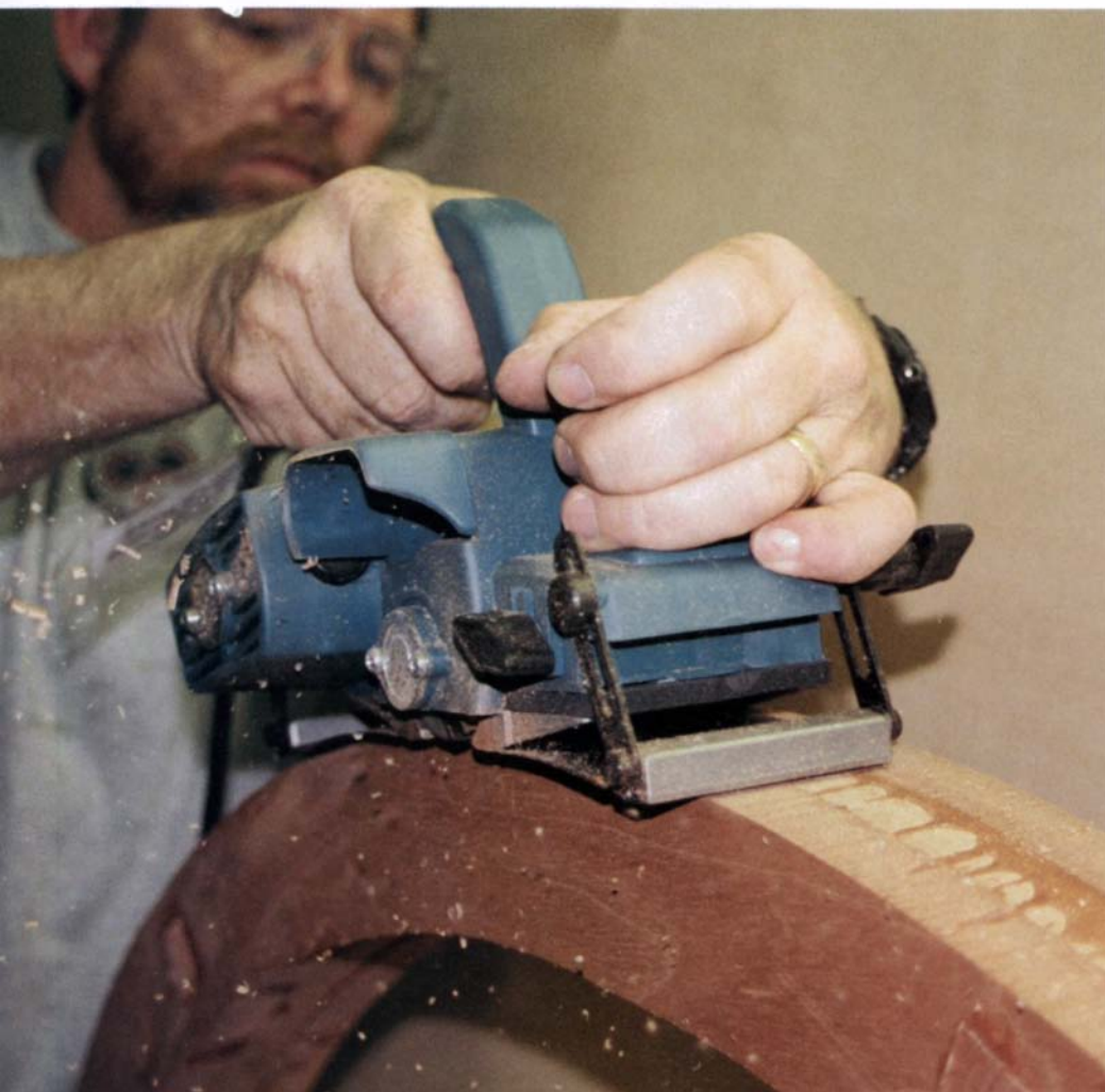
Fair that curve. The Virutex curve planer has an adjustable sole plate. It will cut concave radii as tight as 17\frac{11}{16} in. or convex radii as tight as 16\frac{3}{4} in.
