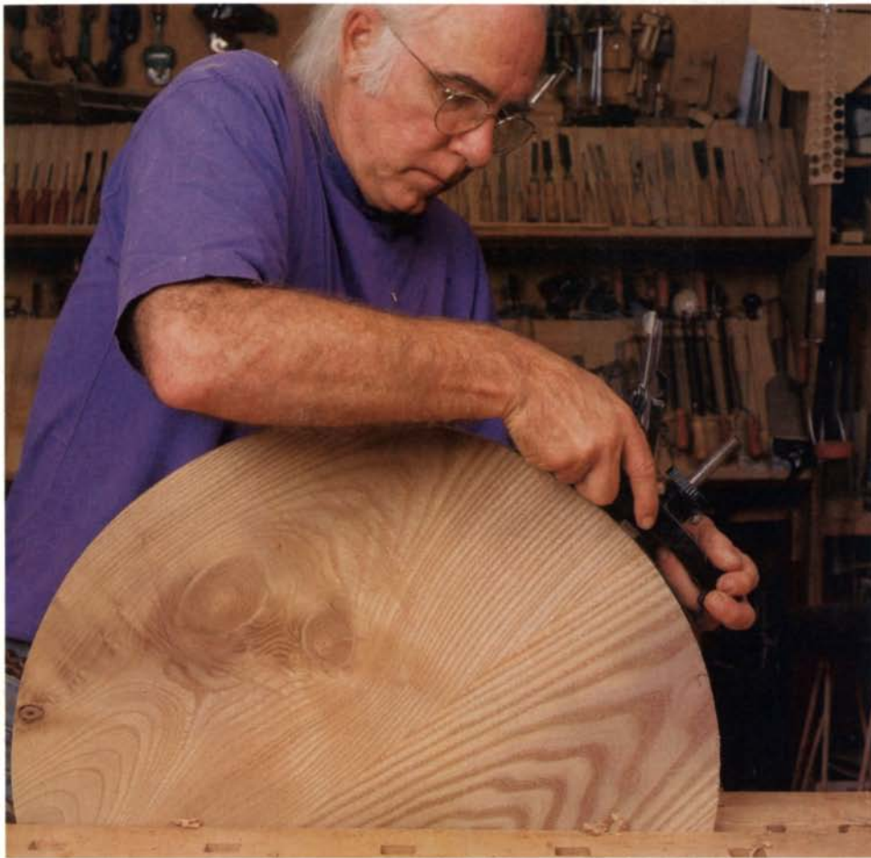
A little more sole. For cutting a true radius like this round tabletop, the compass plane is set very close to the radius of the circle and rides on more of the sole.
