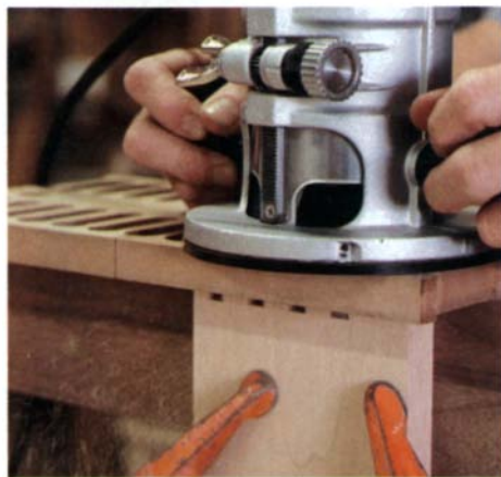
Using the Stots jig is slow work. The router must come to a complete stop before moving on to the next pin or tail cut.
