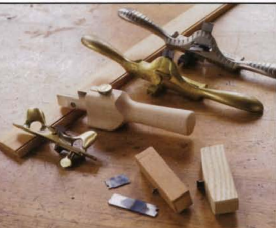
Beading tool. All beading tools work with a scratching action. Front to back: two shopmade scratch stocks, Woodcraft's bronze beading tool, the Veritas beading tool, Lie-Nielsen's bronze beading tool and a Stanley No. 66.
