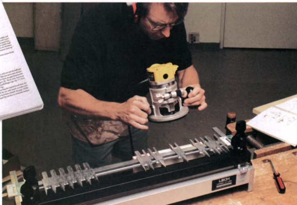
For variably spaced joints, the Leigh jig gives you the most flexibility. But there's a steep learning curve, requiring you to do lots of reading and to have lots of patience.
