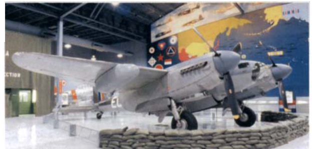
The “wooden wonder.” This British-designed World War II plane, called the Mosquito Bomber, was constructed mostly from wood and bonded with urea formaldehyde glue, which had just been developed.
