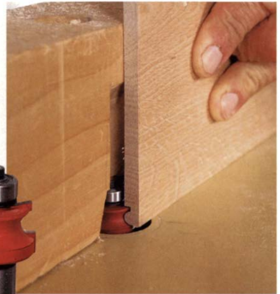
A finer quirk. The author honed the quirk cutter on the router bit at right to achieve a finer quirk.
