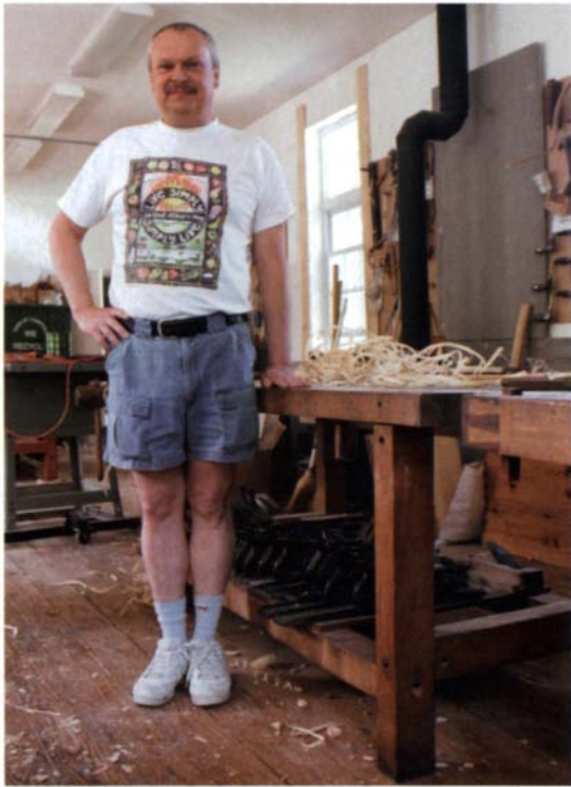
Get the height just right. To determine the proper workbench height, stand with your arm hanging by your side. Bend your wrist so that your palm is facing down.
