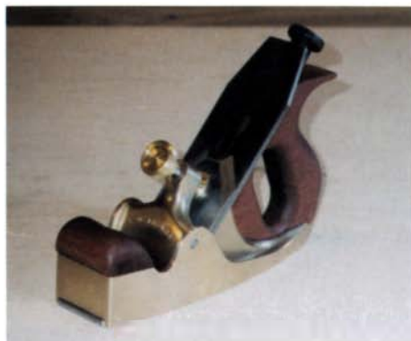
Diamond in the rough. Stephen Thomas machined the plane of his dreams from a rough casting made by The St. James Bay Tool Co.
