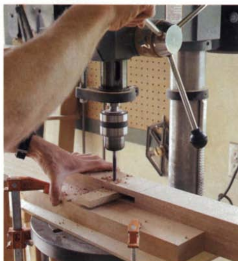
Temporary tenon. A scrap the same thickness as the tenon fills the mortise to prevent tearout as the holes for the pegs are drilled.
