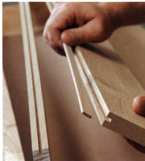
A continuous spline will also register adjoining boards. The spline should be of the same species, with the grain running in the same direction as the panel.
