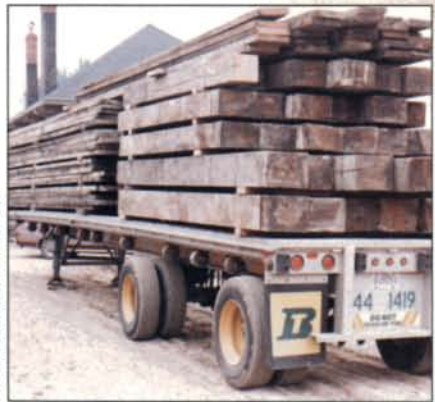
Old timbers, new uses. Original heart pine posts and beams provided the skeletal framework for factories up and down the East Coast. The pile on the back of this flatbed truck was salvaged from an old mill building in Lewiston, Maine, and made into flooring.
