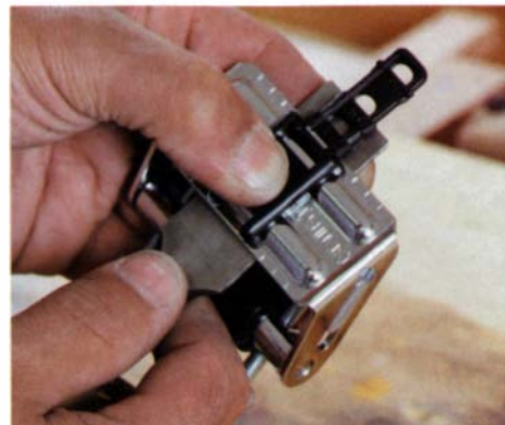
A built-in angle guide makes it easy to position a tool to this guide.
