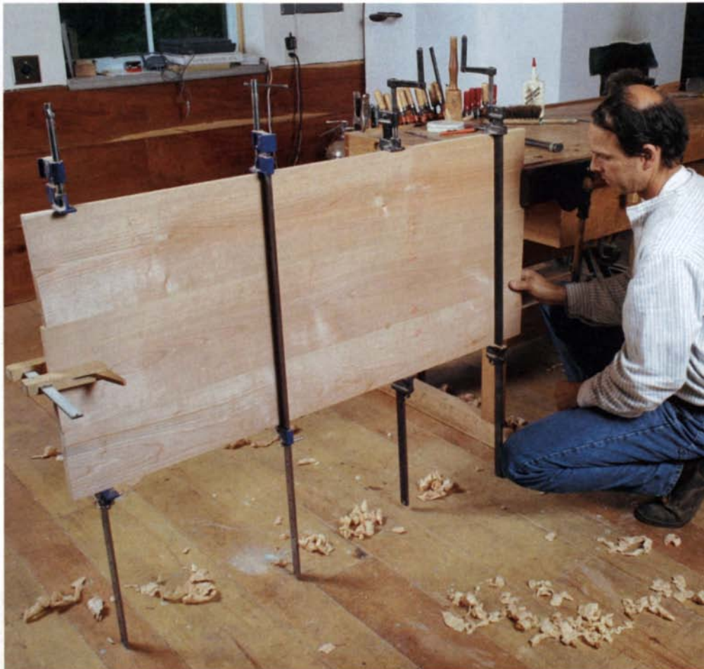
Garrett Hack glues up tabletops using his bench vise. With one board clamped in the vise, he applies glue and stacks the remaining boards in place. Next he applies bar clamps, beginning at the outboard side of the workbench. At the halfway point, he repositions the panel in the vise, allowing the clamps to rest on the floor for support. The remaining clamps are applied with only about 1 in. of the panel gripped by the vise.
