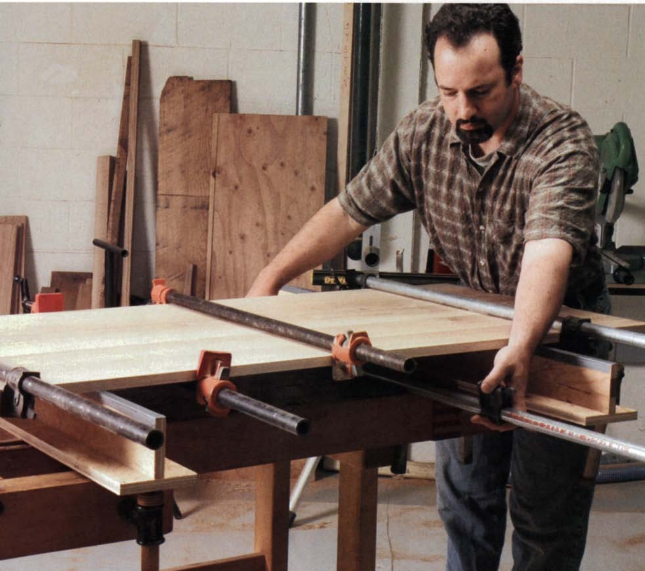
T-supports are made of plywood scrap. With the workpiece lifted a few inches off the bench, T-supports make it easy to slide clamps under the boards without lifting them. Duct tape applied to the supports keeps them from sticking to the workpiece.
