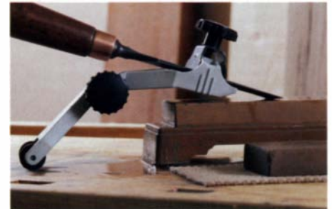
The General is the only guide that rests on and off the stone. The tool is hinged so it can be adjusted for stones of different heights.
