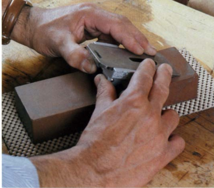
A good grip is important. A six-fingered grip provides stability and good feedback so that you can tell immediately whether a tool has slipped in the guide.
