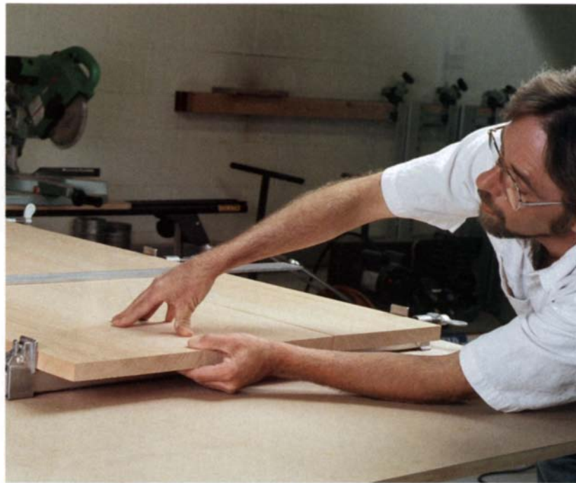
When clamping a tabletop, apply light pressure first. Run a finger across the edge-joints, and feel for ridges. A tap of the fist or a dead-blow mallet is all it takes to align boards.
