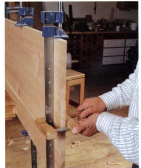
Lightweight cam clamps can be used to hold boards flat against bar clamps.
