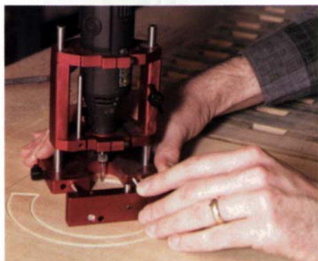
The first plunge-router base for motorized tools. Guitar maker Bishop Cochran sells an extruded aluminum plunge-router base for Dremel, Ryobi and Foredom motorized tools.
