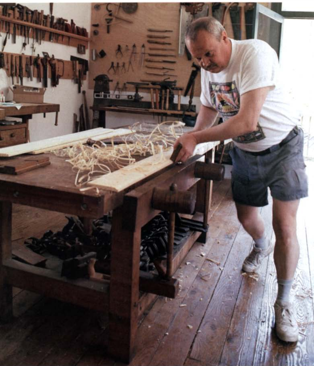
Low bench for handwork. Planing moldings, chopping mortises and jointing boards all require lots of upper-body strength. A low bench—the one in the photo is 31 in. high—allows the author to put a lot of muscle into his motions.
