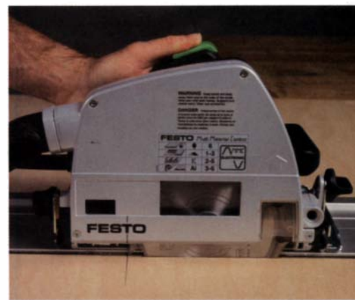
Circular saw from Germany. Festo's plunge-cut circular saw is equipped with speed control, an electronic brake and an efficient dust-collection design.
