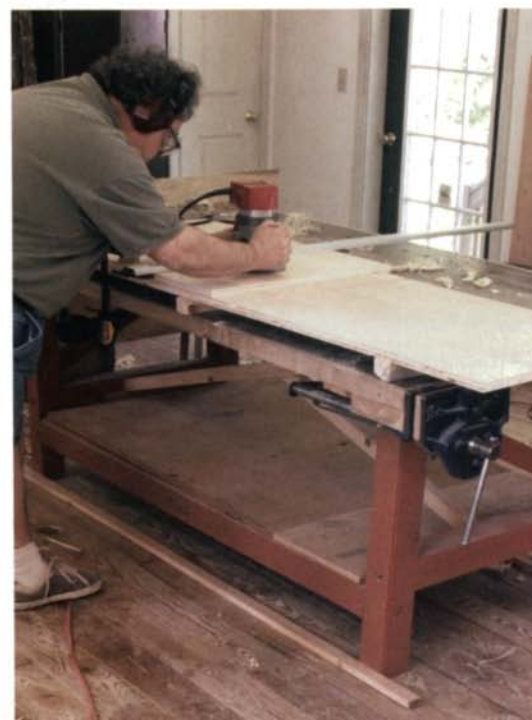
Low bench for handwork. Planing moldings, chopping mortises and jointing boards all require lots of upper-body strength. A low bench—the one in the photo is 31 in. high—allows the author to put a lot of muscle into his motions.
