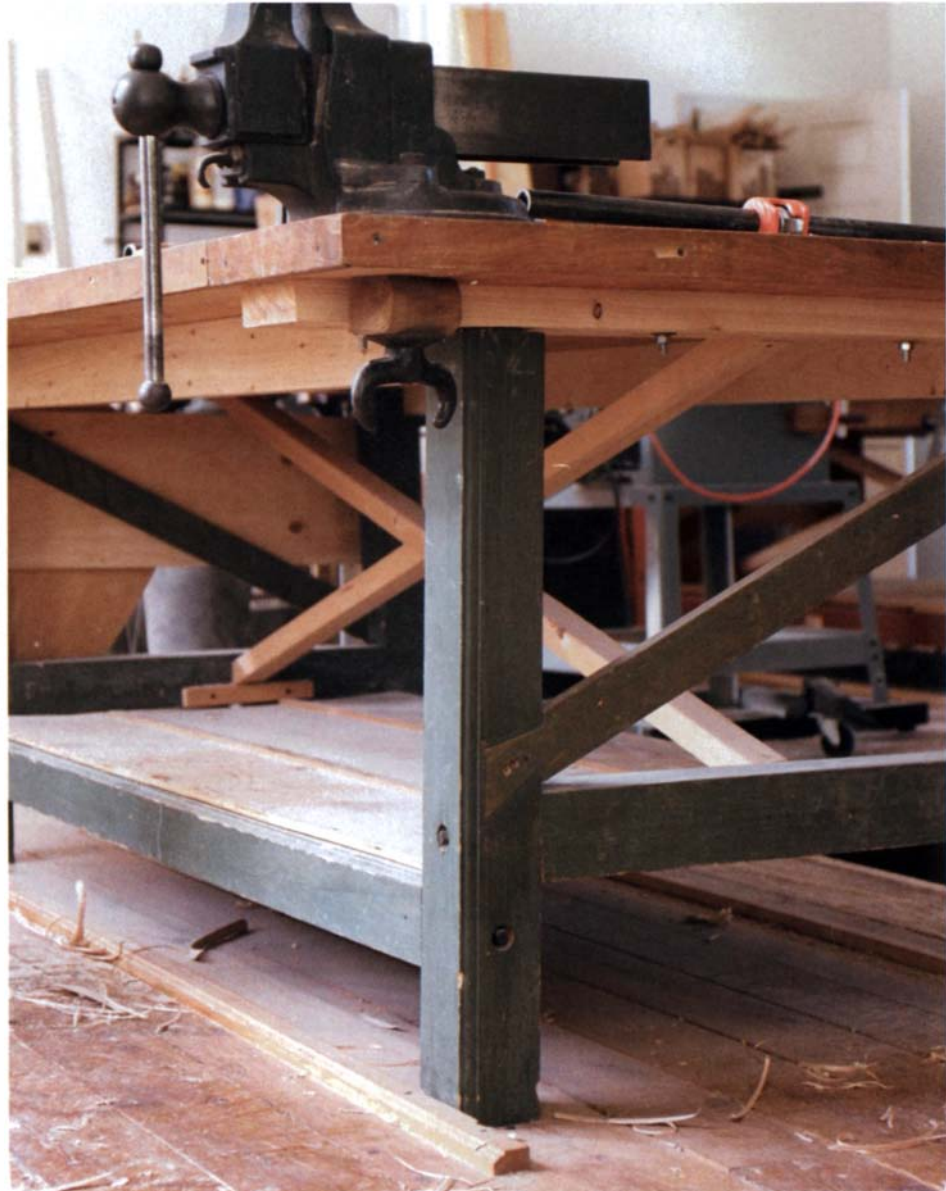
An immovable beast. To keep his benches from racking, the author uses dovetailed diagonal braces. Cleats screwed to the floor prevent the benches from moving.
