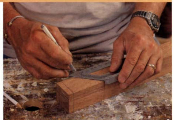
After the initial marking with a sharp pencil, I use an Exacto knife and marking gauge to lay out the joint. I make sure my layout is accurate because I must rely on it as I cut the joint: There are many intermediate steps when it is not possible to do a trial-and-error fit.
