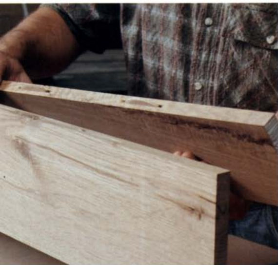
Biscuits won't guarantee a perfect glue-up, but they do make it easier to keep boards in alignment.
