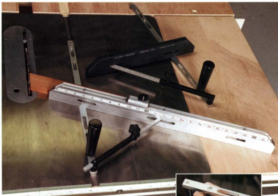
Reinventing the miter guide. Two types of fences are available with the Osborne Manufacturing miter guide: a 15-in. nylon fence and a 25-in. aluminum fence with a flip stop. Detents in the underside of the extension arm provide positive stops for frequently used angle settings.
