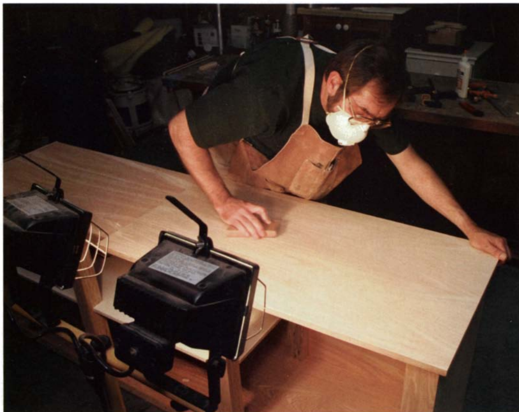
Let there be light. A strong, raking light illuminating the workpiece from a low angle, works best to reveal scratches that need attention. The author uses a tripod-mounted, 1,000-watt quartz halogen light.
