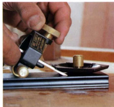
A large, easy-to-tighten hold-down knob and a wide roller make a secure, stable honing guide. An angle-setting gauge with five presets can be purchased separately.
