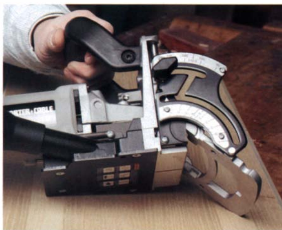
Porter-Cable has a new biscuit joiner. The fence on the model 557 biscuit joiner adjusts from 0° to 135°.
