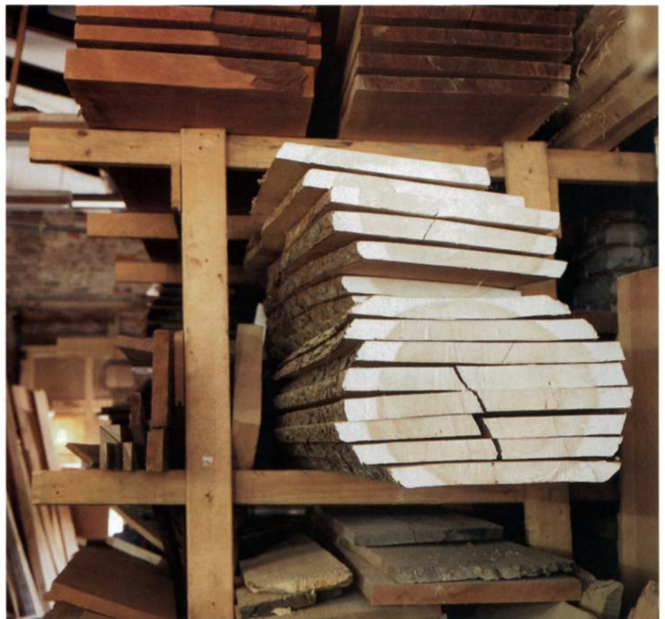
Built to last. Kelly Mehler has used the same basic rack for more than 18 years. He stacks boards in the order they came off the tree and often lets them dry for a year or more.
