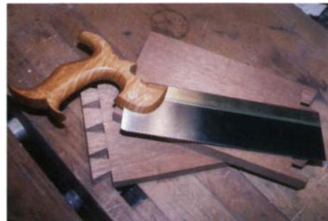
Independence Tool's hand-crafted saw. The dovetail saw is modeled after an 1830 British backsaw.
