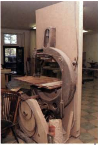
Saving a tool. The author's bandsaw was bought from an old warehouse for $40 and then reworked. The author made a plywood case for the bottom and used old sash weights to counter-weight the guide post, making it easier to adjust.
