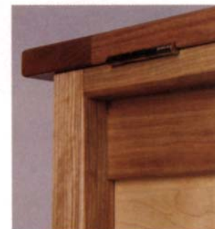
A filler strip holds the hinges. The strip is glued to the rear top rail and butts against the rear legs, whose inside back corners remain unchamfered.
