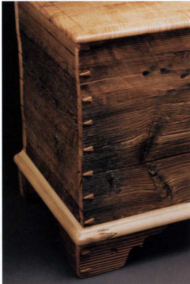
Texture supplied by wheat. Arvid Lyons places lumber recycled from old barns inside grain chutes. The abrasive action of tons of moving grain creates smooth ridges that follow the grain.
