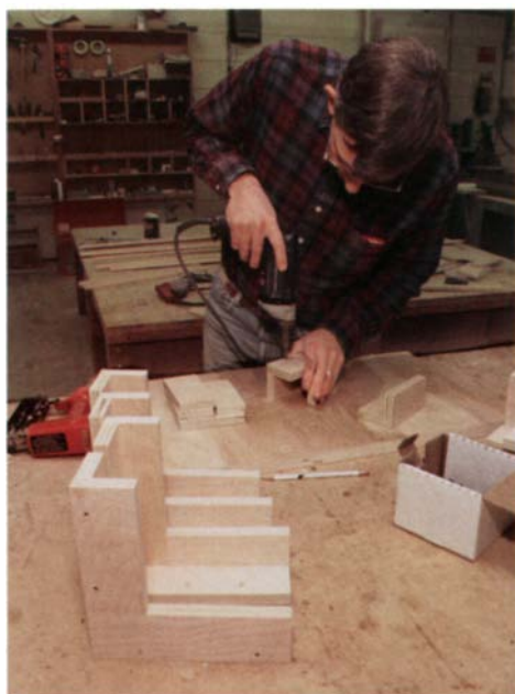
Shop-built brackets are easy to make square. The author mass-produces plywood brackets in the shop, using the tablesaw, an air nailer and a screw gun. Pieces are butt-joined at the corners with glue, nails and screws.
