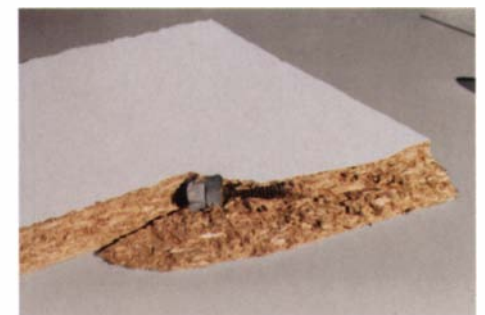
A surprise find in a sheet of melamine. Israeli woodworker Reuven Spiers cut into a nut and bolt that was buried in a sheet of fresh melamine.
