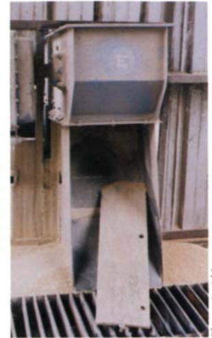
Texture supplied by wheat. Arvid Lyons places lumber recycled from old barns inside grain chutes. The abrasive action of tons of moving grain creates smooth ridges that follow the grain.
