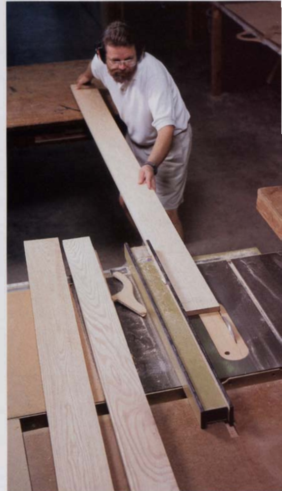
Cut joint-ready edges on a tablesaw, p. 82
