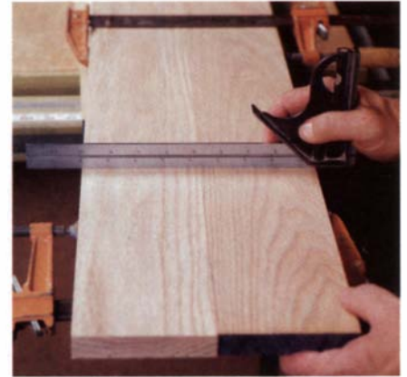
A clean joint line fresh from the table-saw. Sawn edges without further preparation can make perfectly good glue joints.
