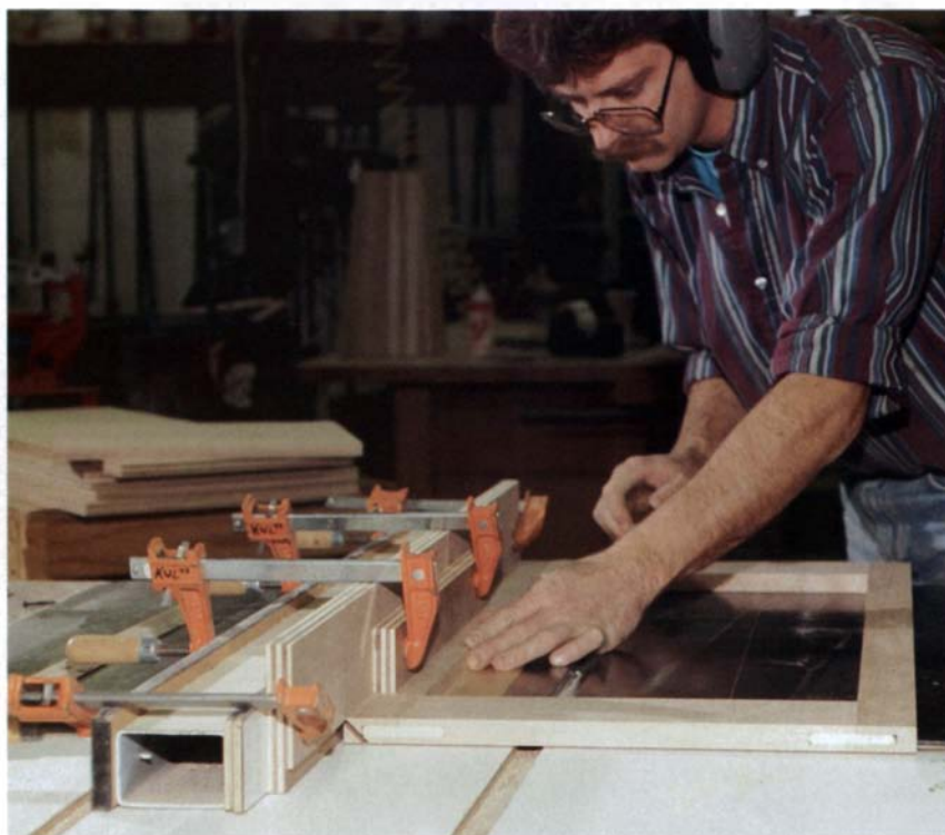
Miter all sides of the stock. The miter cuts are made by pushing dimensioned stock along an auxiliary fence fitted with a hold-down covering the blade and a recess for the offcut. The blade is partly buried in the auxiliary fence.
