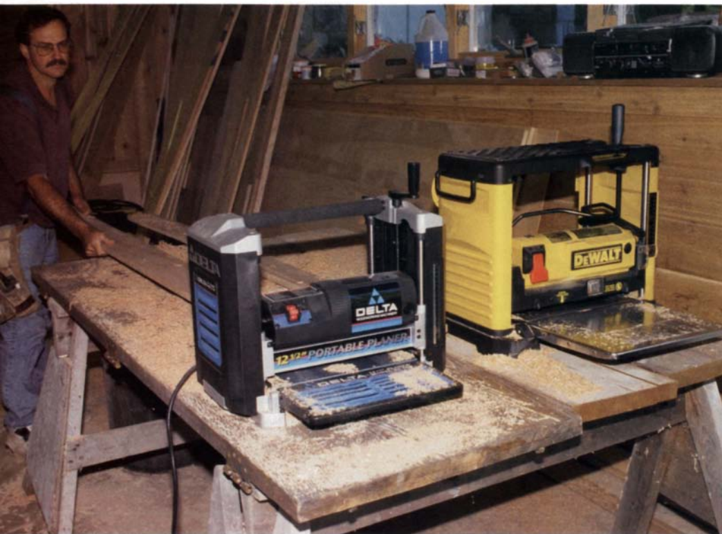
Improved benchtop planers. Delta and DeWalt 12½-in. planers have cutterhead locks, which help reduce snipe. Both machines leave a good finish.
