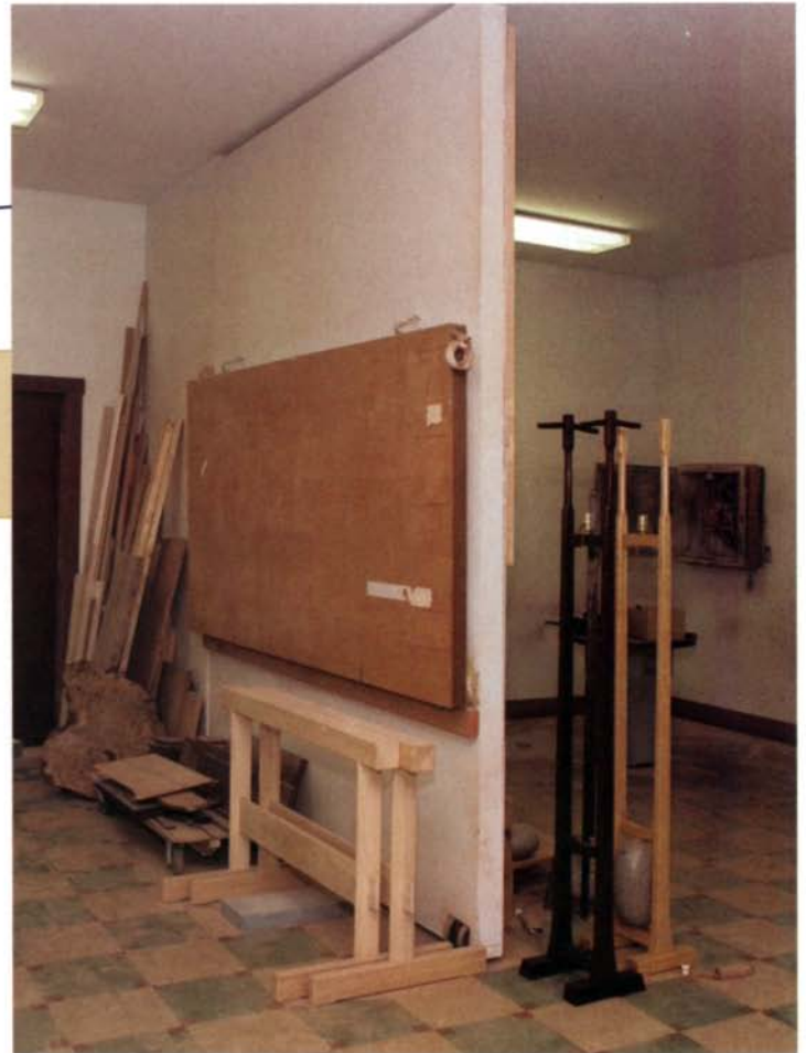
Small touches add comfort to a shop. With the author's vacuum press folded away in the movable wall, you see that a quick paint job on a simple particleboard floor breaks up the monotony of a shop. Beneath the particleboard are 2x4 sleepers and radiant-heat tubing that comes out at his feet, where it does the most good.
