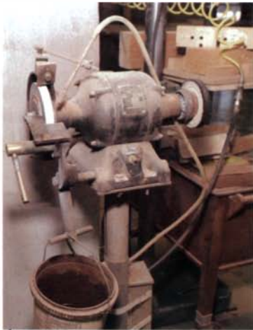
Mister keeps tools cool. Powered by compressed air, this mister blasts coolant from the reservoir onto the grinder pedestal and leading edge of the tool being ground, preventing the tool from being burned.
