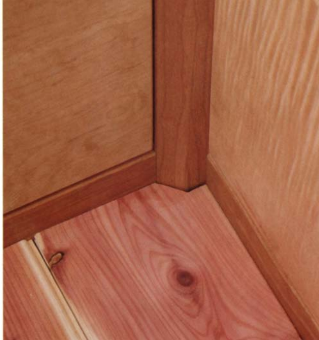
Ledger strips support a plywood bottom panel painted with odorless milk paint (above). A liner of tongue-and-groove aromatic cedar (right) is glued on top of the plywood and is notched to fit around the legs.
