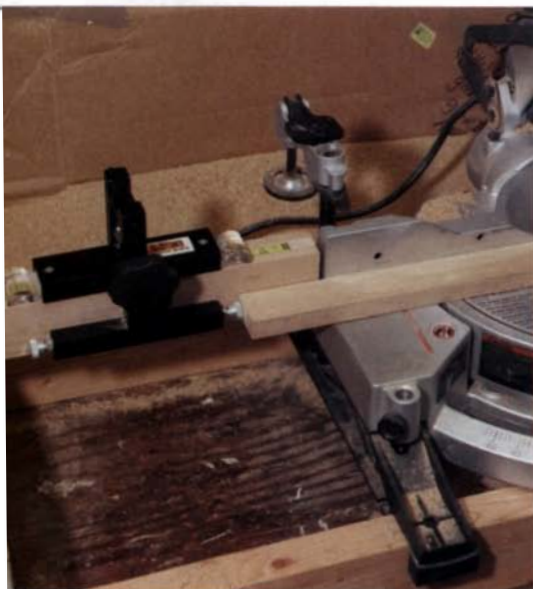
A gauge for stopped cuts. The Broset Precision Stop Block works with chop saws, radial-arm saws and tablesaw crosscut boxes.
