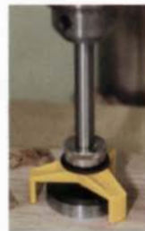
Depth control. SlipStop fits over the shank of a Forstner bit, simplifying controlled-depth cuts.
