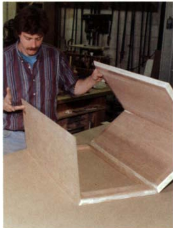
After flipping the case over, spread glue on the exposed miters. Then fold the case into a box, and tape the fourth corner.
