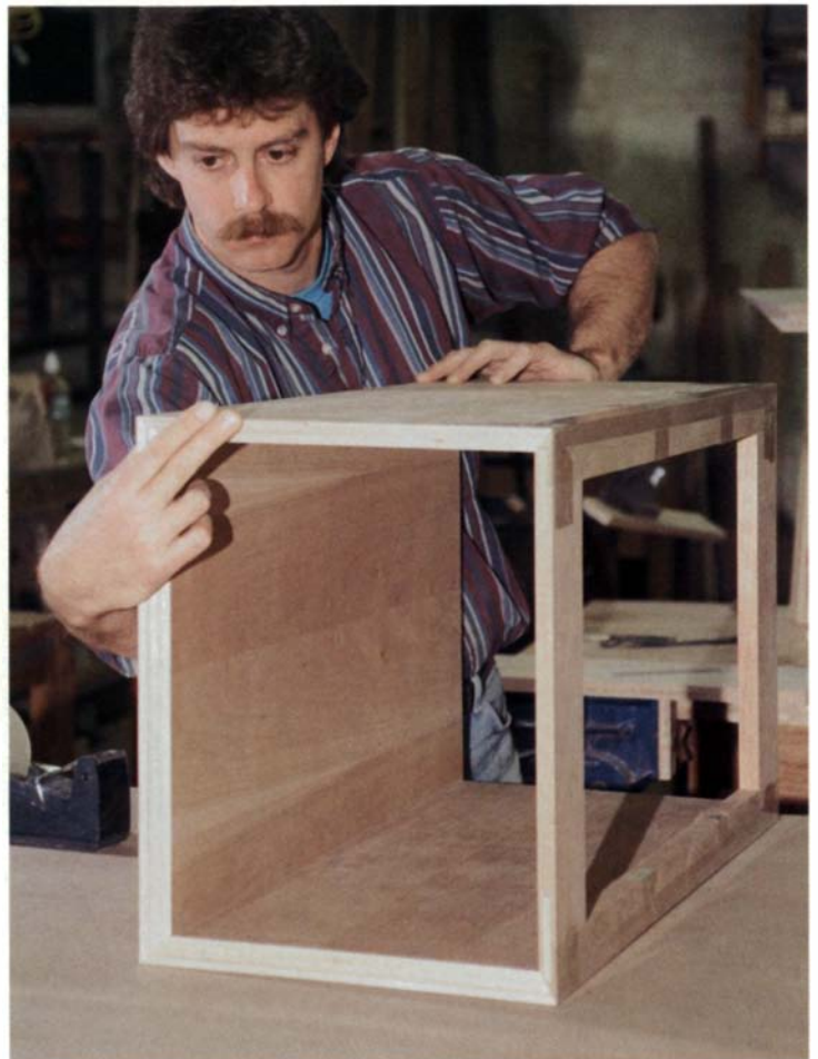
Make sure the corners are flush. Last, tape the top and bottom pieces in place.
