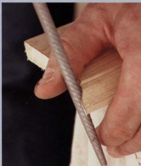
Undercutting with a rasp
