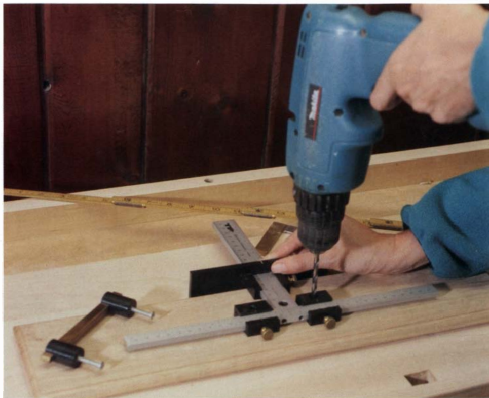
Hole-boring jig for hardware. The True Position drill guide simplifies aligning shelf pins and drawer and door pulls. It can also be used as a guide for 32mm cabinet construction.
