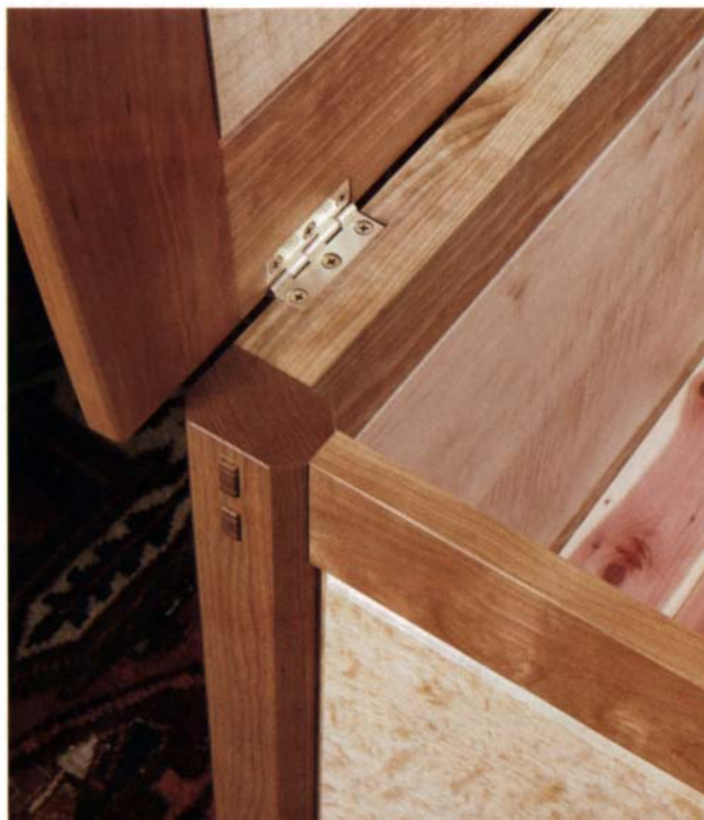
A filler strip holds the hinges. The strip is glued to the rear top rail and butts against the rear legs, whose inside back corners remain unchamfered.
