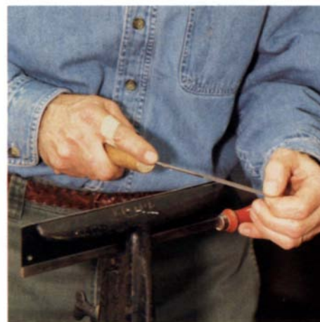
Sharpening a backsaw is a skill. A single pass will sharpen the teeth on this dovetail saw. Each stroke has to be even to keep the teeth uniform.
