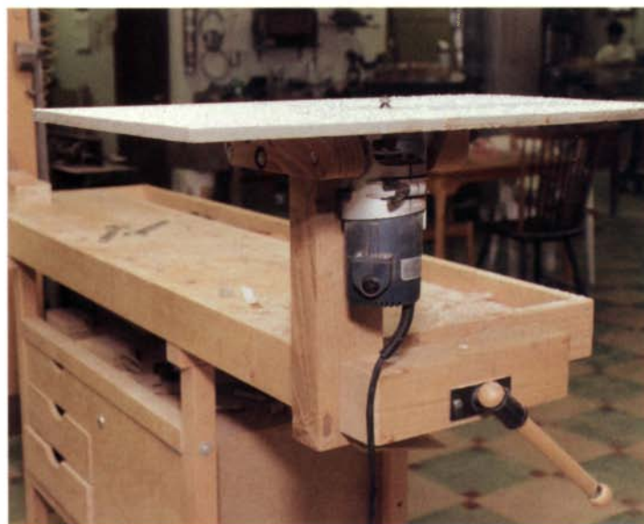
A disappearing router table. Built for convenience, the author's router table can be clamped in a bench vise and ready to use in seconds. It stores out of the way just as quickly.
