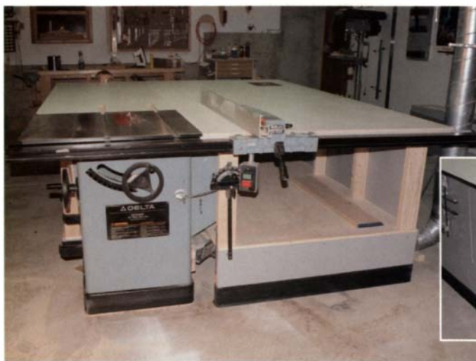
This tablesaw platform can handle anything. Greg Colegrove's massive outfeed/extension table also serves as a router table and has plenty of room for storage.
