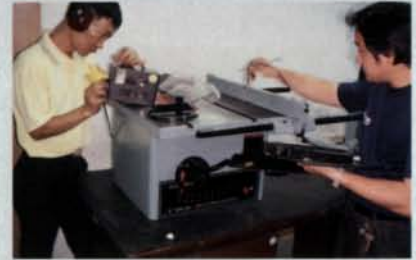
Delta inspectors at work—Vibration and noise level measurements are among quality control checks performed on tablesaws.
