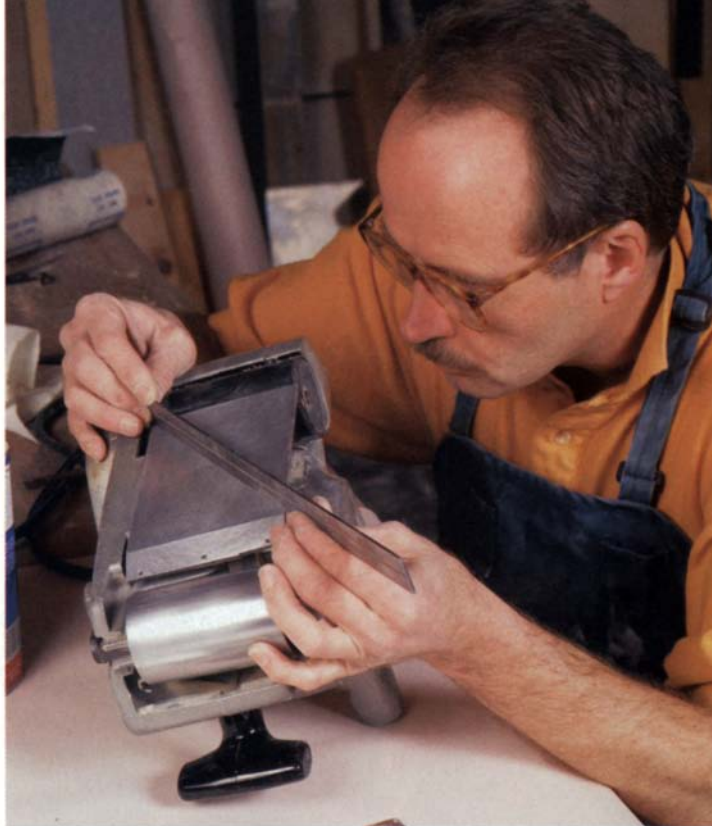
Is it flat? The author checks the platen of a belt sander with a straightedge. High spots should be filed off.
