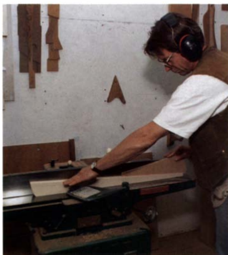
Jointer cleans up tapers quickly. A few light passes over the jointer should clean up any mill marks or other surface irregularities left after roughing out a leg by machine.
