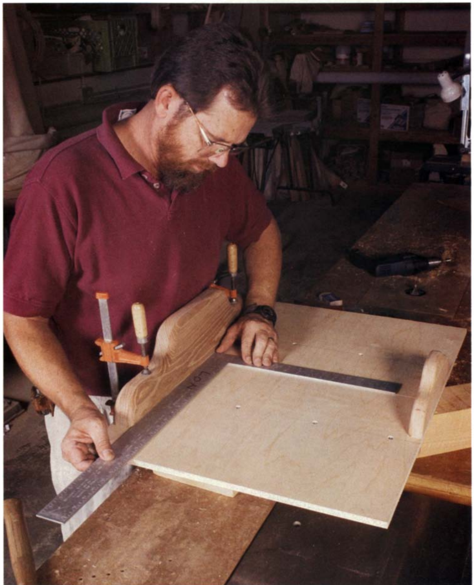
Square the fence to the sawkerf. Check the fence's alignment from both sides of the kerf. Attach the fence with only two screws before you make trial cuts.
