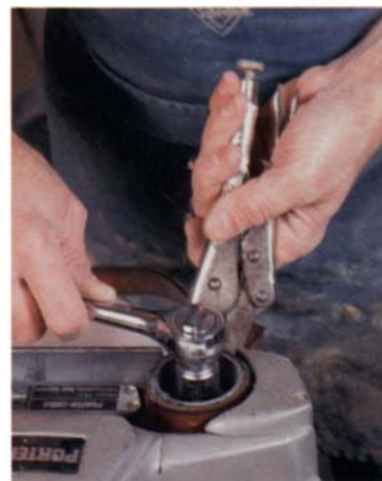
Hold still. An old leather belt and a pair of Vise-Grips hold the rubber drive wheel as the author backs off the axle nut (above). Tire-traction compound improves the grip (right).
