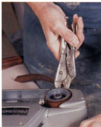
Hold still. An old leather belt and a pair of Vise-Grips hold the rubber drive wheel as the author backs off the axle nut (above). Tire-traction compound improves the grip (right).
