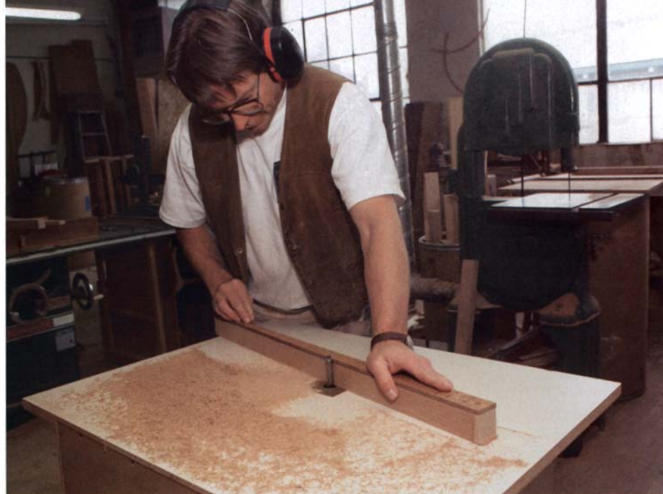
Template routing ensures consistent results. Both bottom-bearing bits (shown above) and top-bearing bits work. Double-faced tape secures the template to the legs.
