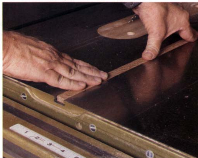
A perfect fit—Runner stock should slide freely in the miter slots (above). Finished runners should be just below the level of the table (right).
