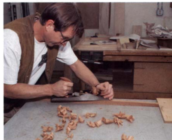
Handplane cleans tapers efficiently. A plane leaves a surface that's ready for finish, but take care to plane with the grain to avoid tearout.
