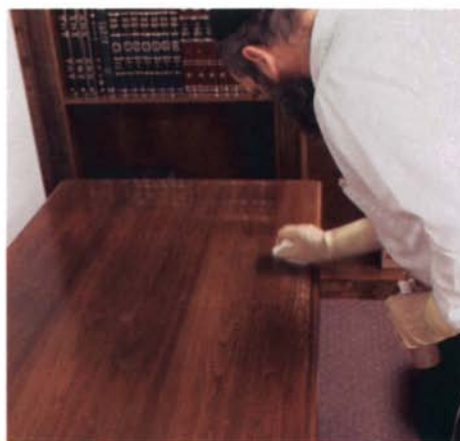
Padding lacquer applied by cloth— Applied with a quick, buffing motion, padding lacquer blends finish repairs and seals in alcohol-soluble dyes.
