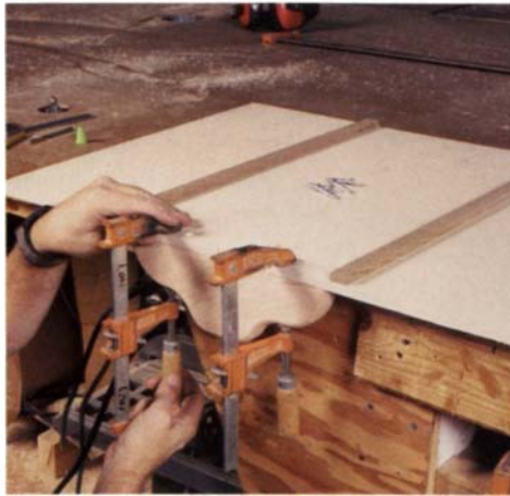
Don't cut that sled in half. After you attach the front brace (left), cut only two-thirds of the way through the platform (right). The kerf is a reference to set the rear fence.
