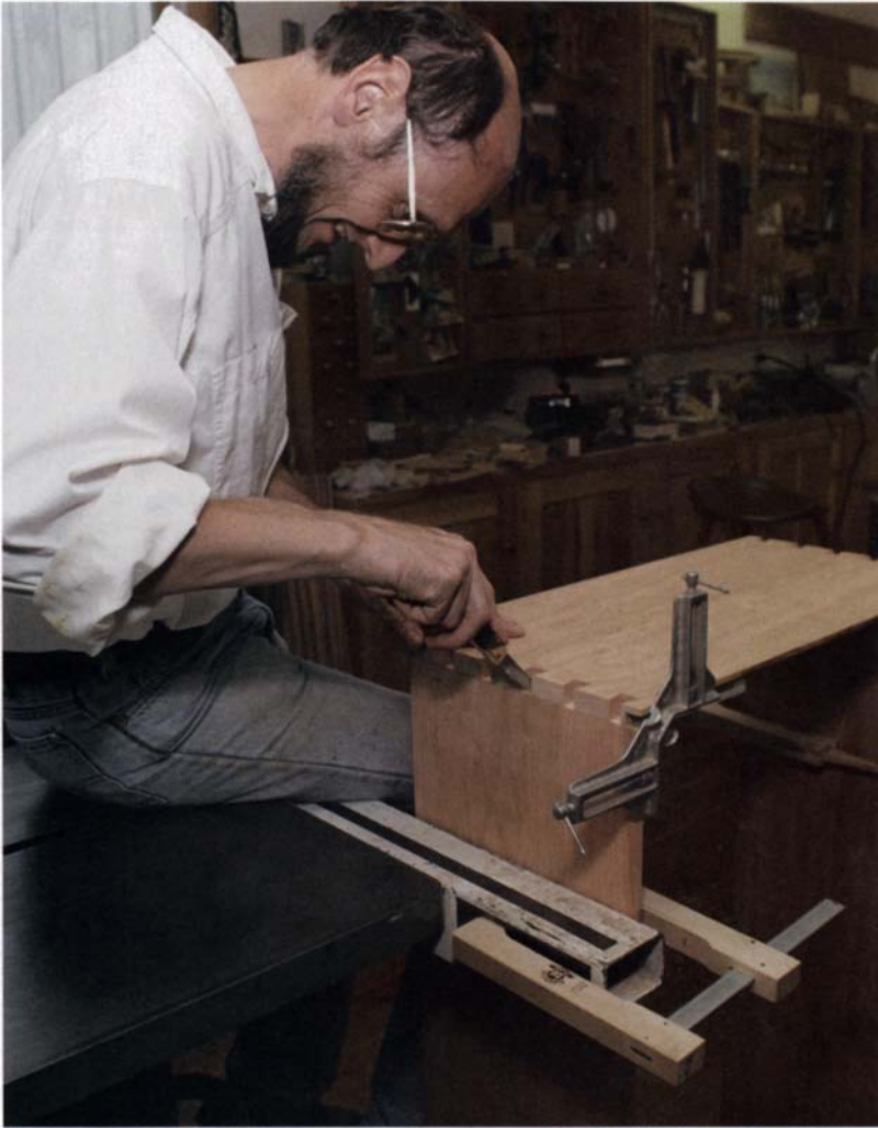
Picture-frame clamp keeps top and side at 90° for layout.
