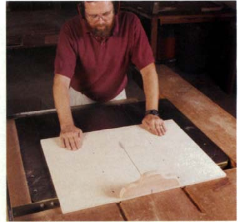
Don't cut that sled in half. After you attach the front brace (left), cut only two-thirds of the way through the platform (right). The kerf is a reference to set the rear fence.
