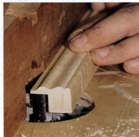
Cut a rabbet for the glass and back panel. After the molding is machined and ripped to width, cut a rabbet 3/8 in. wide by 1/2 in. deep.
