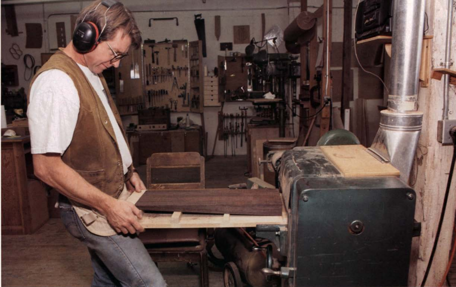
All four legs of a table can be tapered at once. The author's planer jig is made from a piece of \frac{3}{4} -in.-thick plywood and three angled strips of wood to support the legs. Stops at either end of the plywood keep the legs in place.
