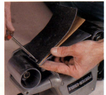
Graphite is cool. This self-lubricating product reduces friction and makes the belt run more smoothly, reducing stress on the machine.
