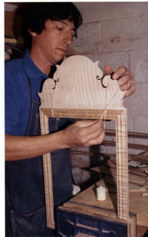
Clamp the fretwork to the frame. Rubber bands are great for holding the odd-shaped fretwork in place while the glue dries.
