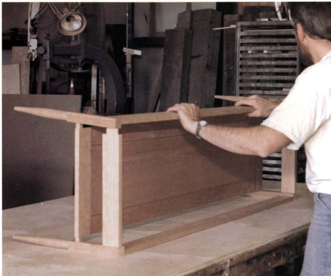
Don't skip the dry-fit. Gluing up all the table parts shouldn't be a nightmare. A dry run pinpoints problems while they can still be corrected.
