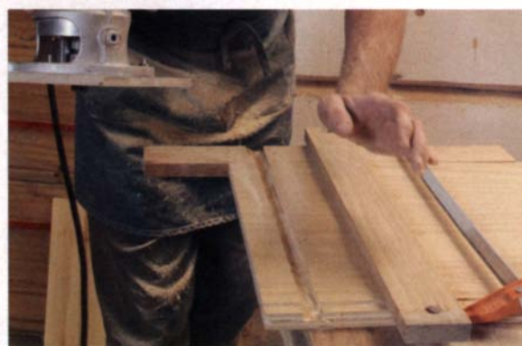
Shopmade T-fence for cutting dadoes—Screw two strips of plywood together at right angles to make a guide fence for cutting dadoes with a router.
