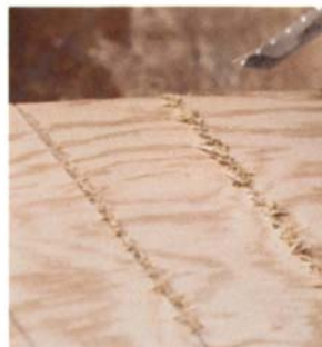
Orbital action —A switch sets the amount of orbital action (right). In non-orbital mode, the tool cuts slowly but leaves a clean kerf. In orbital mode, the saw cuts faster but creates tearout.
