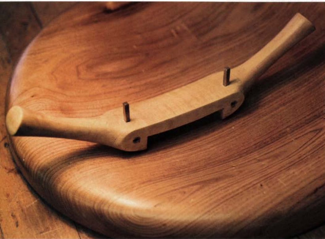
Travisher by Fred Emhoff —A retired tool-and-die maker manufactures these hand tools used for scooping out the seats of chairs.
