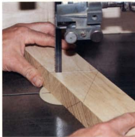
Divide body in two. Cut the center block to create the halves of the plane body—a forward and a rear block.
