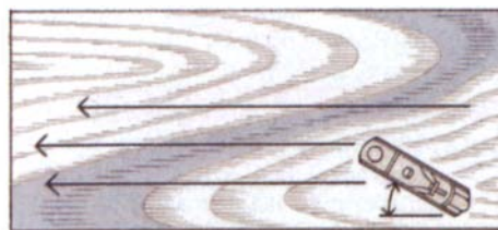
Plane the length of the board with the plane skewed at about 30°. Take very light passes with a freshly sharpened iron, and increase the skew around problem areas.
