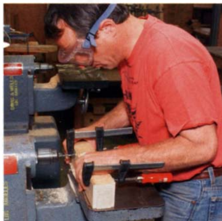
With blocks clamped, index the body. The author drills through the plane cheeks into the body to set the indexing pins.
