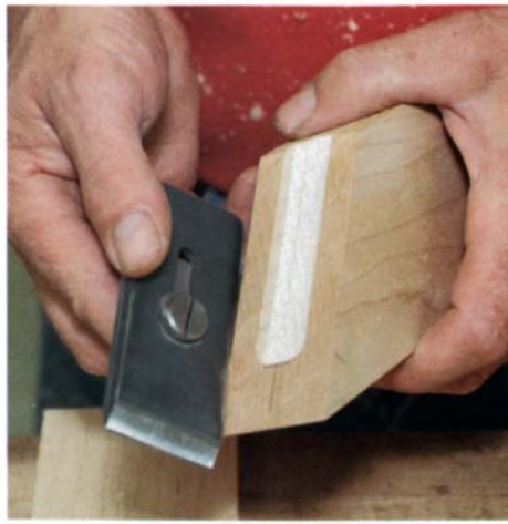
A slot for the cap screw—The rear block is slotted with a 3/4-in. router bit to accommodate the cap screw on the plane-iron assembly.
