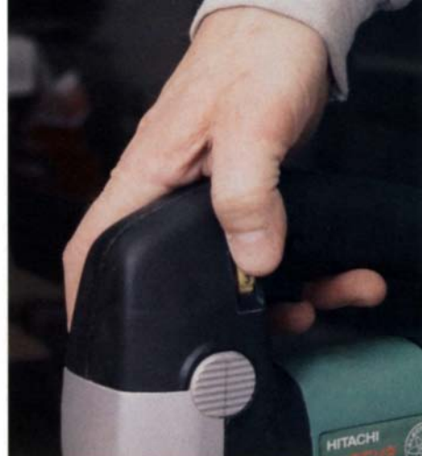
Difficult to get a grip—It takes some maneuvering on Hitachi's jigsaw to move the small, recessed speed dial.
