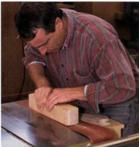
Easy does it. The author uses 120-grit sandpaper clamped to a flat surface to true up the sole of the plane. Using very light pressure, he sands only until the surface is uniformly abraded.
