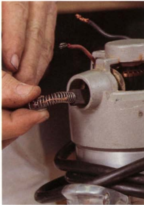
With cap removed, brush pops out. Spring-loaded brushes should come out of their guide channels easily once the end caps are out of the way.
