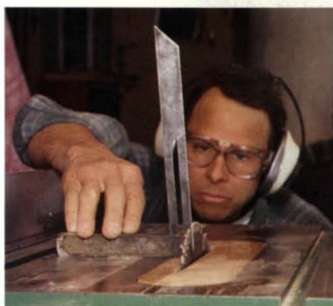
Transfer angles to the saw. The author uses the bevel gauge to set the tablesaw blade at the correct angle.
