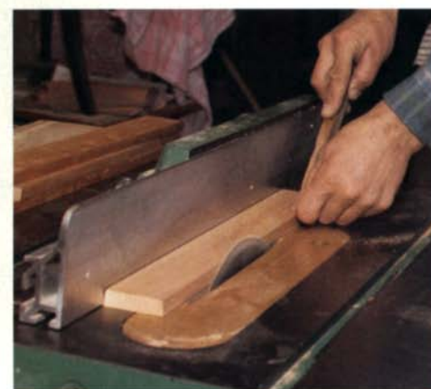
With the angle set, make the cut. Cut all the bevels of the same angle before changing the blade angle.
