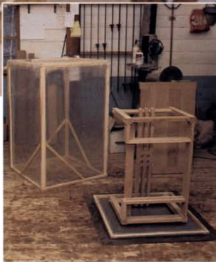
Fuming with ammonia gives white oak that classic golden-brown color. Before it's been fumed (inset), white oak is a pale, almost cool, tan.
