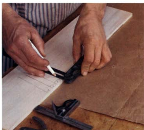
Record each angle. Use a bevel gauge to measure the angles on the drawing. Then record them on scrap.
