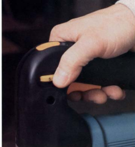
A good location for a speed-control switch—Makita's speed-control dial operates smoothly and is easy to reach.
