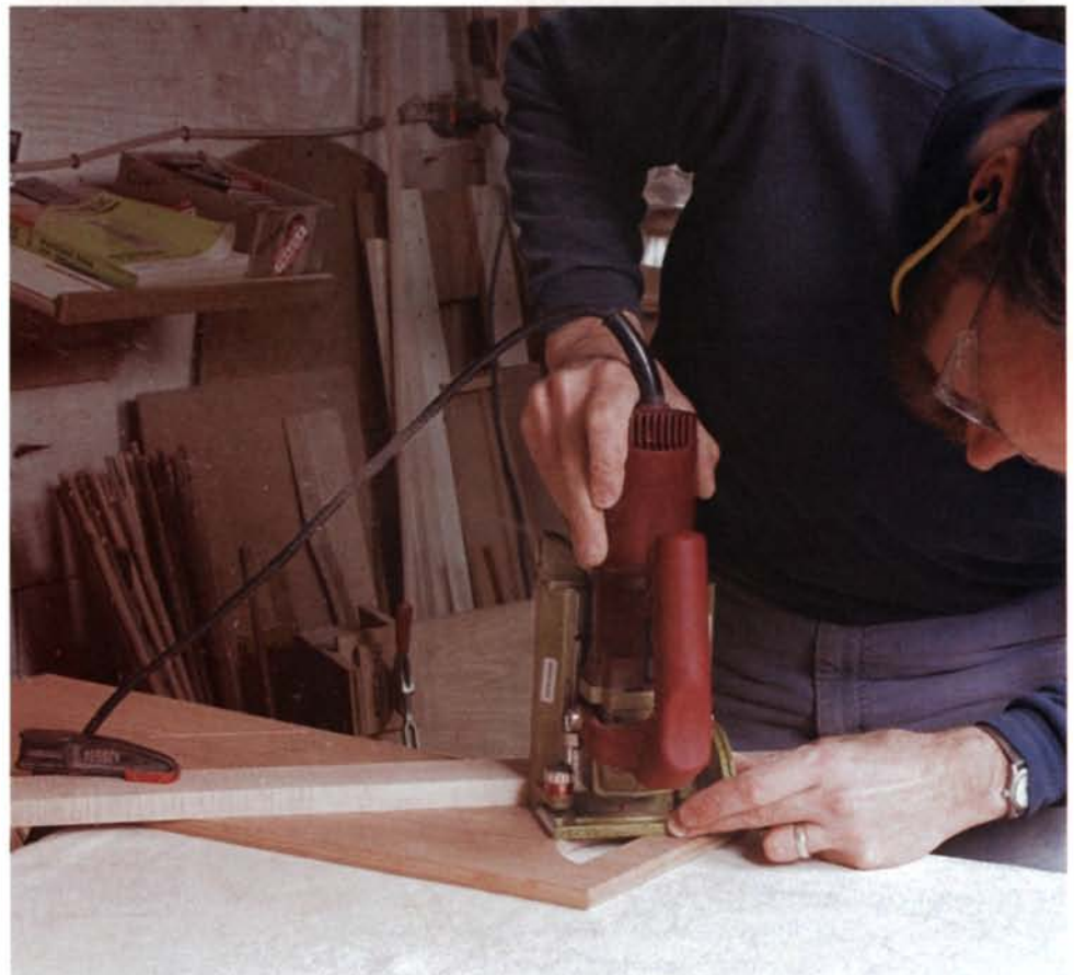
A straight board guides the biscuit joiner. The author places the base of the tool against a board clamped to the side to cut the slots for the shelves.
