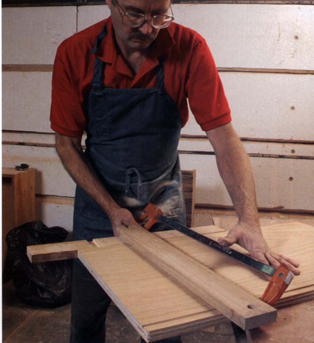
Shopmade T-fence for cutting dadoes—Screw two strips of plywood together at right angles to make a guide fence for cutting dadoes with a router.
