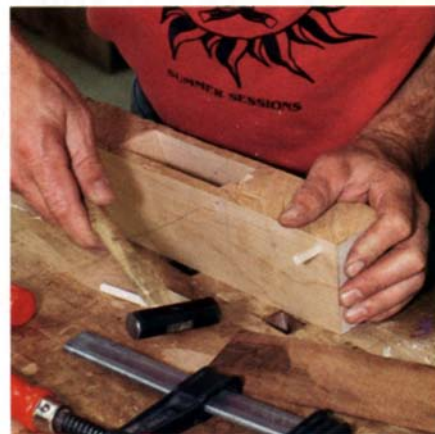
Index pins made of \frac{1}{4} -in. dowel hold plane parts in position during assembly. They will be cut off after the plane is finished.
