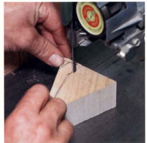
Save the wedge. The triangular offcut will be used later to make a wedge for the plane iron. Don't throw it out.
