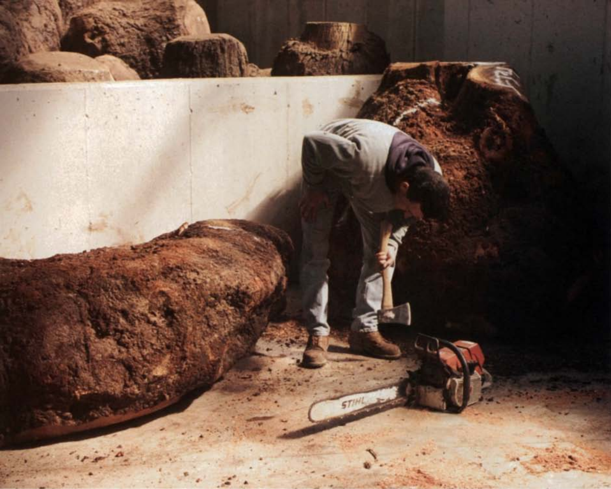
Preparing a burl for the lathe —Stephen Fowler, an employee of the M. Bohlke Veneer Corp., checks for debris before making the end cuts on a redwood burl headed for a rotary lathe.
