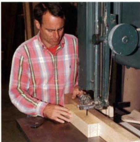
Cut stock in three pieces. Two passes on the bandsaw divide dimensioned stock into two cheeks and a center block.
