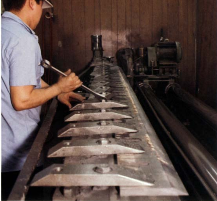
An 18-ft. razor—Keeping the knives sharp is a top priority for veneer makers. It takes about a half hour for automated grinders to sharpen a knife.
