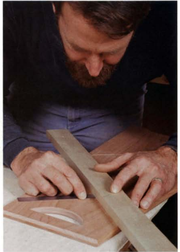
Mark the offsets from the lines just traced. These new marks are used to position a straightedge for the biscuit joiner.
