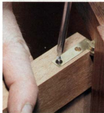
Tap the screw hole with a steel screw, and then replace it with the softer brass screw.
