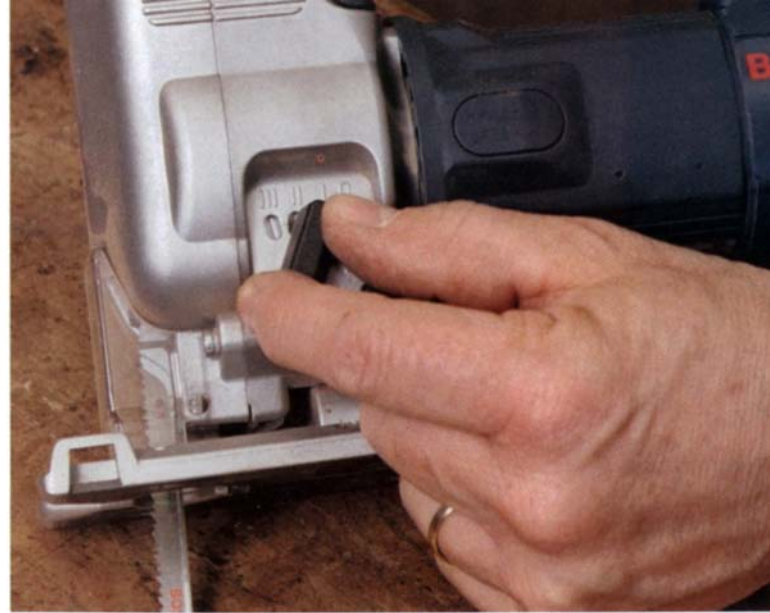
Orbital action —A switch sets the amount of orbital action (right). In non-orbital mode, the tool cuts slowly but leaves a clean kerf. In orbital mode, the saw cuts faster but creates tearout.
