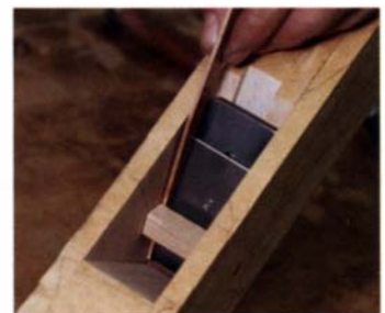
Spacing should be even. A thin strip of wood helps the author make sure the distance separating the cross-pin from the iron is uniform.
