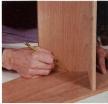
Mark the inside faces of the sides. Transfer the biscuit slot marks from the shelves to the sides.
