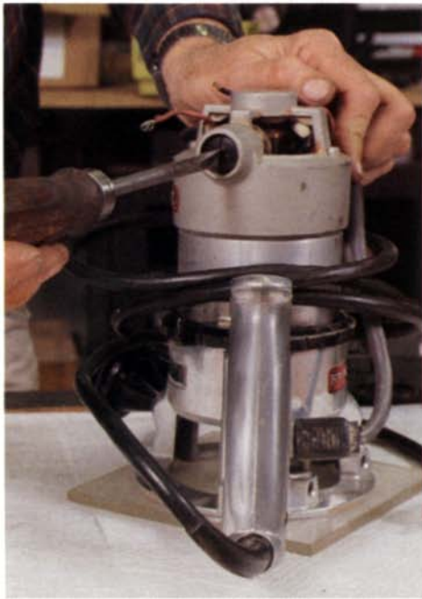
Some tools make access to brushes easy. Brushes in this router are exposed by backing out a slotted cap on each side of the housing with a screwdriver.
