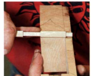
Cheeks should not pinch the cross-pin. When cut correctly, the cross-pin can rotate freely in holes bored through the cheeks.
