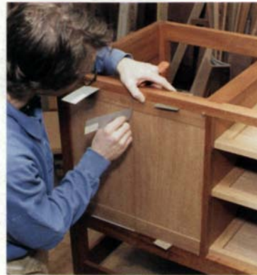
Shims of plastic laminate keep the reveal around the door consistent.
