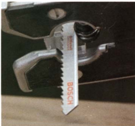
Typical blade guide —Most jigsaws come with a single, free-spinning guide located directly behind the blade. Some have quite a bit of play in them, which may allow the blade to deflect.
