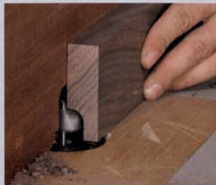
Use a 1/2-in.-radius cove bit for first cut. For support, keep the stock for the molding at least 3 in. wide.
