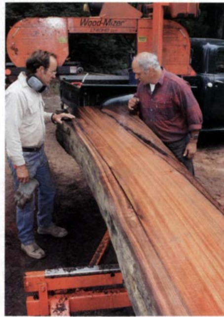
Portable bandsaw mill makes less waste. Roger Moore (right) and Monroe Robinson of Pinocchio's Timber Products check out a log they've just opened. Bandsaw mills generate less waste than chainsaw mills because the blade kerf is so much thinner.
