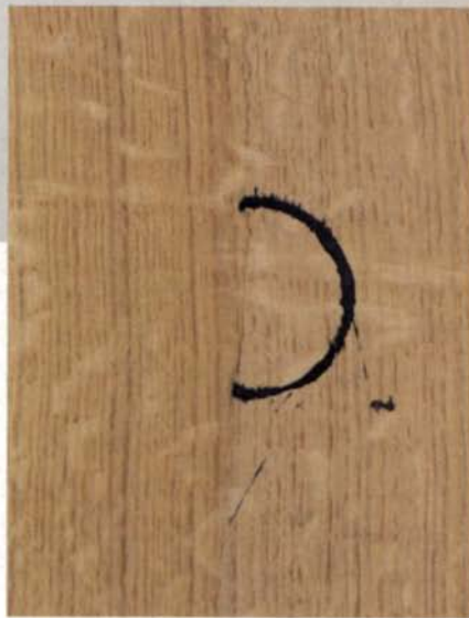
Oxalic acid removes the stain but not the color of the wood. The author used a deck brightener, which has oxalic acid as an active ingredient, on this piece of white oak.
