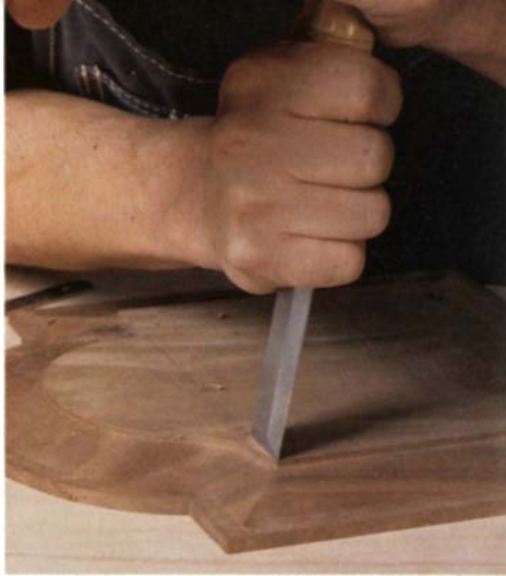
A chisel squares panel corners. A panel-raising router bit leaves corner details unfinished. A chisel cuts the 90° angles at the inside corners.
