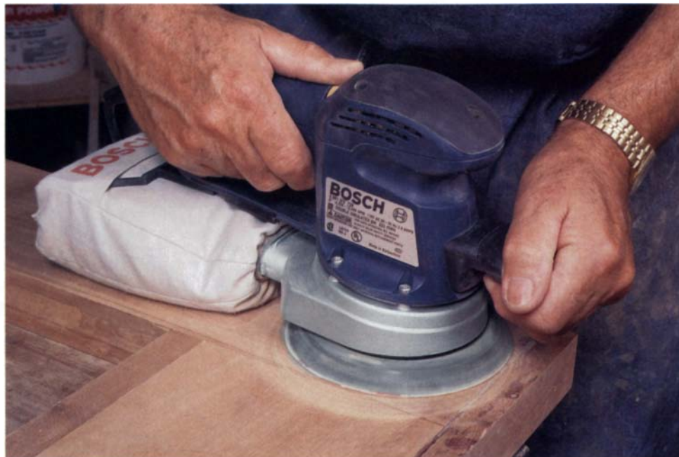
Smooth random-orbit sander —Bosch's new variable-speed, 6-in. random-orbit sander (model 3727) has double bearings at the base of the shaft, reducing vibration.
