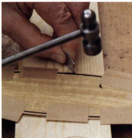
One clean strike with a razor cuts the inlay for an angled seam that will virtually disappear when finished.
