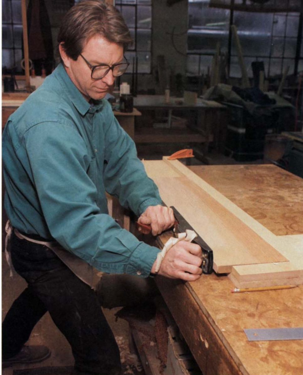
Shooting board simplifies getting a square edge. Once the plane blade is set correctly—at 90° to the bench—a square edge is almost automatic. The side of the plane uses the bench as a reference surface.
