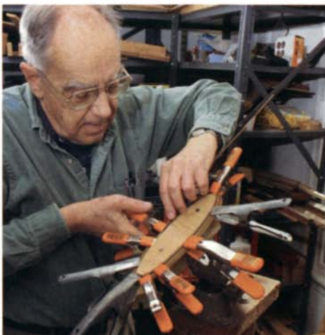
After bending the inlay completely around the form and clamping it in place, allow it to dry overnight.
