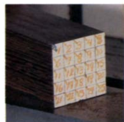
Mark stock before cutting plies. Plies are numbered (above) so they won't get mixed-up as they are band-sawn and then run through a thickness planer (right).
