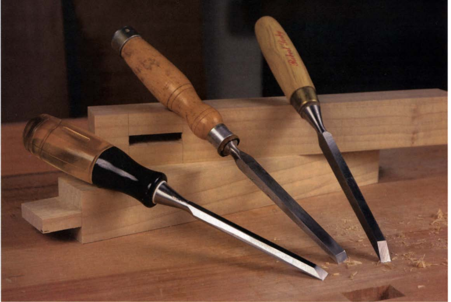
Basic bench chisels —Bevel-edge chisel (left), firmer chisel and mortise chisel all have different tasks in the workshop.
