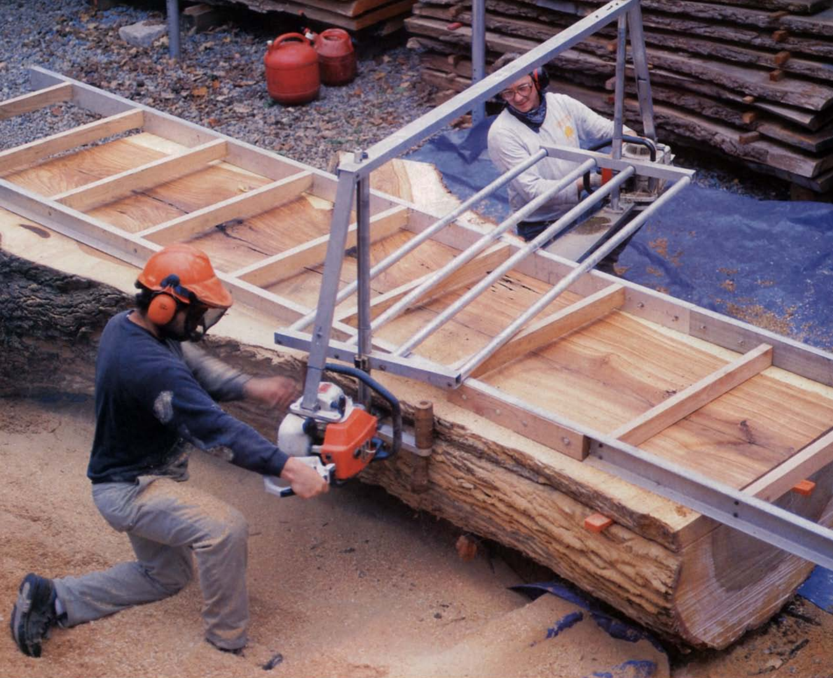
Monster ash requires chainsaw milling. With its 79½-in. bar, this chainsaw mill requires two of Stihl's largest motors for power. Joe Kleinberg, in the foreground, and Rick Johnson have since bought a portable bandsaw mill as well.
