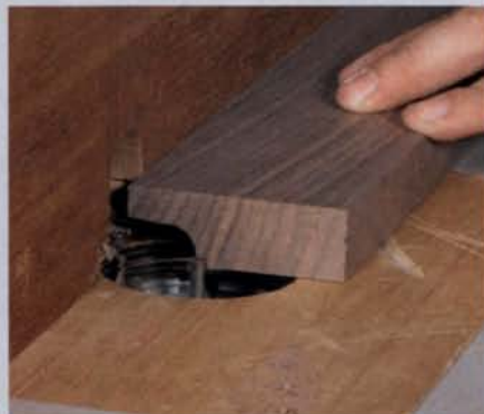
The reveal is machined next. Turn stock on its side, switch to a straight bit and align fence for desired reveal.
