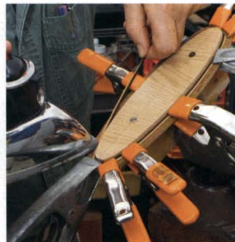
Work in small increments. With a tight radius, the author heats and bends only about 1/4 in. at a time.
