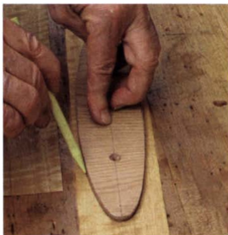
Bending form is also master pattern. The smaller piece of 1/4-in. plywood can be used to mark the veneer.
