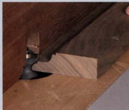
Finish by cutting the bead. Flip molding on its other face; use a 1/2-in.-dia. beading bit to shape the edge.
