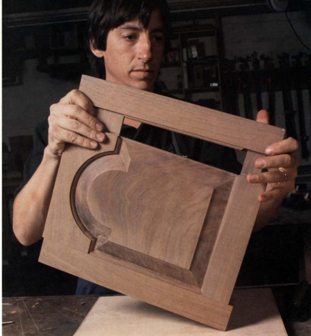
Full-length tenons hold the frame together. The author dry-assembles the completed tombstone door. After glue-up, he trims the door to fit the case opening.
