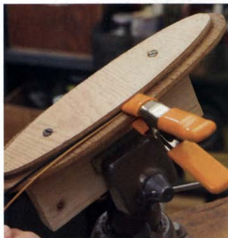
Bend two at once. Dampened light and dark inlay pieces are bent in pairs, as they'll appear around the ellipse.
