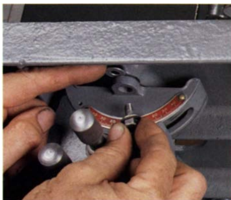
Front-to-back adjustment —A flat washer inserted between the table and either the front or back trunnion will help square the table to the blade.
