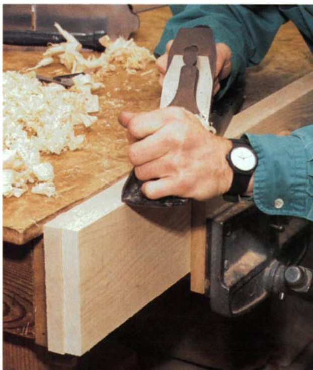
Shooting board simplifies getting a square edge. Once the plane blade is set correctly—at 90° to the bench—a square edge is almost automatic. The side of the plane uses the bench as a reference surface.
