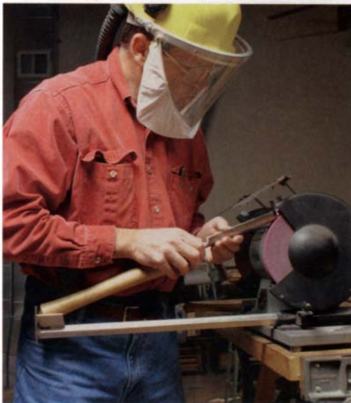
Preparing spindle stock —A roughing-out gouge makes quick work of rounding a square billet.
