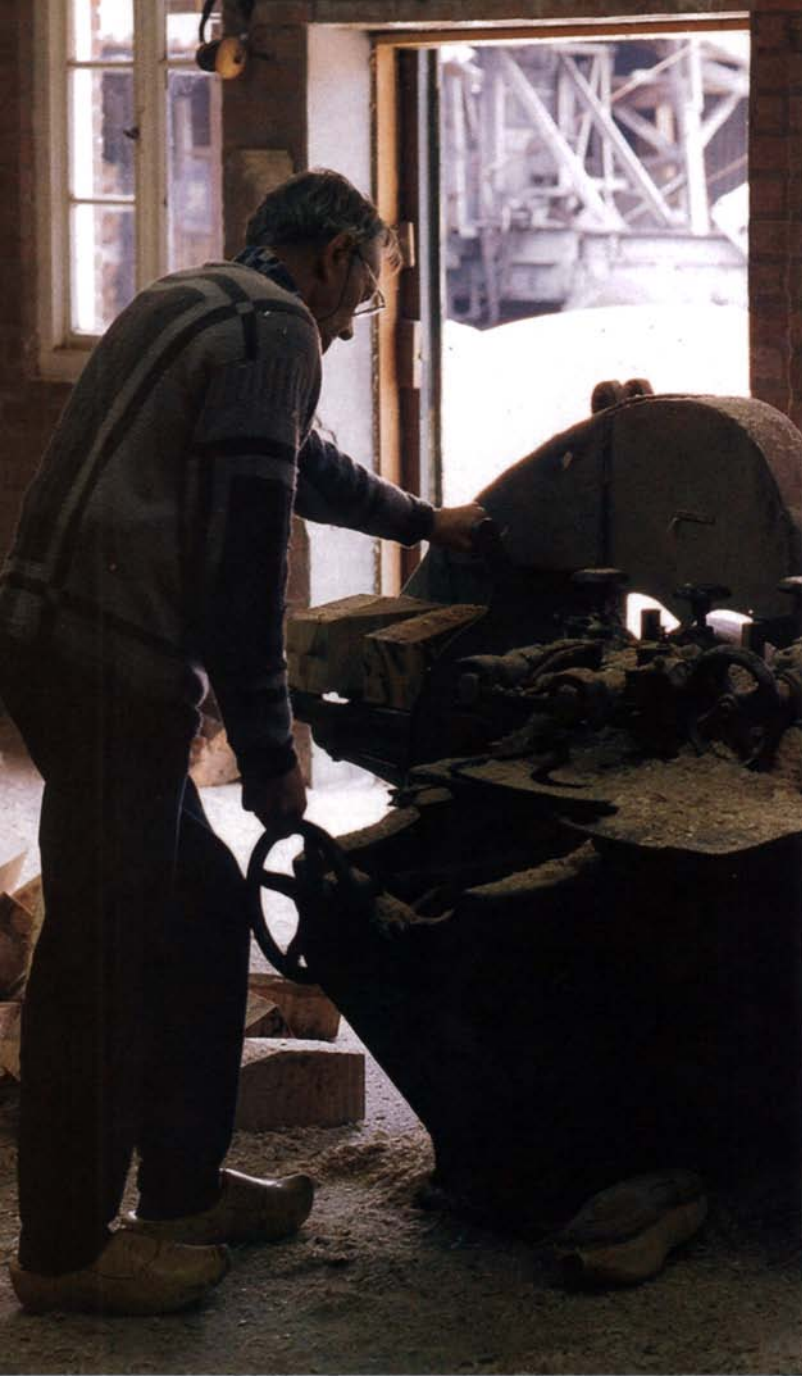
Automated machines shape and carve the klompen. Harry Laarhoven (above) operates a roughing machine—the first step toward shaping the outsides of the shoes. The boring machine in the Nijhuis family plant in Beltrum (right) carves out the insides of a pair of shoes by copying the master blank at center.
