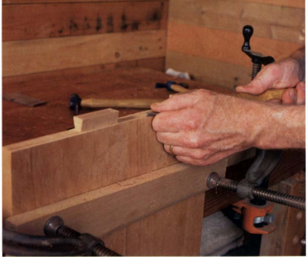
After cutting a dovetail the full width of the upper case side, cope out the dovetail keys (left), and then clean up the shoulder with a chisel (right). Pare carefully: The line of the finished joint depends on the flatness of the shoulder.
