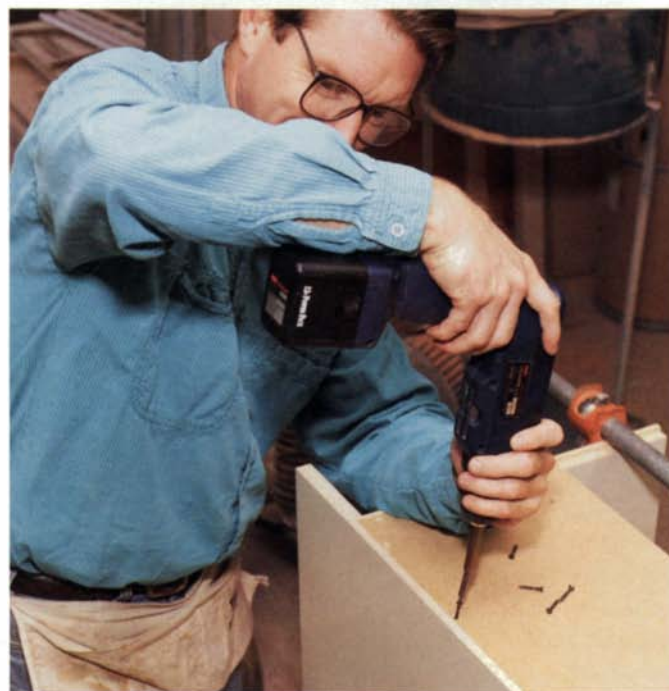
Fiberboard back prevents racking. Although it's only \frac{1}{4} in. thick, the fiberboard back greatly strengthens the table. The fiberboard is glued and screwed into a rabbet all around the back of the table.
