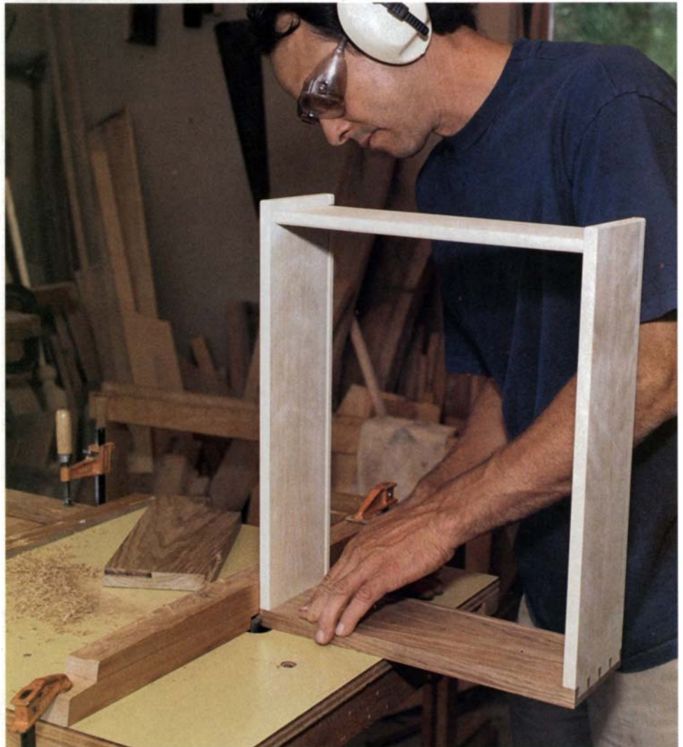
Rout the rabbet. Cut to full depth, but set the fence to slightly less than the thickness of the rabbet so that it can be trued up with a plane. To avoid tearout, rout the sides first and then the top and bottom edges.
