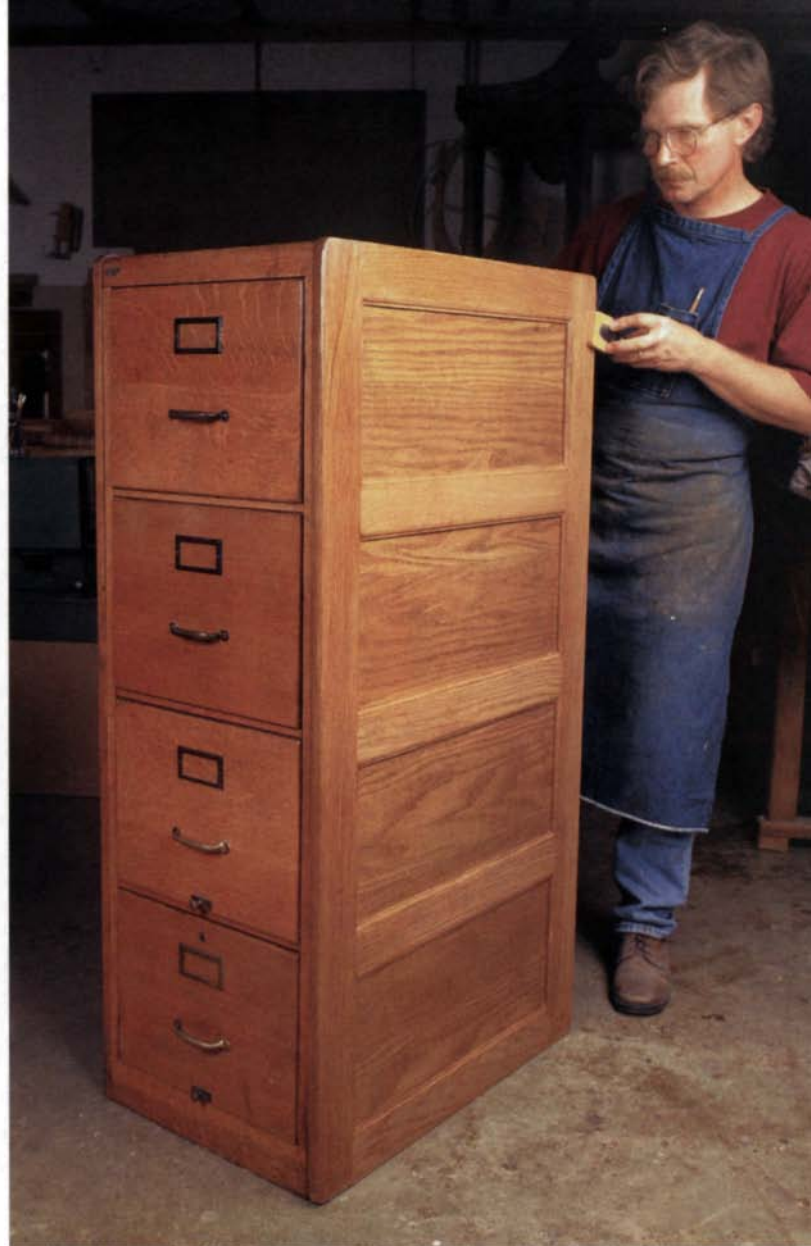
Changing the color of oak—Red oak panels in a white oak frame (left) don't match. So the author stained the piece and dry brushed the red oak to achieve a uniform color (right).
