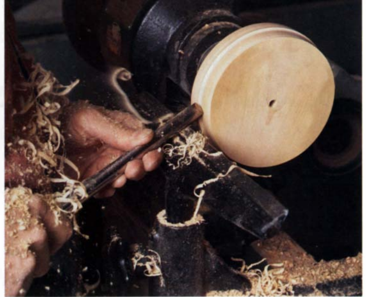
Faceplate work —A bowl gouge allows the author to cut across the grain and create hollows and curves.
