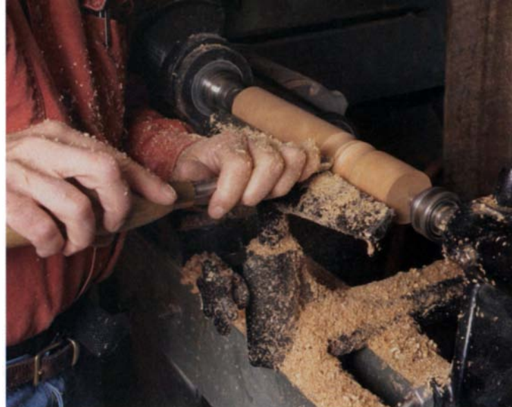
Cutting coves and beads —Much of what's needed for furniture-making can be performed with a spindle gouge.
