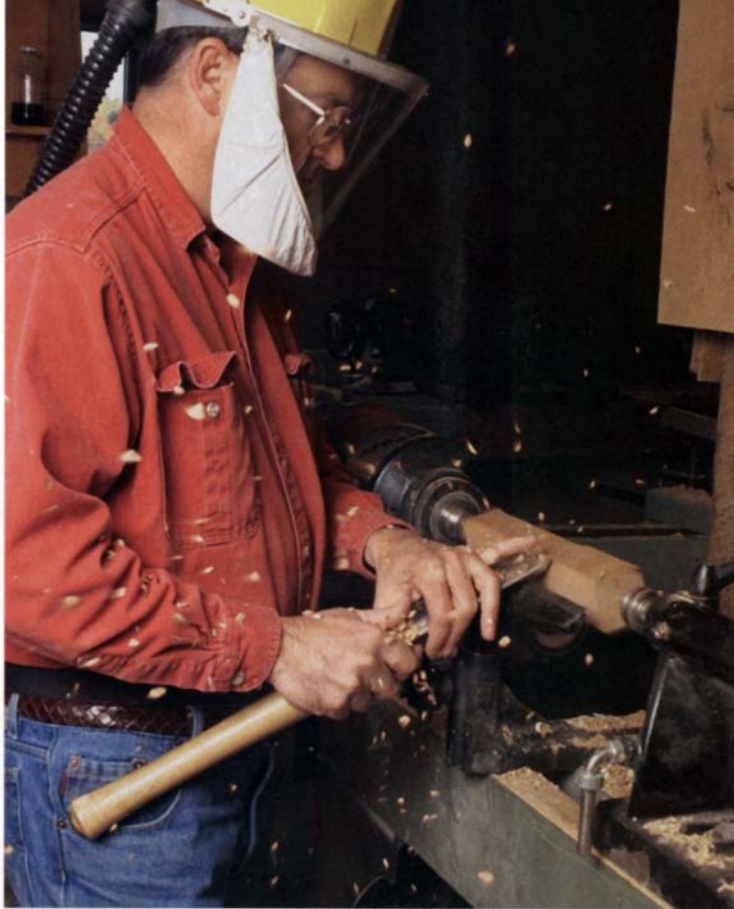
Preparing spindle stock —A roughing-out gouge makes quick work of rounding a square billet.
