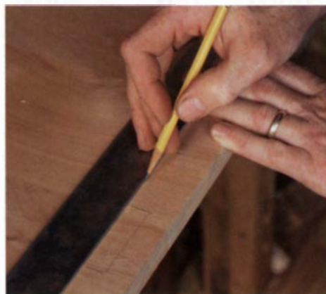
Layout the escapements using the dovetail slots as a guide. When you cut the joints, remember that the escapements are at the back of the cabinet.
