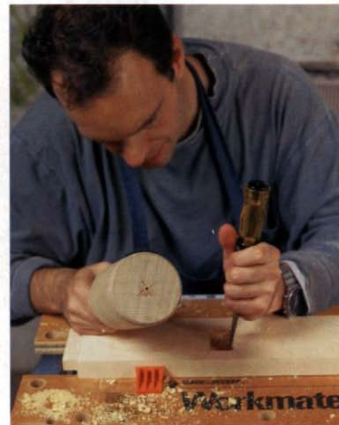
Gusset mortises—After boring holes on the drill press, the author cleans out the mortises by hand.
