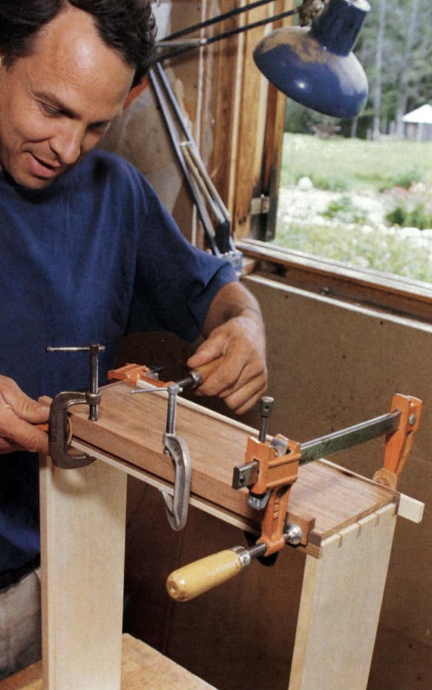
Clamp the bottom and sides in two directions. A rabbeted caul allows you to clamp the cock bead firmly into the drawer face in both planes, producing the least visible gluelines. A flat caul protects the top bead.
