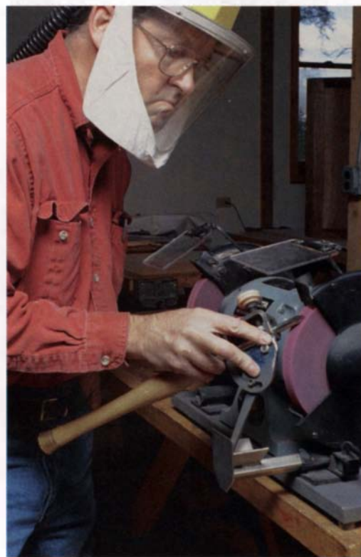
Jigs simplify the task of sharpening. Using a Oneway pocket jig and a gooseneck clamping fixture to hold the tool, the author swings a spindle gouge from side to side across the grinding wheel. Bevel angles are controlled by adjusting both the pocket jig's distance from the grinder and the angle on the gooseneck clamp.
