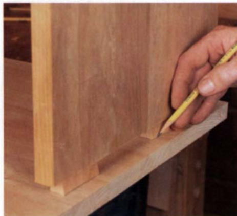
Mark the dovetail slots first. The locations for dovetail slots in the top of the lower cabinet are marked directly from the dovetailed keys.
