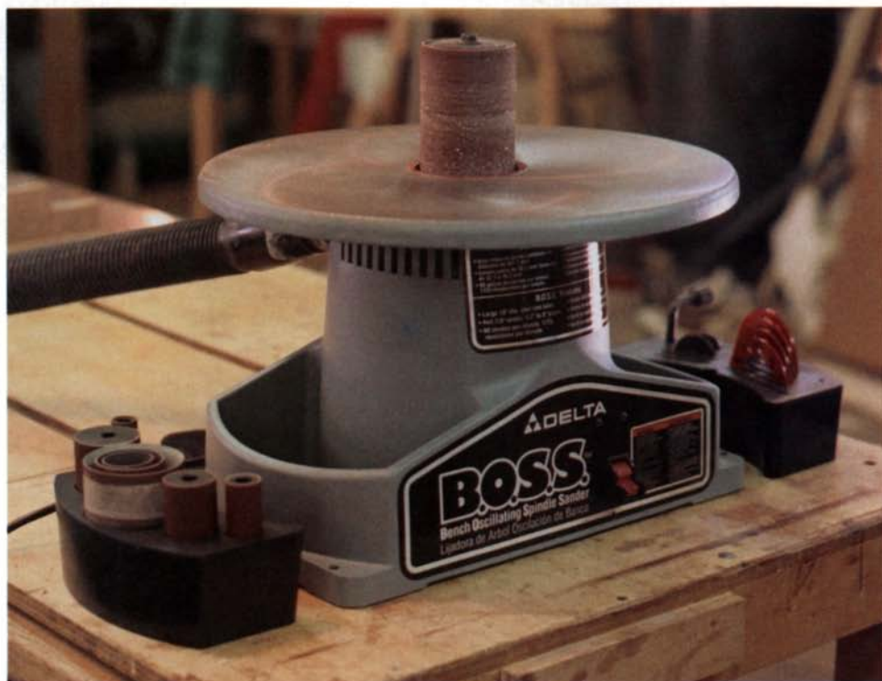
Delta's oscillating spindle sander —The Boss sander and optional kit of different-sized spindles and throat-plate inserts.
