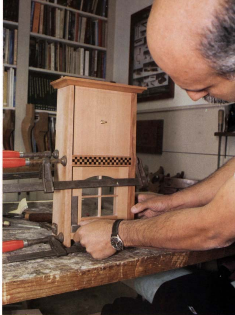
Assemble the clock on its side, turn it upright and then place the top on the clock. Adjust the clamps as necessary to make the case square.
