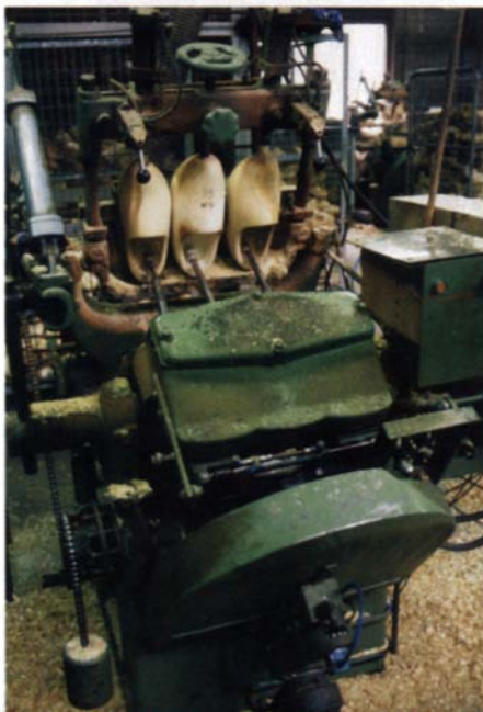
Automated machines shape and carve the klompen. Harry Laarhoven (above) operates a roughing machine—the first step toward shaping the outsides of the shoes. The boring machine in the Nijhuis family plant in Beltrum (right) carves out the insides of a pair of shoes by copying the master blank at center.
