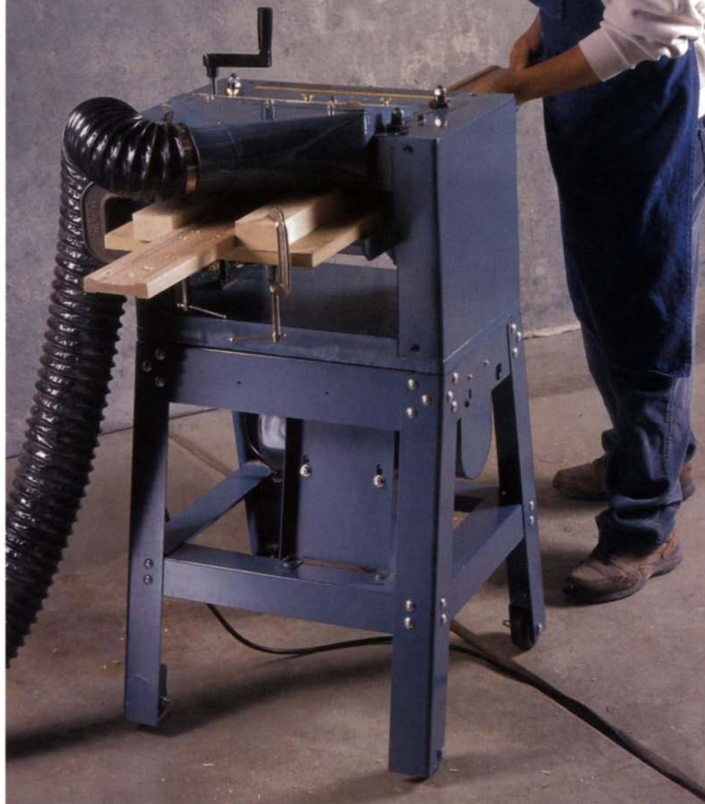
Custom crown molding —The author used a Jet 13-in. Planer/Molder to make 700 ft. of oak molding while restoring his home.
