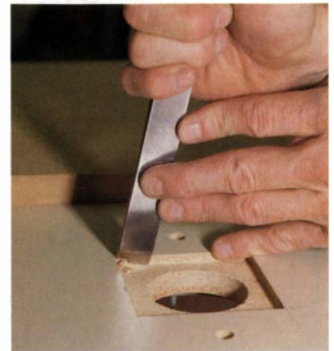
A recess for interchangeable inserts—A plunge router and chisel make short work of a recess in the tabletop that accepts inserts for different-sized bits.
