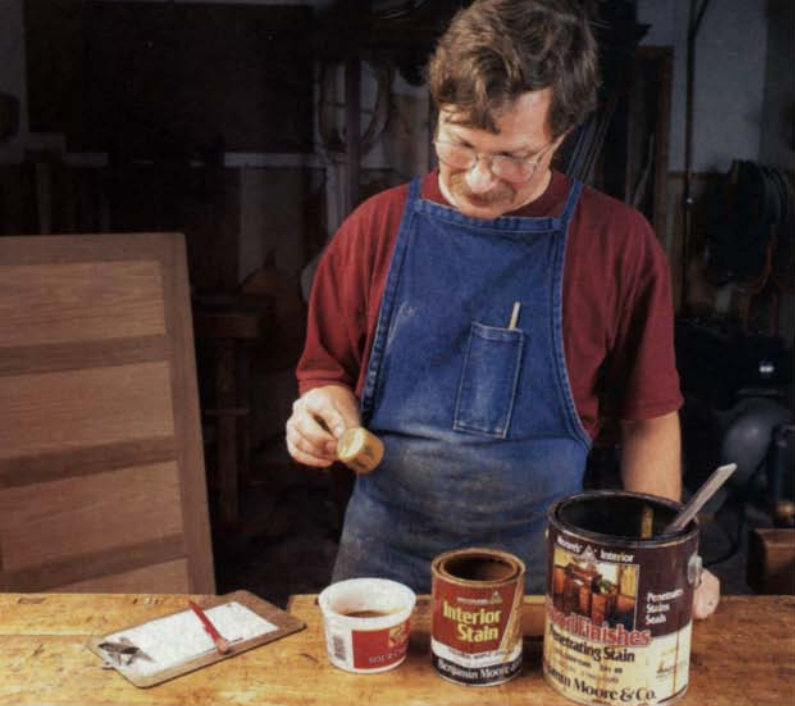
Mix and match stains. Benjamin Moore's golden oak and colonial maple stains are mixed to create a tint matching new millwork to an old white oak filing cabinet under repair.
