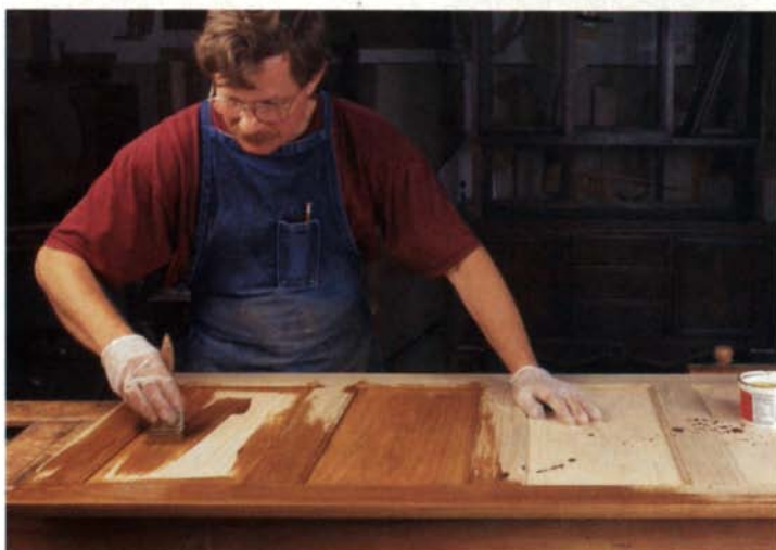
Apply a base coat. The rebuilt side of the case is covered with a first coat of stain and then wiped off.
