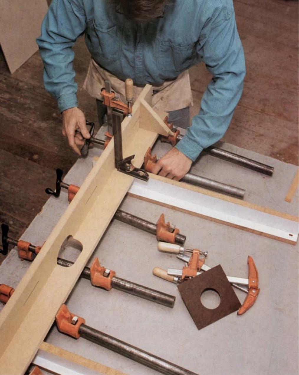
Clamp the fence square. Adjust the clamps (left) to get the two pieces square over the entire length of the fence.
