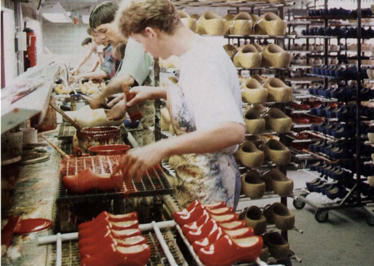
Finishing is still handwork . Some shoes are sold raw, but those that get a finish are painted with a brushing lacquer, one by one, by hand.
