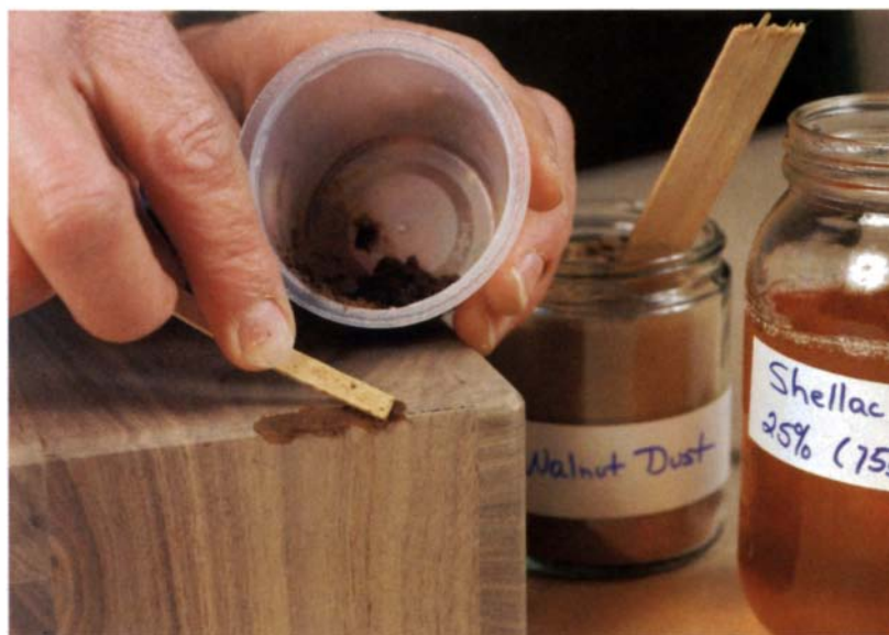
Shopmade putty. The author uses either shellac or hide glue as a binder and mixes it with fine sawdust. The color match is nearly perfect, and the repair virtually disappears.
