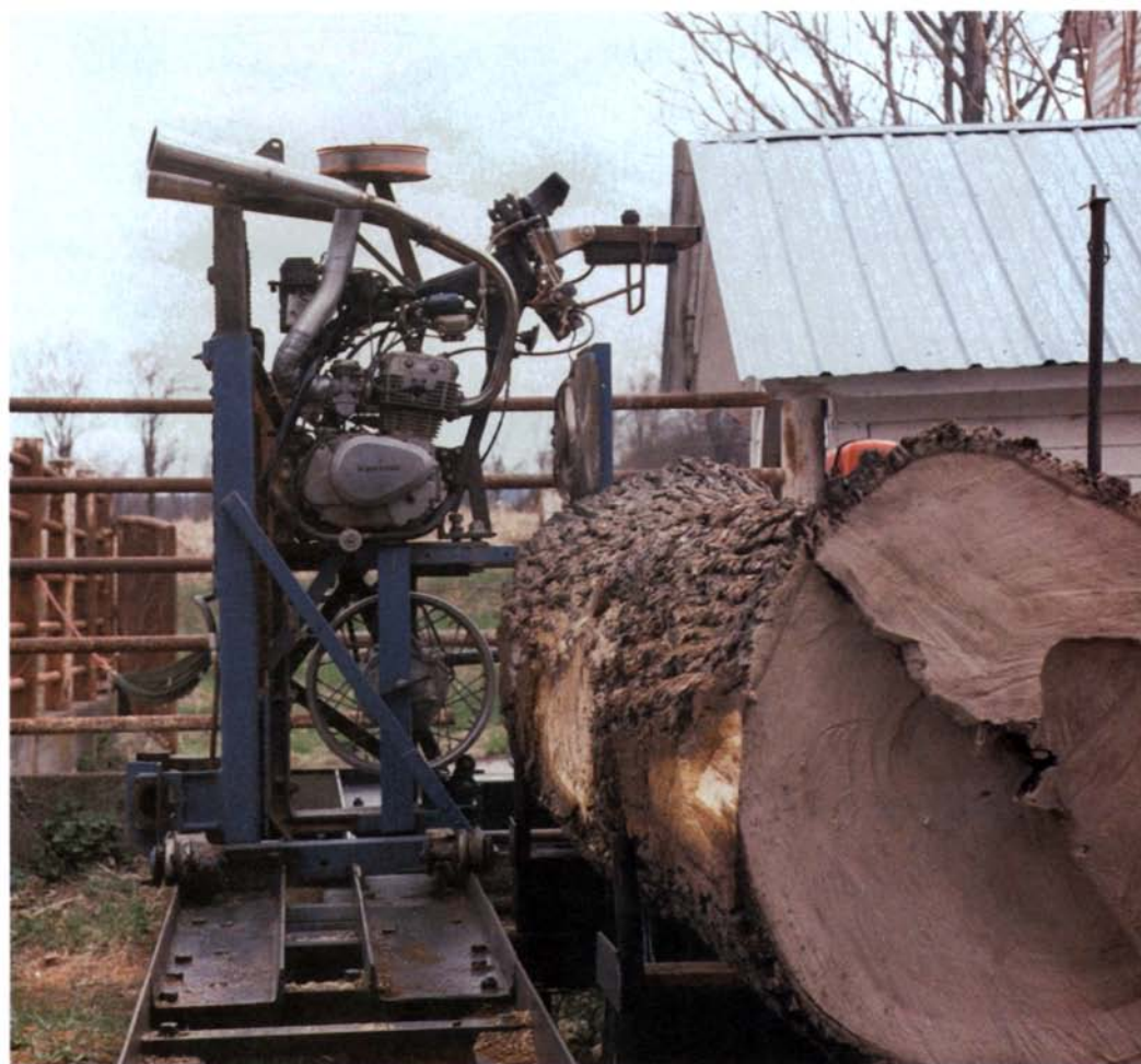
Kawasaki 350cc bandsaw mill. Kelly Barton of Ulster, Pa., built this mill with parts from a motorcycle and a forklift. The black walnut log is from Barton's woodlot. It's 30 in. dia. by 11½ ft. long, nowhere near the mill's maximum capacity.
