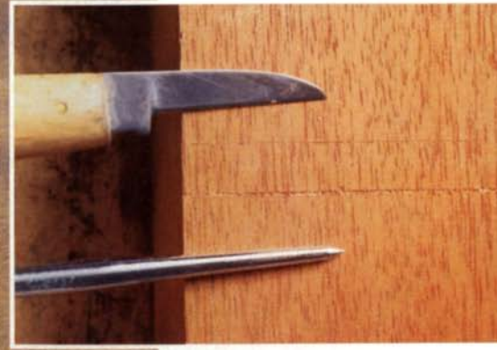
An awl point breaks wood fibers across the grain; a sharp knife cuts them.
