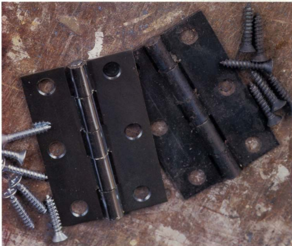
Old hardware, in a hurry —Stephen Winchester takes shiny, zinc-plated hinges and other hardware and turns them a dull black, making them look almost hand-forged. The whole process takes only an hour or two.
