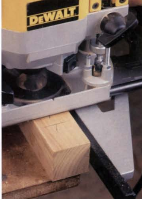
Layout lines are much easier to see when they're not hidden. The pencil marks show where the router base should stop, and the tick marks indicate that you're getting close.
