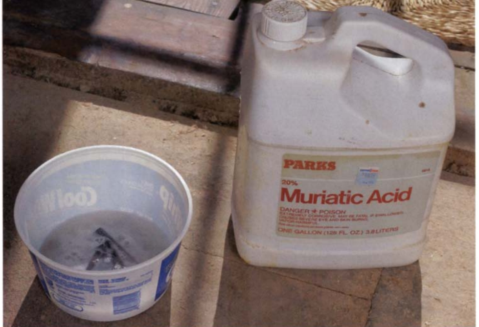
Remove the zinc-plating with muriatic acid. The mixture will smoke, so stand back and don't breathe the fumes.
