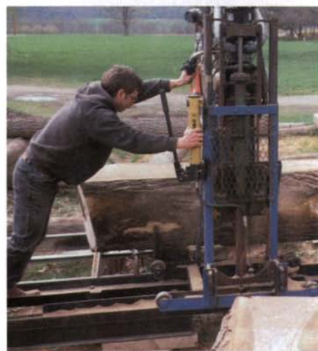
Barton feeds the saw by hand. Blade speed and sharpness, the type of wood, moisture content and the width of the cut affect the speed of travel.
