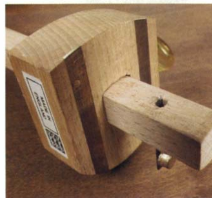
The larger blade of a cutting gauge will produce a cleaner cut across the grain.
