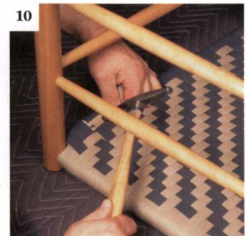
End the weft on the bottom. One tack to the underside of the front rung, after all the rows have been pulled tightly and adjusted for neatness, finishes the job.
