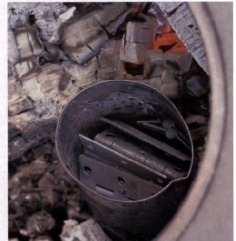
Heat the hardware to red hot. Then let it cool until you can touch it.
