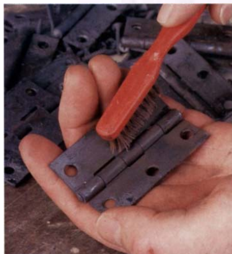
Brush off the scale. An old toothbrush works well for this job.
