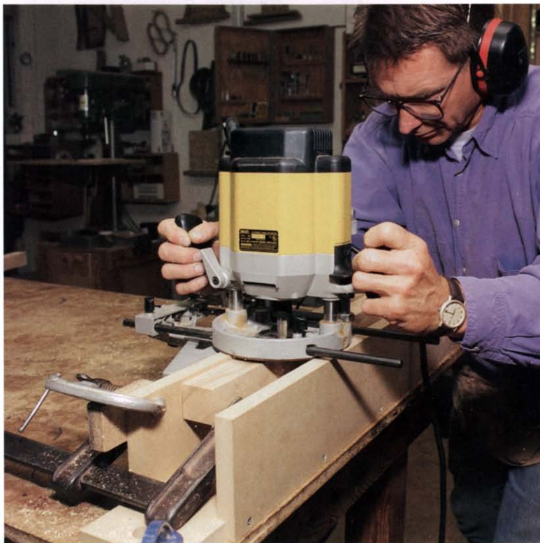
One fixture cuts many mortises —This simple U-shaped box is one of the most versatile mortising fixtures you can build.
