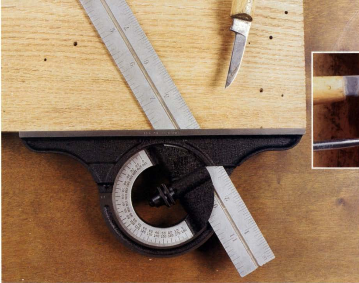
An awl point breaks wood fibers across the grain; a sharp knife cuts them.
