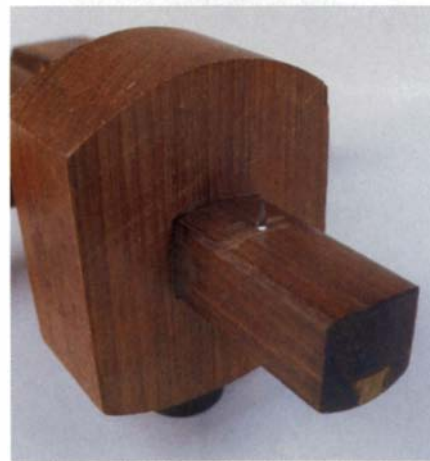
Good lighting, a magnifying glass and careful filing will greatly improve the performance of a pin gauge. The pin may be filed to a small knife edge, which won't tear the wood as much.
