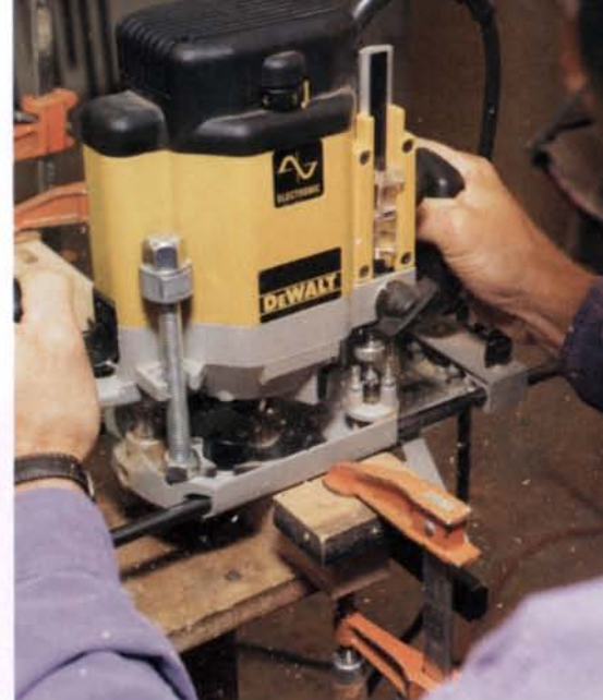
Stops are foolproof. Clamp or screw stops in place to limit the travel of the router, front and back. You won't have to worry about trying to see layout marks when the chips are flying.
