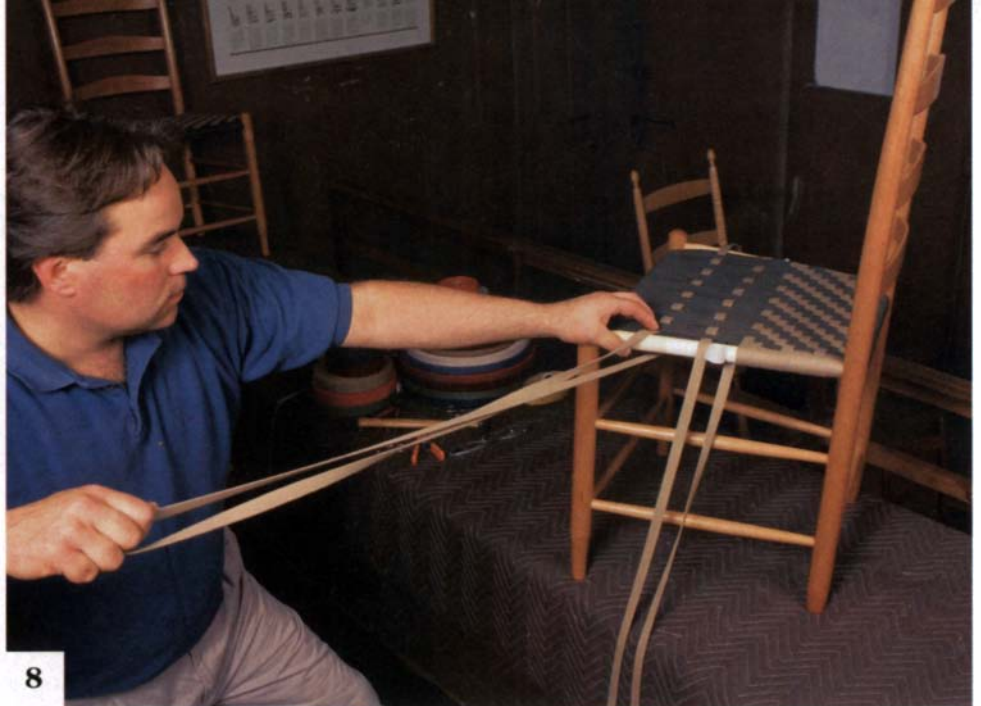
The weft is next. After weaving the tape front to back, the author adds the weft—the side-to-side rows. He starts at the back of the chair.
