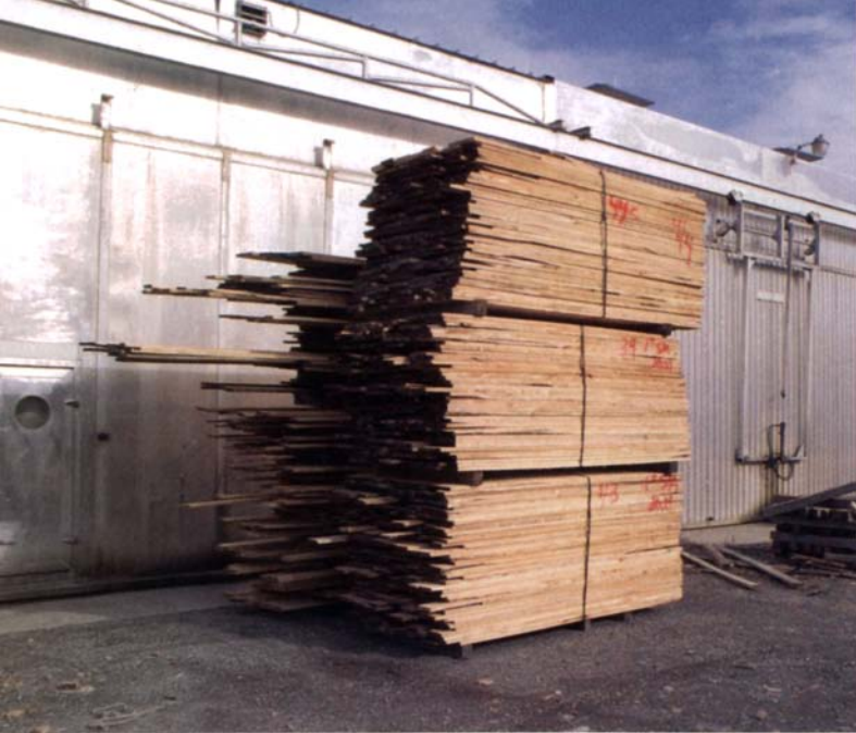
Kilns season wood quickly and uniformly. Commercial kilns are capable of seasoning large quantities of wood.
