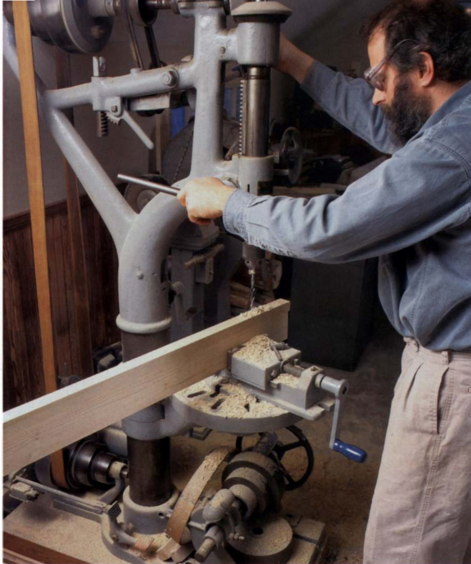
Mortising the stiles —The author uses his drill press with a twist bit to remove most of the stock. You could also use a router, a mortiser or chop out the waste by hand.
