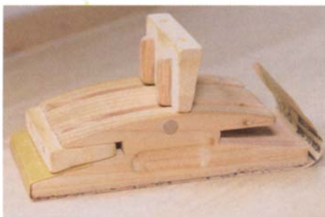
A sanding block that's a pleasure to use. Oregon cabinetmaker Tony Allport designed this Douglas fir and Alaskan yellow cedar sanding block that holds a quarter-sheet of sandpaper.
