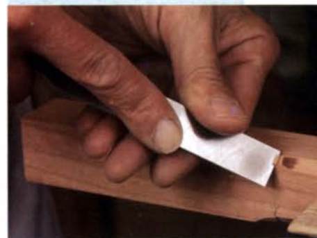
Step 1: Pare to marked baseline. Strive for a fair, even curve, and cut down toward the chamfer.
