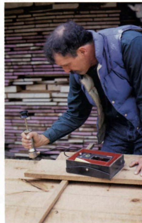
A moisture meter eliminates guesswork, whether you dry your own wood or buy it at a lumberyard.
