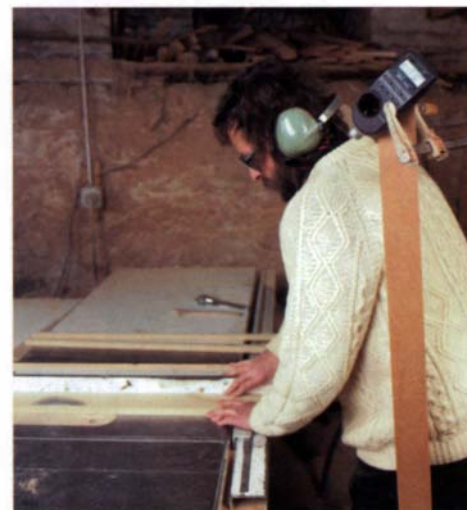
Blades all produced about the same noise levels, around 93 decibels.
