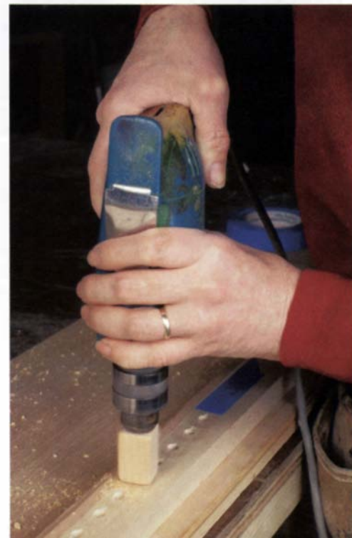
Drilling shelf-pin holes. A template with an end-stop positions the template accurately top to bottom and eliminates the possibility of measuring errors (left). A gauge block ensures a consistent setback from the edge of the case. Different-width gauge blocks can be used for special applications, such as drilling offset pin holes from both sides of one upright (inset photo above and drawing at left). A wooden stop block sets the depth (left). It won't move either, like many metal collars. Blue masking tape indicates where the holes in the case sides should stop.
