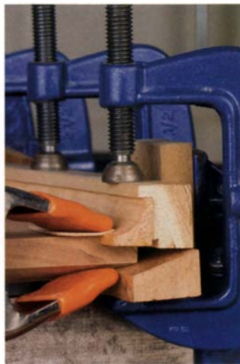
Rabbeted clamping block helps provide pressure in two planes. The author clamps down the cove strip with six C-clamps and into the rabbet with six bar clamps. A spring clamp on each end closes any visible gaps at the ends.
