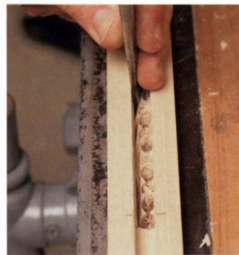
Cleaning out the mortise —After drilling mortises, the author cuts the panel grooves on his shaper. The grooves provide a good reference for paring the mortises with a chisel.
