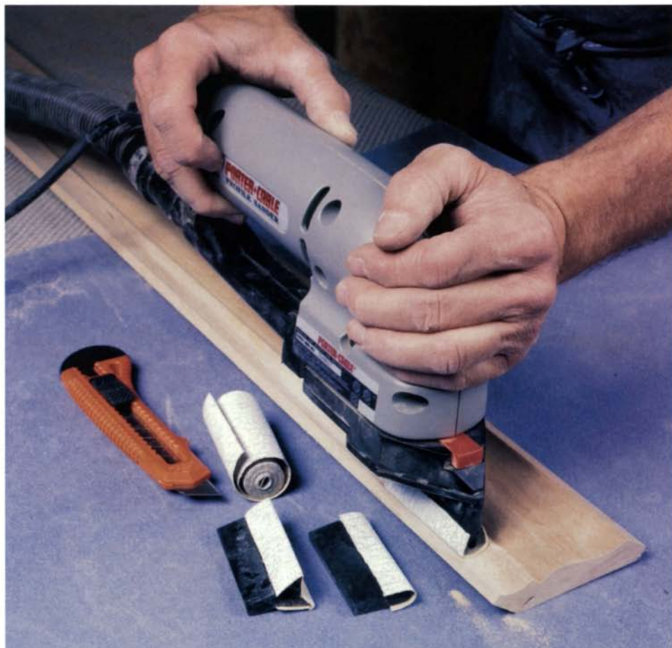
A detail sander for curved profiles —The linear motion of Porter-Cable's Model 444 detail sander, coupled with contoured pads, allows it to sand molding profiles easily.
