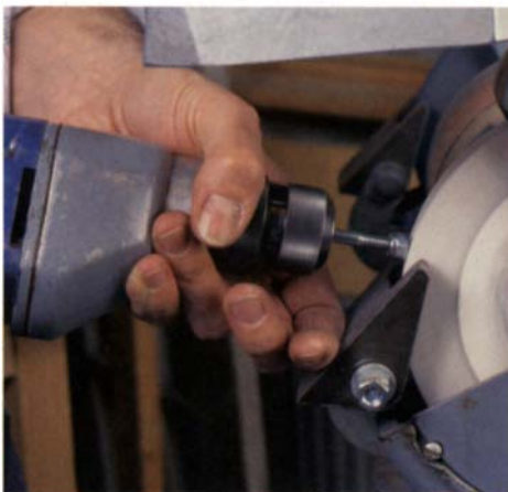
Length protruding from nut is less than depth of insert.
