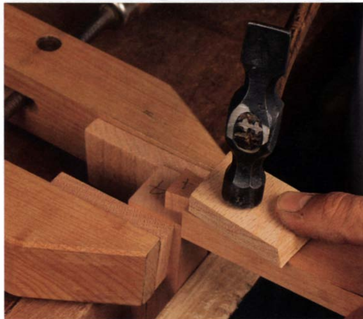
Checking the fit of the top-rail dovetail—A hand screw prevents a leg from splitting if the dovetail is too big. The fit should be snug but not tight.
