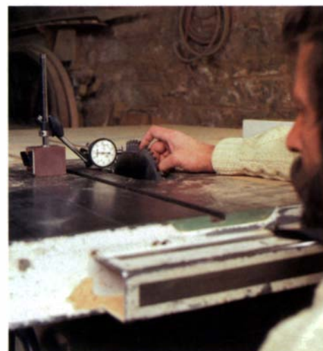
Measuring runout indicates flatness. Blades in this evaluation had runout of between .003 in. and .005 in.
