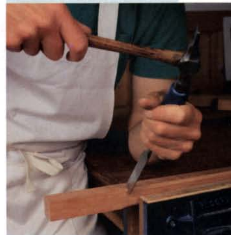
Step 2: Tap a stop for the shoulder at the baseline. Avoid cutting too deeply; just a light tap is needed.
