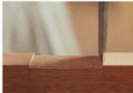
Final chops to size —This last chisel cut on the ends of the mortise for the door stile will make a snug fit for the hinge.
