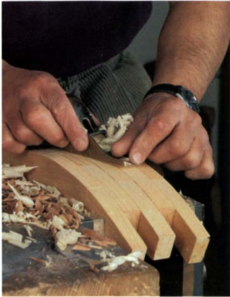
Block planes handle difficult grain. This bricklaid arch presents end grain and long grain and everything in between. For more control, use a two-handed grip, and skew the blade as it cuts.
