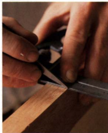
Score hinge locations with the layout knife. No shop should be without this knife; it provides a precision unmatched by a pencil or a scratch awl.
