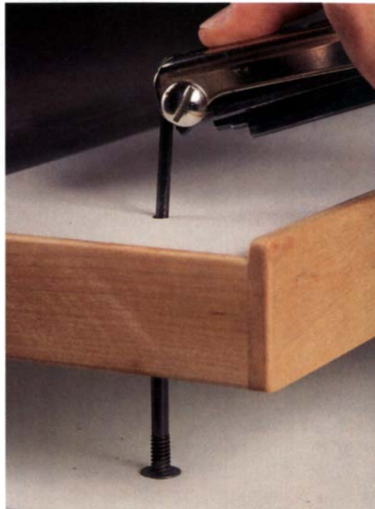
Leveling the table —Connector bolts screwed into threaded inserts allow precise adjustments to the height of the planer table.
