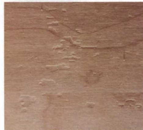
Witness lines show rub-throughs—Separate coats of reactive finishes, like water-based polyurethane, remain distinct, so be careful not to rub into an under layer. Witness lines, which look like feathery rings on this piece of birch, are the result.
