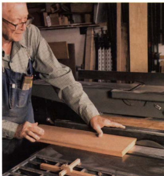
Rip the molding to width. The author cuts one edge, flips the stock around and rips the opposite edge.
