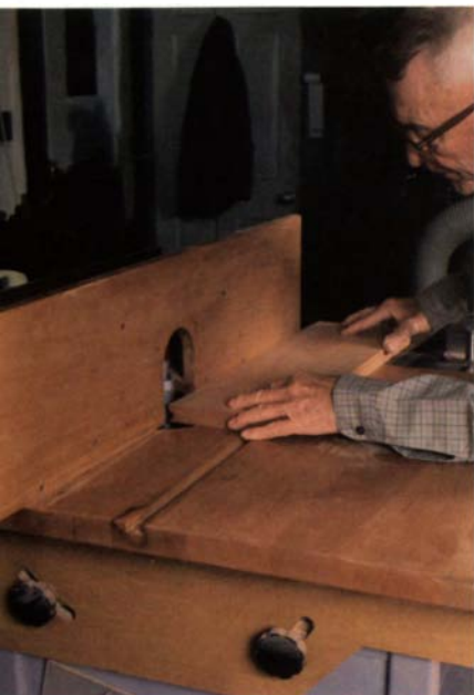
A cove cut is the first step in developing the profile. The author makes a 3/8-in. cove on both edges of a piece of stock.
