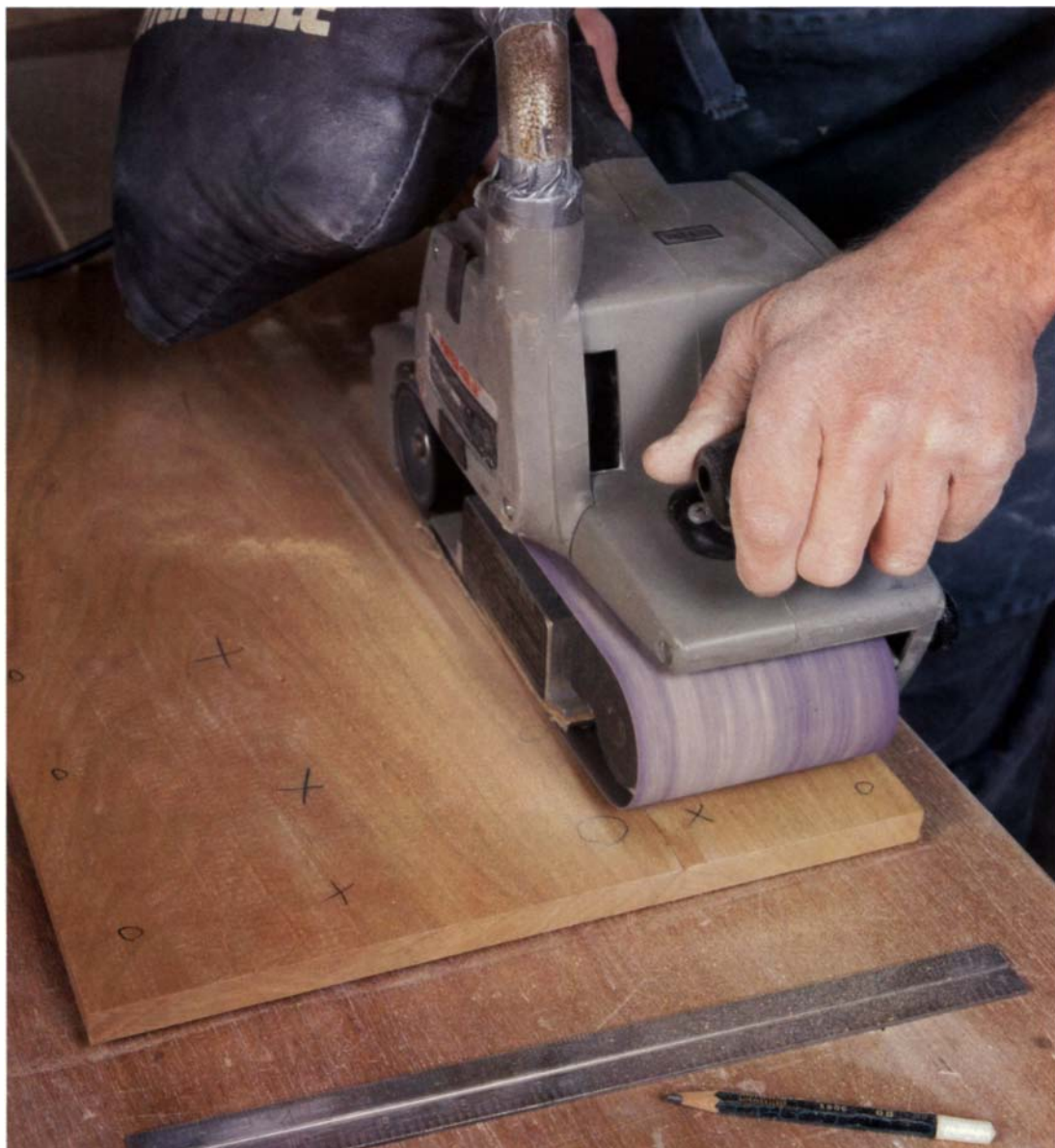
Mark the highs and lows with a soft pencil to indicate which areas need more sanding. The author makes his first pass over the surface of a glued-up cherry panel with high spots marked with X's and low spots marked with O's.
