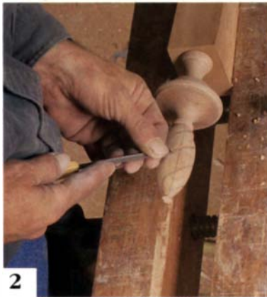
2 Begin carving with a narrow veiner. Be careful not to cut into layout lines.
