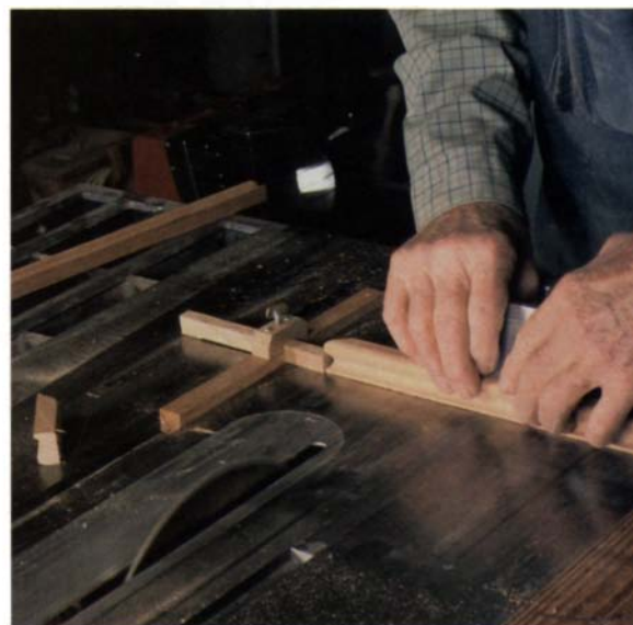
With a shopmade cutoff stop, you don't have to mark each piece. Two miter gauges, set at 45° and 90°, also speed the work.
