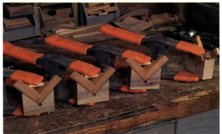
Clamp the parts. Gluing jigs hold the pieces at 90° and give glue squeeze-out a place to go. The dowel bridging the two pieces is temporary.
