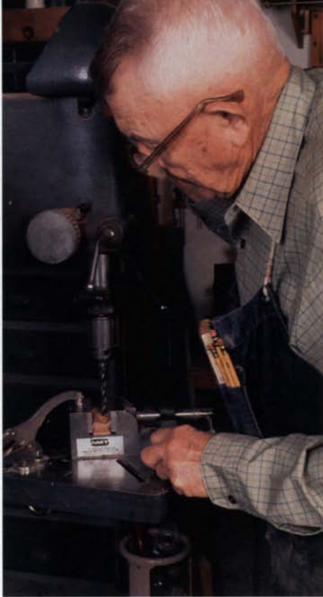
Bore the hole for the scroll profile. The hole is part of the profile and provides registration for the scroll template. A vise holds the workpiece precisely.
