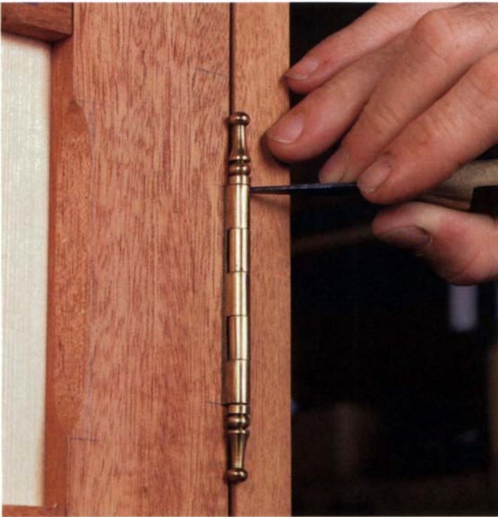
With the door in place, mark the hinge locations for the case. After the doors are fit and hinged, the author puts them back into the cabinet and scribes the top and bottom locations with the layout knife.
