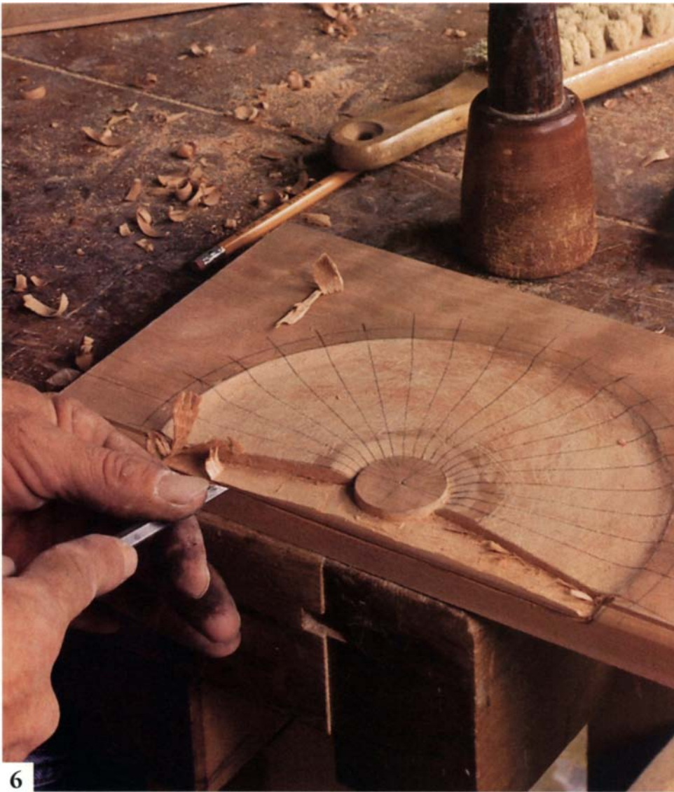
7 A V-parting tool is used to define the rays. Because the surface is S-shaped, wood grain can change direction. Take care not to run tools against the grain, which could cause tearout.
