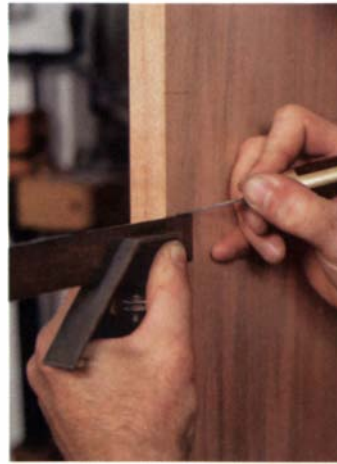
Mortising into the case —The author follows the same procedures as he did for the door-stile mortises. He starts with scribed knife lines (left) and follows that with relief cuts made with the backsaw (right).
