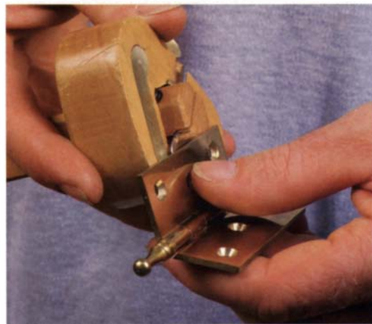
Set the marking gauge for the thinnest part of the leaf. With extruded hinges, an even spacing between the two leaves will be just right if the hinges are mortised to the depth of the thinnest part of the hinge.
