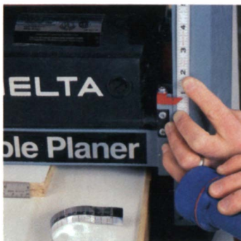
Reset the depth scale —To correct a 3/4 in. loss of cutting depth, install a new scale or reset the old one.
