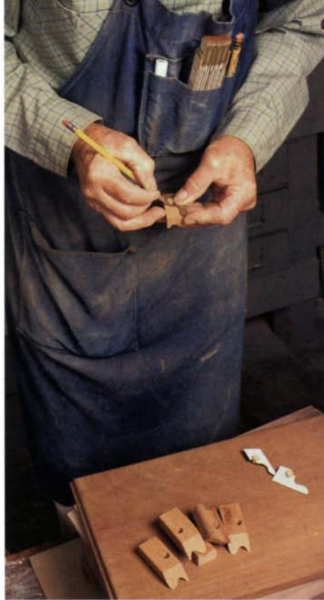
Mark out the scroll. The dowel locates the template on the pieces. The profile is laid out on the back of each foot piece.
