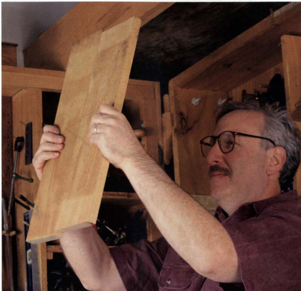
Looking for contact —Author Richard Starr inspects two jointed boards for fit. If he sees light through the joint, he goes back to the bench for more planing.
