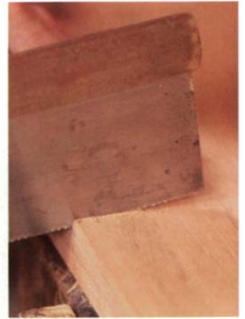
Mortising into the case —The author follows the same procedures as he did for the door-stile mortises. He starts with scribed knife lines (left) and follows that with relief cuts made with the backsaw (right).
