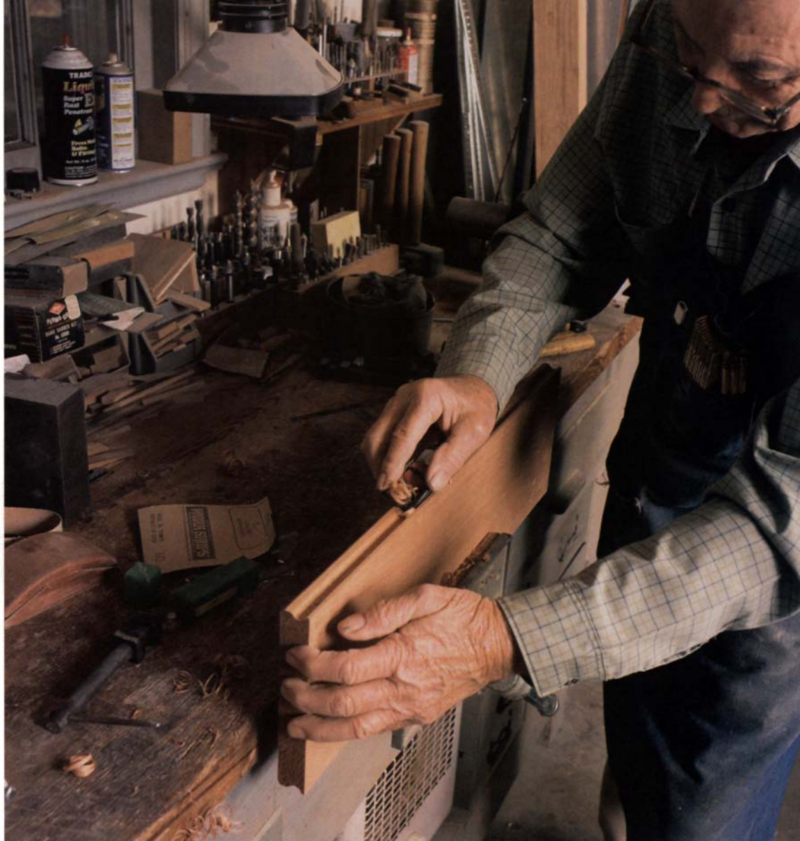
Round over the top edge. A block plane fairs a cove into the rounded edge at the top of the foot.
