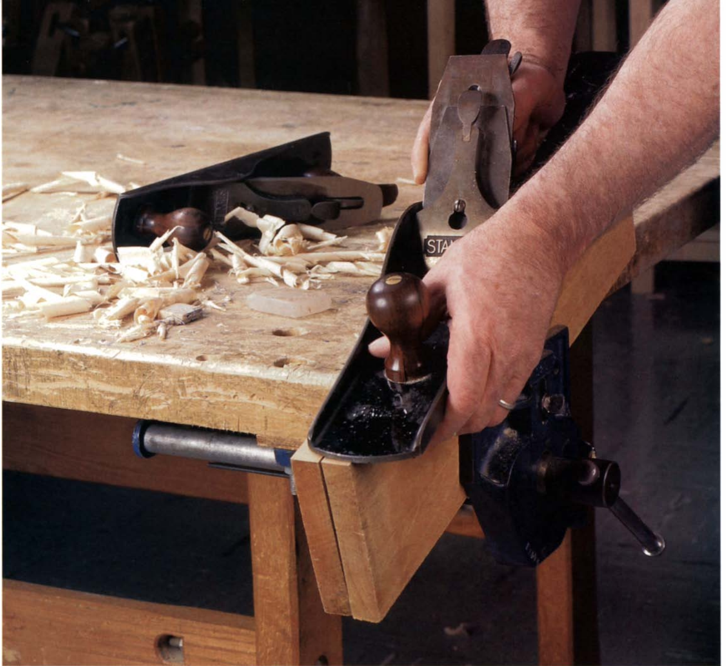
Planing two edges at once saves work. After matching boards to be joined, Starr folds and clamps them slightly tilted in a vise. Planing both boards at once helps stabilize the plane. And boards planed out of square will mate correctly.
