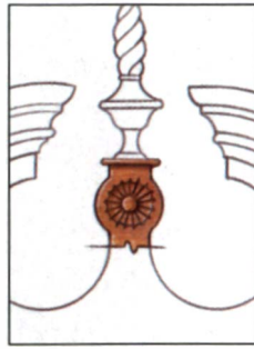
A carved fan punctuates the top of the scroll board. The fan has an outside radius of 2½ in. and a total of 17 rays.
