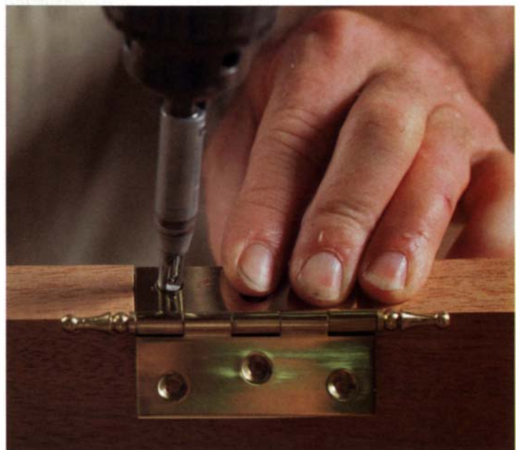
Self-centering bit finds the hole. This bit, with the hinge held firmly where it belongs, locates pilot holes for the screws.
