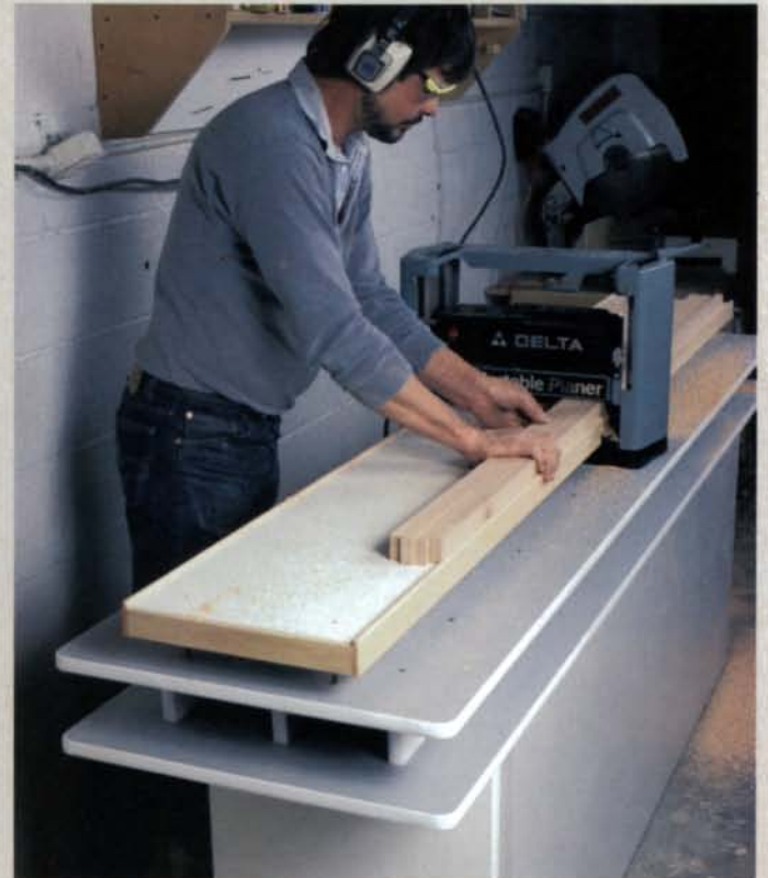
This planer table can be moved. A feed table attached to a portable base allows a planer to be parked in a corner when it's not needed. The base can be set up quickly on any stable surface, like a table or a benchtop.
