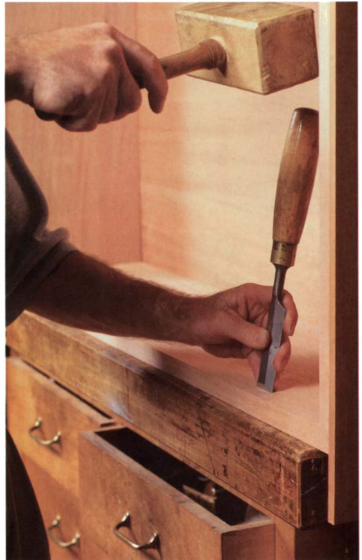
Score and clean out the mortises with a chisel. Sharp tools make this job quick and accurate.
