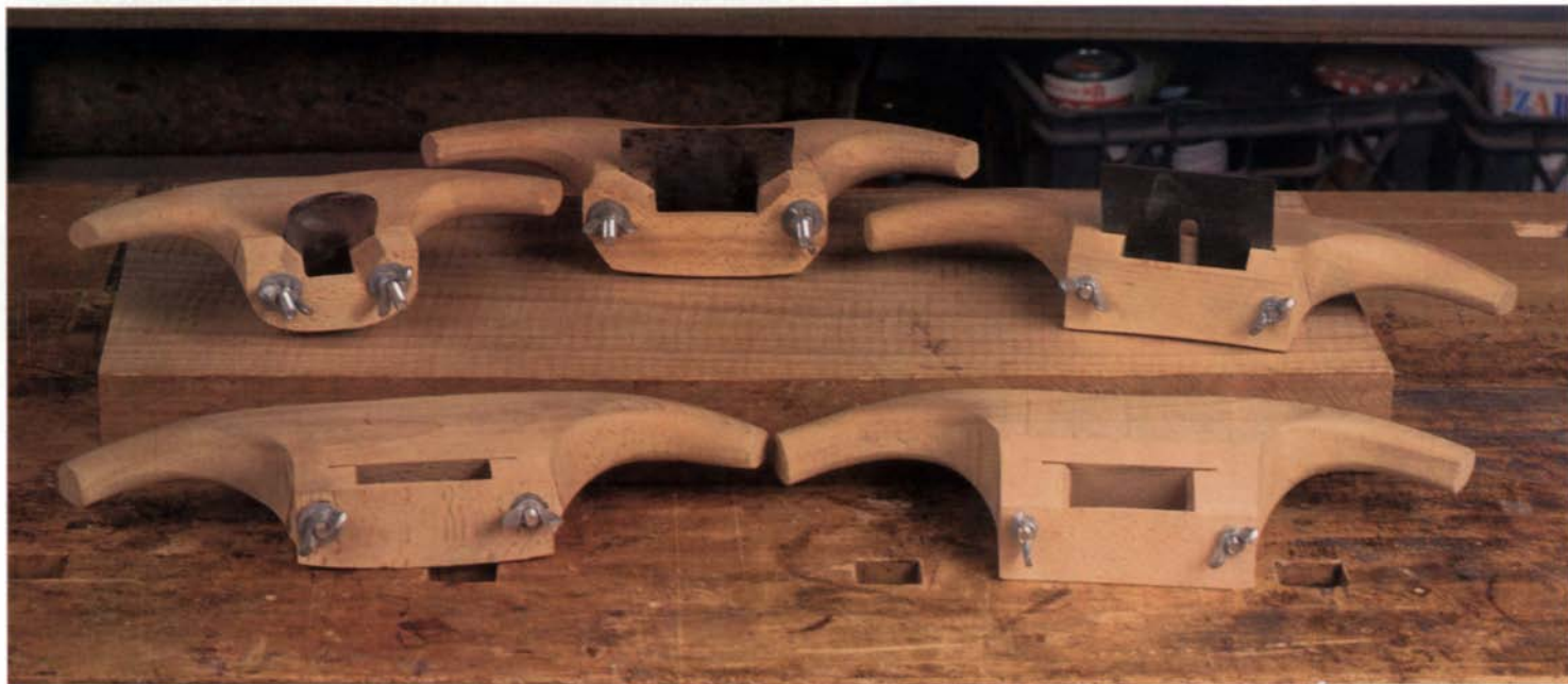
A scraper for any job —Over the years, the author has made a number of wooden-bodied buckhorn scrapers for concave surfaces, convex surfaces and compound curves. Some of the scrapers can share blades.
