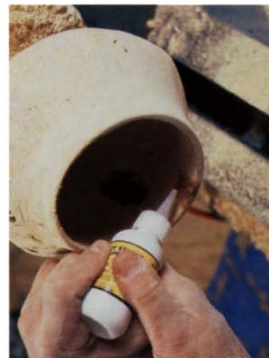
Cyanoacrylate for fixing repairs—The author prefers fast-setting Hot Stuff adhesive for its strength. He mixes mineral oil with sawdust or shavings from the turned piece to maintain a good color match and then applies the glue over that.
