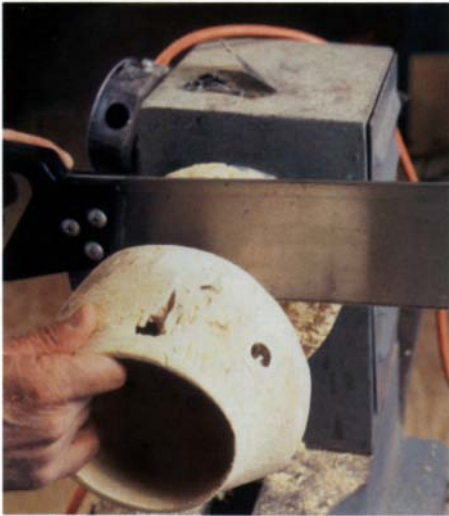
A handsaw is safer than a parting tool when separating the bowl from the waste mounted to the faceplate. The author cleans up the cut on a disc sander so that the bowl will sit flat.
