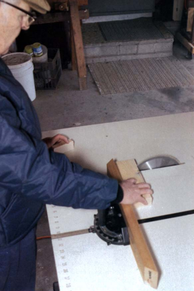
This sliding fence is easy to grip with hands or clamps, and it supports the work right up to the blade.
