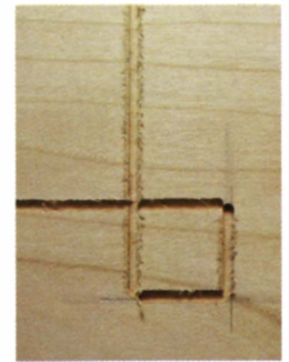
A router cuts the grooves. A \frac{1}{16} -in. straight bit and an edge guide on the router help make grooves of uniform depth. They still must be cleaned up.
