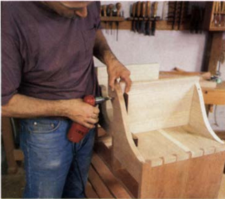
Hold the bonnet frame square, and drill pilot holes for screws. Once the glue has dried, screws are replaced with forged nails.
