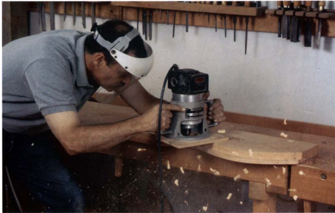
Removing waste quickly —A router does the heavy work quickly. The author will hand-carve the details in this traditional deep molding.
