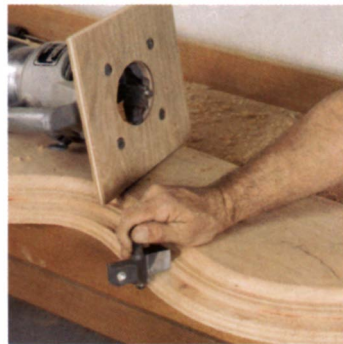
Custom-made router bits establish the overall profile of the gooseneck molding.
