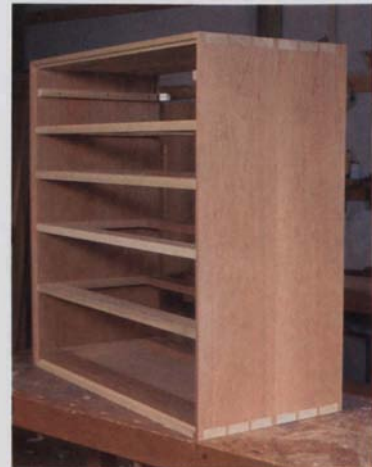
It's really not complicated. The upper case of the highboy starts as a large dovetailed box. Molding covers the joinery at top and bottom.
