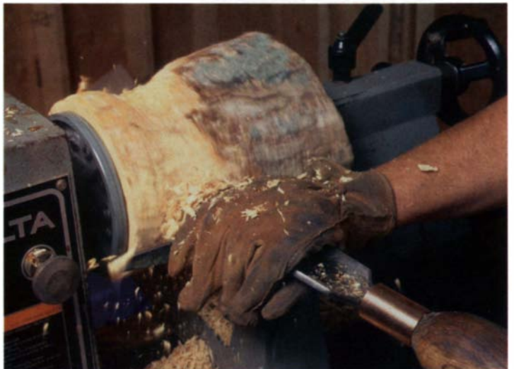
Start the lathe at a slow speed when roughing out the shape with a gouge. Soft, spongy wood cuts differently from sound lumber: It chips or breaks more than it cuts.
