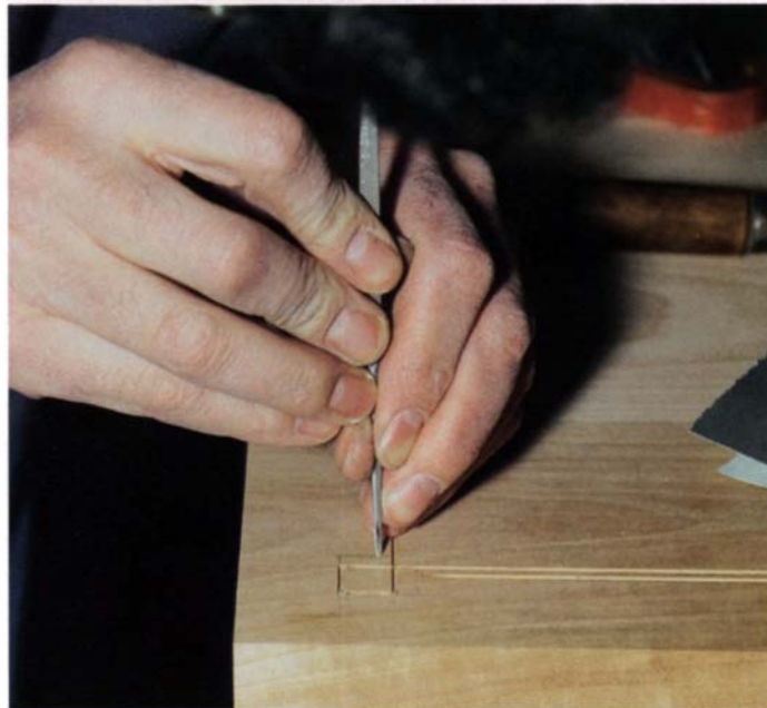
Clean grooves carefully before trying epoxy. The end of a small file ground to form a narrow chisel squares up corners. Fuzzy edges and the bottoms of the grooves should be cleaned up with 320-grit sandpaper.
