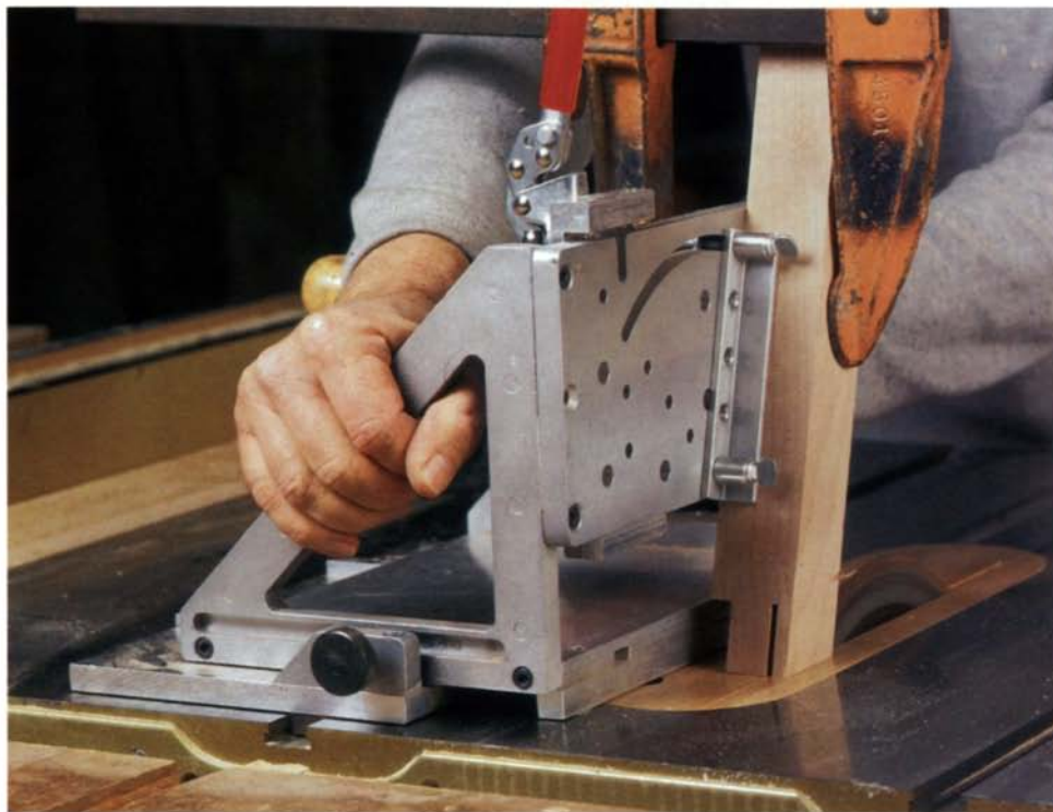
The Shop Fox holds stock for either horizontal or vertical cutting and milling.
