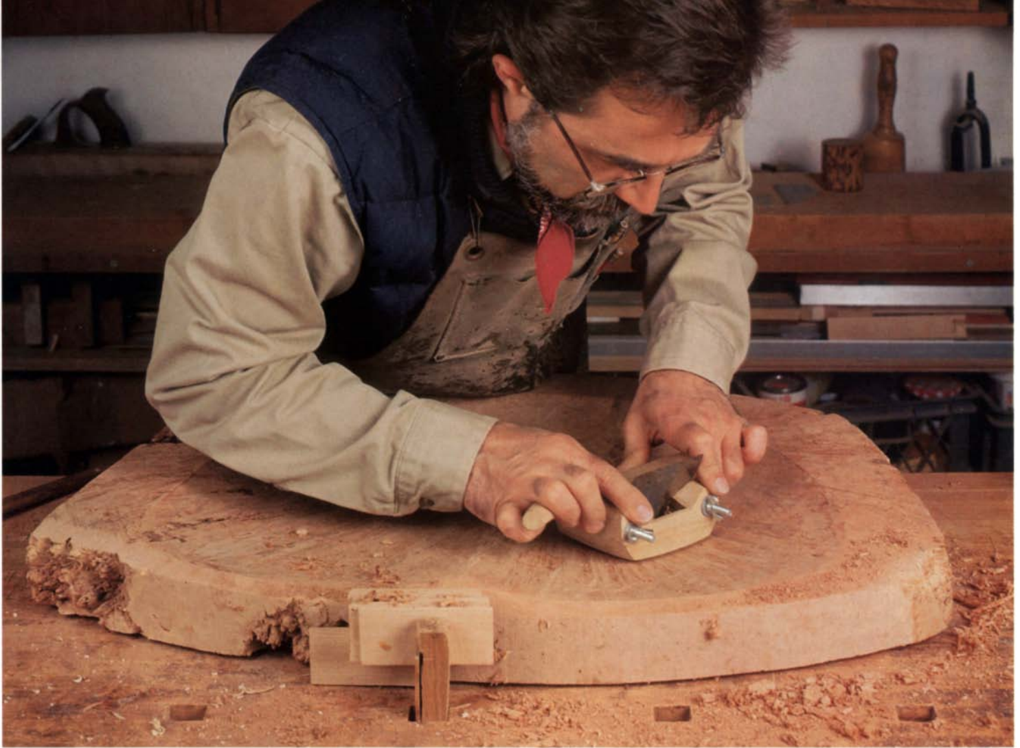
Wooden-bodied buckhorn scrapers take only a few hours to make and can be shaped to fit the curves of any project.
