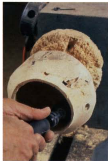
A flexible shaft will reach inside. This homemade tool (a drill chuck holding a sanding drum on the end of a flexible shaft) makes shaping and cleaning out the inside surfaces easier.
