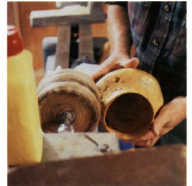
Polishing to a final luster— After several coats of mineral oil and hand-rubbed brushing lacquer applications, the author buffs each piece with tripoli polish applied to a set of heavily oiled cotton pads. He recommends an occasional coat of mineral oil to refresh an aging finish.
