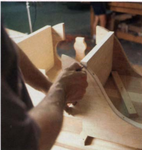
Scribe the curve on the center wall using the scroll-board template.
