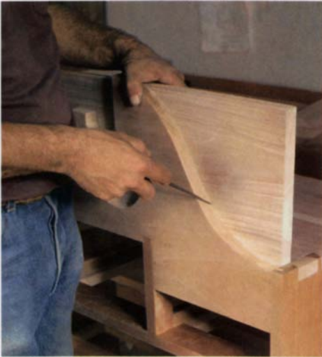
Trace the curve of the scroll board onto stock for the rear framing member.
