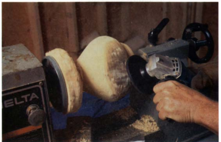
Grinding as an intermediate step —After rough-shaping with the gouge and before sanding to a final smooth shape, the author sometimes uses a grinder with 60-grit paper to remove deep pits and to refine the shape of a vessel.
