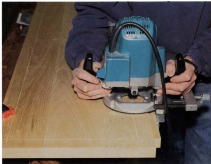
A router cuts the grooves. A \frac{1}{16} -in. straight bit and an edge guide on the router help make grooves of uniform depth. They still must be cleaned up.
