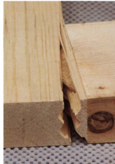
Every joint failure began at the end grain of the rail and split through the joint. In failure, all the biscuit joints looked similar.
