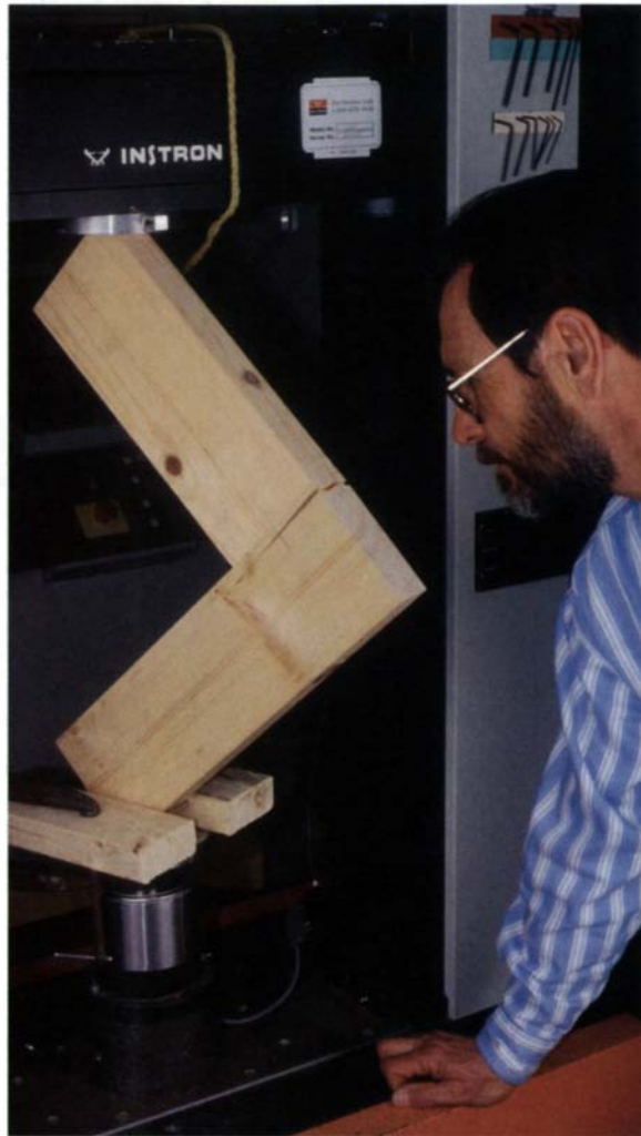
A 20,000-lb. computer-controlled press, owned by the Department of Energy, was used to test the strength of biscuit and loose-tenon joints in ponderosa pine.
