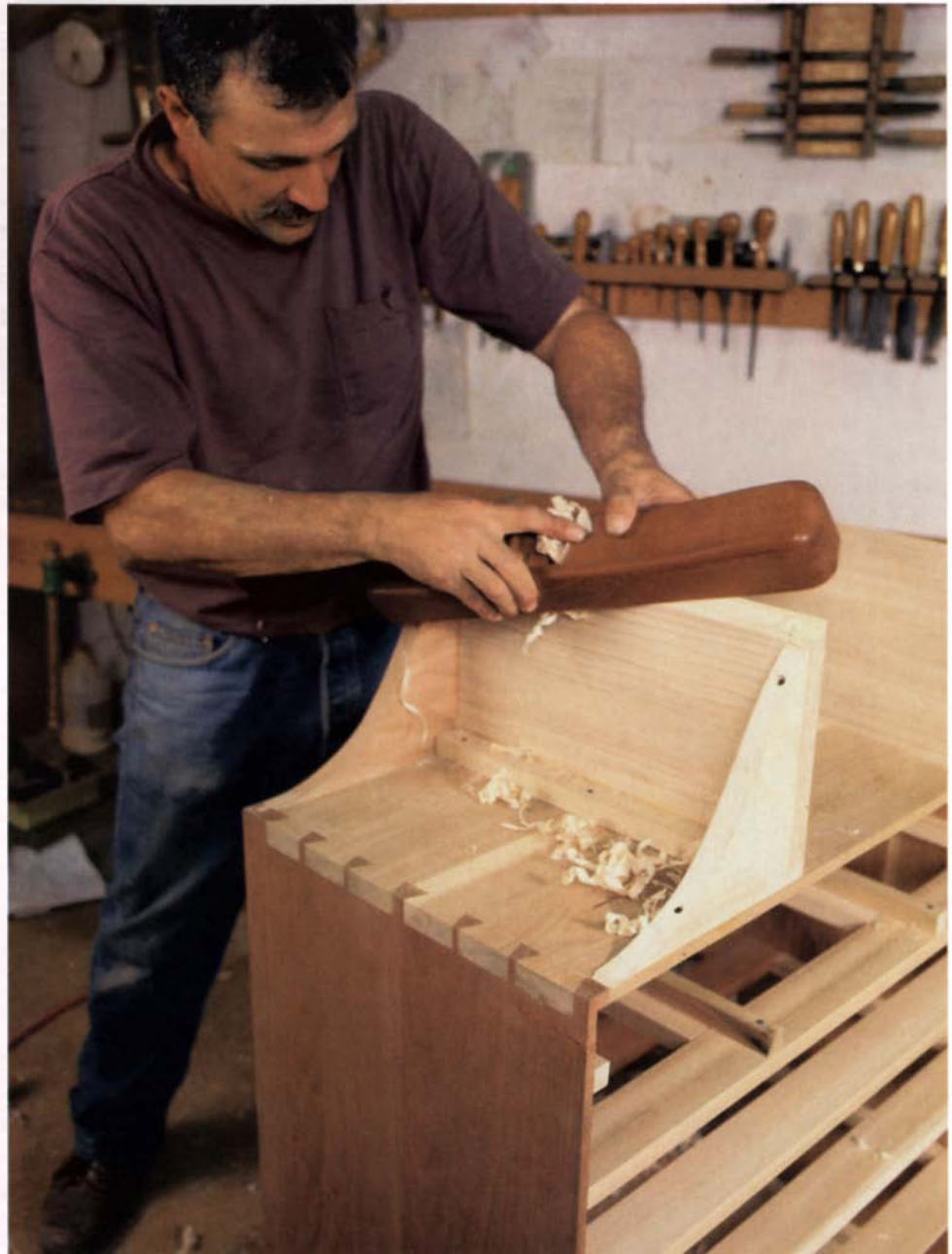
Fair the center walls to the scroll curve. Using a handplane, the author works from front to rear to prevent chipping the scroll board.
