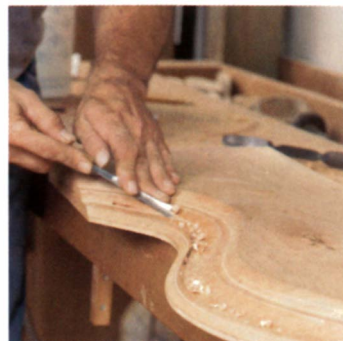
Use a gouge that matches the cove radius. The router-cut blank leaves guide marks for the width and depth of the cove.
