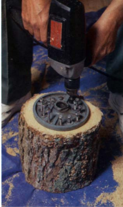
No such thing as overkill —When mounting a decayed piece on the lathe, the author drives a dozen or more 1½-in.-long lag screws through the faceplate into a small log of sweet gum.
