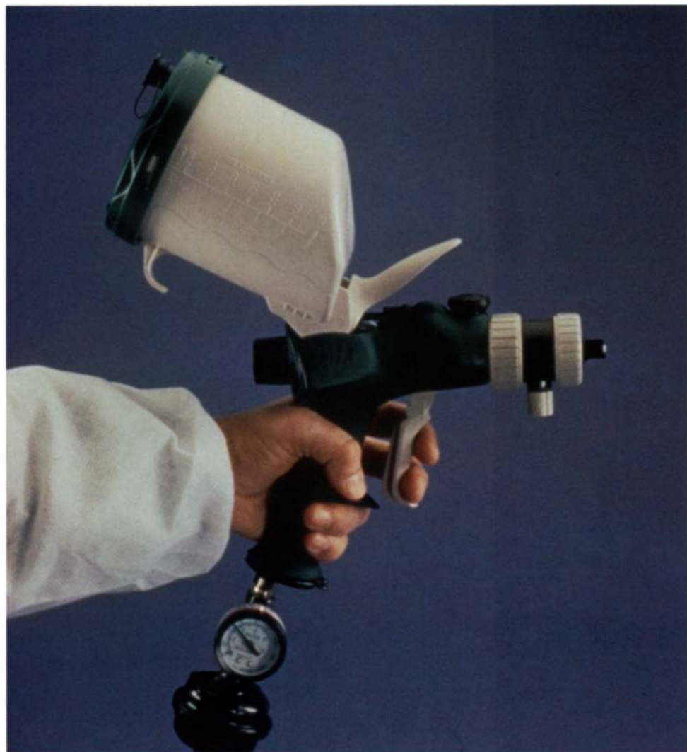
DeVilbiss OMX spray gun has a gravity-fed fluid cup and two triggers. The trigger on top of the gun is used when spraying horizontal surfaces.
